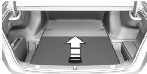
3. Stow the covers of the side storage compartments under the cargo floor panel in the respectively provided recesses.
