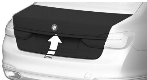
Press button on the exterior of the tailgate. This corresponds with pressing the button
