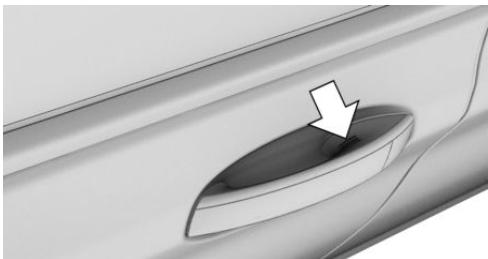
Touch the grooved surface on the handle of a closed vehicle door with your finger and hold it there without grasping the door handle.
