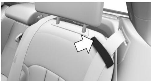
When fastening the safety belts on the rear seats, make sure that the belt guide loop is closed.
