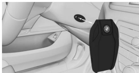
1. Hold the display key with its back against the marked area on the steering column.
