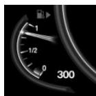
An arrow beside the fuel pump symbol shows which side of the vehicle the fuel filler flap is on.
