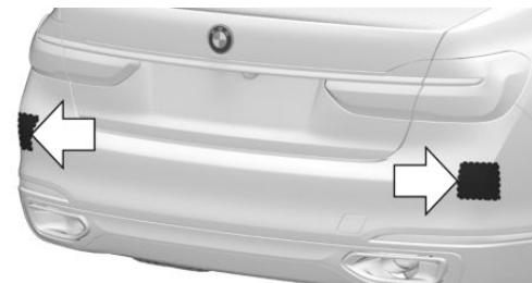
The radar sensors are located in the rear bumper.
