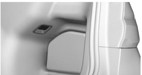
A socket is located on the right side in the cargo area. Unfold the cover.
