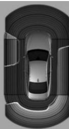
To protect the sides of the vehicle, obstacle markings are displayed on the vehicle at the sides.
