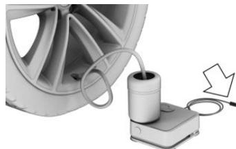
6. With standby state switched on or the engine running, switch on the compressor.
