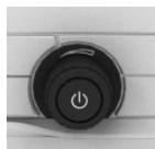
Hold button down until the OFF indicator on the instrument cluster goes out.
