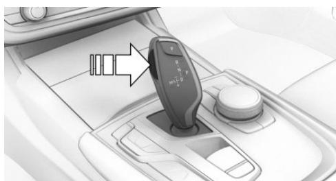
2. With the driver's safety belt fastened, briefly push the selector lever in the desired direction, past a resistance point, if needed. The selector lever automatically
