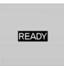
When the drive-ready state is switched on, READY is displayed in the instrument cluster.
