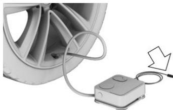
4. Correct the tire inflation pressure to at least 2.0 bar.
