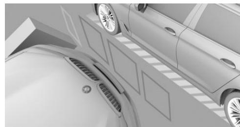
To protect the sides of the vehicle, obstacle markings are displayed on the vehicle at the sides.
