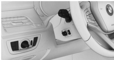
The light switch element is located next to the steering wheel.
