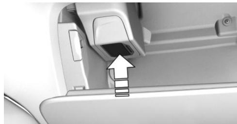
3. Remove the cover of the fragrance cartridge. Hold the cover on the top to slide it from the fragrance cartridge.
