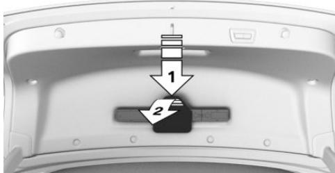
The warning triangle is located on the inside of the tailgate.
