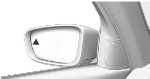
The light in the exterior mirror flashes if vehicles are detected by the rear sensors and your own vehicle is moving backwards.
