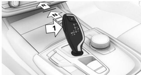
4. Release Start/Stop button and selector lever.
