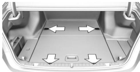
There are four lashing eyes in the cargo area for securing cargo.
