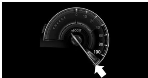
If the electric motor supports the combustion engine, e.g., during rapid acceleration, eBOOST, refer to page 114, is displayed. Depending on the available charge state of the high-voltage battery, there could be more or less eBOOST available. If the charge state of the high-voltage battery is low, eBOOST may not be available.
