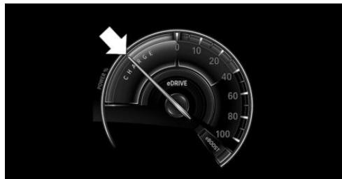
Energy recovery during coasting and braking is indicated as CHARGE in the instrument cluster depending on the driving mode, see arrow. The high-voltage battery is charged. If the high-voltage battery is completely charged, no energy can be recovered.
