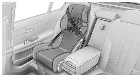
The safety belts in the rear and the front passenger safety belt can be permanently locked to fasten child restraint systems.
