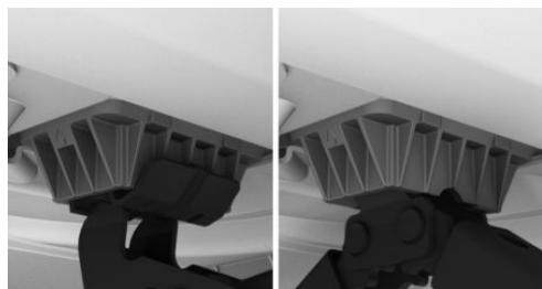
3. Extend the vehicle jack by turning the vehicle jack crank or lever clockwise.
