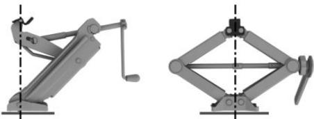
6. Make sure that the vehicle jack foot stands vertically and perpendicularly beneath the jacking point after extending the vehicle jack.
