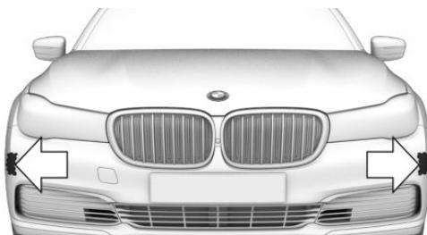
With the respective equipment variant, there are two additional radar sensors in the front bumper.
