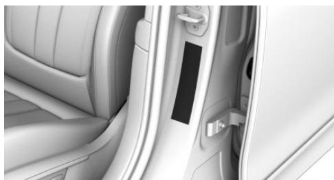
These pressure values can also be found on the tire inflation pressure label on the driver's door pillar.
