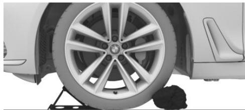
Place wheel chocks or other suitable objects in front and behind the wheel that is diagonal to the wheel to be changed.
