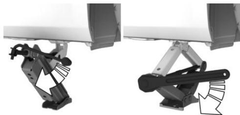
4. Take your hand away from the vehicle jack as soon as the vehicle jack is under load and continue turning the vehicle jack crank or lever with one hand.
