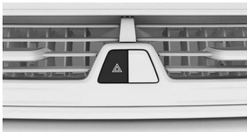
The button is located in the center console. The red light in the button flashes when the hazard warning flashers are activated.
