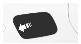
2. Open the fuel filler cap counterclockwise.
