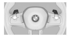
The shift paddles for the Sport Boost function are located on the steering wheel.
