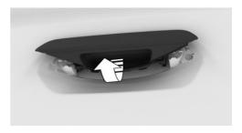
2. The position of the integrated key in the door lock depends on the vehicle. Unlock the door lock with the integrated key by turning it counterclockwise.
