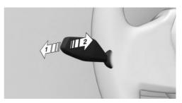
Press the turn signal lever forward, arrow 1, or pull the turn signal lever backward when the high-beam headlights are switched on, arrow 2.
