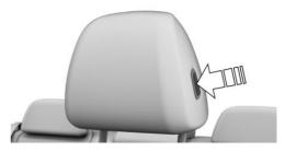
Press the button and push the head restraint up or down.
