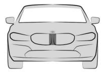
The front camera is located in the radiator arille.
