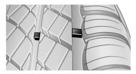
The tire manufacturer's wear indicators are distributed around the tire circumference and have a height of at least 0.06 in/1.6 mm.
