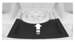
Slightly lift the storage tray with the wheel change set and emergency wheel and pull it to the back.
