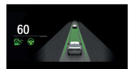
An example of active Driver Assistance: Indicator and warning lights for Distance Control and Assisted Driving Mode are displayed. At the same time, the Distance Control is animated in Assisted View.
