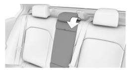
Pull lever and fold the center section forward.
