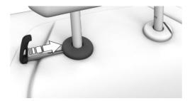
Press and hold the integrated key and the button at the same time, arrows 1, and pull out the head restraint completely.
