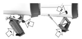
Insert the jack into the rectangular recess of the jacking point closest to the wheel to be changed.
