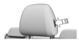
Press the button and push the head restraint forward or backward.
