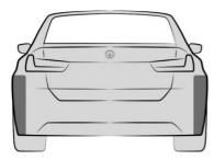
The radar sensors are located on the side of the rear bumper.
