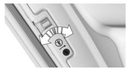
Unlock or lock the safety switch on the rear doors using the integrated key. To lock, turn in the corresponding arrow direction on the door.
