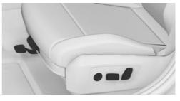
The lever and switches for adjusting the seats are located on the front seats.
