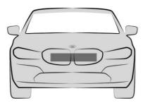
The front radar sensor is located in the radiator grille.
