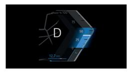
The efficient range of the power gauge is colored blue. Additionally, the bonus range will be displayed.
