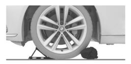
Place chocks or other suitable objects in front and behind the wheel that is diagonal to the wheel being changed.
