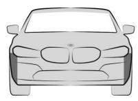
The radar sensors are located on the side of the front bumper.
