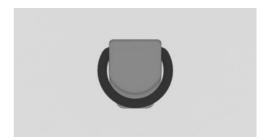
The lashing eyes are located in the cargo area.
