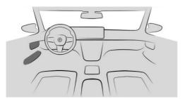
The seat adjustment menu button is located on the front door.
