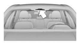
The cameras behind the windshield are located near the interior mirror.
