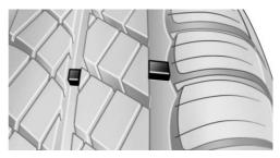
Distributed over the tire circumference are the tire manufacturer's wear indicators with a height of at least 0.06 in/1.6 mm, which serve as an indicator of tire tread wear.
