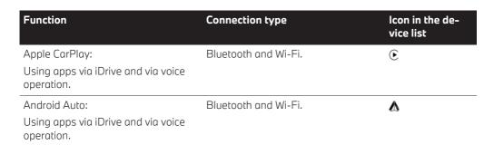
The following connection types require onetime pairing with the vehicle:
