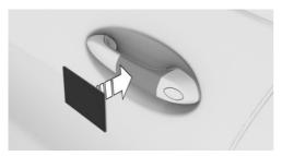
Hold activated Key Card directly on the center of the external door handle of the driver's door. If the Key Card is not detected, slightly change the position of the Key Card and repeat the procedure.
