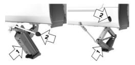
2. Insert the jack into the rectangular recess of the jacking point closest to the wheel to be chanaed.
