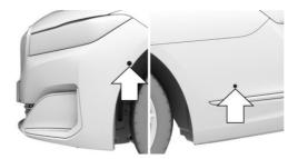
The ultrasonic sensors for Parking Assistant are located to the side in the front and rear bumpers.
