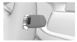
Turn the thumbwheel on the wiper lever.
