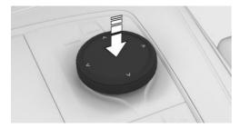
▶ Tilt in four directions to switch between displays, for example.
