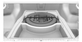
The emergency wheel and the wheel change tools are located in the cargo area under the cargo floor panel.
