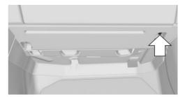
Release mounting, arrow, and carefully bend the trim panel down on the right side.
