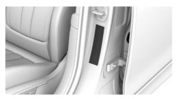
These pressure values can also be found on the tire pressure label on the driver's door pillar.
