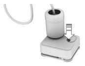
Let the compressor run for a maximum of 10 minutes to fill the tire with sealant and reach a tire pressure of approx. 2 bar.
