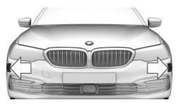
The radar sensors are located to the side in the front bumper.
