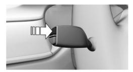
2. Press and hold the button on the turn signal lever.
