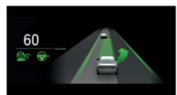
An example: the indicator and warning lights for the Active Cruise Control with Stop&Go function and the Automatic Lane Change Assistant indicate a lane change to the next lane. At the same time, the lane change to the next lane is shown with animation in the Assisted Driving View.
