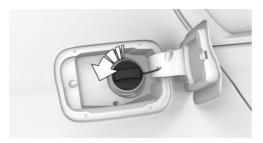
3. Place the fuel cap in the bracket attached to the fuel filler flap.
