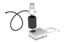
4. Screw the filler hose of the sealant bottle onto the tire valve of the faulty wheel.
