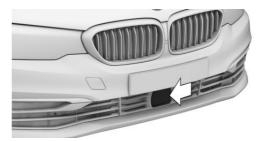
The front radar sensor is located in the front bumper.
