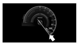
If the electric motor supports the combustion engine, for instance during rapid acceleration, eBOOST, refer to page 125, is displayed. Depending on the available charge state of the high-voltage battery, there could be more or less eBOOST available. If the charge state of the high-voltage battery is low, eBOOST may not be available.
