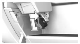
Insert the fragrance cartridge without pressure into the cartridge holder. The cartridge snaps lightly into place.
