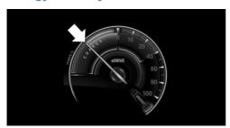
Energy recovery during coasting and braking is indicated as CHARGE in the instrument cluster depending on the driving mode, see arrow. The high-voltage battery is charged. If the high-voltage battery is completely charged, no energy can be recovered.
