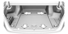
There are four lashing eyes in the cargo area for securing cargo.
