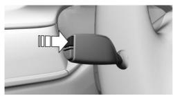
Press the button on the turn signal lever. Information is displayed in the instrument cluster. Pressing the button repeatedly displays additional information.
