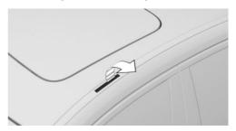
The fixing points are located in the roof drip rail above the doors.
