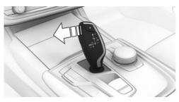
Press the selector lever to the left from selector lever position D.
