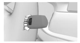
Turn the thumbwheel on the wiper lever.
