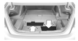
4. Lift the cargo floor panel by its handle towards the back and up and lower it.
