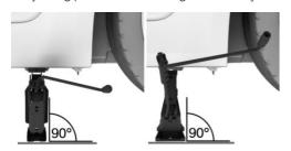
Crank the vehicle up, until the vehicle jack is with the entire surface on the ground and the relevant wheel is maximum 1.2 inches/3 cm above ground.
