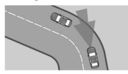
When the desired speed is too high for a curve, the speed is reduced slightly. Because curves may not be anticipated in advance, drive into a curve at an appropriate speed.
