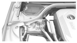
The starting aid terminal in the engine compartment acts as the battery's positive terminal. Open the cover of the starting aid terminal.
