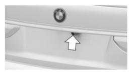
The camera lens is located in the handle of the trunk lid.
