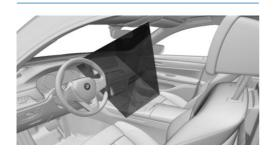
The gestures that are performed underneath the interior mirror are captured by a camera in the roofliner.
