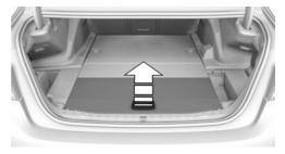
3. Stow the covers of the side storage compartments under the cargo floor panel in the respectively provided recesses.
