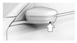
One camera is located at the bottom of each exterior mirror housing.
