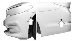
With the four side ultrasound sensors, arrows, and the ultrasound sensors of PDC Park Distance Control in the bumpers, the parking
