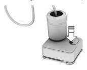
Let the compressor run for max. 10 minutes to fill the tire with sealant and achieve a tire inflation pressure of approx. 2.0 bar.
