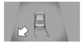
In the PDC Park Distance Control view, the respective boundary area flashes red, if vehicles are detected by the sensors.
