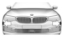
Depending on the vehicle equipment, two additional radar sensors are located in the front bumpers.
