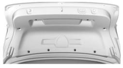
Reach into the handle recess on one side and carefully pull the interior trim downward, arrow 1, to the point where the two holding pins, arrows 2, behind the interior trim are released.
