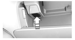
Remove the cover of the fragrance cartridge. Hold the cover on the top to slide it from the fragrance cartridge.
