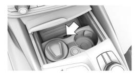
A USB interface is located in the center console. Properties:
