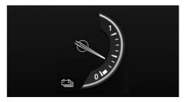
The Onboard Computer in the instrument cluster, refer to page 154, can also indicate the charge state of the high-voltage battery.
