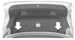
Press against the interior trim, arrows, so that the four holding pins engage in the trunk lid.
