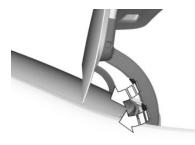
2. On the expanding rivet, carefully pry out the inside pin by a small distance using a screwdriver. Then carefully pry out the expanding rivet all the way using the screwdriver.
