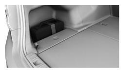
The onboard vehicle tool kit is located in the left storage compartment of the cargo area, under or next to the charging cable.
