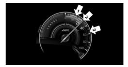
In ePOWER mode, the range for electric driving is colored blue, arrow 1. The range highlighted in blue can vary depending on the driving situation and eDRIVE mode.
