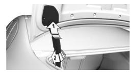
6. Fasten the hinge cover using the expanding rivet, arrow 1, and press onto the hinge cover
