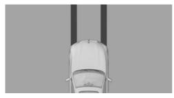
The vehicle wash view assists when entering a vehicle wash by displaying the floor and the vehicle's own track.
