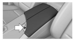
The storage compartment in the armrest can be locked with an integrated key to separately secure the tailgate, refer to page 44, e.g.
