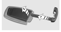
3. Using a pointed object, press battery in direction of arrow and lift it out.
