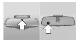
Photocells are used for control:
