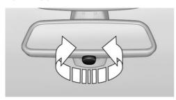
Turn the knob to reduce the blinding effect by the interior mirror.
