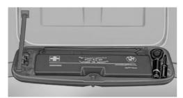
The onboard vehicle tool kit is located in a fold-down cover in the tailgate.
