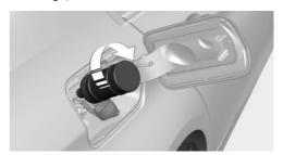
Press the bottle down, see arrow.The vehicle tank will be filled.
