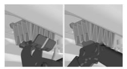
Extend the vehicle jack by turning the crank clockwise.
