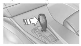
To release the lock: press button, arrow.
