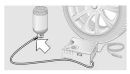
4. Insert the sealant container on the compressor housing in an upright position.
