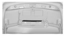
The warning triangle is located in the container on the inside of the tailgate.
