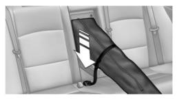
Tighten the retaining strap.
