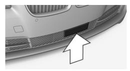
Always keep radar sensor clean and unobstructed.
