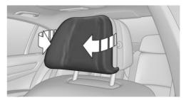
Fold the side extensions on the head restraint forward for increased lateral support in the resting position.
