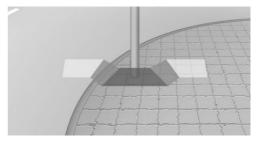
Obstacle markings can be faded into the image of the rearriew camera.
