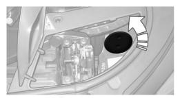
Unscrew the bulb holder counterclockwise.
