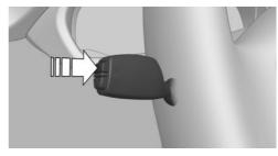
Press and hold button on signal lever.
