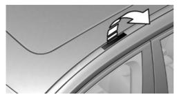
The anchorage points are located in the roof drip rail above the doors.
