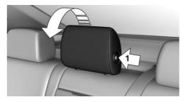
Press button, arrow 1, and fold the head restraint forward.
