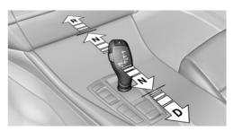
With the driver's safety belt fastened, tap the selector lever in the desired direction, beyond a resistance point, if needed.
