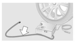
Screw the connection hose onto the connector of the sealant container.
