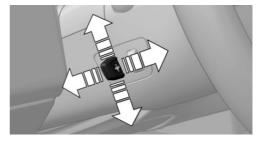
Press the switch to move the steering wheel to the preferred height and angle to suit your seating position.
