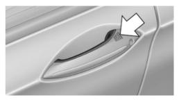
Touch the surface on the handle of a vehicle door, arrow, with your finger and hold it there without grasping the door handle.
