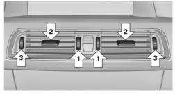
➤ Thumbwheels to vary the ventilation temperature in the upper body region, arrow 1.
