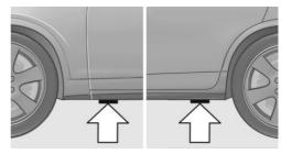
The jacking points for the vehicle jack are located at the positions shown.
