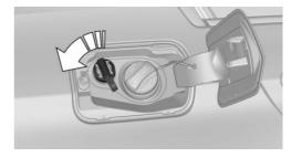
The fuel cap for diesel exhaust fluids is next to the fuel cap for the fuel tank.
