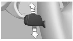
With the ignition switched off, press the lever either up or down past the resistance point for approx. 2 seconds.
