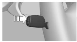
Press and hold button on signal lever.
