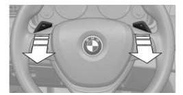
The shift paddles on the steering wheel allow you to shift gears quickly while keeping both hands on the steering wheel.
