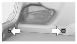
There are four lashing eyes in the cargo area for securing cargo.
