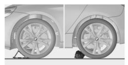
If a wheel needs to be changed on a slight down-hill grade, place wheel chocks or other suitable objects, e.g. a stone, under the wheels of the front and rear axle.
