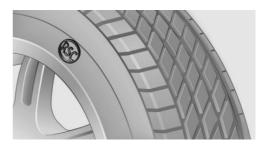
RSC label on the tire sidewall.
