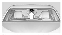
The camera is installed near the interior mirror.
