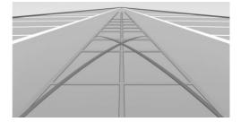
Turn the steering wheel to the point where the pathway line covers the corresponding turning radius line.
