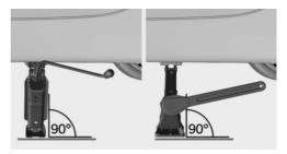
Crank up the vehicle jack until the entire surface of the jack is in contact with the ground and the wheel in question is raised a maximum of 1.2 inches/3 cm off the ground.
