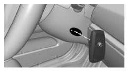
Hold the remote control with its back against the marked area on the steering column. 2. Start the engine within 10 seconds.
