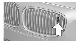
The camera is automatically heated when the external temperatures are low.
