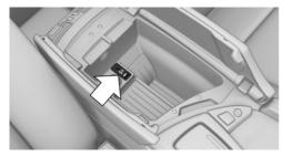
The USB interface and the AUX-IN port are located in the center armrest.
