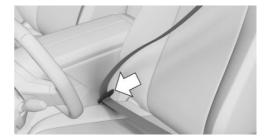
To ease accessibility to the seat belt buckle, an adjustable slider is available on the belt to help position the buckle when not in use.
