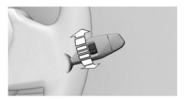
Turn the thumbwheel on the wiper lever.
