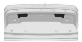
Depending on the equipment: pull down the trunk lid with the recessed grips.
