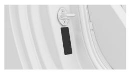
The vehicle identification number can be found on the nameplate, on the right-hand side of the vehicle.
