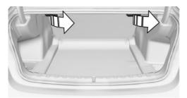
Pull the corresponding lever in the cargo area to release the rear seat backrest.
