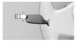
2. Press and hold the button until the values are reset.
