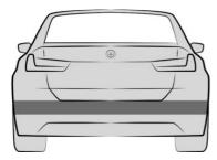
The ultrasonic sensors of the parking assistance systems are located in the rear bumper.
