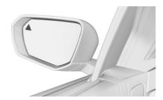
The warning light in the exterior mirror warns of a possible collision.
