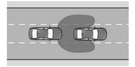
Radar sensors monitor the area behind the vehicle.
