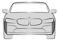
The radar sensors are located to the side in the front bumper.
