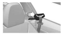
The seat-belt extender extends automatically and keeps the seat belt ready to put on, arrow. After the belt is put on, it goes back into the resting position.
