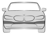
The ultrasonic sensors of the parking assistance systems are located in the front bumper.
