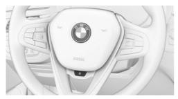
Button for steering wheel heating
