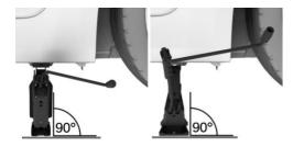
7. Crank the vehicle up until the vehicle jack has the entire surface on the ground and the relevant wheel is maximum 1.2 inches/3 cm above ground.
