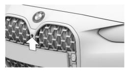
The front camera is located in the radiator arille.
