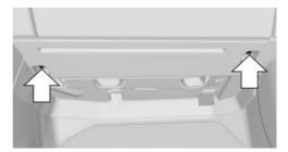
Loosen fasteners, arrows, and open cover.
