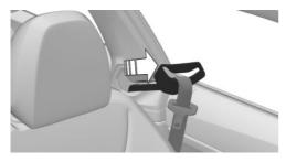
The seat-belt extender extends automatically and keeps the seat belt ready to put on, arrow. After the belt is put on, it goes back into the resting position.
