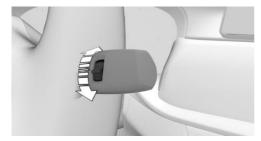
Turn the thumbwheel on the wiper lever.
