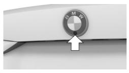
The camera is located in the nameplate of the trunk lid.
