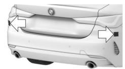
The radar sensors are located in the bumper.
