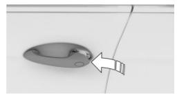
2. Guide one finger of your other hand from the back under the cover and push the cover out. Use the thumb for counter support to prevent the cover from falling out of the door handle.
