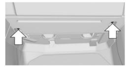
Loosen fasteners, arrows, and open cover.
