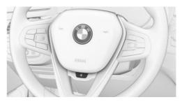
Button for steering wheel heating
