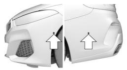
The ultrasound sensors of the Automatic Parking Assistant are located on the side of the vehicle.
