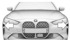
The radar sensors are located in the bumper.
