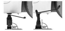
7. Crank the vehicle up, until the vehicle jack is with the entire surface on the ground and the relevant wheel is maximum 1.2 inches/3 cm above ground.
