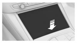
2. A socket is located between the cup holders. Pull off the cover.
