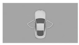
Steptronic transmission: the maximum opening angles of the doors are displayed in selector lever position P. As soon as the vehicle begins moving, the opening angles are replaced by parking aid lines.
