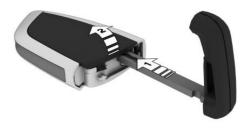
3. Push battery in arrow direction using a pointed object and lift it out.
