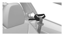
The seat-belt extender extends automatically and keeps the safety belt ready to put on, arrow. After the belt is put on, it goes back into the idle position.
