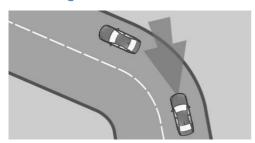
When the set speed is too high for a curve, the speed is reduced slightly. Because curves may not be anticipated in advance, drive into a curve at an appropriate speed.
