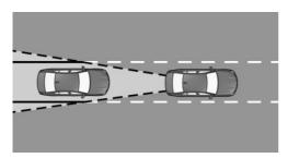
Radar sensors monitor the area behind the vehicle.
