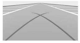
Turning circle lines can only be superimposed on the camera image together with lanes. Turning circle lines show the course of the smallest possible turning radius on a level road.
