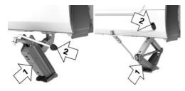
2. Insert the vehicle jack into the rectangular recess of the jacking point closest to the wheel to be changed.
