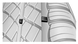
Wear indicators are distributed around the tire circumference. These wear indicators have the legally required minimum height of 0.063 in/1.6 mm.
