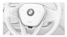
Button for heated steering wheel
