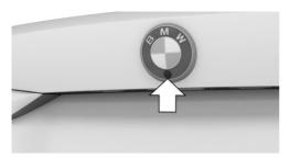
The camera lens is located in the nameplate of the trunk lid.
