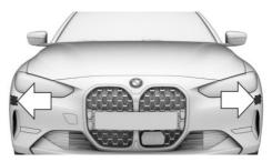
Depending on the vehicle equipment, two additional radar sensors are located in the front bumpers.
