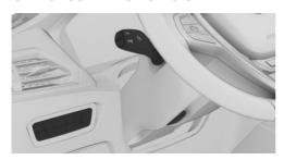
The light switch element is located next to the steering wheel.
