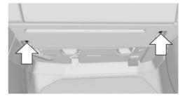
Loosen fasteners, arrows, and open cover.
