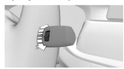
Turn the thumbwheel on the wiper lever.
