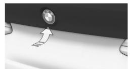
Press the button on the exterior of the trunk lid.
