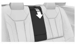
Pull lever and fold the center section forward.
