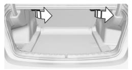
Pull the corresponding lever in the cargo area to release the rear seat backrest.
