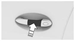
Hold the near field communication antenna of the smartphone directly and centered on the outside door handle of the driver's door.
