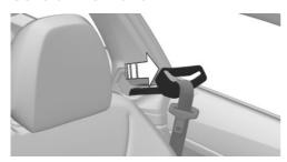
The seat-belt extender extends automatically and keeps the safety belt ready to put on, arrow. After the belt is put on, it goes back into the idle position.
