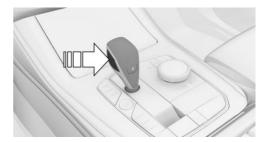
Push the selector lever in the desired direction, past a resistance point, if needed. The selector lever automatically returns to the center position when released.
