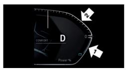
Pointer in the area of arrow 1: display of the energy recovered by coasting or when decelerating, CHARGE.
