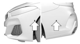
With the four side ultrasound sensors, arrows, and the ultrasound sensors in the bumpers, the parking spaces are measured and the distances to obstacles determined.
