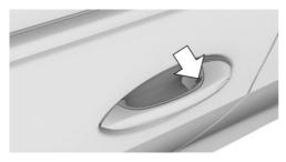
Touch the grooved surface on the handle of a closed vehicle door with your finger and hold it there without grasping the door handle.
