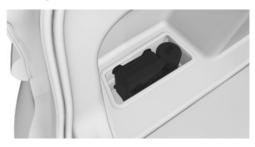
The Mobility System is located in a bag in the left storage compartment of the cargo area. Release the tensioning strap to remove.
