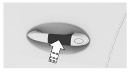
Hold activated key card directly and centered on the outside door handle of the driver's door.
