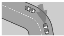
When the desired speed is too high for a curve, the speed is reduced slightly. Because curves may not be anticipated in advance, drive into a curve at an appropriate speed.
