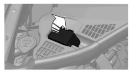
The starting aid terminal in the engine compartment acts as the battery's positive terminal.
