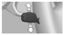
With radio-ready state switched off, press the lever either up or down past the resistance point.
