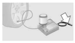
7. With the ignition switched on or the engine running, switch on the compressor.
