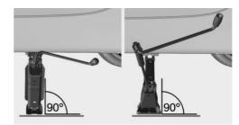
7. Crank up the vehicle jack until the entire surface of the jack is in contact with the ground and the wheel in question is raised a maximum of 1.2 inches/3 cm off the ground.
