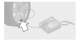
3. Attach the connection hose directly to the compressor.
