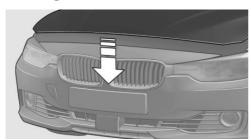
Let the hood drop from a height of approx. 16 inches/40 cm and push down on it to lock it fully. The hood must engage on both sides.
