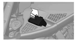
The starting aid terminal in the engine compartment acts as the battery's positive terminal. Open the cover of the starting aid terminal.
