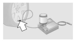
6. With the compressor switched off, insert the plug into a power socket inside the vehicle.
