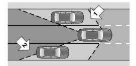
Two radar sensors in the rear bumper monitor the area behind and next to the vehicle at speeds above approx. 30 mph/50 km/h.
