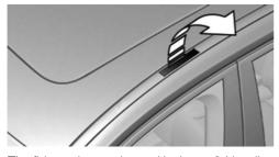
The fixing points are located in the roof drip rail above the doors.
