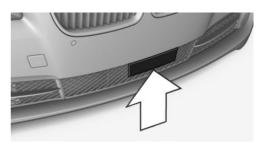
Always keep radar sensor clean and unobstructed.
