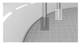
Depending on the vehicle equipment, obstacle markings can be faded into the image of the rearriew camera.
