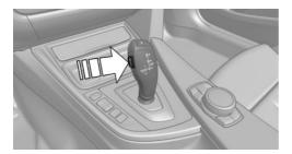
2. With the driver's safety belt fastened, briefly push the selector lever in the desired direction, past a resistance point, if needed. The selector lever automatically returns to the center position when released.
