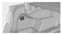
The socket is located on the left side in the cargo area.
