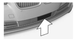
Always keep radar sensor clean and unobstructed.
