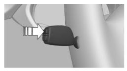
Press and hold button on signal lever.
