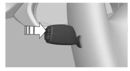
Press and hold button on signal lever.
