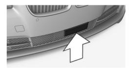
Always keep radar sensor clean and unobstructed.
