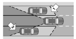
Two radar sensors in the rear bumper monitor the area behind and next to the vehicle at speeds above approx. 30 mph/50 km/h.
