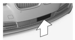
Always keep radar sensor clean and unobstructed.
