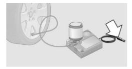
7. With the ignition switched on or the engine running, switch on the compressor.
