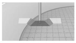
If the vehicle is equipped accordingly, obstacle markings can be faded into the image of the rearview camera.
