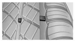
Wear indicators are distributed around the tire's circumference and have the legally required minimum height of 0.063 inches/1.6 mm.
