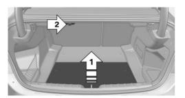
Raise the cargo floor panel, arrow 1, and latch at top, if needed, arrow 2.
