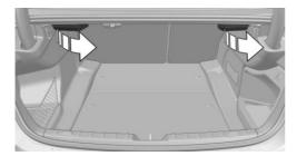
The unlocked rear seat backrest moves forward slightly.
