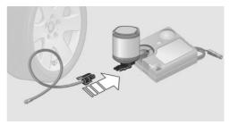
Slide the sealing container upright into the holder on the compressor housing, ensuring that it engages audibly.
