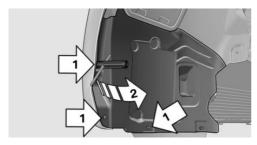
2. Pull off the bulb connector, arrow 1.
