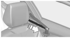
After the door is closed and the vehicle key has been detected in the vehicle's interior, the belt carrier extends automatically and keeps the safety belt ready to put on, arrow. After the belt is put on, it goes back into the idle position.
