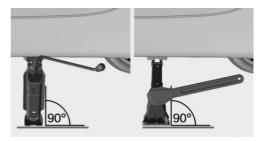
Crank up the vehicle jack until the entire surface of the jack is in contact with the ground and the wheel in question is raised a maximum of 1.2 inches/3 cm off the ground.
