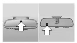
Photocells are used for control:
