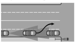
If a vehicle ahead of you unexpectedly moves into another lane from behind a stopped vehicle, you yourself must react, as the system does not react to stopped vehicles.
