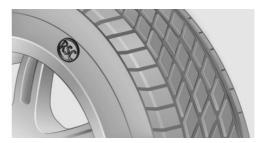
RSC label on the tire sidewall.
