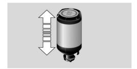
Take the connection hose completely out of the compressor housing. Do not kink the hose.
