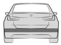
The ultrasonic sensors are located in the rear bumper.
