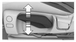
Pull the lever up or press it down as often as needed until the seat has reached the desired height.
