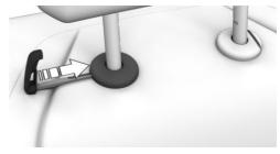
Press and hold the integrated key and the button at the same time, arrows 1, and pull out the head restraint completely.
