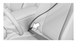
To ease accessibility to the seat belt buckle, an adjustable slider is available on the belt to help position the buckle when not in use.
