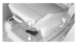
Pull the lever up or press it down as often as needed until the seat has reached the desired. inclination.
