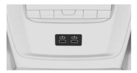
Depending on the equipment, there are two USB ports in the center console in the rear.
