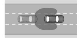
Radar sensors monitor the area behind the vehicle.
