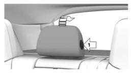
Press button, arrow 1, and fold the head restraint back.
