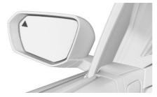
The warning light in the exterior mirror warns of a possible collision with a detected vehicle.
