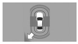
In the Park Distance Control view, the respective boundary area flashes red if vehicles are detected by the sensors.
