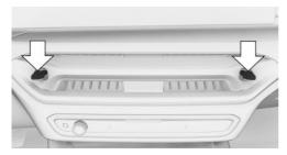
Setting the air flow direction and air volume at the vent.
