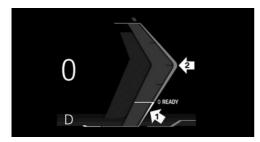
Needle in range of arrow 1: display for energy recovery such as while decelerating CHARGE. Needle in range of arrow 2: the drive power in percent, POWER.
