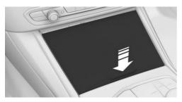
A socket is located between the cup holders. Detach the cover.
