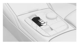
Pull the selector lever from selector lever position D to D/S.
