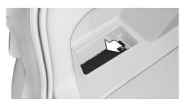
The on-board toolkit is located in the left storage compartment in the cargo area, under a cover.
