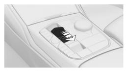
Pull the selector lever from selector lever position D to D/S.
