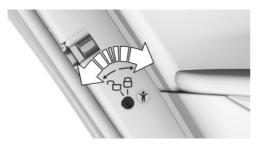
Unlock or lock the safety switch on the rear doors using the integrated key.
