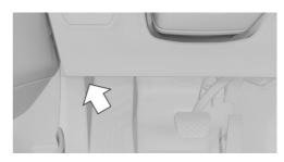
There is a diagnostic socket on the driver's side for reading out vehicle data.
