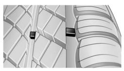
The tire manufacturer's wear indicators are distributed over the tire circumference. These indicators have a height of min. 0.06 in/1.6 mm. and serve as an indicator for tire tread wear.
