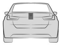
The regryiew camera is located in the handle strip on the rear of the vehicle.
