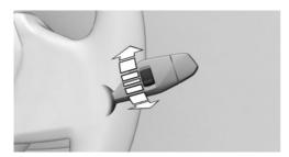
Turn the thumbwheel on the wiper lever.
