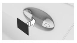
Hold activated Key Card directly on the center of the external door handle of the driver's door.
