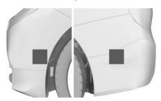
The ultrasonic sensors of the parking assistance systems are located on the side in the front and rear bumpers.
