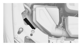
The engraved vehicle identification number can be found in the engine compartment, on the right-hand side of the vehicle.
