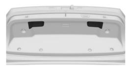
Depending on vehicle equipment: Pull down the trunk lid using the recessed grips.
