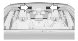
With climate comfort windshield: the marked area is not covered with heat-reflective coating.
