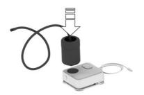
4. Screw the filler hose of the sealant bottle onto the tire valve of the faulty wheel.
