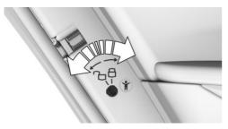
Unlock or lock the safety switch on the rear doors with the integrated key.
