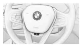
Button for steering wheel heating
