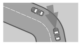
When the set speed is too high for a curve, the speed is reduced slightly. Because curves may not be anticipated in advance, drive into a curve at an appropriate speed.
