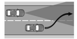
If a vehicle driving ahead of you suddenly merges into your lane, the system may not be able to automatically restore the selected distance. It may not be possible to restore the selected distance in certain situations, including if you are driving significantly faster than vehicles driving ahead of you, for instance when
