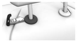
Press and hold the integrated key and the button at the same time, arrows 1, and pull out the head restraint completely.
