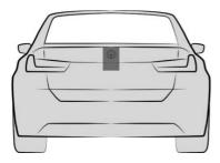
The regryiew camera is located in the handle on the rear end.
