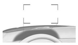
The protective glass of the Head-up display is located between the steering wheel and the windshield.
