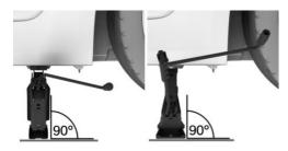
Crank the vehicle up until the vehicle jack has the entire surface on the ground and the relevant wheel is maximum 1.2 inches/3 cm above ground.
