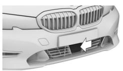
The radar sensor is located in the front bumper.
