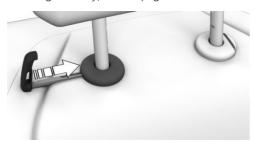
4. Press and hold the integrated key and the button at the same time, arrows 1, and pull out the head restraint completely.
