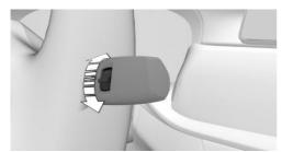
Turn the thumbwheel on the wiper lever.
