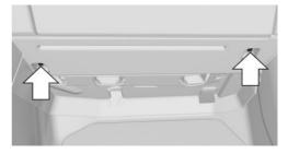
Loosen fasteners, arrows, and open cover.
