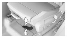
Pull the lever up or press it down as often as needed until the seat has reached the desired tilt
