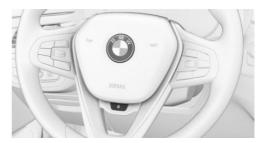
Button for heated steering wheel
