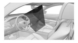
The camera in the roofliner detects gestures that are carried out in the area of the center console at the height of the Control Display.
