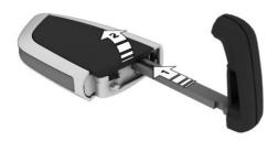
3. Push battery in the direction of the arrow using a pointed object and lift it out.
