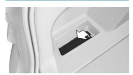
The onboard vehicle tool kit is located in the left storage compartment of the cargo area under a cover.
