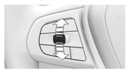
Press the rocker switch up or down once while the system is interrupted. The system will be activated.
