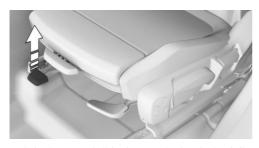
Pull the lever and slide the seat in the desired direction.
