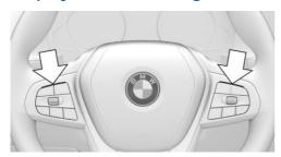
The two LED lights above the buttons illuminate analogously to the displays in the instrument cluster:
