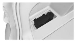
The Mobility System is located in a bag in the left storage compartment of the cargo area. Release the tensioning strap to remove.
