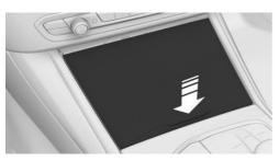
A socket is located between the cup holders. Pull off the cover.
