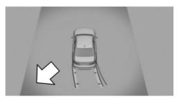
In the PDC Park Distance Control view, the respective boundary area flashes red, if vehicles are detected by the sensors.
