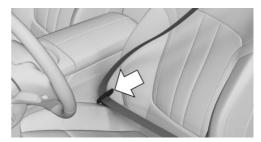
When the safety belt is fastened, the driver's and passenger's belt straps are automatically tightened once after driving away.
