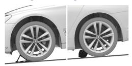
If you need to change a wheel on a slight downhill grade, place chocks and other suitable objects, for instance a rock, under the wheels of both the front and rear axles against the rolling direction.
