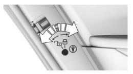
Unlock or lock the safety switch on the rear doors with the integrated key.
