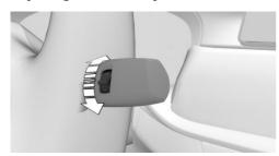
Turn the thumbwheel on the wiper lever.
