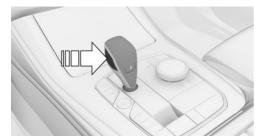
Push the selector lever in the desired direction, past a resistance point, if needed. The selector lever automatically returns to the center position when released.
