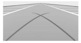
Turning radius lines can only be superimposed on the camera image together with pathway lines.
