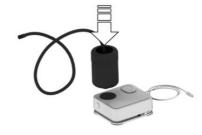
4. Screw the filling hose of the sealant container onto the tire valve of the nonworking wheel.
