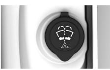
The washer fluid reservoir is located in the engine compartment.
