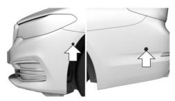
With the four side ultrasound sensors, arrows, and the ultrasound sensors of PDC Park Distance Control in the bumpers, the parking spaces are measured and the distances to obstacles determined.
