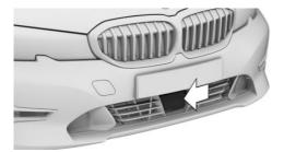
The radar sensor is located in the front bumper. Always keep radar sensor clean and unobstructed.
