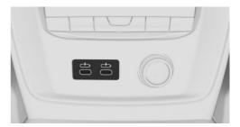
A USB interface with two USB ports is located in the center console in the rear.
