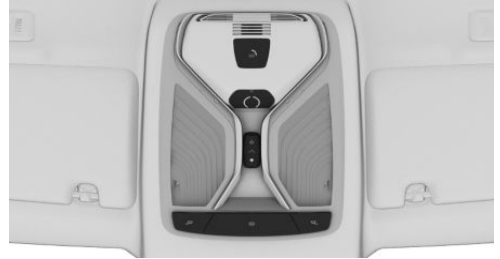
SOS button in the roofliner.
