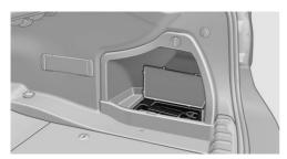
The onboard vehicle tool kit is located on the right side in the cargo area in a storage compartment. Open the cover.
