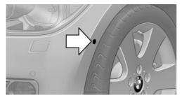
The four ultrasound sensors for measuring parking spaces are located in the front and rear on the side of the vehicle.
