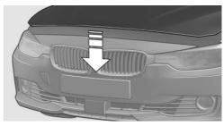
Let the hood drop from a height of approx. 16 inches/40 cm and push down on it to lock it fully.
