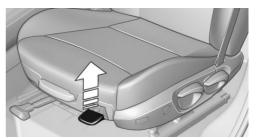
Pull the lever and move the seat to the desired tilt. After releasing the lever, apply your weight to the seat or lift it off to make sure the seat engages properly.
