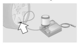
With the compressor switched off, insert the plug into a power socket inside the vehicle.
