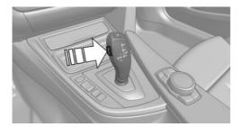
With the driver's safety belt fastened, briefly push the selector lever in the desired direction, past a resistance point, if needed. The selector lever automatically returns to the center position when released.
