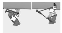
Take your hand away from the vehicle jack as soon as the vehicle jack is under load and continue turning the vehicle jack crank or lever with one hand. Make sure that the vehicle jack foot stands vertically and at a right angle beneath the jacking point.
