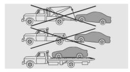
The vehicle should only be transported on a loading platform.
