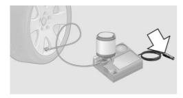
7. With the ignition switched on or the engine running, switch on the compressor.
