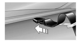
Push the corresponding head restraint down as far as it will go. 4. Pull the corresponding lever in the cargo area to release the rear seat backrest.
