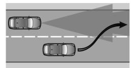
A vehicle driving in front of you is not detected until it is completely within the same lane as your vehicle.
