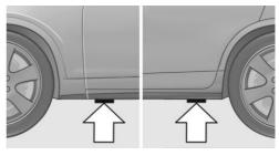
The jacking points for the vehicle jack are located at the indicated positions.
