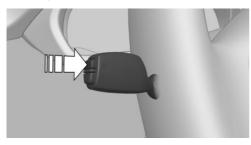
Press and hold button on signal lever.
