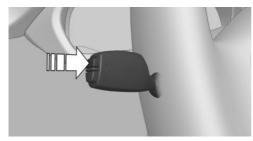
Press and hold button on signal lever.
