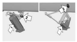
Insert the vehicle jack into the rectangular recess of the jacking point closest to the wheel to be changed.
