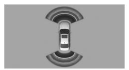
The approach of the vehicle to an object is shown on the Control Display. Objects that are farther away are already displayed on the Control Display before a signal sounds.
