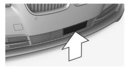
Always keep radar sensor clean and unobstructed.
