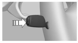
Press and hold button on signal lever.
