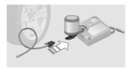
Slide the sealing container upright into the holder on the compressor housing, ensuring that it engages audibly.
