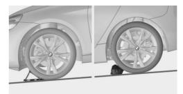
If you need to change a wheel on a slight downhill grade, place chocks and other suitable objects, for instance a rock, under the wheels of both the front and rear axles against the rolling direction.
