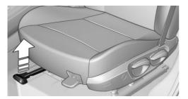
Pull the lever and slide the seat in the desired direction.
