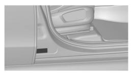
The vehicle identification number can be found on the type label, on the right-hand side of the vehicle.
