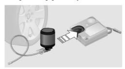
Remove the valve cap from the tire valve and screw the connection hose onto the tire valve of the nonworking wheel.
