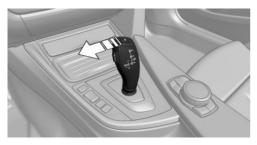
Press the selector lever to the left out of selector lever position D.
