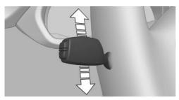
With radio-ready state switched off, press the lever either up or down past the resistance point.
