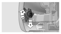
3. Insert the new bulb, connect the connector and screw on the wheel house panel.
