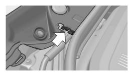
Press down on the holder and tighten the three screws.
