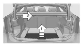
Raise the cargo floor panel, arrow 1, and latch at top, if needed, arrow 2.
