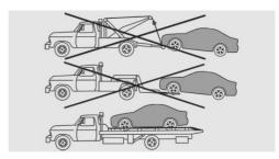
The vehicle should only be transported on a loading platform.
