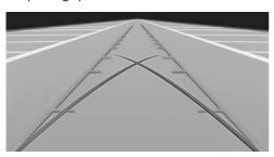
Turn the steering wheel to the point where the pathway line covers the corresponding turning radius line.
