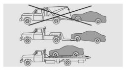
Your vehicle should be transported with a tow truck with a so-called lift bar or on a flat bed.
