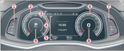
Fig. 2 Overview of instrument cluster (Audi virtual cockpit)
