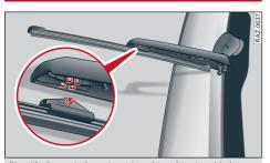
Fig. 49 Rear window wiper: Attaching the wiper blade
