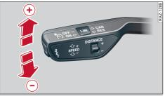
Fig. 137 Control lever: Setting a new speed
