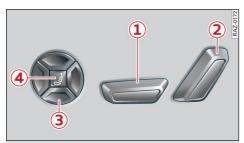
Fig. 51 Front seat: Buttons for seat adjustment
