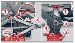
Fig. 227 Door sill: Applying the jack under the door sill
