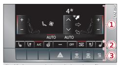
Fig. 95 Centre console: Lower display and row of buttons
