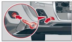
Fig. 232 Front bumper: Fitting the towline anchorage
