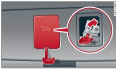
Fig. 31 Inside of boot lid: Access to manual release
