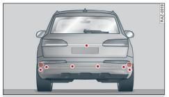
Fig. 126 Rear area: Sensors and cameras
