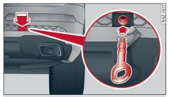
Fig. 233 Rear bumper: Fitting the towline anchorage
