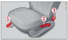
Fig. 50 Front seat: Adjuster controls
