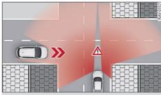
Fig. 156 Detected intersecting traffic
