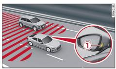
Fig. 152 Driving situation and warning signal on exterior mirror
