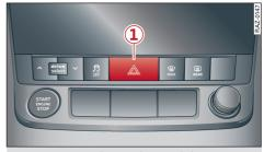
Fig. 37 Centre console: Hazard warning lights
