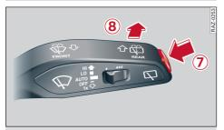
Fig. 47 Control lever: Rear window wiper
