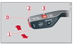
Fig. 136 Control lever: Operating adaptive cruise assist
