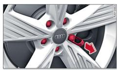
Fig. 223 Wheel: Wheel bolts with caps
