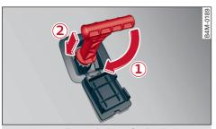
Fig. 103 Footwell: Manual release of parking lock
