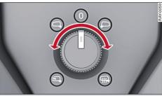
Fig. 41 Driver's door: Adjuster knob for exterior mirrors
