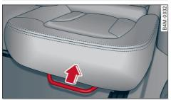
Fig. 55 Second row of seats: Adjusting the seat position
