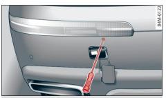
Fig. 242 Rear lights in left side of bumper: Loosening screw
