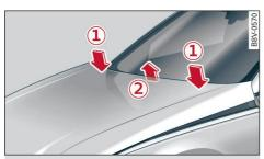
Fig. 205 Pressing back/checking the bonnet after system deployment
