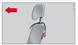
**Fig. 78** Rear backrest: Hooking strap into top tether anchorage
