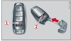
Fig. 26 Vehicle key: Removing battery holder
