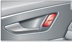
Fig. 21 Driver's door: Central locking switch
