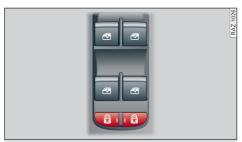
Fig. 32 Driver's door: Controls
