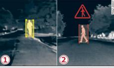
Fig. 131 Instrument cluster: Pedestrian highlighting and warning feature
