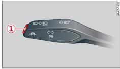
**Fig. 150** Turn signal lever: Button for lane departure warning and lane guidance function of adaptive cruise assist\*
