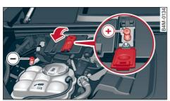
**Fig. 230** Engine compartment: Terminals for jump leads or battery charger
