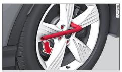
Fig. 225 Wheel: Loosening the wheel bolts
