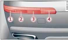
**Fig. 241** Rear lights: Overview of bulbs in left side of bumper
