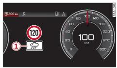
Fig. 129 Instrument cluster: Traffic sign recognition
