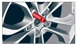
Fig. 229 Wheel: Mounting pin in wheel bolt hole nearest to the top
