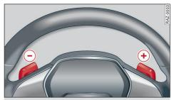
Fig. 102 Steering wheel: Paddle levers\*
