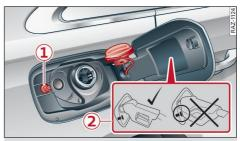
Fig. 202 Fuel tank flap with tank cap attached
