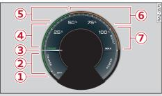
Fig. 6 Instrument cluster: Power meter
