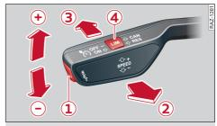
Fig. 132 Control lever: Switching the system on
