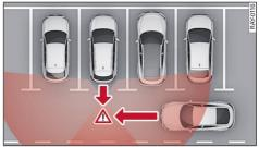
Fig. 165 Areas covered by sensors for rear cross-traffic as-
