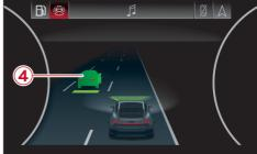
Fig. 144 Instrument cluster: Overtake prevention without or with surroundings shown
