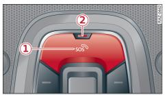
Fig. 177 Front headliner: Cover for emergency call button
