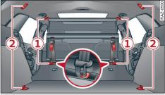
Fig. 87 Backrest folded down: Load guard
