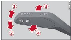
Fig. 36 Control lever: Switching light functions on/off
