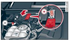
Fig. 213 Engine compartment: Terminals for jump leads or battery charger
