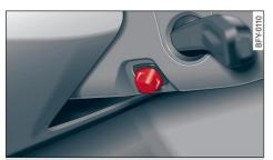
**Fig. 60** Steering column: Button for adjusting the steering wheel position
