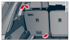
Fig. 56 Second row of seats: Folding the seat down
