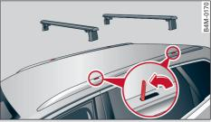
Fig. 94 Roof railing: Attachment points
