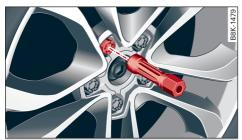
Fig. 228 Wheel: Hexagonal socket for turning wheel bolts
