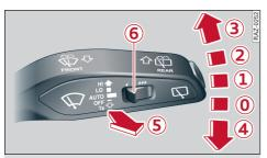
Fig. 46 Control lever: Windscreen wipers
