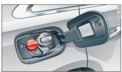
**Fig. 203** Vehicle as seen from the rear right: Unscrewing the AdBlue cap
