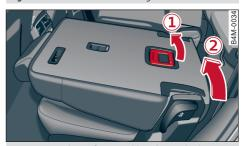
Fig. 57 Second row of seats: Folding the seat back up
