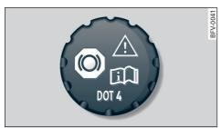
Fig. 212 Engine compartment: Cap of brake fluid reservoir
