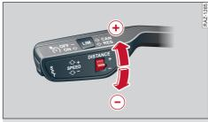
Fig. 142 Control lever: Setting the distance
