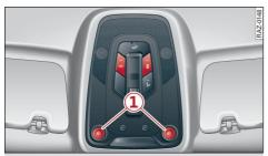
Fig. 38 Headliner: Interior lights
