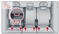
**Fig. 75** Rear seat bench in second row of seats: Bottom ISOFIX anchorages
