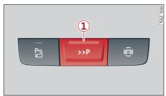
Fig. 170 Centre console: Button for park assist plus
