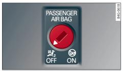
**Fig. 71** Glove box: Key-operated switch for deactivating front passenger's airbag
