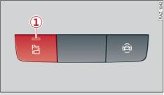
Fig. 161 Centre console: Button for parking aid
