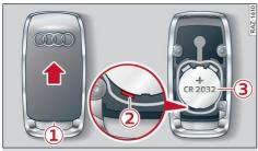
Fig. 98 Remote control: Changing battery
