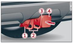
Fig. 120 Rear bumper: Towing bracket
