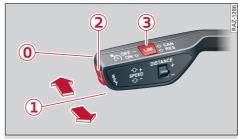
Fig. 143 Control lever: Operating adaptive cruise assist
