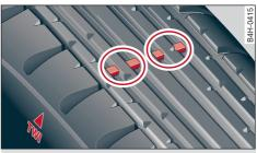
Fig. 215 Tyre tread: Tread wear indicators
