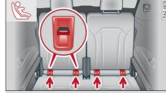
**Fig. 76** Rear seat bench in third row of seats: Bottom ISO-FIX anchorages
