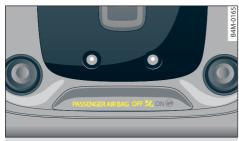
**Fig. 72** Headliner: Indicator lamp for status of front passenger's airbag
