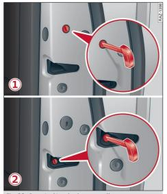
Fig. 23 Door: Locking the door manually
