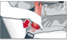
Fig. 66 Latch plate and buckle
