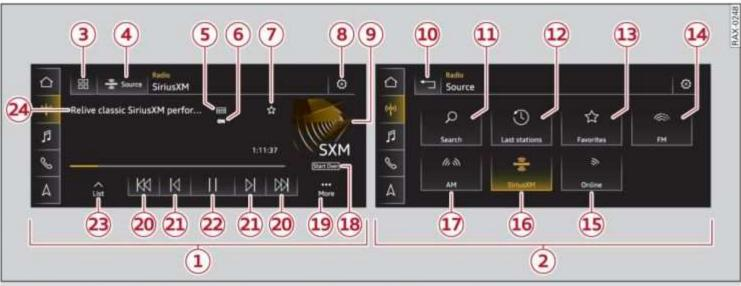
Fig. 161 Upper display: left side: playback view of radio functions, right side: sources
