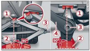
Fig. 188 Sill: positioning the vehicle jack
