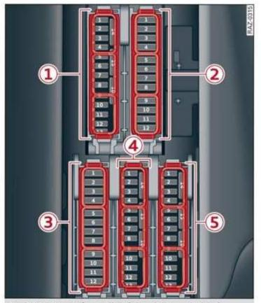
Fig. 198 Driver's footwell (left-hand drive vehicle): fuse panel with plastic clip
