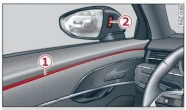
Fig. 127 Front door: warning strip
