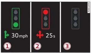
Fig. 103 Instrument cluster: traffic light information display
