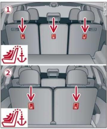
Fig. 74 ① Second row rear bench seat / ② third row rear bench seat: top tether anchors for securing a child safety seat with an upper strap
