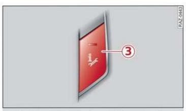
Fig. 150 Front headliner: online roadside assistance button
