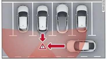
Fig. 137 Sensor detection range for rear cross-traffic assist
