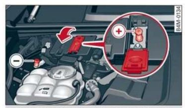
Fig. 191 Engine compartment: connectors for jump start cables or a charger
