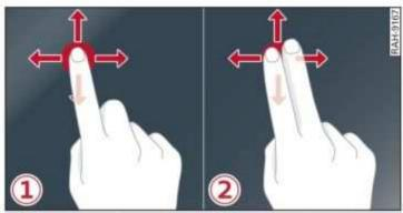
Fig. 12 Touch display: 1 dragging with one finger, 2 dragging with two fingers
