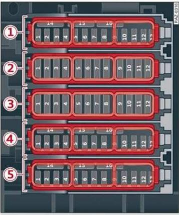
Fig. 199 Front passenger's footwell (right-hand drive vehicle): fuse panel with plastic clip
