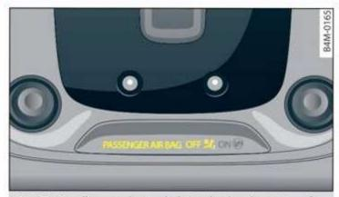
Fig. 71 Headliner: indicator light to display the status of the front passenger's airbag
