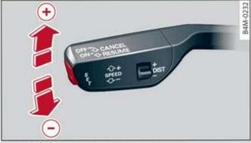
Fig. 110 Operating lever: changing the speed
