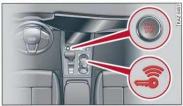
Fig. 90 Center console: starting the engine
