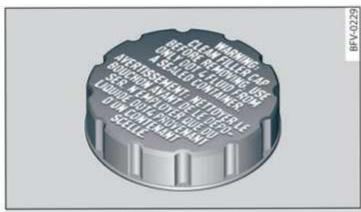
Fig. 173 Engine compartment: cap on brake fluid reservoir
