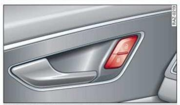
Fig. 21 Driver's door: central locking switch
