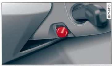
Fig. 60 Steering column: switch for adjusting the steering wheel position
