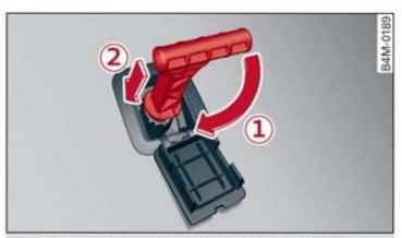
Fig. 94 Footwell: releasing the parking lock using the emergency release
