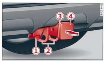
Fig. 95 Rear bumper: trailer hitch
