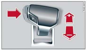
Fig. 92 Center console: shifting manually with the selector lever
