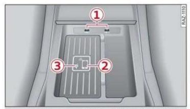
Fig. 146 Storage compartment under the center armrest: Audi phone box with connections
