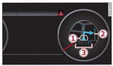
Fig. 156 Instrument cluster: default view: turning maneuver when route guidance has started
