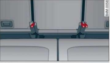
Fig. 83 Luggage compartment: release straps\*
