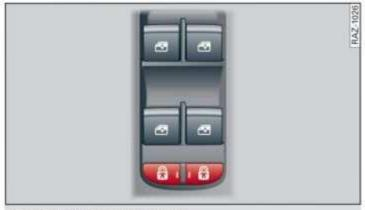
Fig. 32 Driver's door: controls
