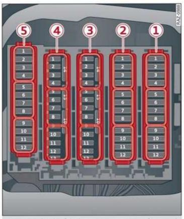
Fig. 202 Left side of the luggage compartment: fuse panel with plastic clip (plug-in hybrid drive\*)
