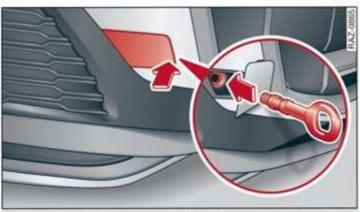
Fig. 194 Front bumper: installing the towing loop (version 2)
