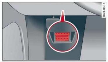
Fig. 203 Driver's side footwell: connection port for the On Board Diagnostic System (OBD)
