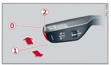
Fig. 116 Lever: using adaptive cruise assist
