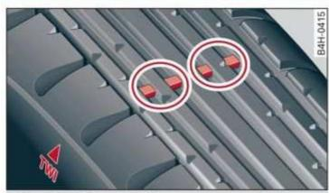
Fig. 177 Tire profile: treadwear indicator
