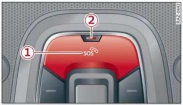
Fig. 149 Front headliner: cover for the emergency call but-
