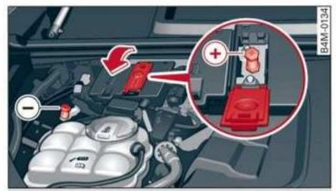
Fig. 174 Engine compartment: connectors for a charger or jump start cables
