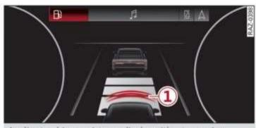
Applies to: driver assistance display without area view Fig. 117 Instrument cluster: safe start monitor
