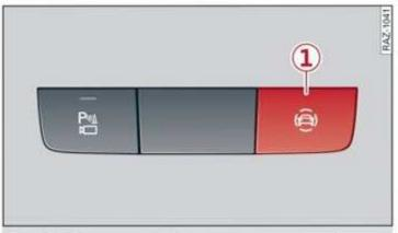
Fig. 100 Center console: driver assistance systems button
