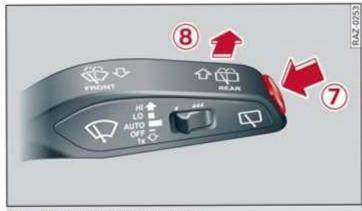
Fig. 47 Lever: rear window wiper
