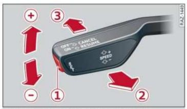
Fig. 105 Operating lever: switching the system on
