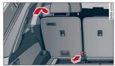
Fig. 57 Second-row seating: folding the seat down
