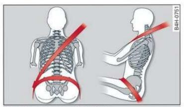
Fig. 64 Lap/shoulder belt positioning
