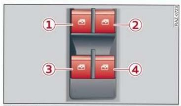
Fig. 33 Driver's door: power window switch
