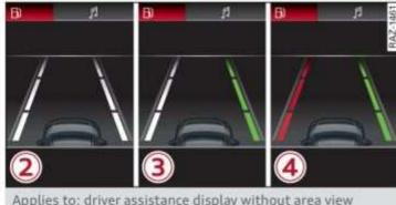
Applies to: driver assistance display without area view Fig. 123 Instrument cluster: lane departure warning
