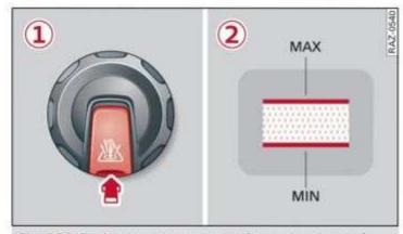
Fig. 172 Engine compartment - Coolant expansion tank (diagram): 1 cover with release button; 2 markings
