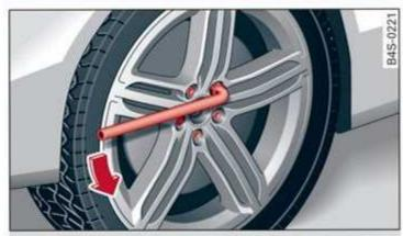
Fig. 186 Wheel: loosening the wheel bolts
