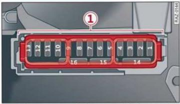
Fig. 200 Driver side cockpit: fuse panel with plastic bracket
