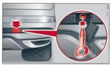
Fig. 195 Rear bumper: installing the towing loop
