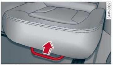
Fig. 56 Second row seats: adjusting the seat position
