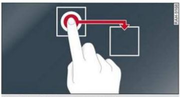
Fig. 9 Touch display: pressing and pulling
