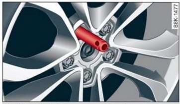
Fig. 190 Wheel: alignment pin in the top hole
