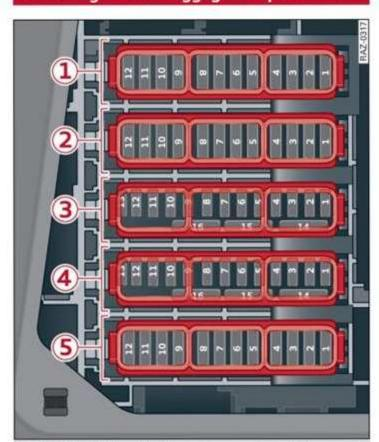
Fig. 201 Left side of the luggage compartment: fuse panel with plastic clip
