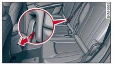
Fig. 82 Second row seats: release strap on the center backrest
