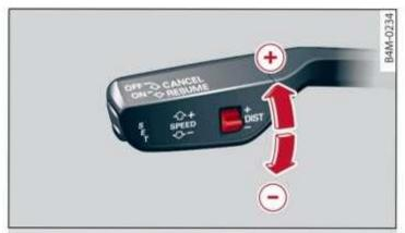
Fig. 115 Operating lever: setting the distance
