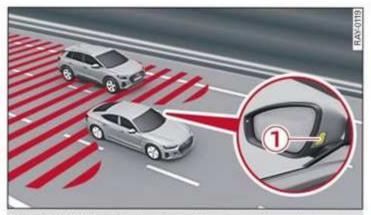
Fig. 124 Driving situations and displays in the exterior mirror
