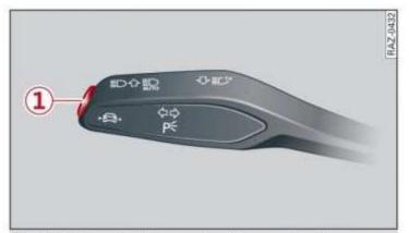
Fig. 122 Turn signal lever: button for lane departure warning and lane guidance for adaptive cruise assist\*
