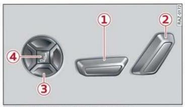
Fig. 52 Front seat: seat adjustment buttons
