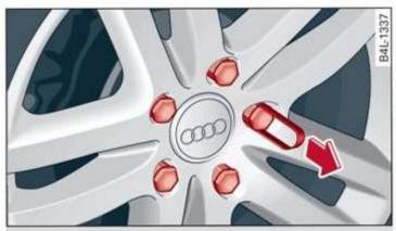
Fig. 184 Wheel: wheel bolts with caps
