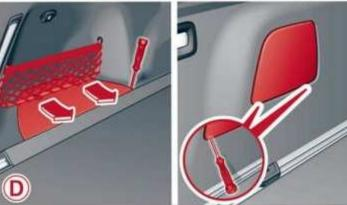
Fig. 197 Driver's side cockpit: cover (C), left side of luggage compartment: cover (D) (opening on the right only in vehicles with plug-in hybrid drive\*)
