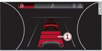
Applies to: driver assistance display without area view Fig. 112 Instrument cluster: brake intervention request
