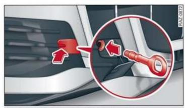
Fig. 193 Front bumper: installing the towing loop (version 1)
