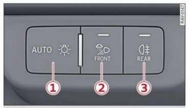
Fig. 35 Instrument panel: light button module
