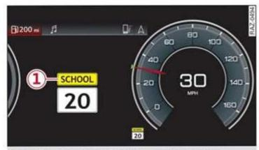
Fig. 102 Instrument cluster: traffic sign recognition
