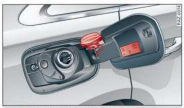
Fig. 166 Fuel filler door with attached fuel cap
