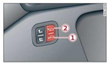
Fig. 81 Left side of the luggage compartment: rear lowering button
