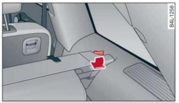
Fig. 80 Luggage compartment: removing and installing the luggage compartment cover
