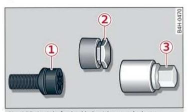
Fig. 185 Anti-theft wheel bolt with cap and adapter
