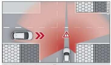
Fig. 128 Detected cross-traffic
