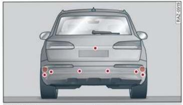
Fig. 99 Rear area: sensors and cameras
