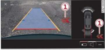
Fig. 138 Upper display: rear cross-traffic assist display
