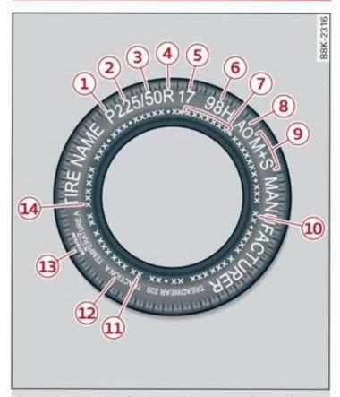
Fig. 176 Tire designations on the sidewall
