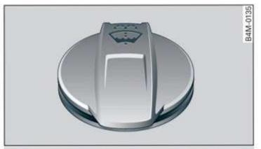
Fig. 175 Engine compartment: washer fluid reservoir cap
