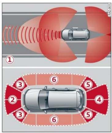
Fig. 96 Sensor coverage area
