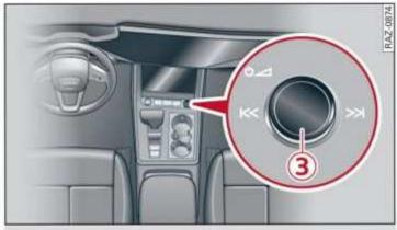
Fig. 20 MMI On/Off knob with joystick function
