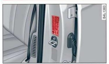
Fig. 178 Driver's side B-pillar: tire pressure label
