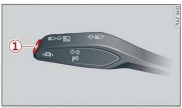
Fig. 111 Turn signal lever: button for lane guidance and lane departure warning
