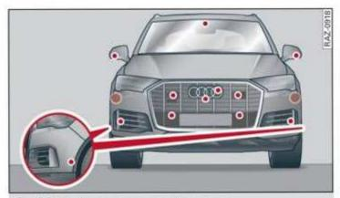
Fig. 98 Front area: sensors and cameras
