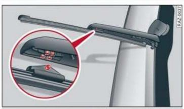
Fig. 49 Rear window wiper: installing the wiper blade
