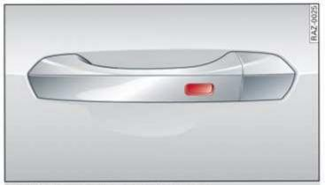
Fig. 25 Door handle: sensor for locking
