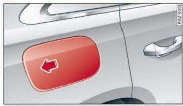
Fig. 165 Right rear side of the vehicle: opening the fuel filler door
