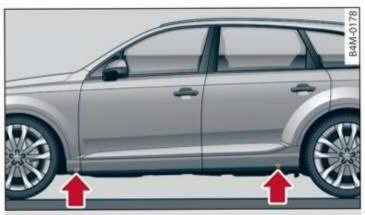
Fig. 187 Sill panels: markings
