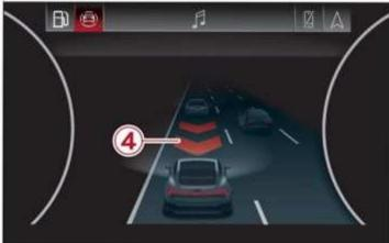
Applies to: vehicles with adaptive cruise assist: Fig. 121 Instrument cluster: distance warning with or
