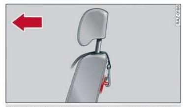
Fig. 75 Rear backrest; securing the upper belt to the top tether anchor
