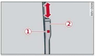
Fig. 48 Windshield wipers: changing the wiper blades
