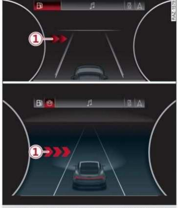
Fig. 129 Instrument cluster: intersection assistant direction display with or without area view
