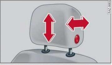
Fig. 62 Front seat: adjusting the head restraint
