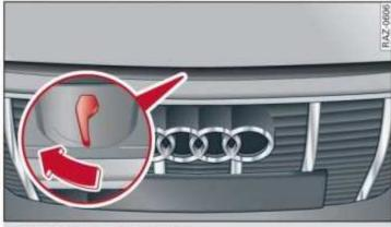
Fig. 168 Unlocked hood: lever
