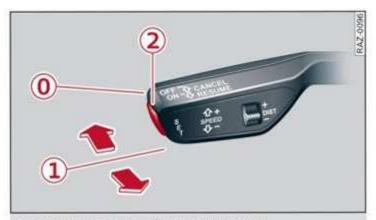
Fig. 109 Lever: using adaptive cruise assist
