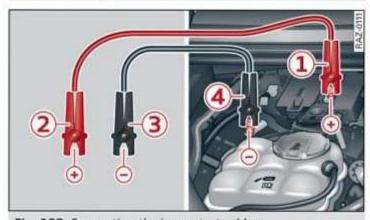
Fig. 192 Connecting the jump start cables
