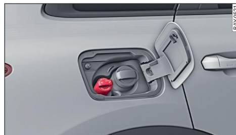
Fig. 116 Vehicle as seen from the rear right: Unscrewing the AdBlue cap
