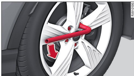
Fig. 138 Wheel: Loosening the wheel bolts
