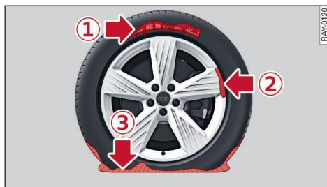
Fig. 132 Tyres: Irreparable tyre damage
