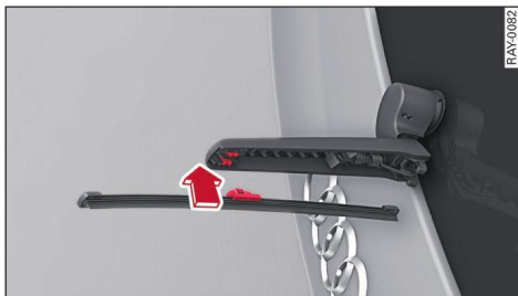
Fig. 26 Rear window wiper: Attaching the wiper blade
