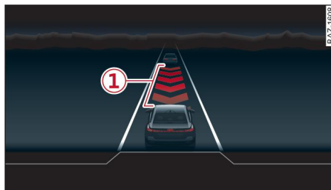
Fig. 78 Instrument cluster showing distance warning
