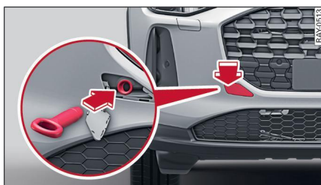
Fig. 142 Front bumper: Fitting the towline anchorage
