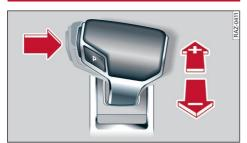
**Fig. 94** Center console: shifting manually with the transmission selector
