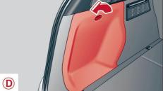
**Fig. 196** Driver's side cockpit (left-hand drive/right-hand drive vehicles): cover (a), left side of luggage compartment: cover (b)
