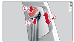
**Fig. 71** Belt height adjustment for the front seats - safety belt relay
