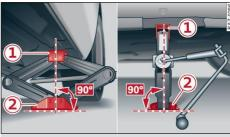
Fig. 187 Sill: positioning the vehicle jack
