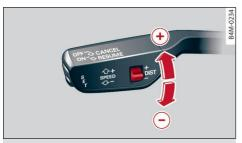
Fig. 121 Lever: setting the distance
