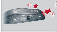
Fig. 53 Lever: rear window wiper
