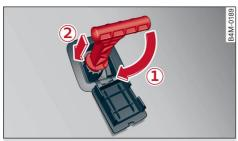
**Fig. 97** Driver's side footwell: releasing the parking lock using the manual release
