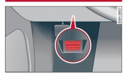
**Fig. 201** Driver's side footwell: connection port for the On Board Diagnostic System (OBD)
