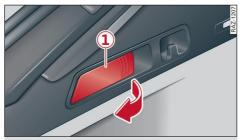
Fig. 82 Luggage compartment: release lever
