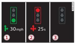
Fig. 113 Instrument cluster: traffic light information display
