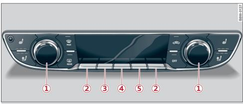
Fig. 90 3-zone deluxe automatic climate control system: controls
