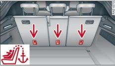
**Fig. 75** Rear backrest: top tether anchors to secure a child safety seat with an upper belt
