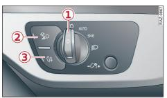
Fig. 42 Instrument panel: light switch with buttons
