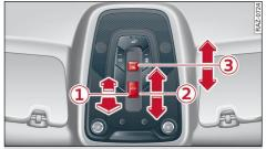
Fig. 40 Headliner: panoramic glass roof and sunshade\* buttons
