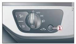
Fig. 48 Light switch: instrument illumination
