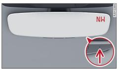
Fig. 56 Rearview mirror: digital compass is turned on
