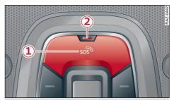
Fig. 147 Front headliner: cover for the emergency call but-
