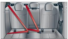
Fig. 77 Rear bench seat: securing unused safety belts
