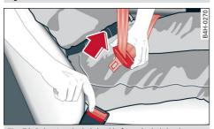
Fig. 70 Releasing the belt buckle from the belt latch
