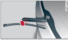
Fig. 55 Rear window wiper: installing the wiper blade
