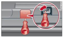
Fig. 36 Inner luggage compartment lid: access to the manual release
