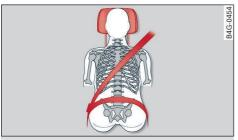
Fig. 64 Correctly-adjusted head restraint
