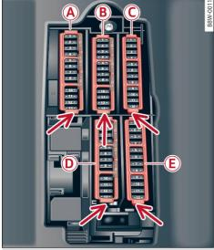
Fig. 197 Driver's footwell (left-hand drive vehicle): fuse panel with plastic clip
