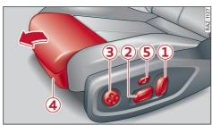
Fig. 58 Front seat: adjusting the seat
