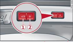
Fig. 34 Luggage compartment lid: (1) closing button\*, (2) lock button\* (vehicles with convenience key\*)
