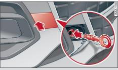
Fig. 192 Front bumper: installing the towing eye
