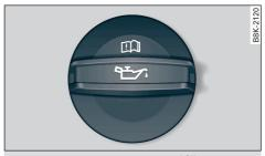
**Fig. 170** Engine compartment: engine oil filling opening cover (example)
