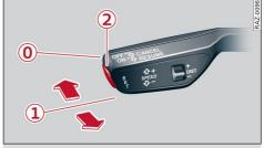
Fig. 122 Lever: operating the Audi adaptive cruise control
