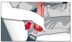
Fig. 69 Belt buckle and belt latch
