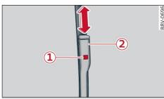
Fig. 54 Windshield wipers: replacing the wiper blades
