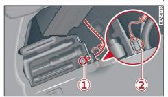
**Fig. 103** Left side of the luggage compartment: charging connector manual emergency release
