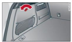
**Fig. 102** Left side of luggage compartment: charging connector manual release cover
