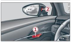
Fig. 131 Front door: exit warning
