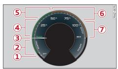
Applies to: vehicles with Audi virtual cockpit **Fig. 7** Instrument cluster: power meter
