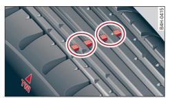
**Fig. 176** Tire profile: treadwear indicator
