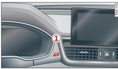
Fig. 9 Instrument cluster: reset button
