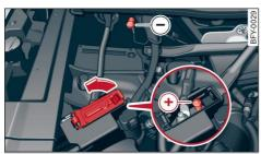
Fig. 190 Engine compartment: connectors for jump start cables or a charger
