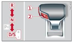
Fig. 93 Center console: transmission selector
