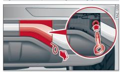
Fig. 194 Rear bumper: installing the towing eye (version 2)
