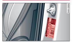
**Fig. 177** Driver's side B-pillar: tire pressure label
