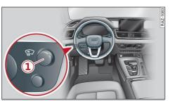
Fig. 21 Instrument panel: knob for the head-up display
