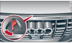
Fig. 167 Unlocked hood: lever
