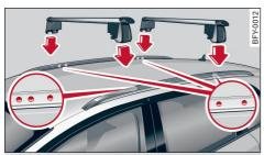
Fig. 88 Roof rail: mounting points
