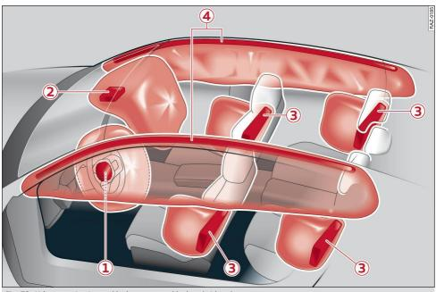
Fig. 72 Airbag overview image (deployment area/deployed airbags)
