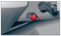
**Fig. 63** Steering column: switch for adjusting the steering wheel position
