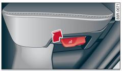
Fig. 61 Adjusting the backrests
