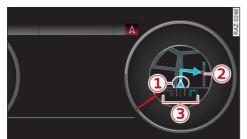
Fig. 154 Instrument cluster: default view: turning maneuver when route quidance has started
