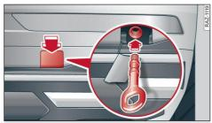
Fig. 193 Rear bumper: installing the towing eye (version 1)
