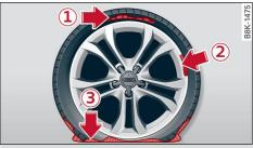
Fig. 181 Tire: tire damage that cannot be repaired
