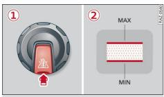
Fig. 171 Engine compartment - coolant expansion tank (diagram): ① cover with release button; ② coolant expansion tank markings
