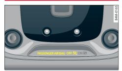
Fig. 73 Headliner: indicator light to display the status of the front passenger's airbag
