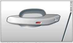
Fig. 29 Door handle: sensor for locking
