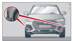
Fig. 109 Front area: sensors and cameras
