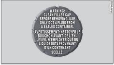
Fig. 172 Engine compartment: cap on brake fluid reservoir
