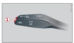
Fig. 128 Turn signal lever: button for Audi active lane assist
