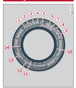
**Fig. 175** Tire designations on the sidewall
