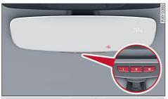
Fig. 41 Rearview mirror: buttons for the garage door open-
