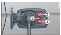
Fig. 101 Charging unit: charging port and buttons/charging display
