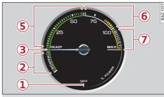
Applies to: vehicles with analog instrument cluster **Fig. 8** Instrument cluster: power meter
