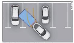
Fig. 134 Orientation line display when parking
