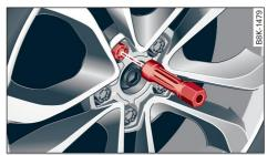
Fig. 188 Wheel: internal hex socket to turn the wheel bolts
