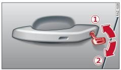
Fig. 26 Driver's door: door lock cylinder
