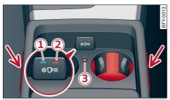
Fig. 79 Center console: climatized cup holder
