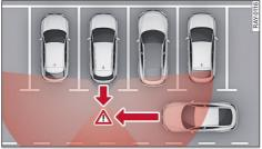
Fig. 139 Sensor detection range for rear cross-traffic assist
