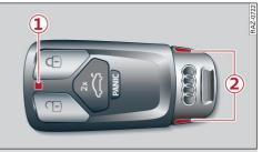
Fig. 30 Vehicle key: removing the battery holder
