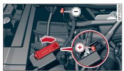
**Fig. 173** Engine compartment: connectors for a charger or jump start cables
