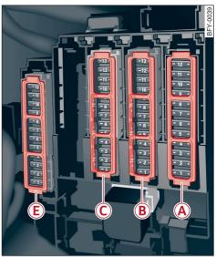
**Fig. 200** Left side of the luggage compartment: fuse panel with plastic clip
