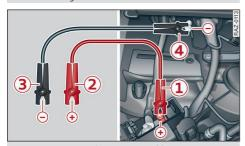
Fig. 191 Connecting the jump start cables
