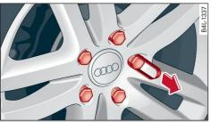
Fig. 184 Wheel: wheel bolts with caps
