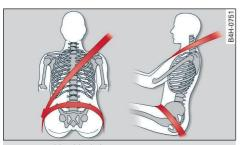
Fig. 67 Lap/shoulder belt positioning
