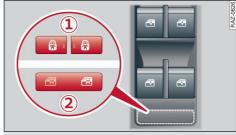
Fig. 37 Driver's door: controls
