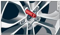
Fig. 189 Wheel: alignment pin in the top hole
