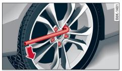
Fig. 185 Wheel: loosening the wheel bolts
