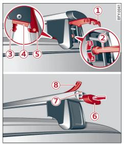
Fig. 89 Roof rail: installing a roof rack
