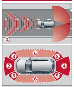
Fig. 107 Sensor detection ranges
