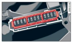
Fig. 199 Driver side cockpit: fuse panel with plastic bracket
