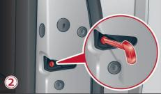
Fig. 27 Door: mechanically locking
