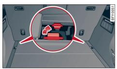
Fig. 87 Luggage compartment: installing the cargo floor
