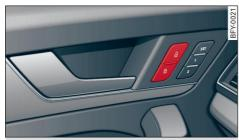
Fig. 25 Driver's door: central locking switch
