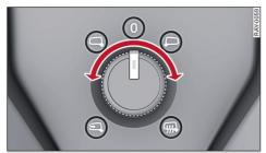
Fig. 49 Driver's door: knob for the exterior mirrors
