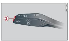
**Fig. 124** Turn signal lever: button for traffic jam assist and Audi active lane assist
