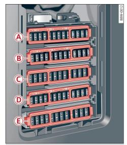
Fig. 198 Front passenger's footwell (right-hand drive vehicle): fuse panel with plastic clip
