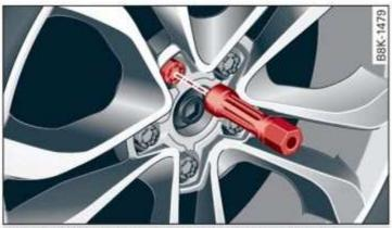
Fig. 193 Wheel: internal hex socket to turn the wheel holts
