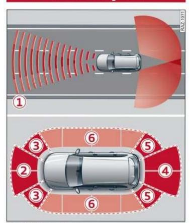
Fig. 112 Sensor detection ranges
