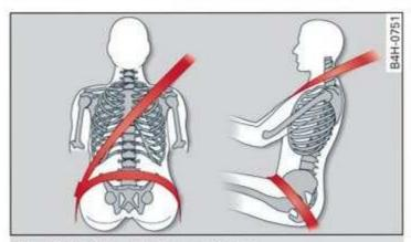
Fig. 67 Lap/shoulder belt positioning
