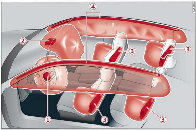
Fig. 72 Airbag overview image (enlarged section: deployed airbags)
