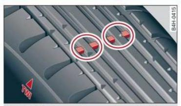
Fig. 181 Tire profile: treadwear indicator
