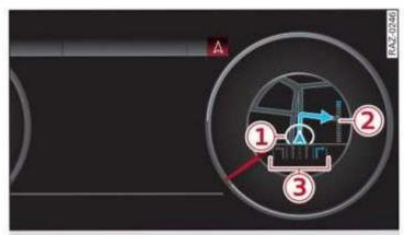
Fig. 159 Instrument cluster: default view: turning maneuver when route guidance has started
