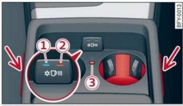
Fig. 79 Center console: climatized cup holder
