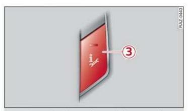
Fig. 153 Front headliner: online roadside assistance button
