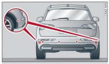
Fig. 115 Rear area: sensors and cameras
