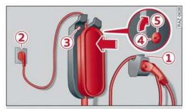
Fig. 110 Wall mount clip: securing the Audi charging system
