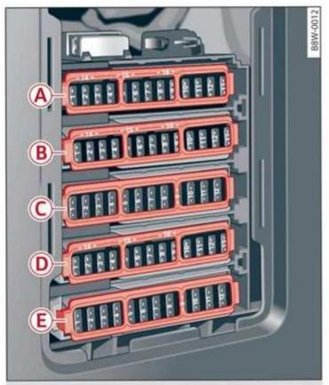
Fig. 203 Front passenger's footwell (right-hand drive vehicle): fuse panel with plastic clip
