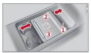
Fig. 149 Front center console: Audi phone box with connections
