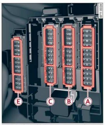
Fig. 205 Left side of the luggage compartment: fuse panel with plastic clip
