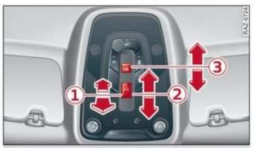
Fig. 41 Headliner: panoramic glass roof and sunshade\* buttons
