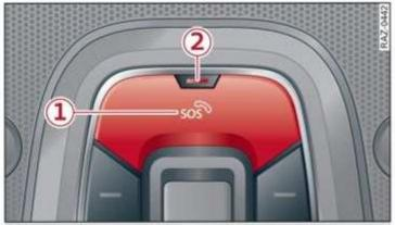
Fig. 152 Front headliner: cover for the emergency call but-
