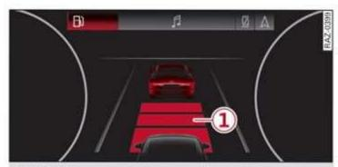
Fig. 125 Instrument cluster: brake intervention request
