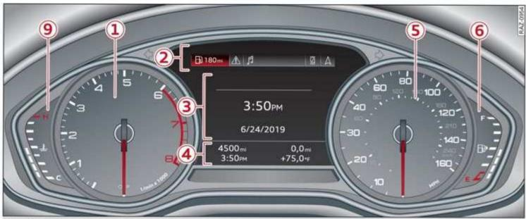
Fig. 4 Instrument cluster overview (analog)
