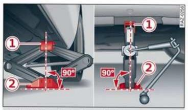
Fig. 192 Sill: positioning the vehicle jack
