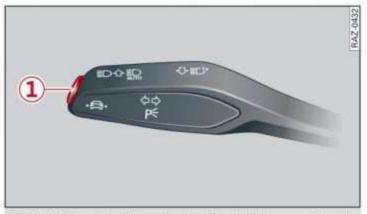
Fig. 129 Turn signal lever: button for traffic jam assist and Audi active lane assist
