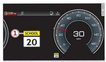
Fig. 117 Instrument cluster: traffic sign recognition
