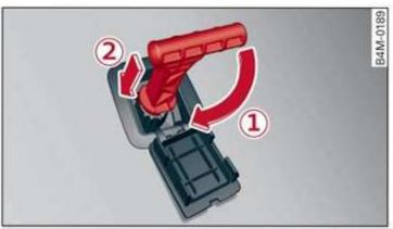
Fig. 98 Driver's side footwell: releasing the parking lock using the manual release
