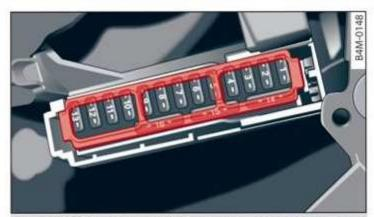
Fig. 204 Driver side cockpit: fuse panel with plastic bracket
