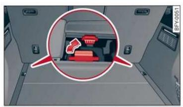
Fig. 88 Luggage compartment: installing the cargo floor
