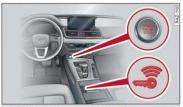
Fig. 93 Center console: starting the engine
