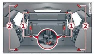
Fig. 85 Backrest folded forward: partition net
