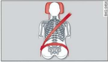
Fig. 64 Correctly-adjusted head restraint
