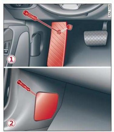
Fig. 200 Driver's side footwell (left-hand drive vehicles): footrest 1, front passenger's side footwell (right-hand drive vehicles): cover 2
