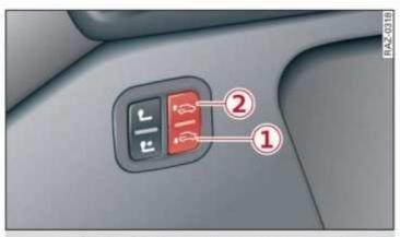
Fig. 82 Left side of the luggage compartment: rear lowering button
