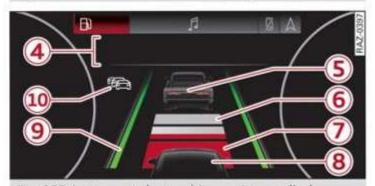
Fig. 122 Instrument cluster: driver assistance display
