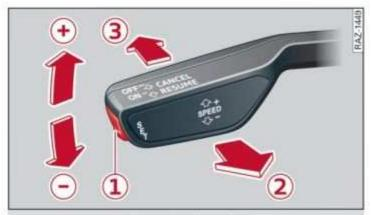
Fig. 119 Operating lever: switching the system on
