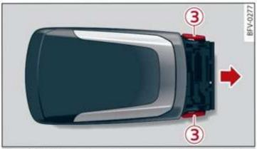
Fig. 32 Vehicle key (rear side): removing the battery holder
