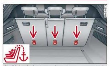
Fig. 75 Rear backrest: top tether anchors to secure a child safety seat with an upper belt
