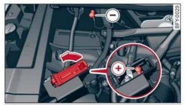
Fig. 178 Engine compartment: connectors for a charger or jump start cables
