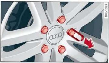
Fig. 189 Wheel: wheel bolts with caps
