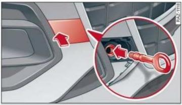
Fig. 197 Front bumper: installing the towing loop
