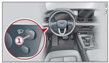
Fig. 22 Instrument panel: knob for the head-up display
