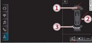
Fig. 138 Center display: distance display
