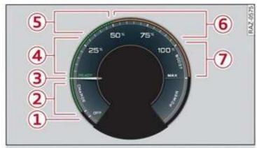
Applies to: vehicles with Audi virtual cockpit Fig. 8 Instrument cluster: power meter
