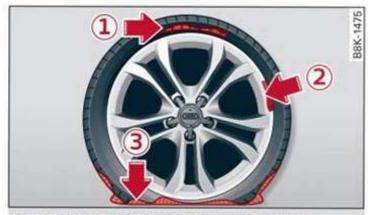
Fig. 186 Tire: tire damage that cannot be repaired
