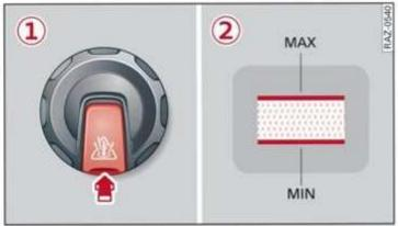
Fig. 176 Engine compartment - coolant expansion tank (diagram): 1 cover with release button; 2 coolant expansion tank markings
