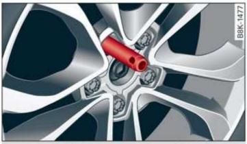
Fig. 194 Wheel: alignment pin in the top hole
