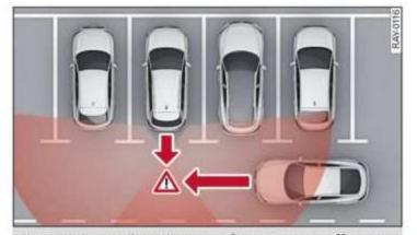
Fig. 144 Sensor detection range for rear cross-traffic assist
