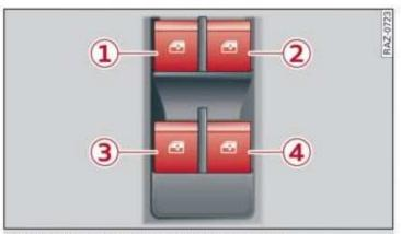
Fig. 40 Driver's door: power window switch
