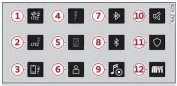
Fig. 19 Center display: frequently used symbols in the status bar
