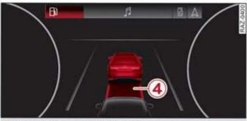
Applies to: vehicles with Audi adaptive cruise control Fig. 131 Instrument cluster: distance warning
