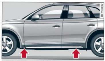
Fig. 191 Sill panels: markings
