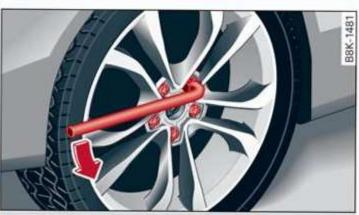
Fig. 190 Wheel: loosening the wheel bolts
