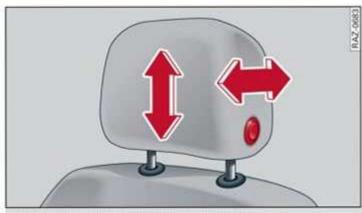
Fig. 65 Front seat: adjusting the head restraint
