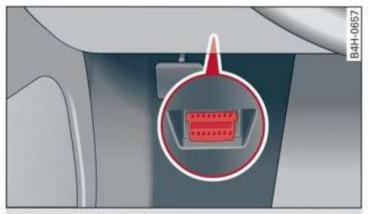
Fig. 206 Driver's side footwell: connection port for the On Board Diagnostic System (OBD)
