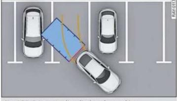
Fig. 139 Orientation line display when parking
