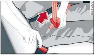
Fig. 70 Releasing the belt buckle from the belt latch
