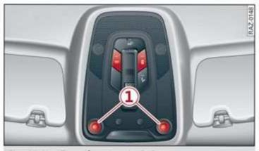
Fig. 45 Headliner: front interior lighting
