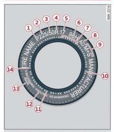
Fig. 180 Tire designations on the sidewall
