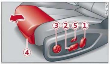
Fig. 58 Front seat: adjusting the seat
