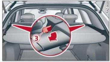
Fig. 81 Luggage compartment: removing and installing the luggage compartment cover
