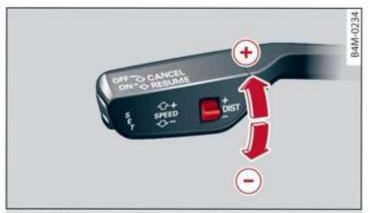
Fig. 126 Operating lever: setting the distance
