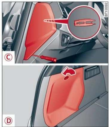
Fig. 201 Driver's side cockpit (left-hand drive/right-hand drive vehicles): cover ©, left side of luggage compartment: cover ©
