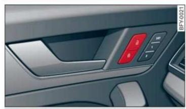
Fig. 26 Driver's door: central locking switch
