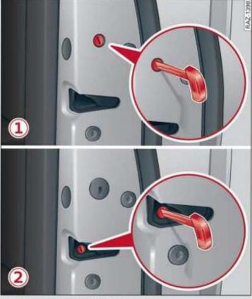
Fig. 28 Door: mechanically locking
