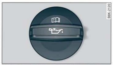
Fig. 175 Engine compartment: engine oil filling opening cover (example)
