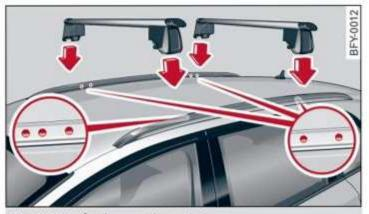
Fig. 89 Roof rail: mounting points
