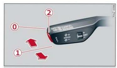
Fig. 123 Operating lever: operating adaptive cruise control
