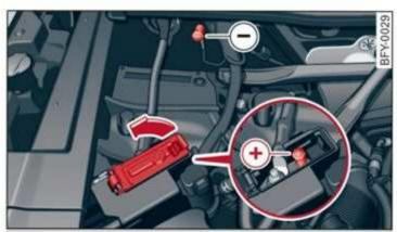
Fig. 195 Engine compartment: connectors for jump start cables or a charger
