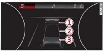
Applies to: vehicles with adaptive cruise control: Fig. 130 Instrument cluster: display of the current distance
