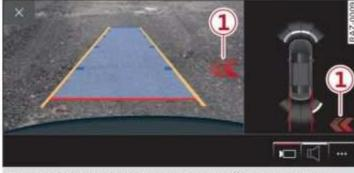
Fig. 145 Center display: rear cross-traffic assist display
