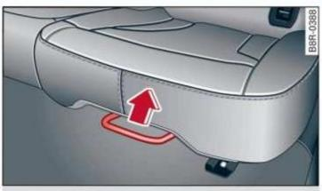
Fig. 60 Adjusting the seat position
