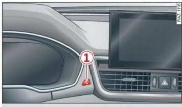
Fig. 10 Instrument cluster: reset button
