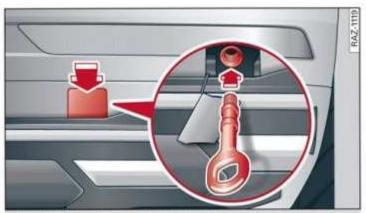
Fig. 198 Rear bumper: installing the towing loop (version 1)
