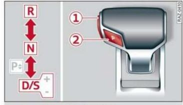
Fig. 94 Center console: selector lever
