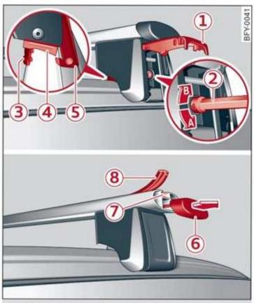
Fig. 90 Roof rail: installing a roof rack
