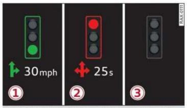
Fig. 118 Instrument cluster: traffic light information display
