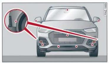
Fig. 114 Front area: sensors and cameras
