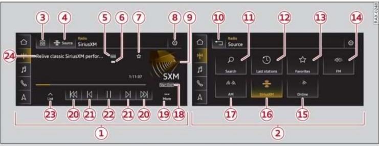
Fig. 165 Center display: left side: playback view of radio functions, right side: sources
