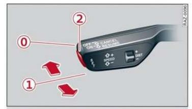
Fig. 127 Lever: operating the Audi adaptive cruise control
