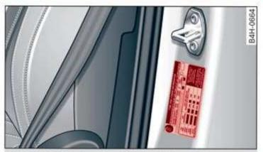
Fig. 182 Driver's side B-pillar: tire pressure label
