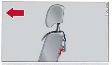
Fig. 76 Rear backrest: securing the upper belt to the top tether anchor
