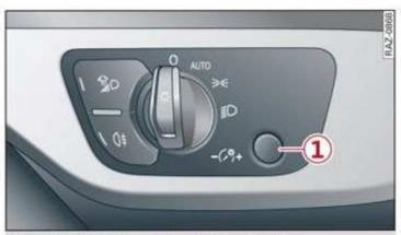
Fig. 48 Light switch: instrument illumination
