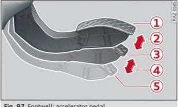
Fig. 97 Footwell: accelerator pedal
