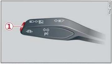
Fig. 133 Turn signal lever: button for Audi active lane assist
