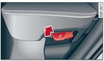
Fig. 61 Adjusting the backrests
