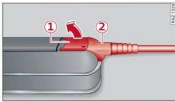
Fig. 109 Control unit: removing and attaching the cable
