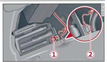
Fig. 104 Left side of the luggage compartment: charging connector manual emergency release
