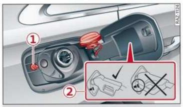
Fig. 170 Fuel filler door with attached fuel cap
