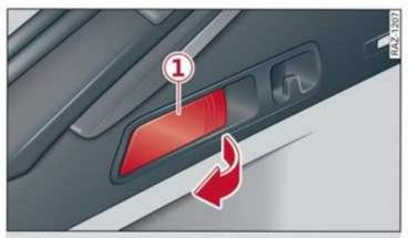
Fig. 83 Luggage compartment: release lever
