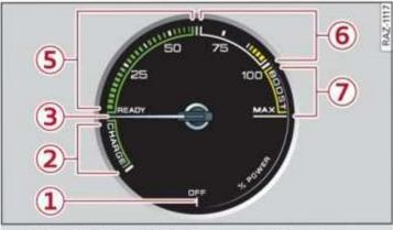
Applies to: vehicles with analog instrument cluster Fig. 9 Instrument cluster: power meter
