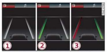
Fig. 132 Instrument cluster: driver assistance display
