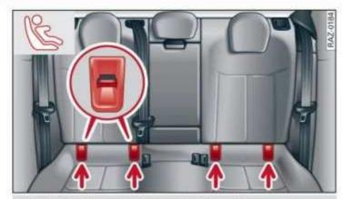
Fig. 74 Rear bench seat: lower LATCH anchors
