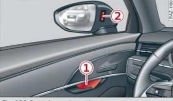
Fig. 136 Front door: exit warning
