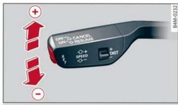
Fig. 124 Operating lever: changing the speed
