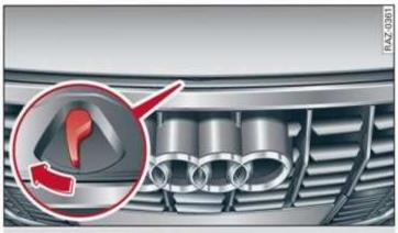
Fig. 172 Unlocked hood: lever
