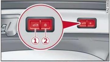
Fig. 35 Luggage compartment lid: 1 closing button\*, 2 lock button\* (vehicles with convenience key\*)
