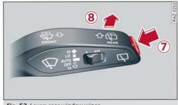
Fig. 53 Lever: rear window wiper
