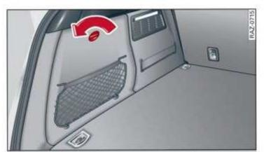
Fig. 103 Left side of luggage compartment: charging connector manual release cover
