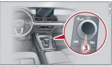
Fig. 25 MMI On/Off knob with joystick function
