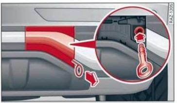
Fig. 199 Rear bumper: installing the towing loop (version 2)
