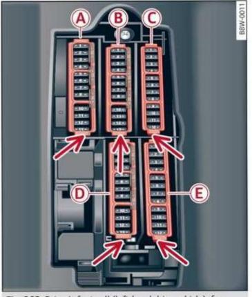
Fig. 202 Driver's footwell (left-hand drive vehicle): fuse panel with plastic clip
