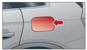
Fig. 101 Left rear side of the vehicle: opening the highvoltage charging port door
