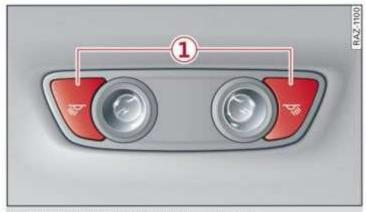
Fig. 46 Headliner: reading lights, version 1
