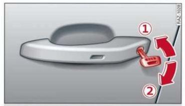
Fig. 27 Driver's door: door lock cylinder
