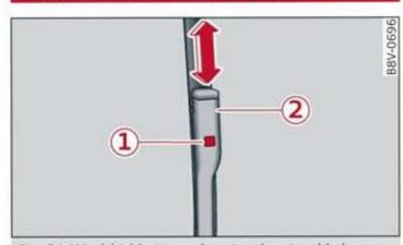
Fig. 54 Windshield wipers: changing the wiper blades
