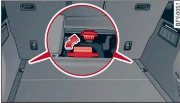
Fig. 85 Luggage compartment: installing the cargo floor
