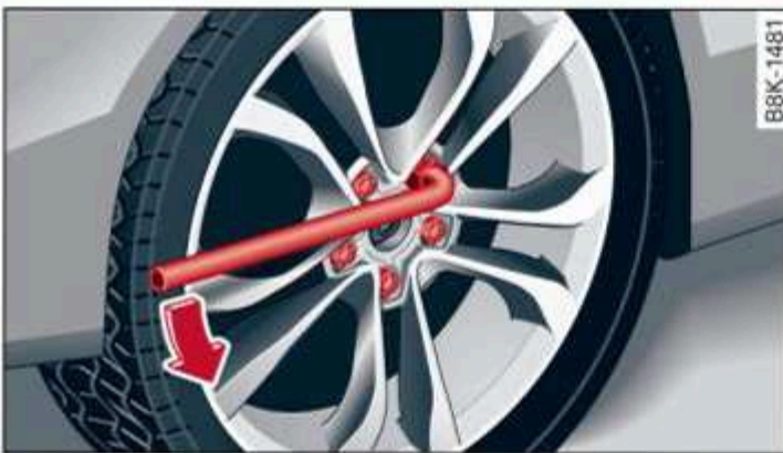
Fig. 171 Wheel: loosening the wheel bolts
