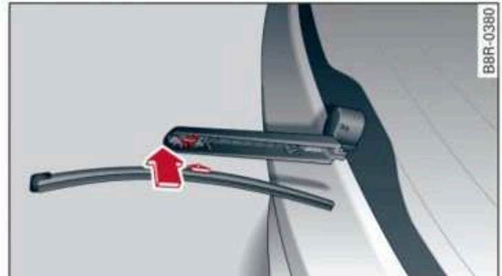
Fig. 52 Rear window wiper: installing the wiper blade
