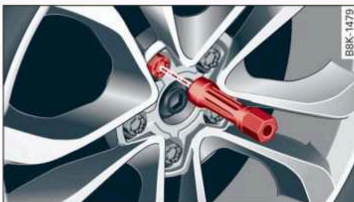
Fig. 174 Wheel: internal hex socket to turn the wheel bolts
