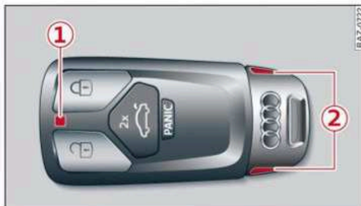
Fig. 28 Vehicle key: removing the battery holder
