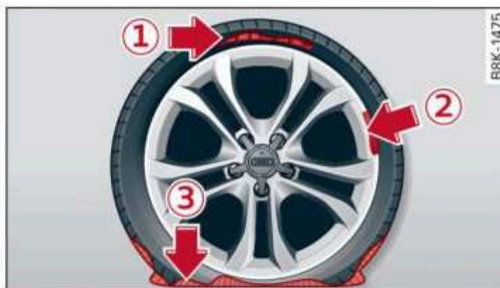
Fig. 167 Tire: tire damage that cannot be repaired
