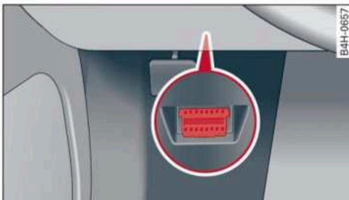
Fig. 187 Driver's side footwell: connection port for the On Board Diagnostic System (OBD)
