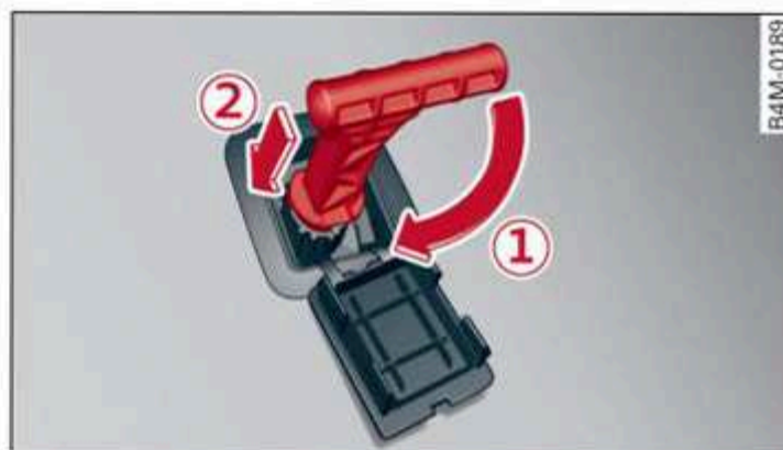
Fig. 94 Driver's side footwell: releasing the parking lock using the emergency release
