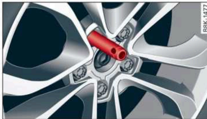
Fig. 175 Wheel: alignment pin in the top hole
