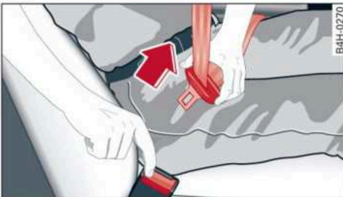
Fig. 67 Releasing the belt buckle from the belt latch
