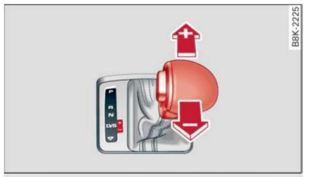
Fig. 137 Center console: shifting the gears manually
