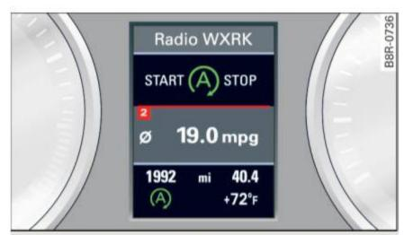
Fig. 104 Instrument cluster: Engine switched off (stop phase)
