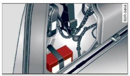
Fig. 213 Luggage compartment left side: compressor
