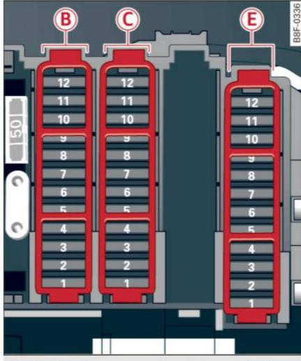
**Fig. 226** Right luggage compartment: fuse panel with plastic clip
