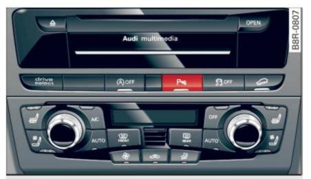
Fig. 145 Center console: Parking system switch
