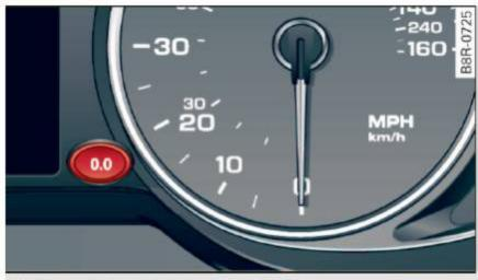
Fig. 7 Instrument cluster: reset button
