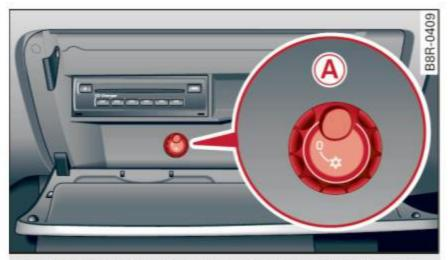
Fig. 94 Glove box with cooling box open and switched on
