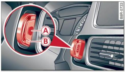
Fig. 28 Ignition switch with ignition key
