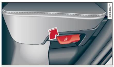
Fig. 72 Release lever for the outer backrest
