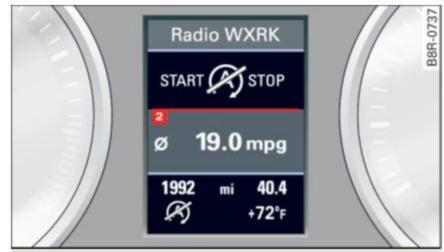
Fig. 105 Instrument cluster: Engine-Stop temporarily unavailable
