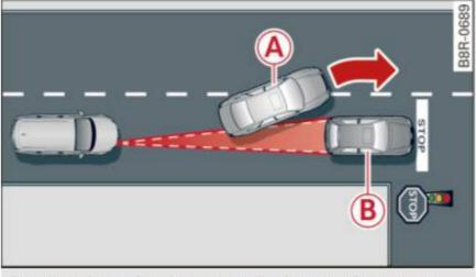
Fig. 118 Example: object changing lanes and stationary object
