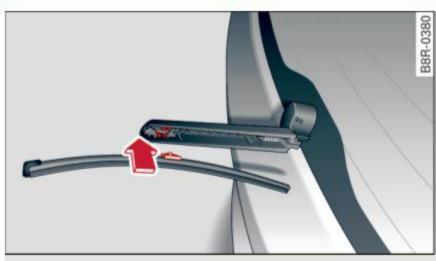
Fig. 59 Rear wiper: Removing the wiper blade
