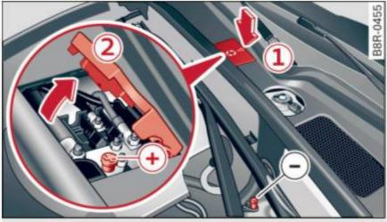
Fig. 202 Engine compartment: Connectors for charger and jumper cables
