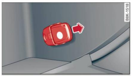
Fig. 100 Glove compartment: Adapter for emergency key
