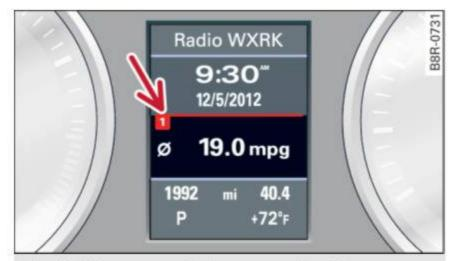
Fig. 16 Trip computer display: memory level 1
