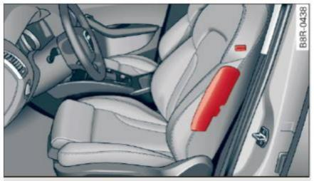
Fig. 169 Side airbag location in the driver's seat
