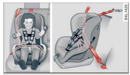
Fig. 176 Schematic overview: installation of the seat using the vehicle's safety belt system
