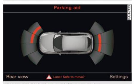
Fig. 146 MMI display: visual distance display
