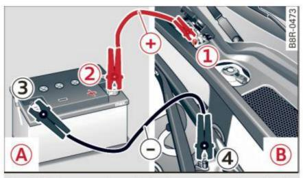
Fig. 228 Jump starting with the battery of another vehicle:
