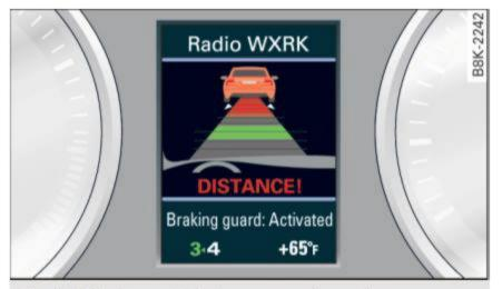
Fig. 126 Instrument cluster: approach warning
