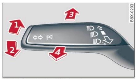
Fig. 50 Turn signal and high beam lever
