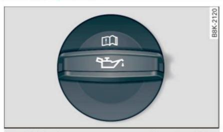
Fig. 199 Engine compartment: cover on the engine oil filler neck
