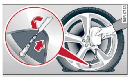
Fig. 215 Performing the repair
