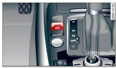
Fig. 103 Center console: Parking brake
