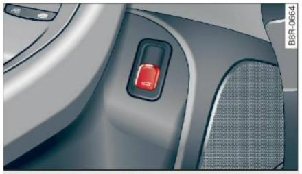
Fig. 36 Driver's door: Unlocking the rear lid
