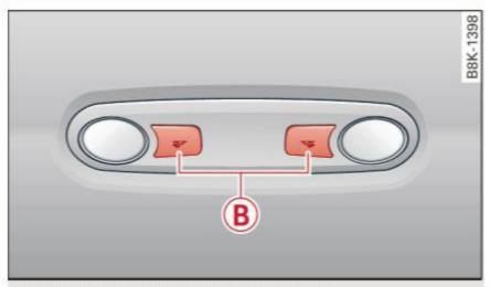
Fig. 52 Rear headliner: rear reading lights
