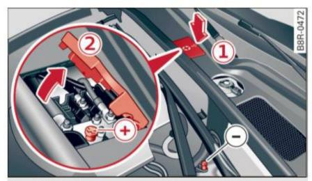
Fig. 227 Engine compartment: Connectors for jumper cables and charger
