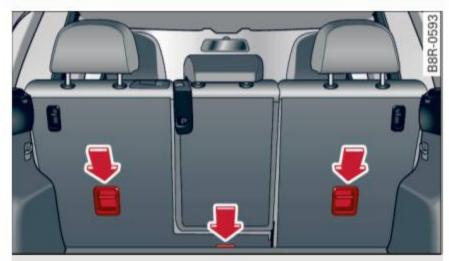
Fig. 182 Tether anchors: attachment hook locations behind the rear seatbacks
