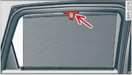
Fig. 55 Sun shade pulled up on a rear window
