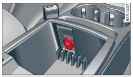
Fig. 92 Center console: 12-volt socket
