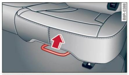
Fig. 67 Fore-and-aft adjustment
