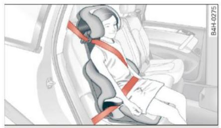
Fig. 177 Rear seat: child properly restrained in a booster seat
