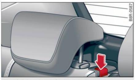
Fig. 73 Release button for the center backrest
