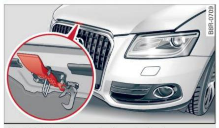
Fig. 196 Release lever under the engine hood
