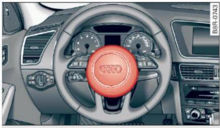
Fig. 165 Location of driver airbag: in steering wheel
