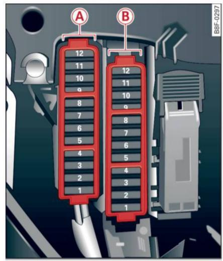
Fig. 225 Right side of the cockpit: fuse panel with plastic clip
