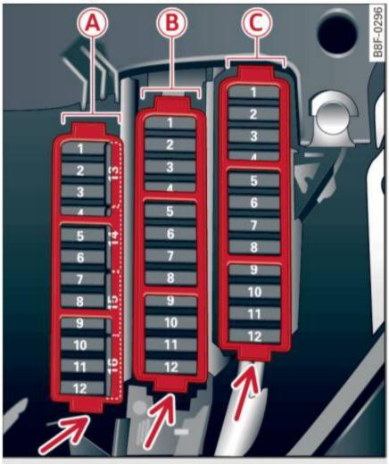
Fig. 224 Left side of the cockpit: fuse panel with plastic clip
