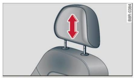
Fig. 68 Front seats head restraints: adjusting the height
