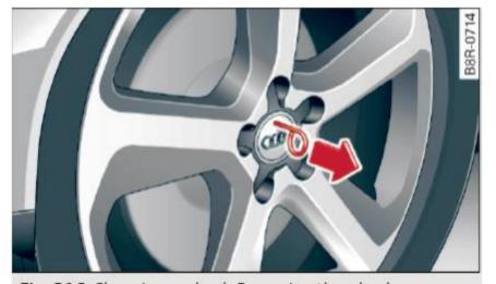
Fig. 216 Changing a wheel: Removing the wheel cover
