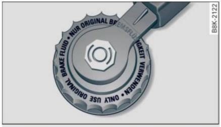
Fig. 201 Engine compartment: cover on the brake fluid reservoir
