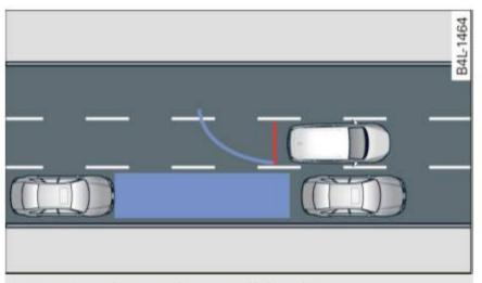
Fig. 142 Parking mode 2: parallel parking
