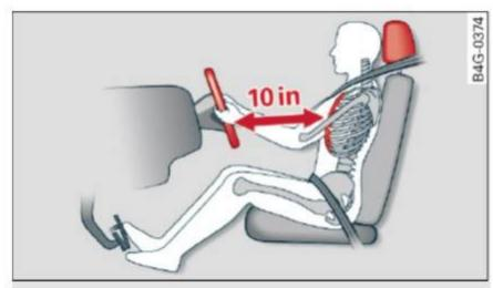
Fig. 151 Correct seating position
