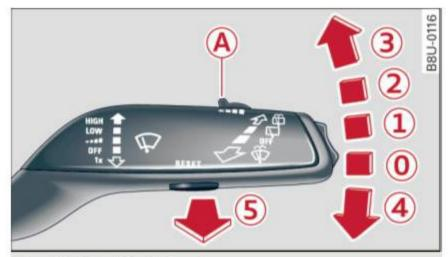
Fig. 56 Windshield wiper lever
