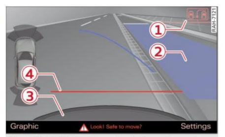
Fig. 149 MMI display: blue surface in the parking spot
