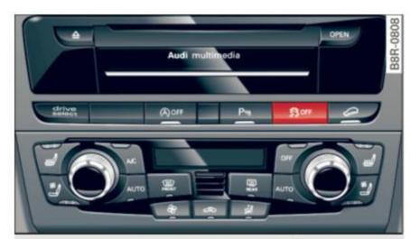
Fig. 186 Version B: Upper center console, \$\mathcal{B}\$ OFF button
