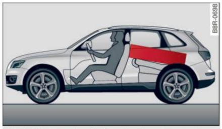
**Fig. 153** Safe load positioning: place heavy objects as low and as far forward as possible.
