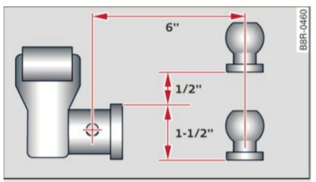
Fig. 189 Permitted ball position of the trailer hitch
