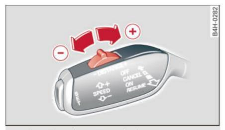
Fig. 124 Selector lever: setting the distance
