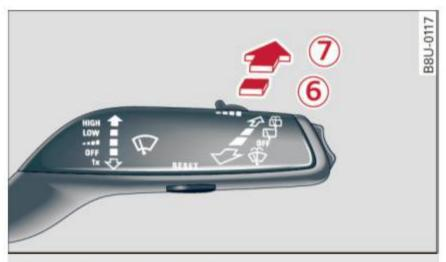
Fig. 57 Rear wiper actuation
