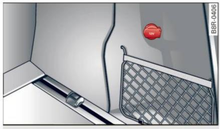
Fig. 91 Section of the trim panel of the luggage compartment: 12-volt socket
