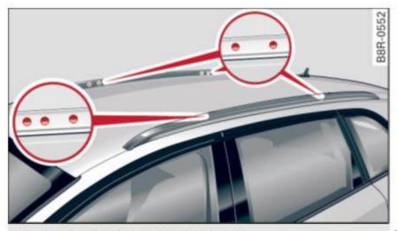
Fig. 81 Roof rack attachment points
