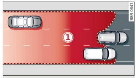
Fig. 127 Sensor detection range
