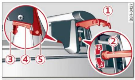
Fig. 83 Roof railing: installing a roof rack
