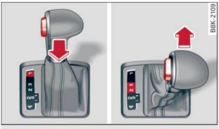
Fig. 135 Shift gate: selector lever lock positions and release button highlighted
