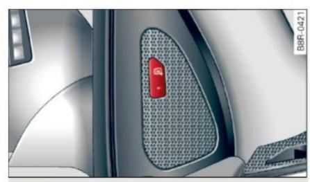
Fig. 131 Driver's door: Side assist button
