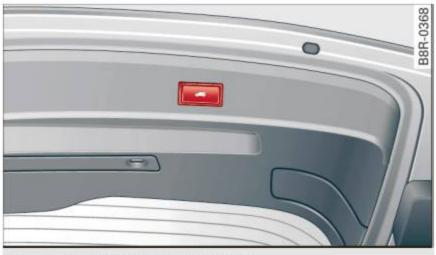
Fig. 37 Locking switch in the rear lid
