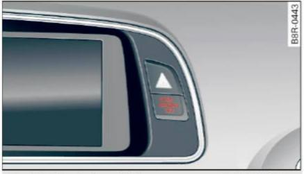
Fig. 168 Section from the instrument panel: PASSENGER AIR BAG OFF light
