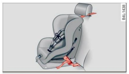
Fig. 183 Tether strap: proper routing and mounting
