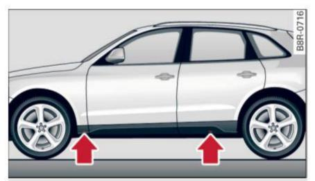
Fig. 219 Sill panels: markings
