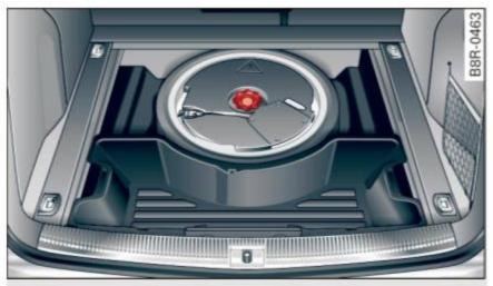
Fig. 212 Inflatable spare tire with compressor
