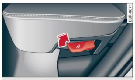
Fig. 66 Adjusting seatback angle
