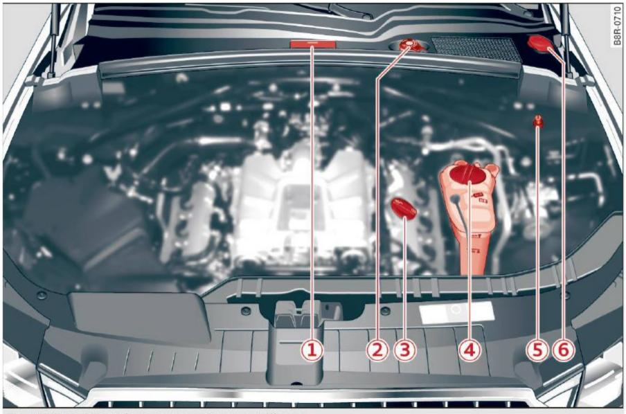
Fig. 197 Typical layout for containers and engine oil filler cap
