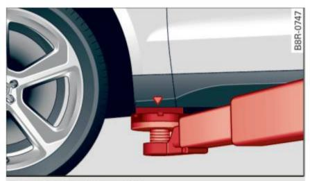
Fig. 234 Front lifting point
