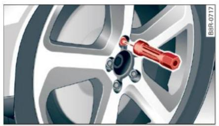
Fig. 221 Changing a wheel: using the screwdriver handle (with the blade removed) to turn the bolts
