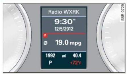
Fig. 11 Display: outside temperature
