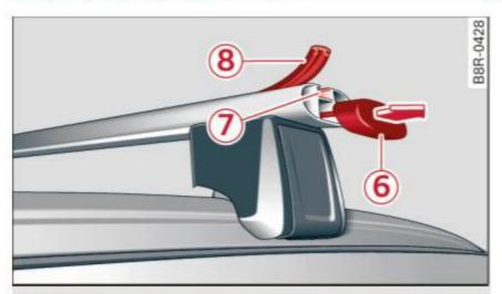
Fig. 84 Roof railing: installing cover profile into the roof rack
