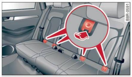
Fig. 179 Lower anchorages, covers marked
