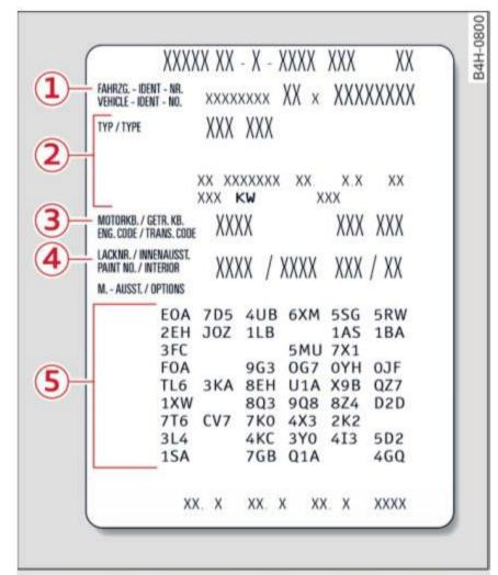
Fig. 237 Vehicle identification label: inside the luggage compartment
