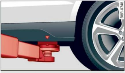
Fig. 235 Rear lifting point
