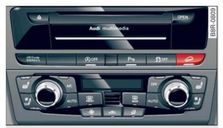
Fig. 187 Top of the center console: hill descent assist but-
