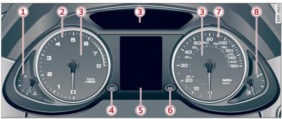
Fig. 3 Overview of the instrument cluster
