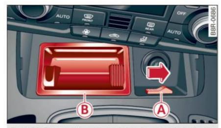
Fig. 139 Front center console: Removing the ashtray insert
