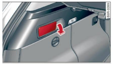
Fig. 74 Luggage compartment: release lever
