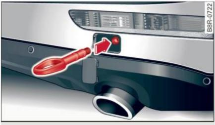
Fig. 232 Rear bumper: Screwing in towing loop
