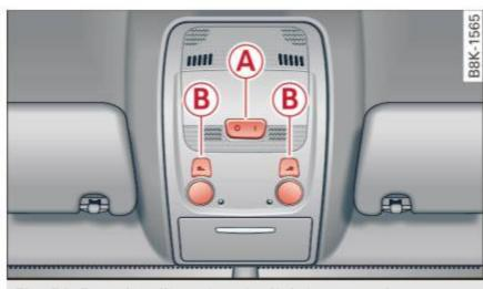
Fig. 51 Front headliner: interior lighting controls
