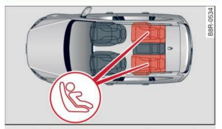
Fig. 178 Schematic overview: LATCH anchorage point locations
