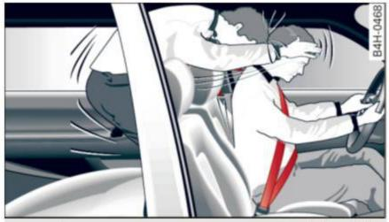
Fig. 158 A rear passenger not wearing a safety belt will fly forward and strike the driver
