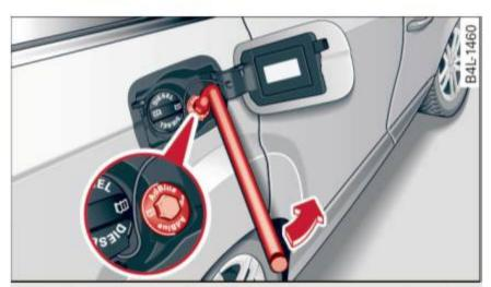
Fig. 193 Right rear side of the vehicle: removing the AdBlue cap
