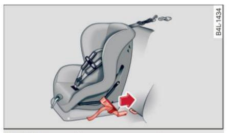
Fig. 181 Lower anchorages: proper mounting
