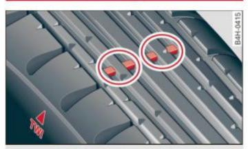
Fig. 205 Tire profile: tread wear indicator
