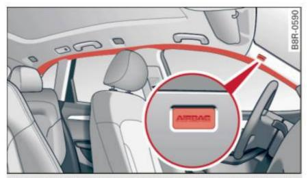
Fig. 171 Side curtain system, driver's side: side curtain airbag location
