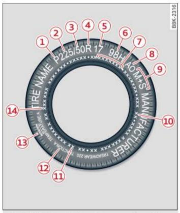
Fig. 204 Tire designations on the sidewall
