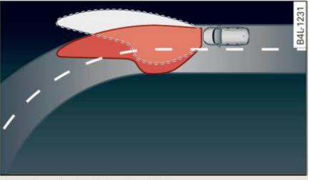
Fig. 48 Adaptive light when driving
