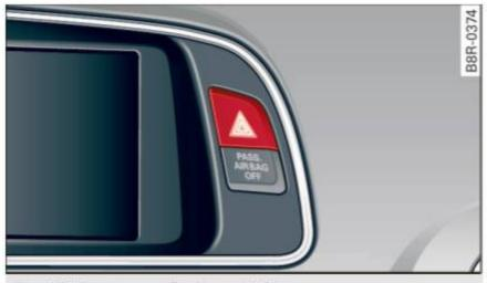
Fig. 49 Emergency flasher switch
