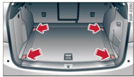
Fig. 75 Location of the tie-down rings in the luggage compartment
