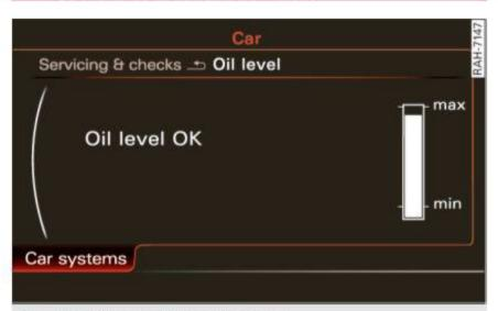
Fig. 198 Display: Oil level indicator
