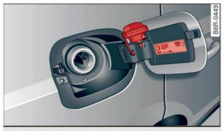
Fig. 191 Fuel filler flap with attached fuel cap
