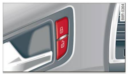
Fig. 32 Driver's door: power locking switch
