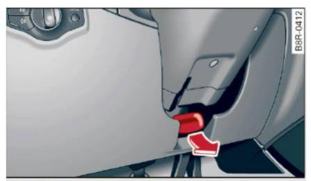
Fig. 98 Lever under the steering column
