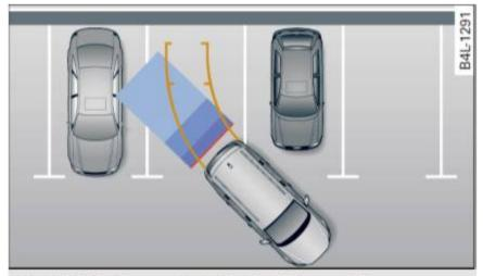
Fig. 141 Parking mode 1: Backing into a parking space
