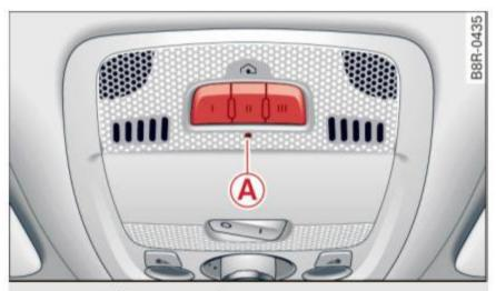
Fig. 44 Headliner: control unit
