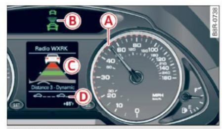
Fig. 121 Instrument cluster: adaptive cruise control
