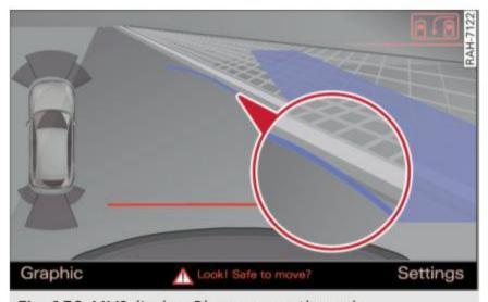
Fig. 150 MMI display: Blue curve on the curb
