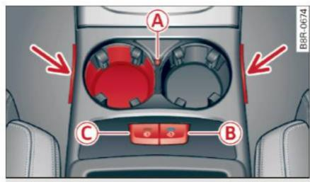
Fig. 87 Center console: climatized cupholder
