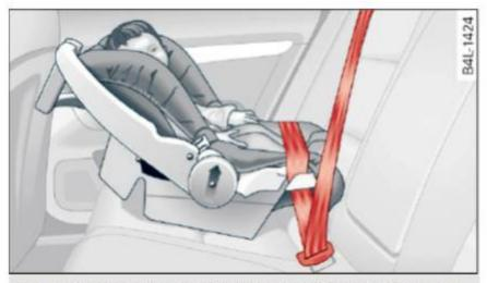
**Fig. 174** Schematic overview: rearward-facing infant seat, properly installed on the rear seat
