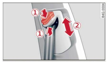
Fig. 164 Safety belt height adjustment for the front seats – loop-around fittings
