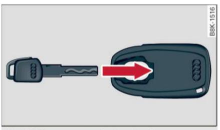
Fig. 101 Insert emergency key into the adapter
