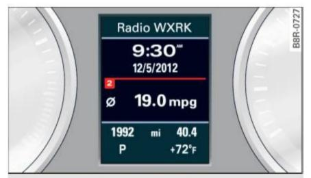
Fig. 9 Instrument cluster: center display
