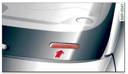
Fig. 236 Vehicle Identification Number (VIN) plate: location on driver's side dash panel
