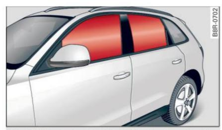
Fig. 172 Illustration of principle: Inflated side curtain airbags on the left side
