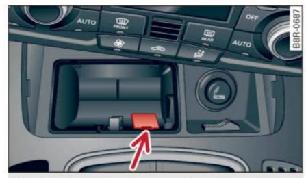
Fig. 140 Selector lever emergency release
