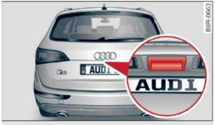
Fig. 35 Position of handle in the rear lid
