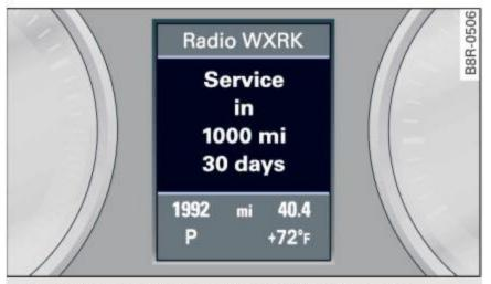
Fig. 14 Instrument cluster: Service interval display
