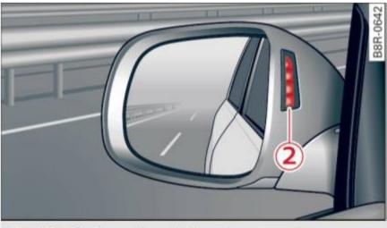
Fig. 128 Display on the exterior mirror
