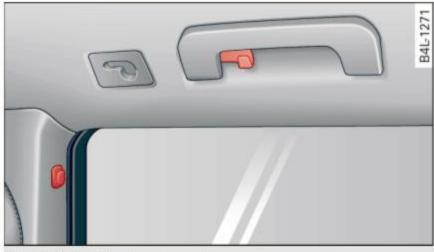
Fig. 96 Coat hooks at rear doors
