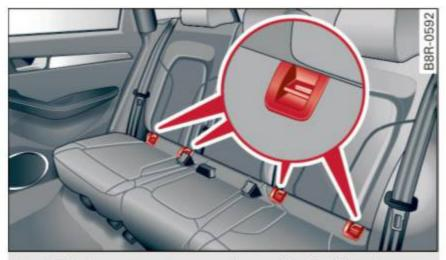
Fig. 180 Rear seats: lower anchorage bracket locations
