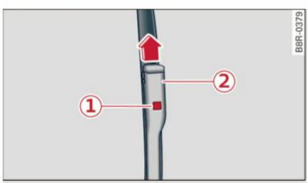
Fig. 58 Removing the wiper blade
