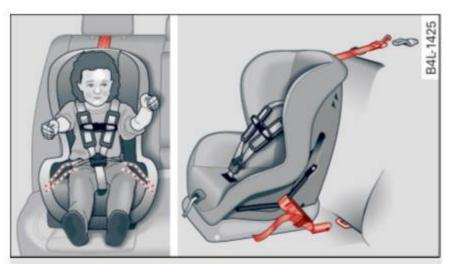
Fig. 175 Schematic overview: installation of the attachments applicable to a LATCH seat
