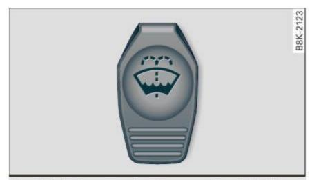
Fig. 203 Engine compartment: cover on the windshield and headlight\* washer fluid reservoir
