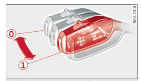
Fig. 120 Selector lever: switching on/off
