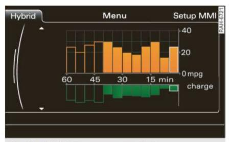
Fig. 114 MMI display: consumption display
