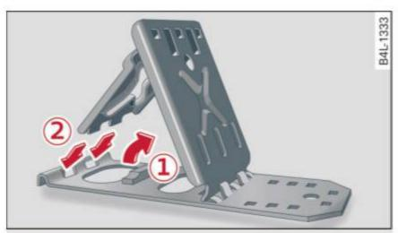
Fig. 210 Opening folding chocks
