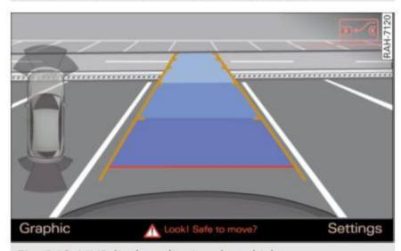
Fig. 148 MMI display: aligning the vehicle
