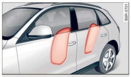
Fig. 170 Inflated side airbags on left side of vehicle
