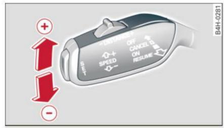
Fig. 122 Selector lever: changing the speed
