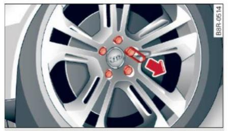
Fig. 217 Changing a wheel: removing the wheel bolt caps
