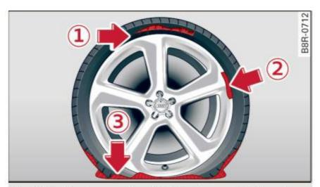
Fig. 214 Tire damage, for which the tire repair kit is not suitable
