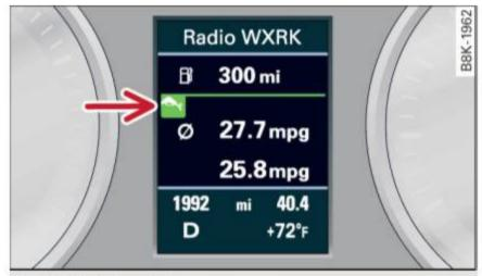
Fig. 18 Display: efficiency program
