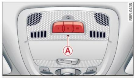
Fig. 44 Headliner: control unit
