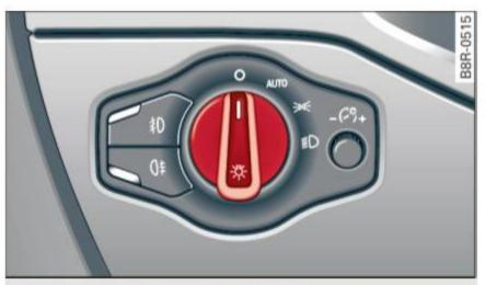
Fig. 46 Instrument panel: light switch
