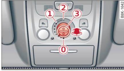
Fig. 42 Section from headliner: Knob for Panoramic sliding sunroof
