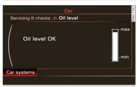
Fig. 198 Display: Oil level indicator
