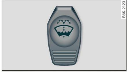
Fig. 203 Engine compartment: cover on the windshield and headlight\* washer fluid reservoir
