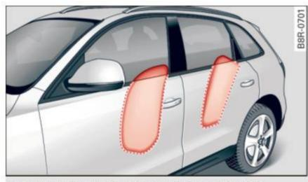
Fig. 170 Inflated side airbags on left side of vehicle
