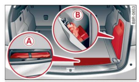
Fig. 115 Luggage compartment: vehicle tool bag and tire repair set
