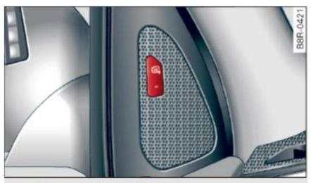
Fig. 131 Driver's door: Side assist button
