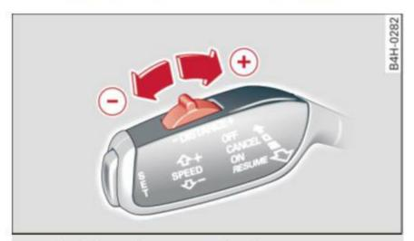
Fig. 124 Selector lever: setting the distance
