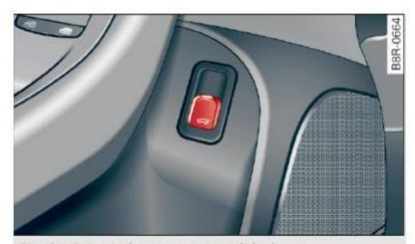
Fig. 34 Driver's door: remote rear lid release
