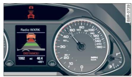
Fig. 125 Instrument cluster: request for driver intervention
