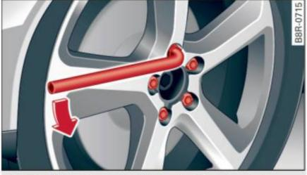
Fig. 218 Changing a wheel: loosening the wheel bolts
