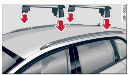
Fig. 82 Roof railing: positioning the roof rack
