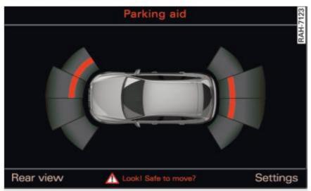
Fig. 146 MMI display: visual distance display
