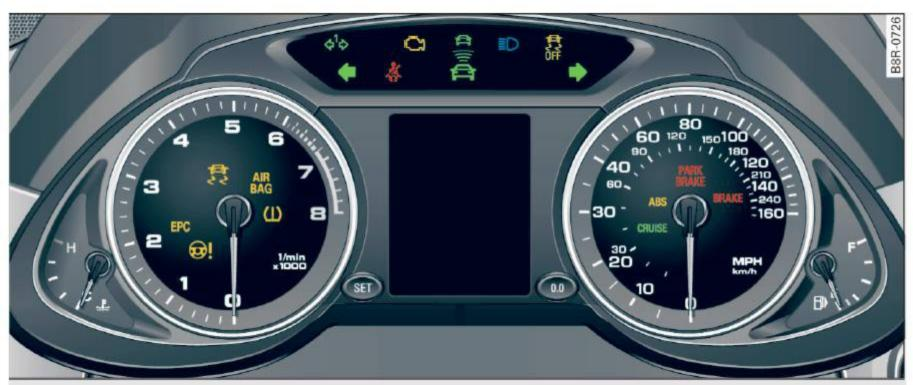
Fig. 8 Instrument cluster with warning/indicator lights
