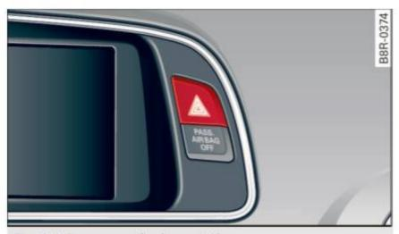
Fig. 49 Emergency flasher switch
