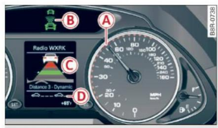
Fig. 121 Instrument cluster: adaptive cruise control
