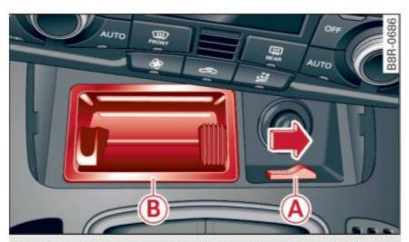
Fig. 139 Front center console: Removing the ashtray insert
