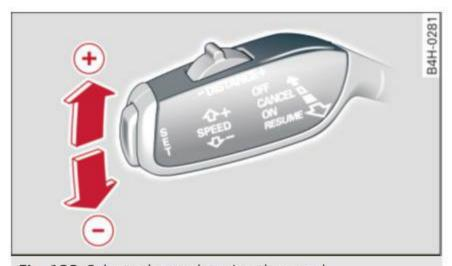
Fig. 122 Selector lever: changing the speed
