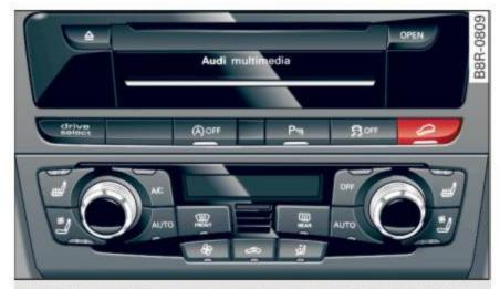
Fig. 187 Top of the center console: hill descent assist button
