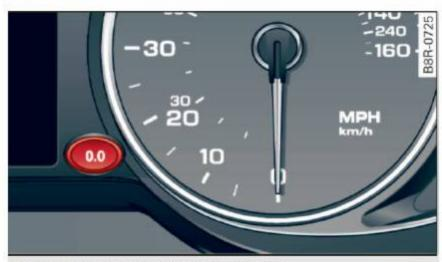
Fig. 7 Instrument cluster: reset button
