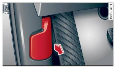
Fig. 195 Driver's side footwell: engine hood release lever
