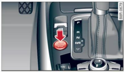
Fig. 102 Center console: START ENGINE STOP button
