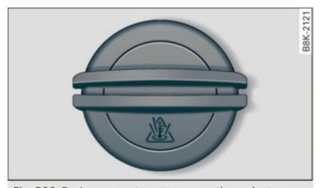
**Fig. 200** Engine compartment: cover on the coolant expansion tank
