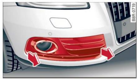
Fig. 229 Front bumper: removing the cover cap
