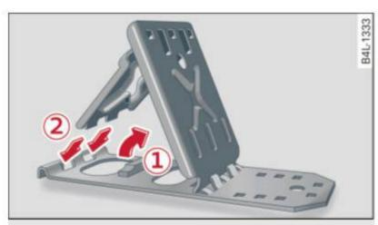
Fig. 212 Opening folding chocks
