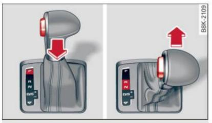
Fig. 132 Shift gate: selector lever lock positions and release button highlighted
