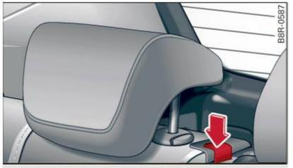
Fig. 70 Release button for the center backrest
