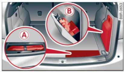
Fig. 112 Luggage compartment: vehicle tool bag and tire repair set
