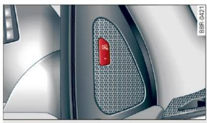
Fig. 128 Driver's door: Side assist button
