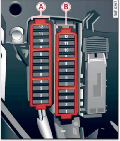
Fig. 227 Right cockpit: fuse panel with plastic clip
