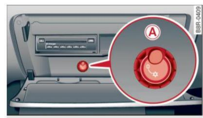
Fig. 91 Glove box with cooling box open and switched on
