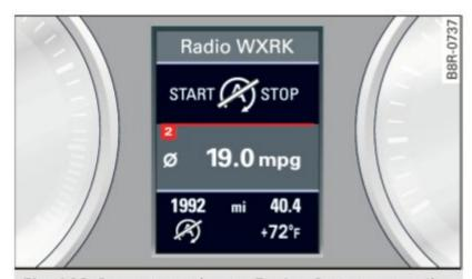
**Fig. 102** Instrument cluster: Engine-Stop temporarily unavailable
