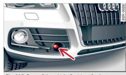
Fig. 113 Front of the vehicle: Position of radar sensor
