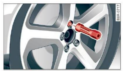
Fig. 223 Changing a wheel: using the screwdriver handle (with the blade removed) to turn the bolts
