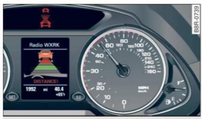
Fig. 122 Instrument cluster: request for driver intervention
