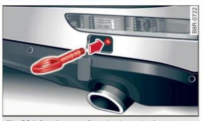
Fig. 234 Rear bumper: Screwing in towing loop
