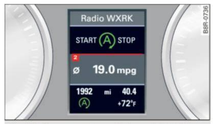
**Fig. 101** Instrument cluster: Engine switched off (stop phase)
