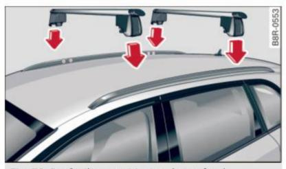
Fig. 79 Roof railing: positioning the roof rack
