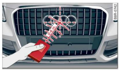
**Fig. 149** Distance between the radiator grille and the hand transmitter
