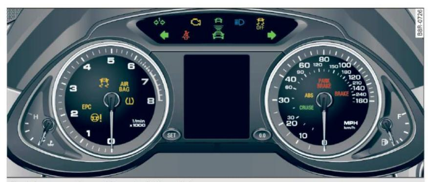
Fig. 8 Instrument cluster with warning/indicator lights
