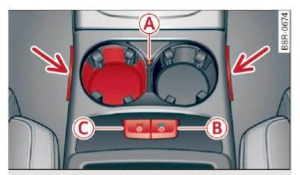
Fig. 84 Center console: climatized cupholder
