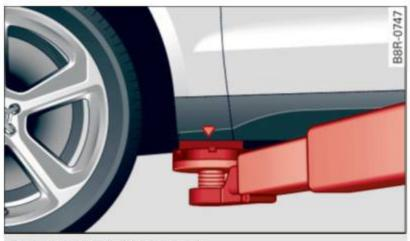
Fig. 236 Front lifting point
