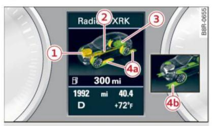
Fig. 109 Instrument cluster: energy flow display
