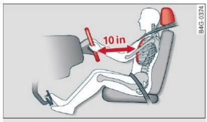
Fig. 151 Correct seating position
