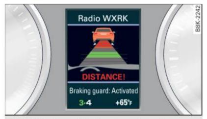
Fig. 123 Instrument cluster: approach warning
