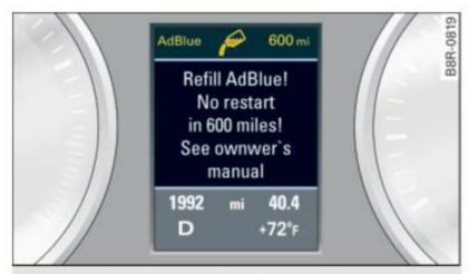
Fig. 193 Instrument cluster: indicator in the display
