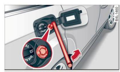
**Fig. 194** Right rear vehicle side: removing the AdBlue cap
