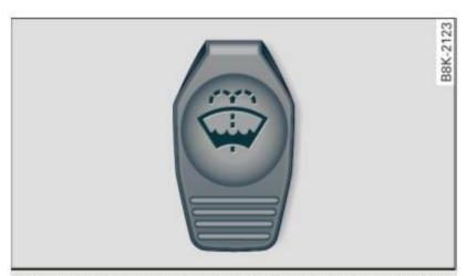
Fig. 204 Engine compartment: cover on the windshield and headlight\* washer fluid reservoir
