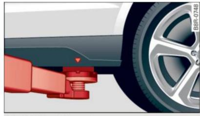
Fig. 237 Rear lifting point
