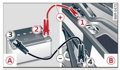
Fig. 230 Jump starting with the battery of another vehicle: (A) booster battery, (B) discharged vehicle battery
