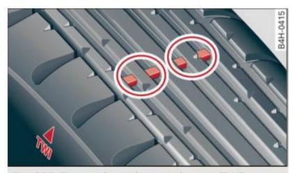
Fig. 207 Tire tread: tread wear indicators (TWI)
