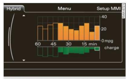
Fig. 111 MMI display: consumption display
