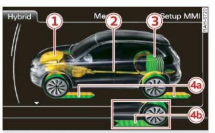
Fig. 110 MMI display: energy flow display
