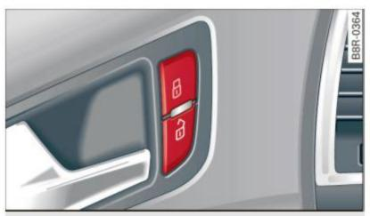
Fig. 32 Driver's door: power locking switch
