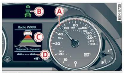
Fig. 118 Instrument cluster: adaptive cruise control
