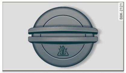
**Fig. 201** Engine compartment: cover on the coolant expansion tank
