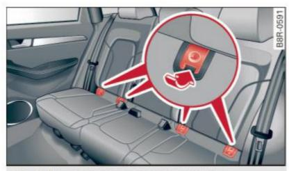
Fig. 179 Lower anchorages, covers marked
