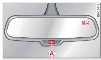
**Fig. 59** Inside rear view mirror: digital compass activated
