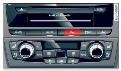
Fig. 142 Center console: Parking system switch
