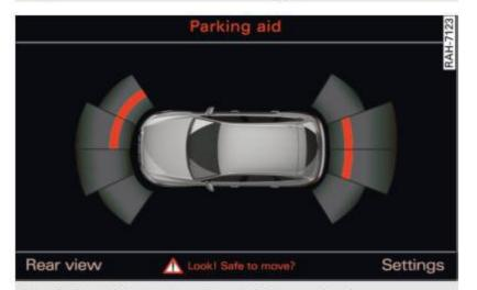
Fig. 143 MMI display: visual distance display
