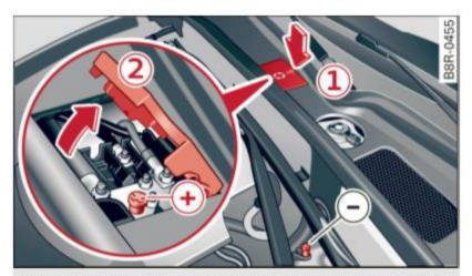
Fig. 203 Engine compartment: Connectors for charger and jumper cables
