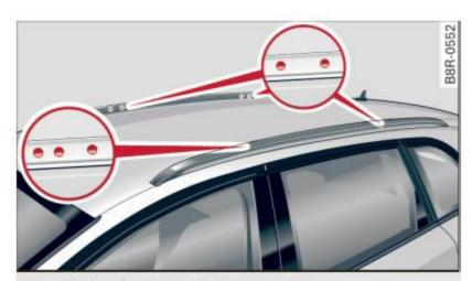
Fig. 78 Roof rack attachment points
