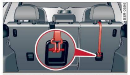
Fig. 184 Tether strap: proper routing and mounting
