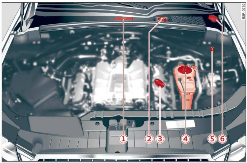
Fig. 198 Typical layout for containers and engine oil filler cap
