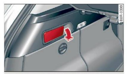
Fig. 71 Luggage compartment: release lever
