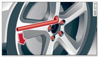
Fig. 220 Changing a wheel: loosening the wheel bolts
