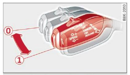
Fig. 117 Selector lever: switching on/off
