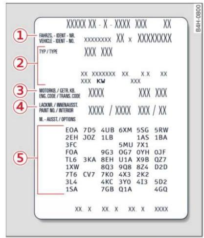
Fig. 239 Vehicle identification label: inside the luggage compartment
