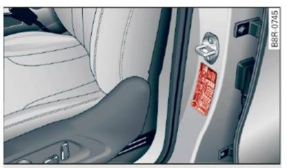
Fig. 205 Tire pressure label: located on driver's side Bpillar
