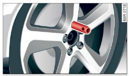
**Fig. 224** Changing a wheel: alignment pin inside the top hole
