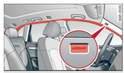
Fig. 171 Side curtain system, driver's side: side curtain airbag location
