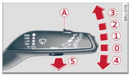
Fig. 53 Windshield wiper lever
