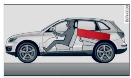
**Fig. 153** Safe load positioning: place heavy objects as low and as far forward as possible.
