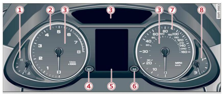
Fig. 3 Overview of the instrument cluster
