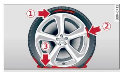
Fig. 216 Tire damage, for which the tire repair kit is not suitable
