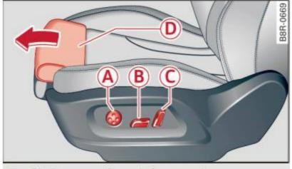
Fig. 61 Front seat: Controls for seat adjustment
