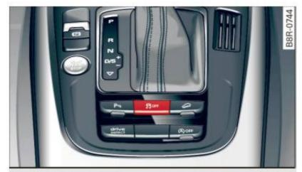
Fig. 185 Version A: Lower center console, 🗗 OFF button
