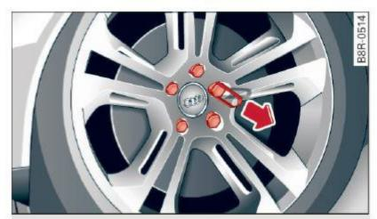
Fig. 219 Changing a wheel: removing the wheel bolt caps
