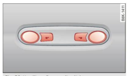
Fig. 50 Headliner: Rear reading lights
