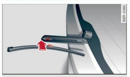
Fig. 56 Rear wiper: Removing the wiper blade
