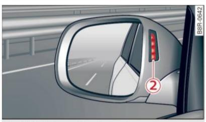
Fig. 125 Display on the exterior mirror
