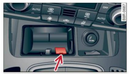
Fig. 137 Selector lever emergency release
