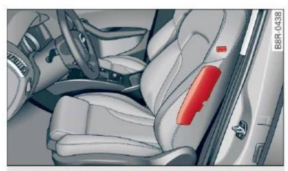
Fig. 169 Side airbag location in the driver's seat
