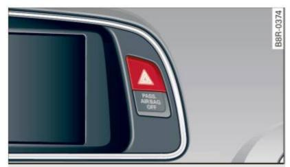
Fig. 47 Emergency flasher switch
