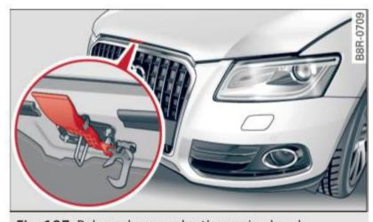
Fig. 197 Release lever under the engine hood
