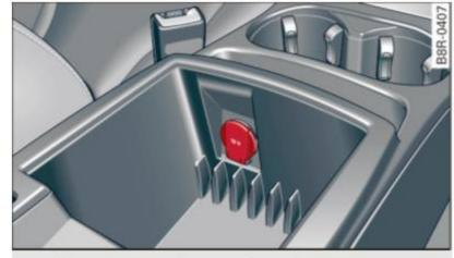
Fig. 89 Center console: 12-volt socket
