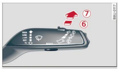
Fig. 54 Rear wiper actuation
