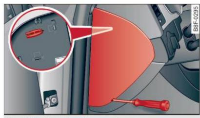
Fig. 225 Left cockpit: fuse panel cover
