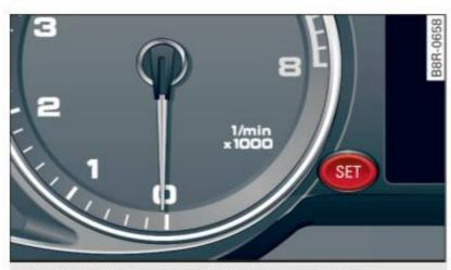
Fig. 104 SET button in the instrument cluster
