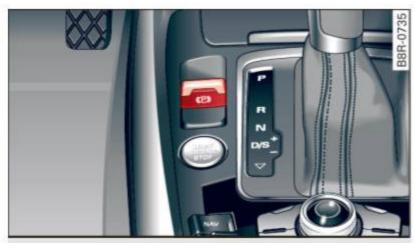
Fig. 100 Center console: Parking brake
