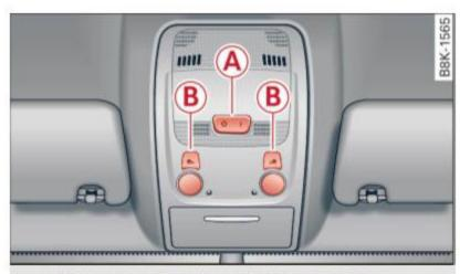
Fig. 49 Headliner: Front interior/reading lights
