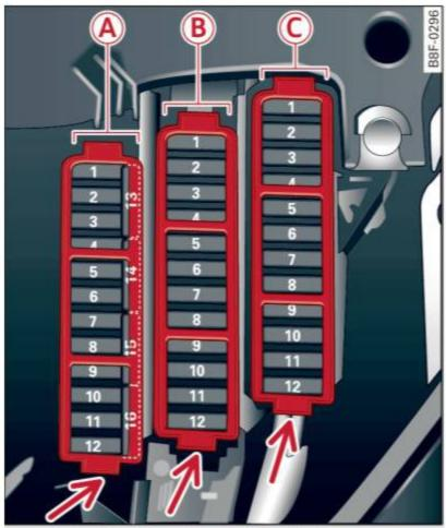
Fig. 226 Left cockpit: fuse panel with plastic clip
