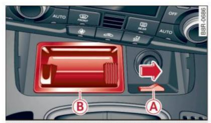
Fig. 136 Front center console: Removing the ashtray insert
