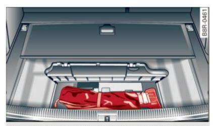
Fig. 211 Luggage compartment: onboard tool kit and vehicle jack
