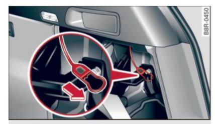
**Fig. 192** Luggage compartment: Emergency opening of fuel filler flap
