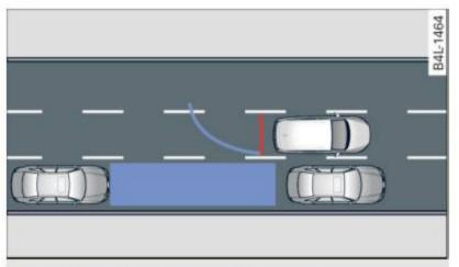
Fig. 139 Parking mode 2: parallel parking
