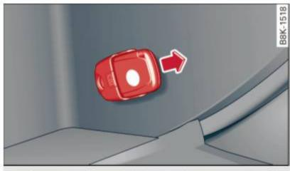
**Fig. 97** Glove compartment: Adapter for emergency key
