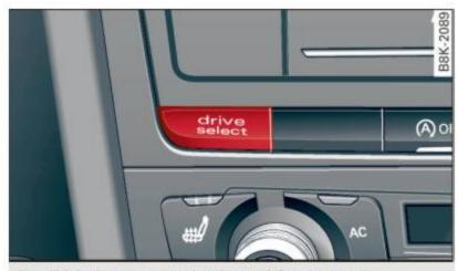
Fig. 129 Center console: Control for drive select
