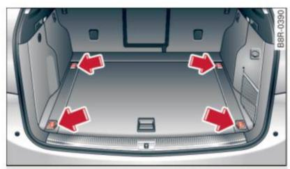
Fig. 72 Location of the tie-down rings in the luggage compartment
