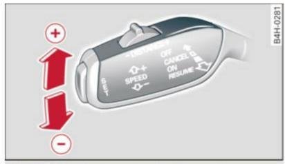
Fig. 119 Selector lever: changing the speed
