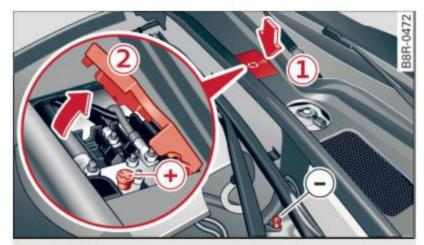
Fig. 229 Engine compartment: Connectors for jumper cables and charger
