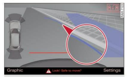
Fig. 147 MMI display: Blue curve on the curb
