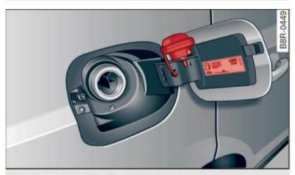
Fig. 191 Fuel filler flap with attached fuel cap
