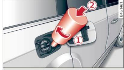
Fig. 195 AdBlue filler tube: inserting the refill bottle
