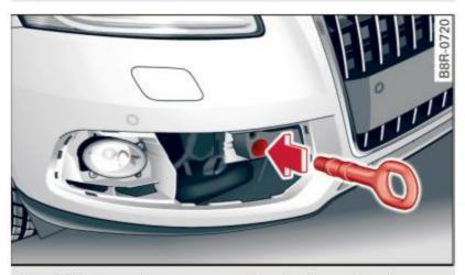
Fig. 232 Front bumper: screwing in the towing loop
