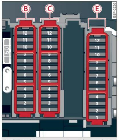
**Fig. 228** Right luggage compartment: fuse panel with plastic clip
