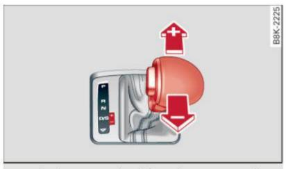
Fig. 134 Center console: shifting the gears manually
