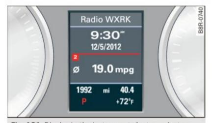
**Fig. 131** Display in the instrument cluster: selector lever in position P
