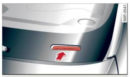
Fig. 238 Vehicle Identification Number (VIN) plate: location on driver's side dash panel
