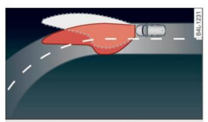
Fig. 46 Adaptive light when driving
