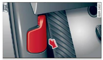
Fig. 196 Driver's side footwell: engine hood release lever
