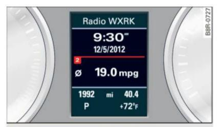
Fig. 9 Instrument cluster: center display
