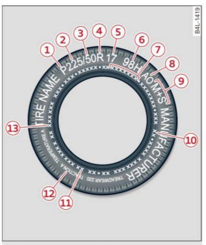
Fig. 209 Tire specification codes on the sidewall of a tire
