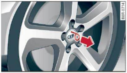
Fig. 218 Changing a wheel: Removing the wheel cover
