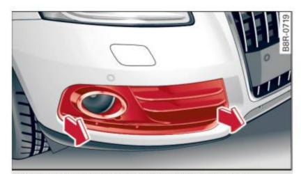
Fig. 231 Front bumper: removing the cover cap
