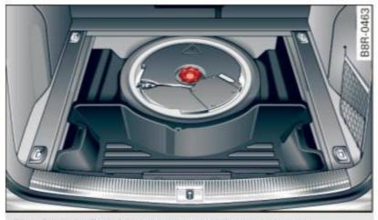
Fig. 214 Inflatable spare tire with compressor
