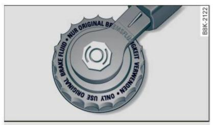
**Fig. 202** Engine compartment: cover on the brake fluid reservoir
