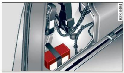
Fig. 215 Luggage compartment left side: compressor
