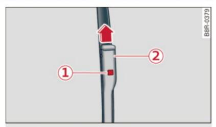
Fig. 55 Removing the wiper blade
