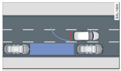
Fig. 153 Parking mode 2: parallel parking
