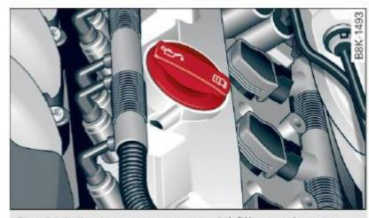
Fig. 210 Engine compartment: Oil filler cap location
