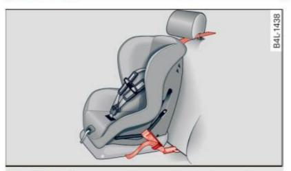
Fig. 196 Tether strap: proper routing and mounting
