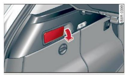
Fig. 76 Luggage compartment: release lever
