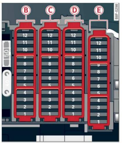
Fig. 237 Right luggage compartment: fuse panel with plastic clip
