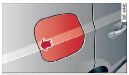
Fig. 203 Right rear vehicle side: Opening the fuel filler flap
