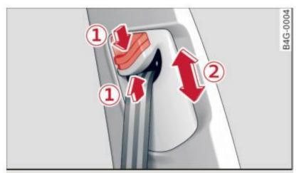
Fig. 178 Safety belt height adjustment for the front seats – loop-around fittings
