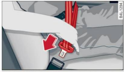
Fig. 174 Belt buckle and tongue on the driver's seat
