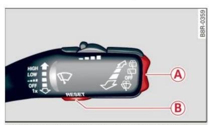
Fig. 17 Windshield wiper lever: controls for the trip computer
