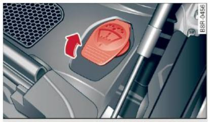
Fig. 214 Engine compartment: Windshield and headlight\* washer fluid container
