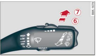
Fig. 59 Rear wiper actuation
