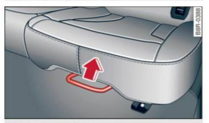
Fig. 69 Fore-and-aft adjustment
