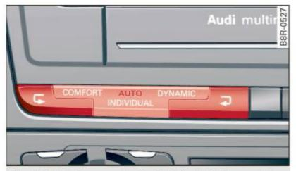
Fig. 143 Center console: Control for Audi drive select
