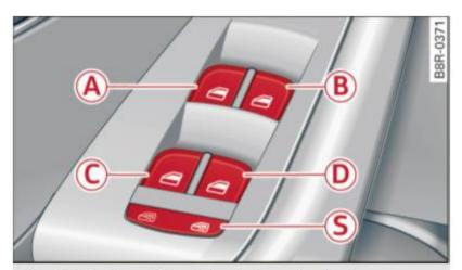
Fig. 45 Section of the driver's door: Controls
