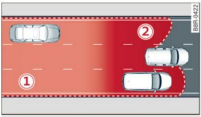
Fig. 135 Schematic illustration: Sensor detection area
