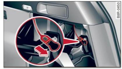
Fig. 205 Luggage compartment: Emergency opening of fuel filler flap
