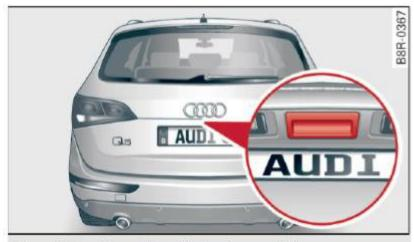
Fig. 40 Position of handle in the rear lid
