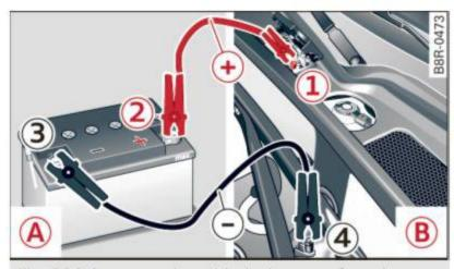
Fig. 239 Jump starting with the battery of another vehicle: (A) booster battery, (B) discharged vehicle battery
