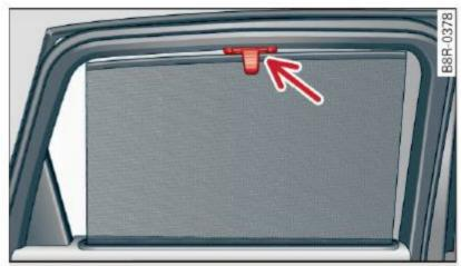
Fig. 57 Sun shade pulled up on a rear window
