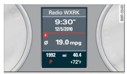
**Fig. 145** Display in the instrument cluster: selector lever in position P
