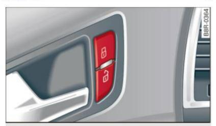
Fig. 37 Driver's door: power locking switch
