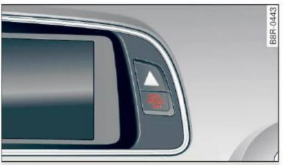
Fig. 182 Section from the instrument panel: PASSEN-GER AIR BAG OFF light
