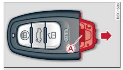
Fig. 29 Remote master key: Removing the battery holder
