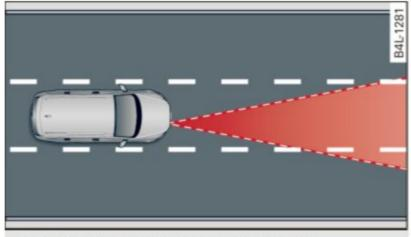
Fig. 113 Radar sensor measurement range
