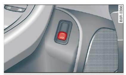
Fig. 39 Driver's door: remote rear lid release
