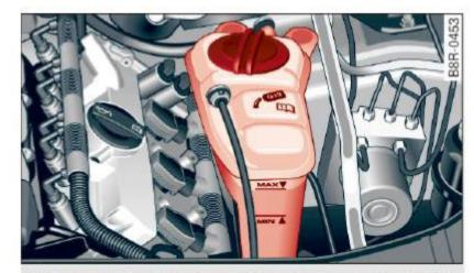
Fig. 211 Engine compartment: Coolant expansion tank
