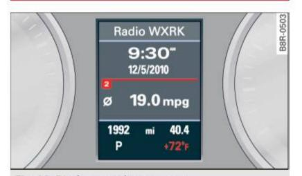
Fig. 11 Display: outside temperature
