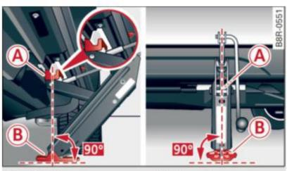
Fig. 231 Close-up: proper positioning of jack
