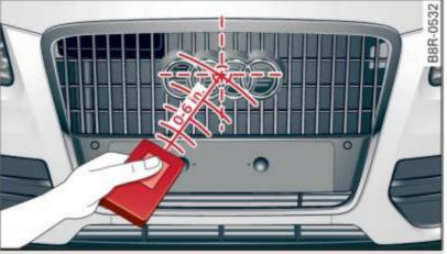
Fig. 163 Radiator grille: location of transmitter unit
