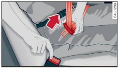
Fig. 177 Releasing the tongue from the buckle
