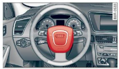
Fig. 179 Location of driver airbag: in steering wheel
