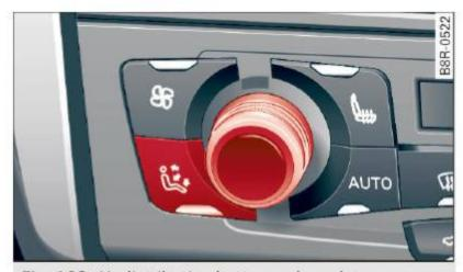
Fig. 103 Air distribution button and regulator
