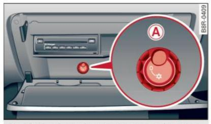
Fig. 96 Glove box with cooling box open and switched on
