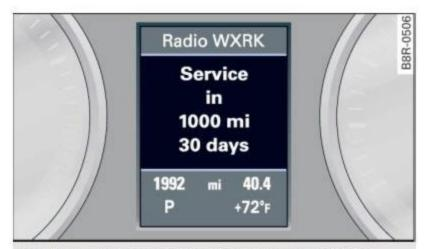
Fig. 14 Instrument cluster: Service interval display
