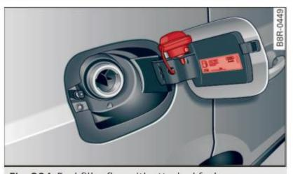
Fig. 204 Fuel filler flap with attached fuel cap
