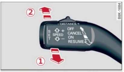
Fig. 114 Control lever: Switching on and off
