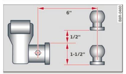
Fig. 202 Permitted ball position of the trailer hitch
