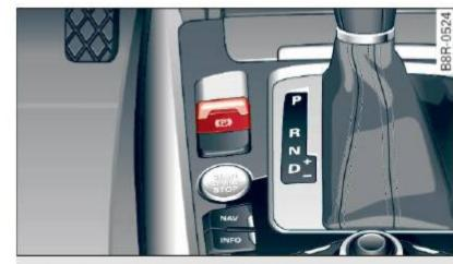
Fig. 109 Center console: Parking brake
