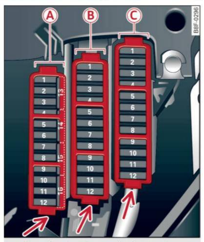
Fig. 235 Left cockpit: fuse panel with plastic clip
