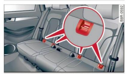
Fig. 193 Rear seats: lower anchorage bracket locations
