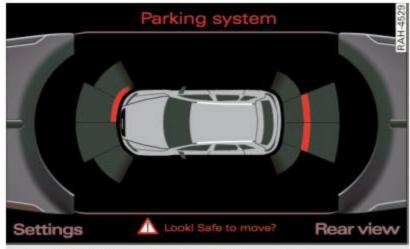
Fig. 157 MMI display: visual distance display
