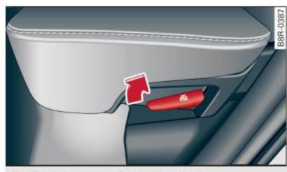
Fig. 74 Release lever for the outer backrest
