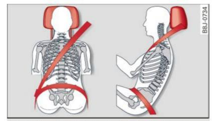
Fig. 175 Head restraint and safety belt position as seen from the side
