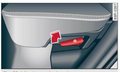
Fig. 68 Adjusting seatback angle
