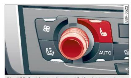
Fig. 105 Seat heating/seat ventilation button and regulator
