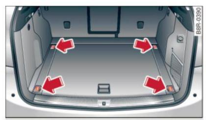
Fig. 77 Location of the tie-down rings in the luggage compartment
