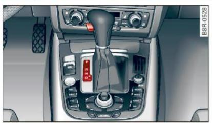
Fig. 144 Shift gate on the center console: selector lever with release button
