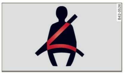
**Fig. 168** Safety belt warning light in the instrument cluster - enlarged
