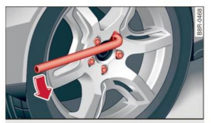
Fig. 229 Changing a wheel: loosening the wheel bolts
