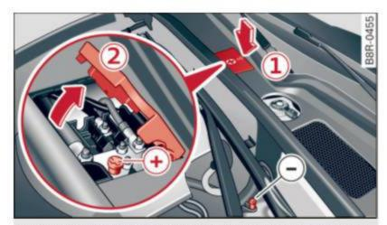
Fig. 213 Engine compartment: Connectors for charger and jumper cables
