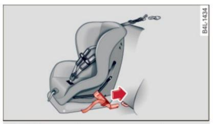
Fig. 194 Lower anchorages: proper mounting
