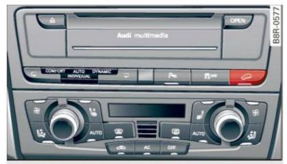
Fig. 200 Top of the center console: hill descent assist button
