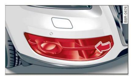
Fig. 240 Front bumper: removing the cover cap
