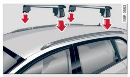
Fig. 84 Roof railing: positioning the roof rack
