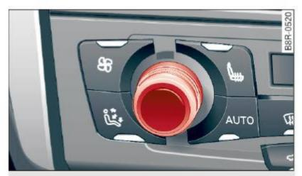
Fig. 101 Temperature setting regulator
