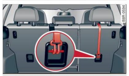
Fig. 197 Tether strap: proper routing and mounting
