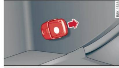
**Fig. 32** Glove compartment: Adapter for emergency key
