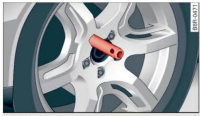
Fig. 233 Changing a wheel: alignment pin inside the top hole
