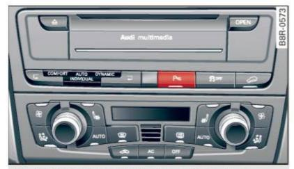
Fig. 156 Center console: Parking system switch
