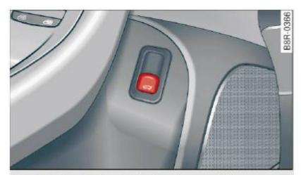
Fig. 41 Driver's door: Unlocking the rear lid
