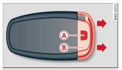
Fig. 30 Remote master key: Removing the mechanical key
