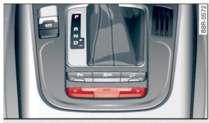
Fig. 142 Shift gate: Control for Audi drive select
