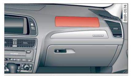
Fig. 180 Location of front passenger's airbag: in the instrument panel
