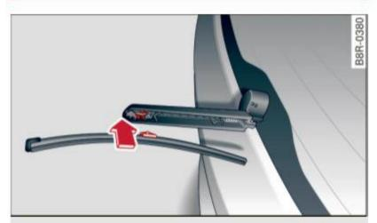
Fig. 61 Rear wiper: Removing the wiper blade
