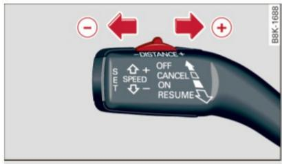
Fig. 118 Control lever: Setting distance
