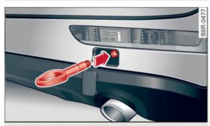
Fig. 243 Rear bumper: Screwing in towing loop
