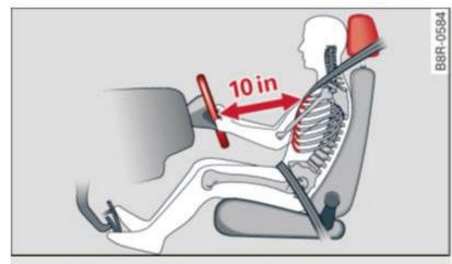
Fig. 165 Correct seating position
