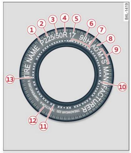
Fig. 219 Tire specification codes on the sidewall of a tire
