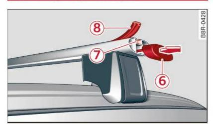
Fig. 86 Roof railing: installing cover profile into the roof rack
