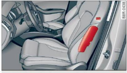
Fig. 183 Side airbag location in the driver's seat
