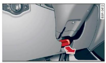
Fig. 106 Lever under the steering column
