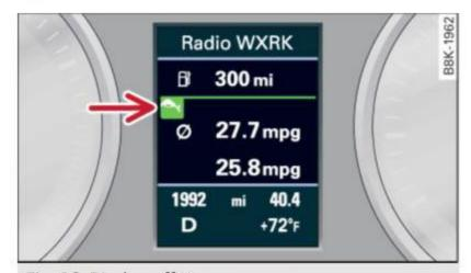
Fig. 18 Display: efficiency program
