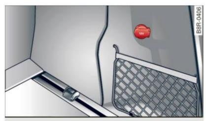
Fig. 93 Section of the trim panel of the luggage compartment: 12-volt socket
