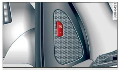
Fig. 134 Driver's door: Side assist button
