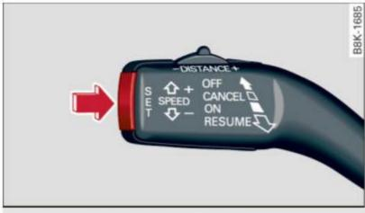
Fig. 115 Control lever: Storing speed
