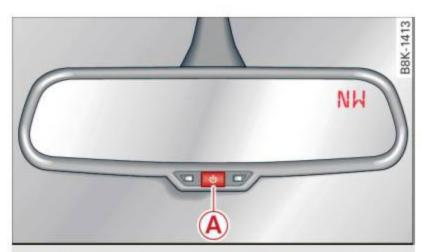
Fig. 64 Inside rear view mirror: digital compass activated
