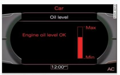
Fig. 209 Display: Oil level indicator
