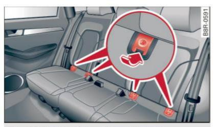
Fig. 192 Lower anchorages, covers marked
