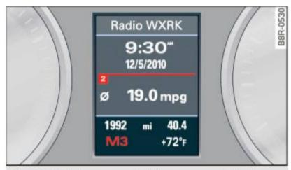
Fig. 148 Display: manual shift program, selected gear
