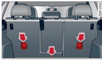
**Fig. 195** Tether anchors: attachment hook locations behind the rear seatbacks
