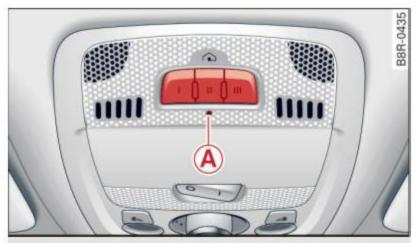
Fig. 162 Overhead console: HomeLink® keypad
