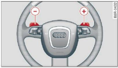
Fig. 149 Steering wheel: Shift buttons
