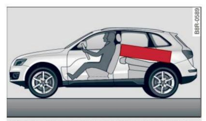
**Fig. 167** Safe load positioning: place heavy objects as low and as far forward as possible.
