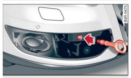
Fig. 241 Front bumper: screwing in the towing loop
