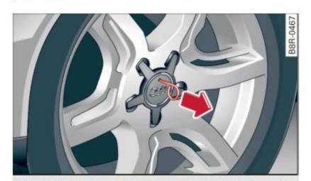
Fig. 227 Changing a wheel: Removing the wheel cover
