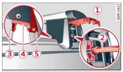
Fig. 85 Roof railing: installing a roof rack
