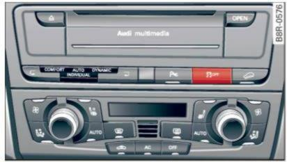
**Fig. 199** Version B: at the top of the center console, 昂 OFF button
