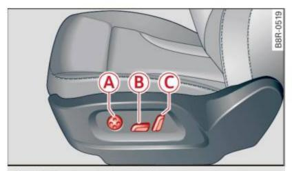
Fig. 66 Front seat: Controls for seat adjustment
