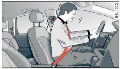
Fig. 173 Driver is correctly restrained in a sudden braking maneuver
