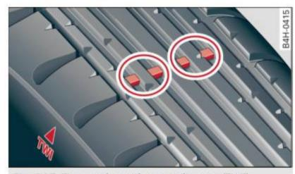
Fig. 217 Tire tread: tread wear indicators (TWI)
