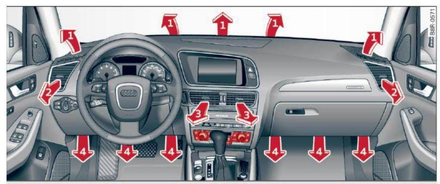
Fig. 104 Instrument panel: Location of air vents
