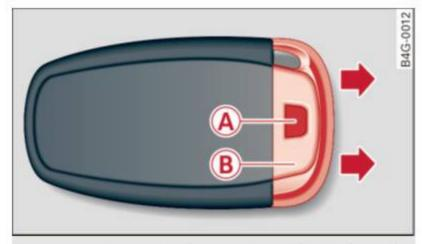
Fig. 28 Remote master key: Removing the mechanical key
