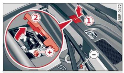
Fig. 238 Engine compartment: Connectors for jumper cables and charger
