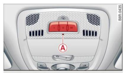
Fig. 164 Overhead console: HomeLink® keypad
