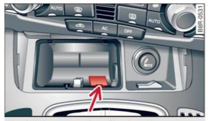
Fig. 151 Emergency release for selector lever
