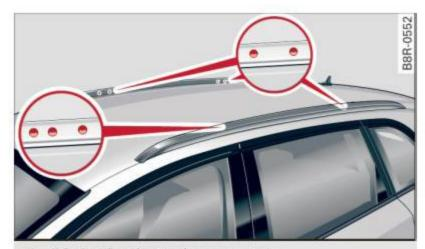
Fig. 83 Roof rack attachment points
