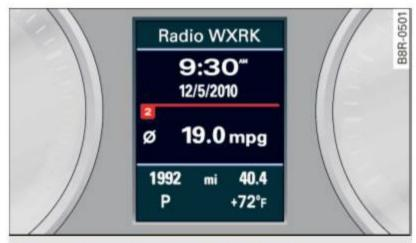
Fig. 9 Instrument cluster: center display
