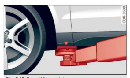
Fig. 245 Front lifting point
