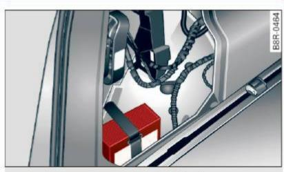
Fig. 226 Luggage compartment left side: compressor
