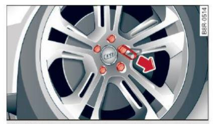
Fig. 228 Changing a wheel: removing the wheel bolt caps
