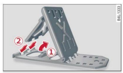
Fig. 223 Opening folding chocks
