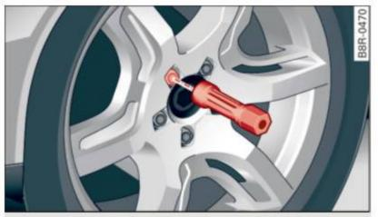
Fig. 232 Changing a wheel: using the screwdriver handle (with the blade removed) to turn the bolts
