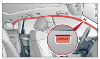
Fig. 185 Side curtain system, driver's side: side curtain airbag location
