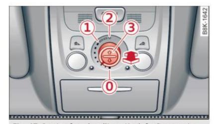
Fig. 47 Section from headliner: Knob for Panoramic sliding sunroof
