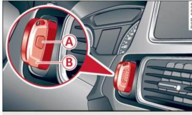
Fig. 31 Ignition switch with ignition key
