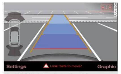
Fig. 159 MMI display: aligning the vehicle
