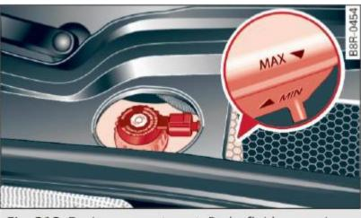
Fig. 212 Engine compartment: Brake fluid reservoir
