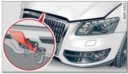
Fig. 207 Release lever under the engine hood
