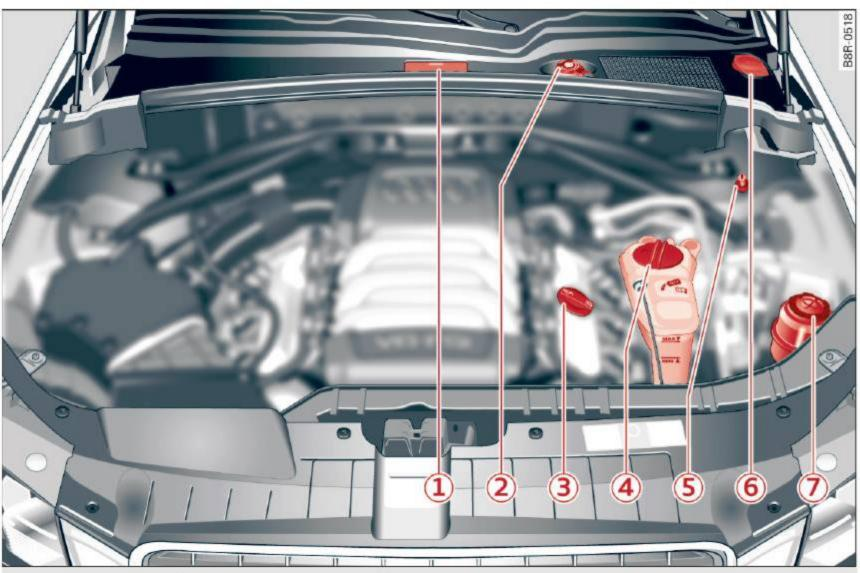
Fig. 208 Typical layout for containers and engine oil filler cap
