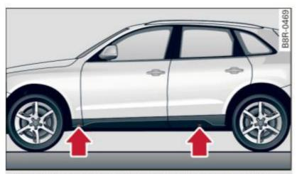
Fig. 230 Changing a wheel: mounting points for the iack
