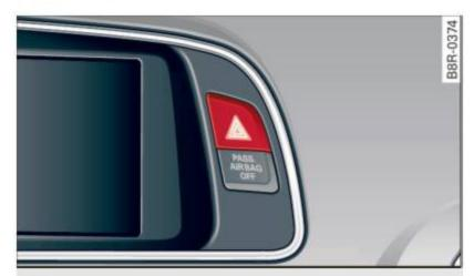
Fig. 52 Emergency flasher switch
