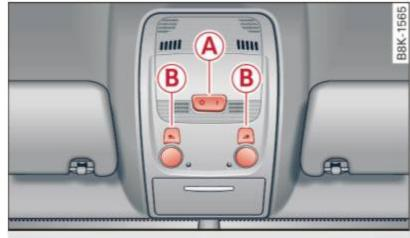
Fig. 54 Headliner: Front interior/reading lights
