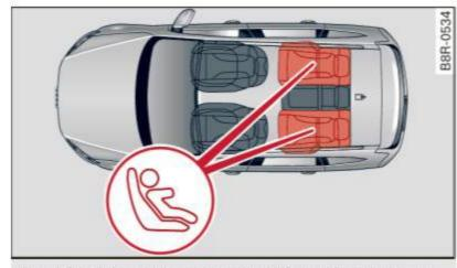
Fig. 191 Schematic overview: LATCH anchorage point locations
