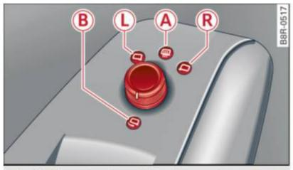
Fig. 62 Forward section of driver's armrest: power mirror controls
