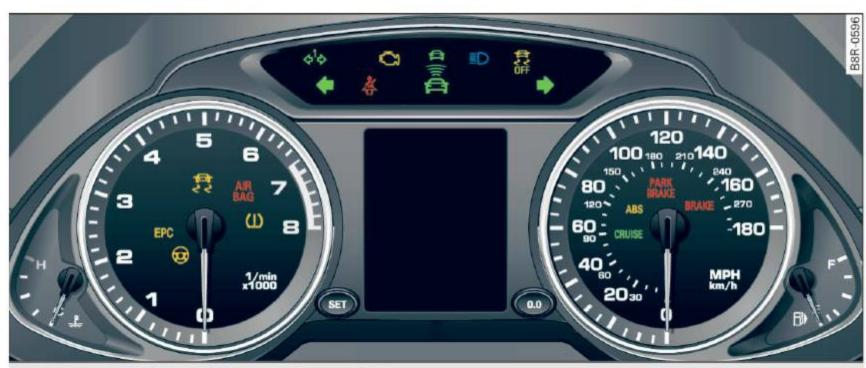
Fig. 8 Instrument cluster with warning/indicator lights
