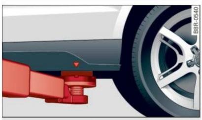
Fig. 246 Rear lifting point
