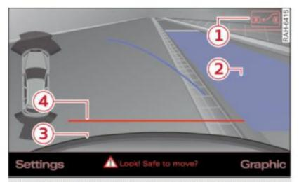
Fig. 160 MMI display: blue surface in the parking spot
