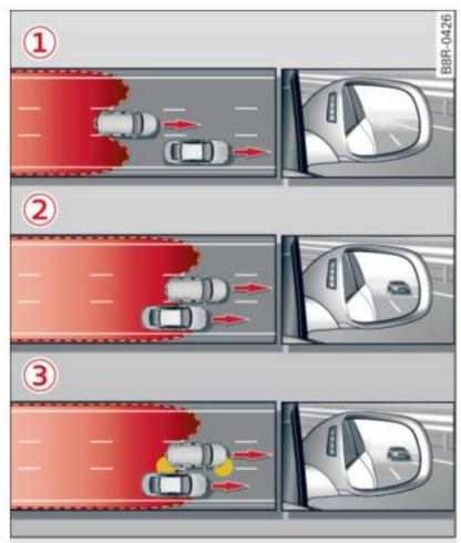
Fig. 139 Side assist: Vehicles dropping back quickly
