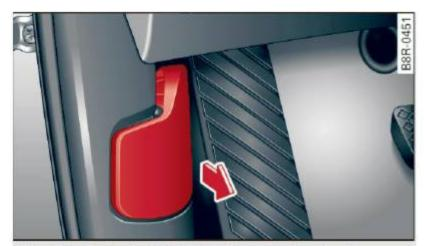
Fig. 206 Driver's side footwell: engine hood release lever
