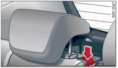
Fig. 75 Release button for the center backrest
