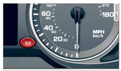
Fig. 7 Instrument cluster: reset button
