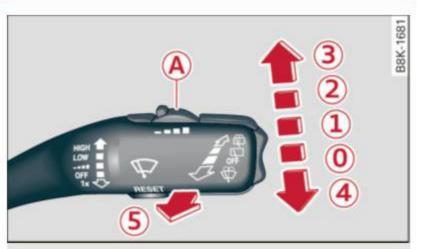
Fig. 58 Windshield wiper lever
