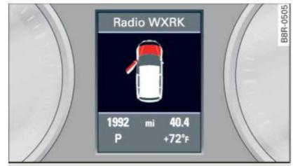
Fig. 13 Display: Open door- and trunk lid warning
