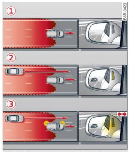
Fig. 136 Side assist: Fast approaching vehicles
