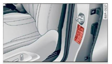
Fig. 215 Tire pressure label: located on driver's side Bpillar
