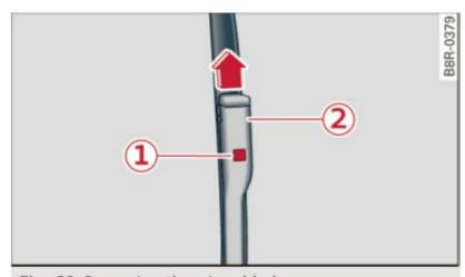
Fig. 60 Removing the wiper blade
