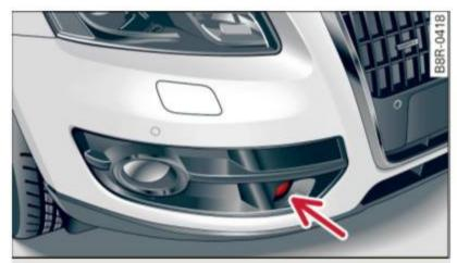
Fig. 112 Front bumper: Position of radar sensor
