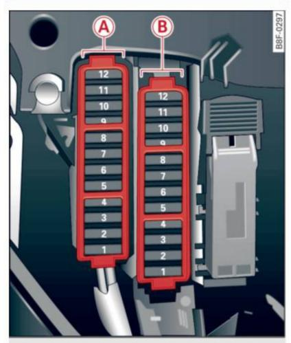
Fig. 236 Right cockpit: fuse panel with plastic clip
