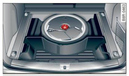
Fig. 225 Inflatable spare tire with compressor
