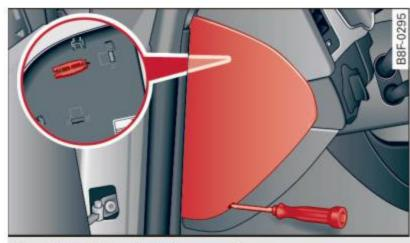
Fig. 234 Left cockpit: fuse panel cover
