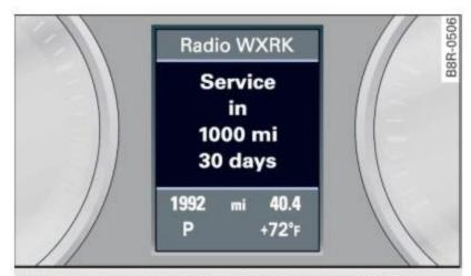
Fig. 14 Instrument cluster: Service interval display
