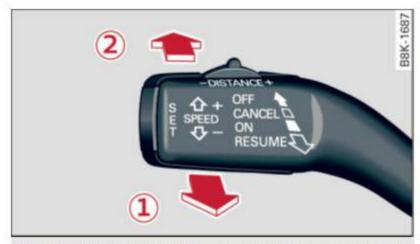
Fig. 116 Control lever: Turning adaptive cruise control off temporarily
