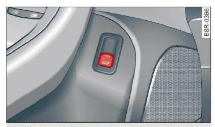
Fig. 39 Driver's door: remote rear lid release
