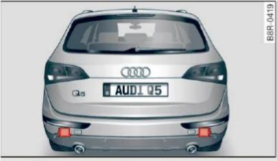
**Fig. 131** Rear bumper: Position of radar sensors (not visible on outside)
