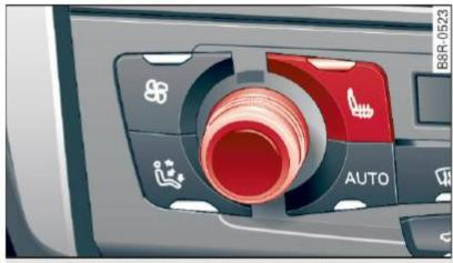
Fig. 104 Seat heating button and regulator
