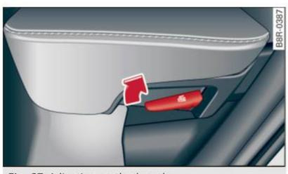
Fig. 67 Adjusting seatback angle
