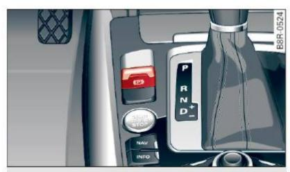
Fig. 108 Center console: Parking brake
