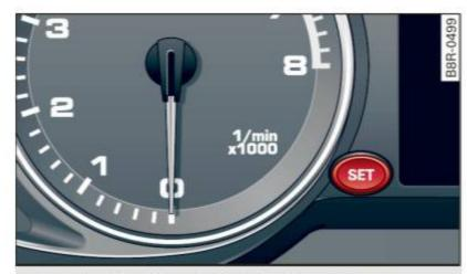
Fig. 4 SET button in the instrument cluster
