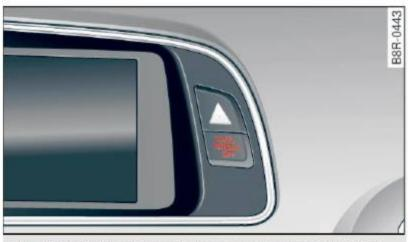
Fig. 181 Section from the instrument panel: PASSEN-GER AIR BAG OFF light
