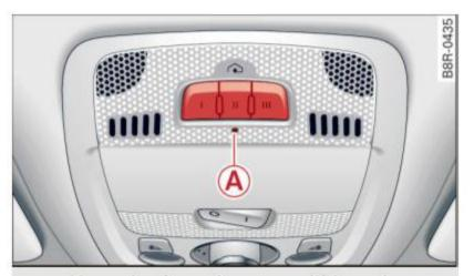
Fig. 163 Overhead console: HomeLink® keypad
