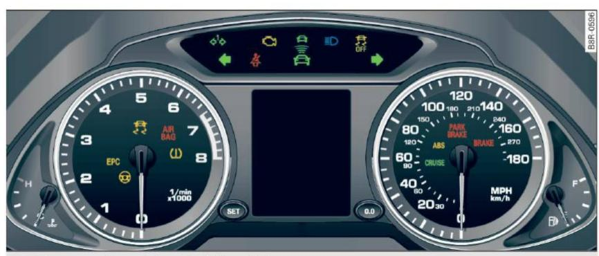
Fig. 8 Instrument cluster with warning/indicator lights
