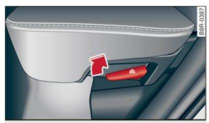
Fig. 73 Release lever for the outer backrest
