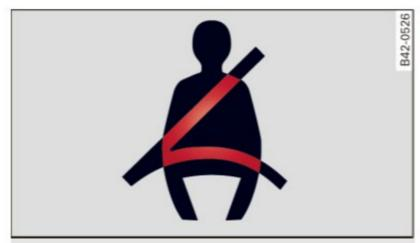
**Fig. 167** Safety belt warning light in the instrument cluster - enlarged
