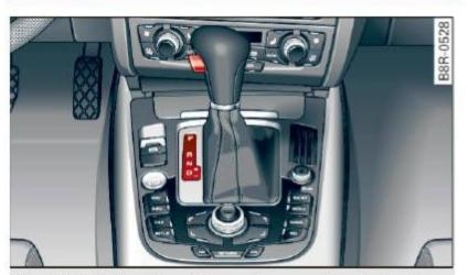
**Fig. 143** Shift gate on the center console: selector lever with release button
