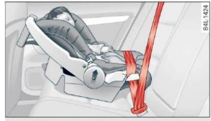
Fig. 186 Schematic overview: rearward-facing infant seat, properly installed on the rear seat
