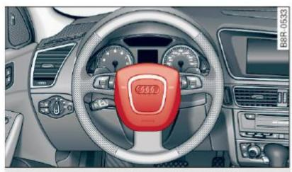
Fig. 178 Location of driver airbag: in steering wheel
