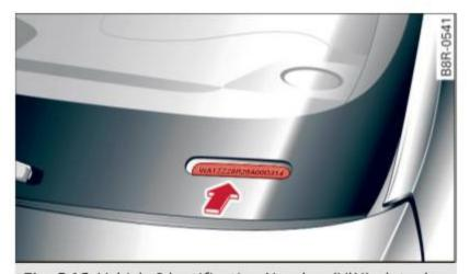
Fig. 246 Vehicle Identification Number (VIN) plate: location on driver's side dash panel
