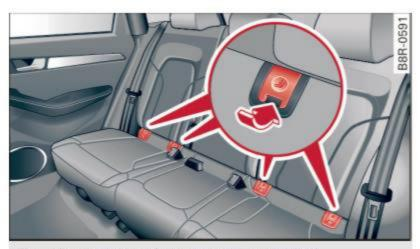
Fig. 191 Lower anchorages, covers marked
