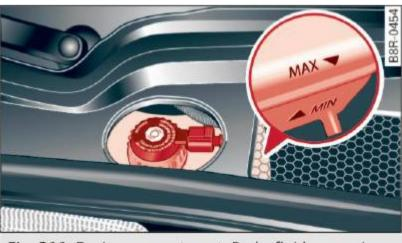
Fig. 211 Engine compartment: Brake fluid reservoir
