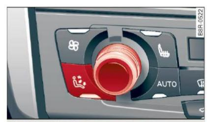
Fig. 102 Air distribution button and regulator
