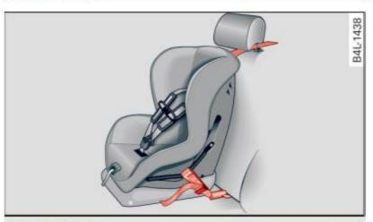
Fig. 195 Tether strap: proper routing and mounting
