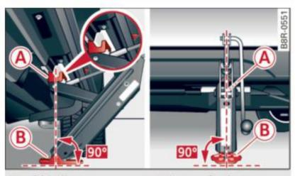
Fig. 230 Close-up: proper positioning of jack
