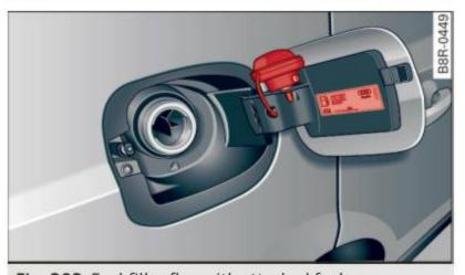
Fig. 203 Fuel filler flap with attached fuel cap
