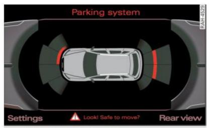
Fig. 156 MMI display: visual distance display
