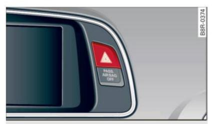
Fig. 52 Emergency flasher switch
