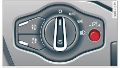
Fig. 50 Instrument lighting
