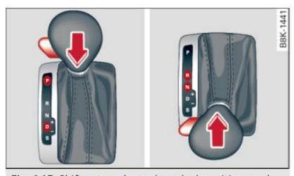
**Fig. 145** Shift gate: selector lever lock positions and interlock button highlighted
