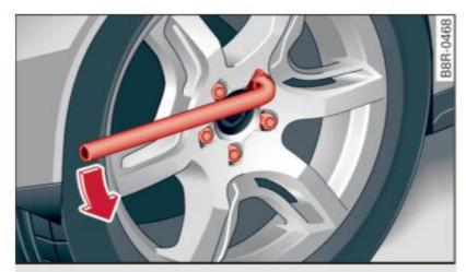
Fig. 228 Changing a wheel: loosening the wheel bolts
