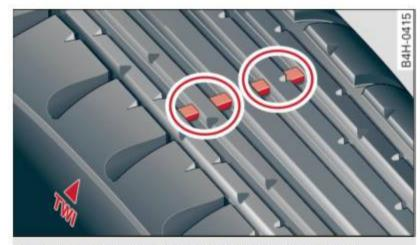
Fig. 216 Tire tread: tread wear indicators (TWI)
