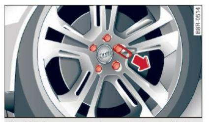
Fig. 227 Changing a wheel: removing the wheel bolt caps
