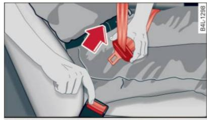
Fig. 176 Releasing the tongue from the buckle
