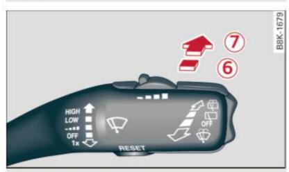
Fig. 58 Rear wiper actuation
