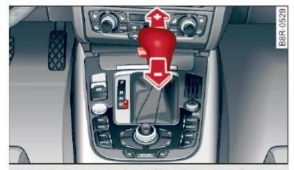
Fig. 146 Center console: shifting the tiptronic® manually
