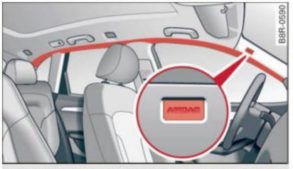
**Fig. 184** Side curtain system, driver's side: side curtain airbag location
