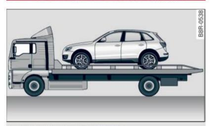
Fig. 243 Vehicle on flat bed truck
