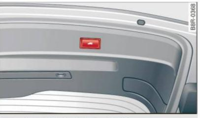
Fig. 42 Locking switch in the rear lid
