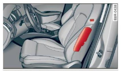
Fig. 182 Side airbag location in the driver's seat
