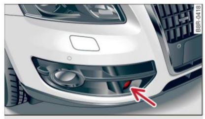
Fig. 111 Front bumper: Position of radar sensor
