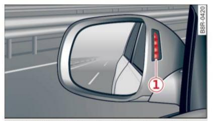
Fig. 132 Signal light on the outside mirror - driver's side
