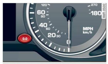
Fig. 7 Instrument cluster: reset button
