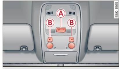
Fig. 54 Headliner: Front interior/reading lights
