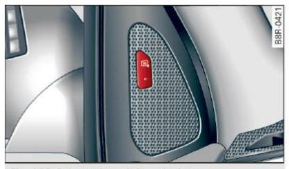
Fig. 133 Driver's door: Side assist button
