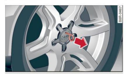
Fig. 226 Changing a wheel: Removing the wheel cover
