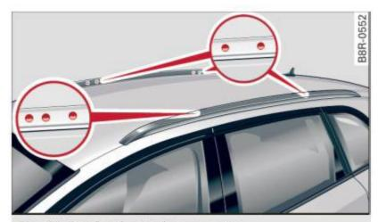
Fig. 82 Roof rack attachment points
