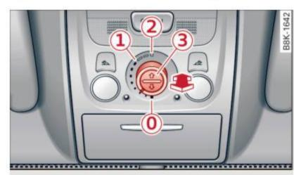
**Fig. 47** Section from headliner: Knob for Panoramic sliding sunroof
