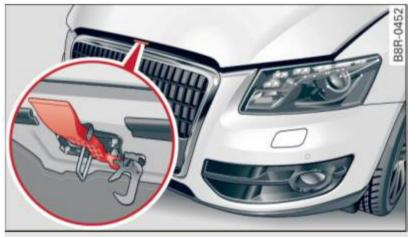
Fig. 206 Release lever under the engine hood
