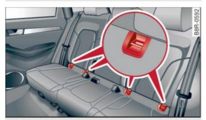
Fig. 192 Rear seats: lower anchorage bracket locations
