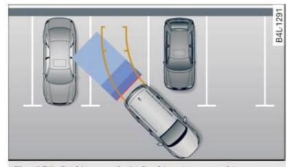
Fig. 151 Parking mode 1: Backing into a parking space
