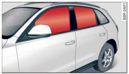
Fig. 185 Illustration of principle: Inflated side curtain airbags on the left side
