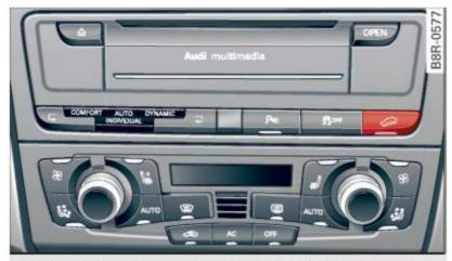
Fig. 199 Top of the center console: hill descent assist button
