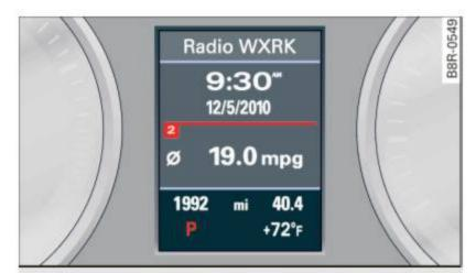
Fig. 144 Display in the instrument cluster: selector lever in position P
