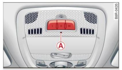
Fig. 161 Overhead console: HomeLink® keypad
