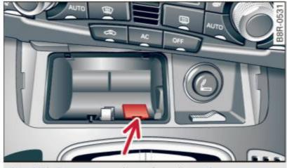
Fig. 150 Emergency release for selector lever
