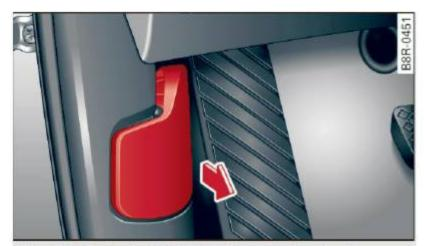
Fig. 205 Driver's side footwell: engine hood release lever
