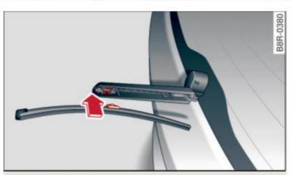
Fig. 60 Rear wiper: Removing the wiper blade
