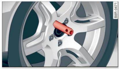
Fig. 232 Changing a wheel: alignment pin inside the top hole
