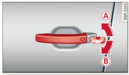
Fig. 46 Key turns for opening and closing
