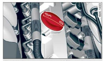
Fig. 209 Engine compartment: Oil filler cap location
