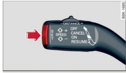
Fig. 114 Control lever: Storing speed
