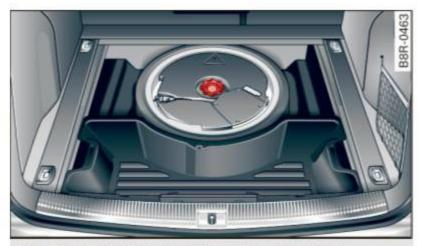
Fig. 224 Inflatable spare tire with compressor
