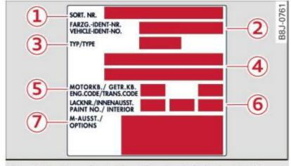
**Fig. 247** The vehicle identification label – inside the luggage compartment
