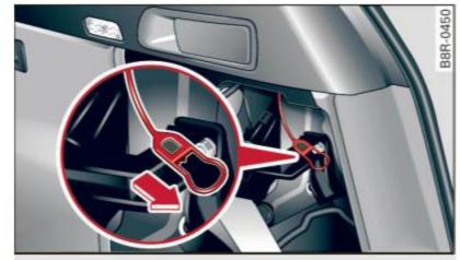
Fig. 204 Luggage compartment: Emergency opening of fuel filler flap
