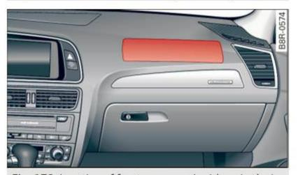
Fig. 179 Location of front passenger's airbag: in the instrument panel
