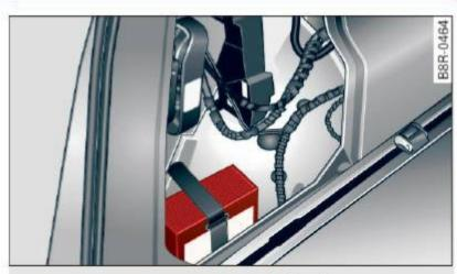
Fig. 225 Luggage compartment left side: compressor
