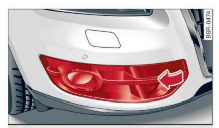
Fig. 239 Front bumper: removing the cover cap
