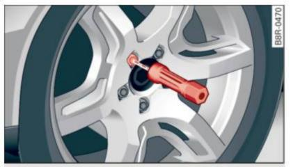
Fig. 231 Changing a wheel: using the screwdriver handle (with the blade removed) to turn the bolts
