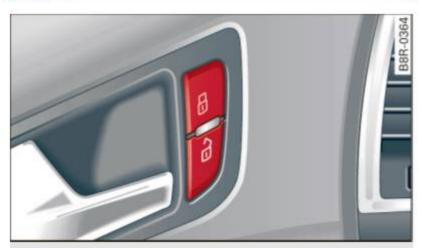
Fig. 37 Driver's door: power locking switch
