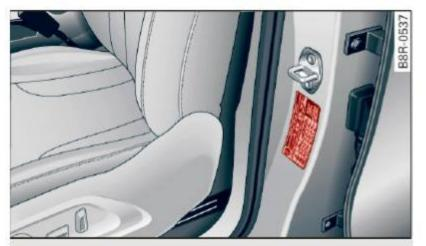
Fig. 214 Tire pressure label: located on driver's side Bpillar
