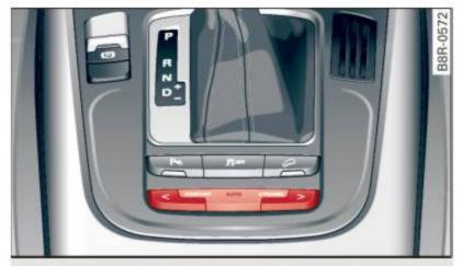
Fig. 141 Shift gate: Control for Audi drive select
