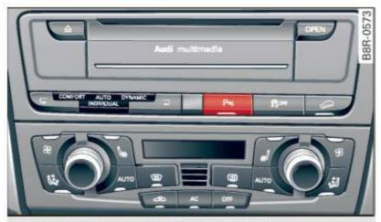
Fig. 155 Center console: Parking system switch
