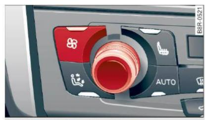
Fig. 101 Fan button and regulator
