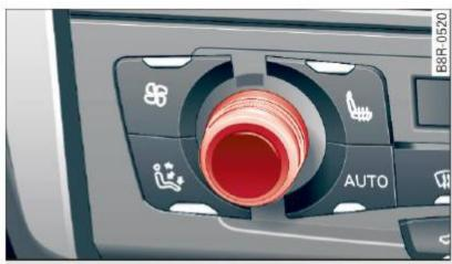
Fig. 100 Temperature setting regulator
