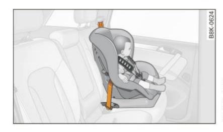
Fig. 190 Rear seat: smaller child in a properly installed forwardfacing convertible child safety seat
