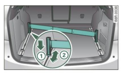
Fig. 91 Luggage compartment: Telescoping tracks
