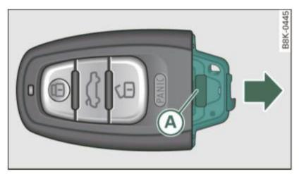
Fig. 32 Remote master key: Removing the battery holder
