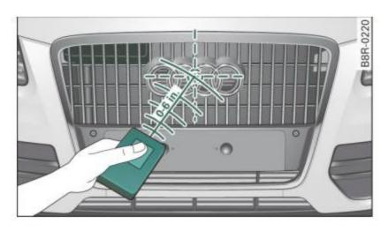
Fig. 164 Radiator grille: location of transmitter unit
