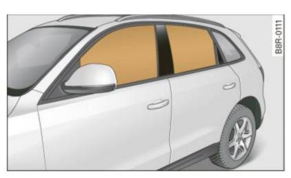
Fig. 188 Illustration of principle: Inflated side curtain airbags on the left side
