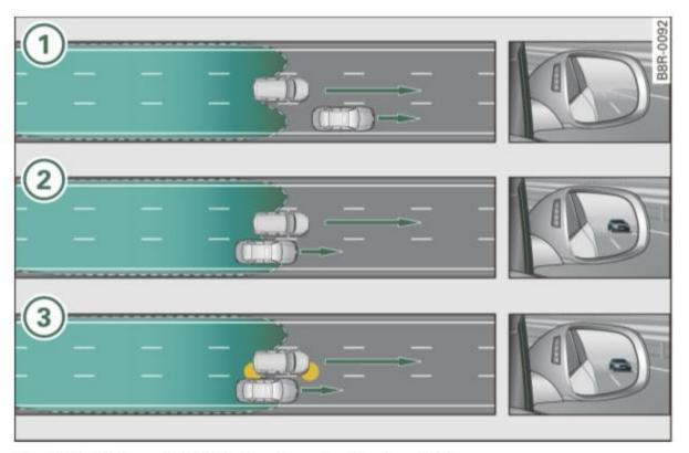
Fig. 137 Side assist: Vehicles dropping back quickly
