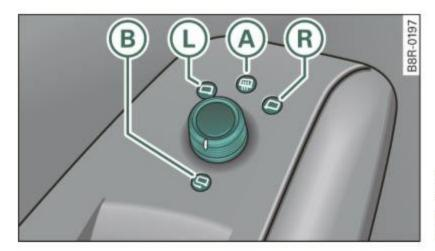
Fig. 71 Forward section of driver's armrest: power mirror controls
