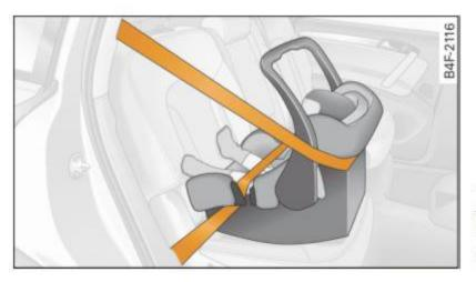
Fig. 189 Rearwardfacing infant seat, properly installed on the rear seat
