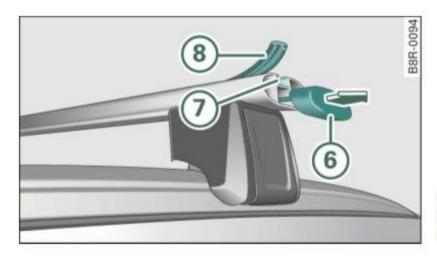
Fig. 98 Roof railing: installing cover profile into the roof rack
