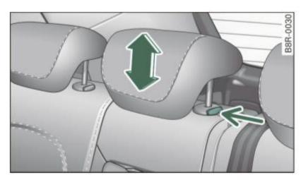
Fig. 80 Rear seats: Head restraint
