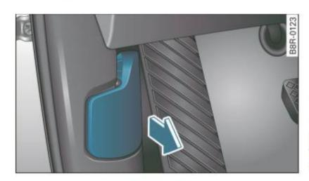
Fig. 209 Driver's side footwell: engine hood release lever
