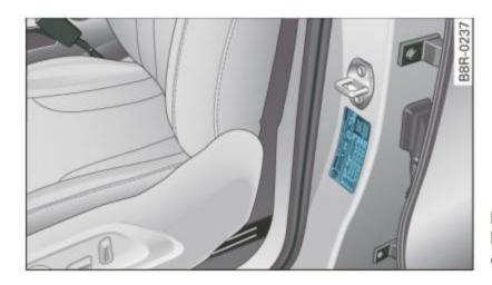
Fig. 218 Tire pressure label: located on driver's side B-pillar
