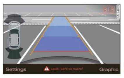
Fig. 159 MMI display: aligning the vehicle
