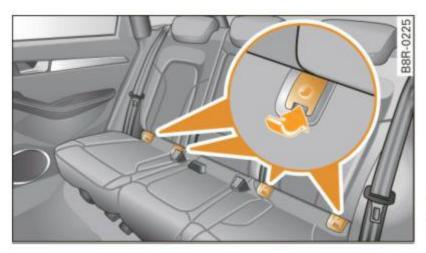
Fig. 194 Lower anchorages, covers marked
