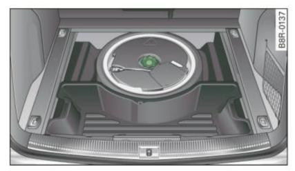
Fig. 226 Inflatable spare tire with compressor
