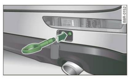
Fig. 244 Rear bumper: Screwing in towing loop
