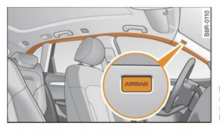
Fig. 187 Side curtain system, driver's side: side curtain airbag location
