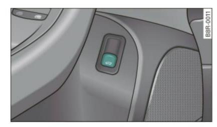
Fig. 43 Driver's door: remote rear lid release
