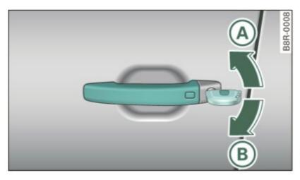
Fig. 40 Key turns for opening and closing
