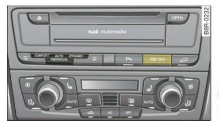
Fig. 202 Version B: at the top of the center console, ESP OFF button
