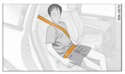
Fig. 192 Child taller than 4 ft. 9 in. properly restrained on the rear seat
