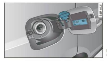
Fig. 207 Fuel filler flap with attached fuel cap
