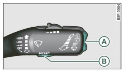
Fig. 19 Windshield wiper lever: controls for the trip computer
