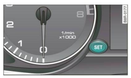
Fig. 3 SET button in the instrument cluster
