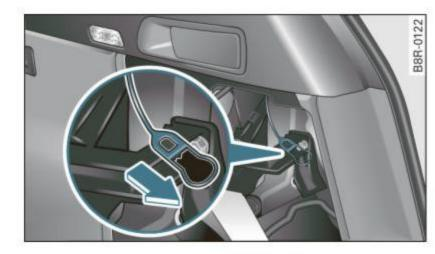
Fig. 208 Luggage compartment: Emergency opening of fuel filler flap
