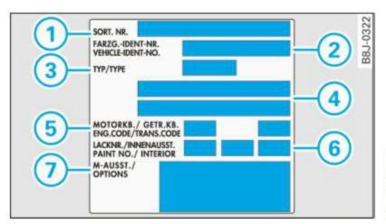
Fig. 249 The vehicle identification label – inside the luggage compartment
