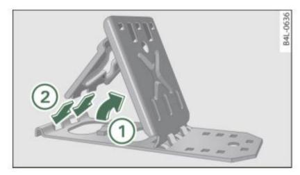
Fig. 224 Opening folding chocks
