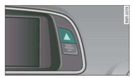
Fig. 59 Emergency flasher switch
