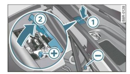
Fig. 216 Engine compartment: Connectors for charger and jumper cables
