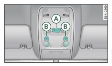
Fig. 61 Headliner: Front interior/reading lights
