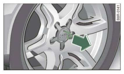
Fig. 228 Changing a wheel: Removing the wheel cover
