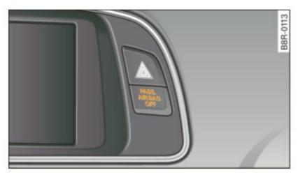
Fig. 184 Section from the instrument panel: PASSENGER AIR BAG OFF light
