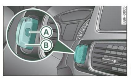
Fig. 34 Ignition switch with ignition key
