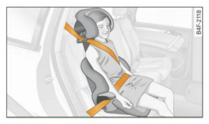
Fig. 191 Rear seat: child properly restrained in a booster seat
