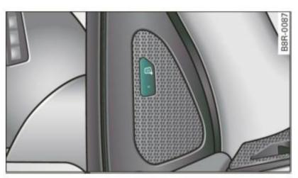
Fig. 132 Driver's door: Side assist button
