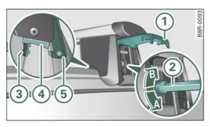
Fig. 97 Roof railing: installing a roof rack
