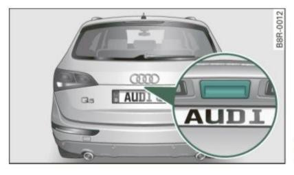
Fig. 44 Position of handle in the rear lid
