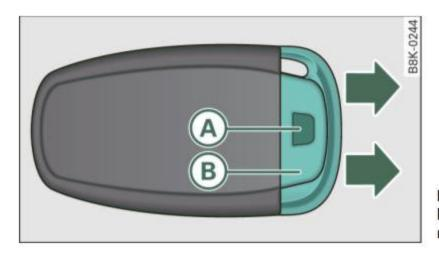
Fig. 33 Remote master key: Removing the mechanical key
