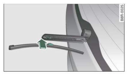
Fig. 69 Rear wiper: Removing the wiper blade
