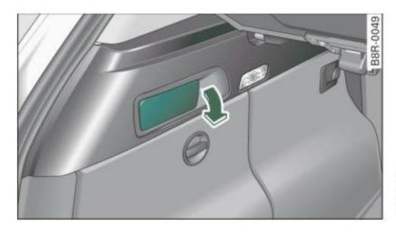
Fig. 84 Luggage compartment: release lever
