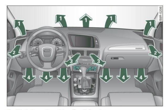
Fig. 121 Instrument panel: Location of air vents
