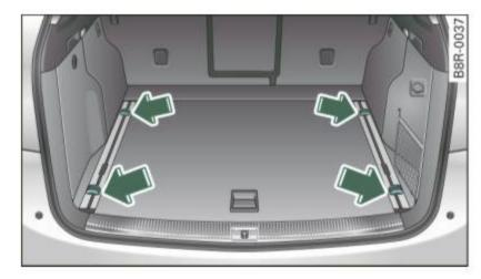
Fig. 87 Overview of the fastening eyelets in the luggage compartment
