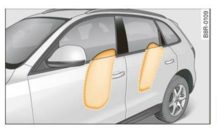
Fig. 186 Inflated side airbags on left side of vehicle
