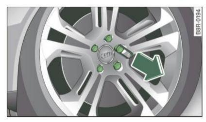
Fig. 229 Changing a wheel: removing the wheel bolt caps
