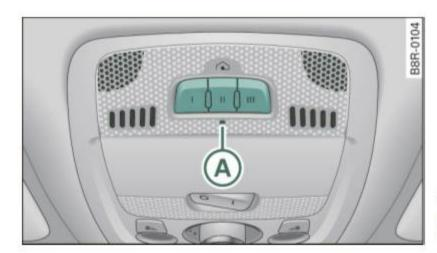
Fig. 165 Overhead console: HomeLink® keypad
