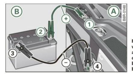
Fig. 240 Jump starting with the battery of another vehicle: (A) discharged vehicle battery, (B) booster battery
