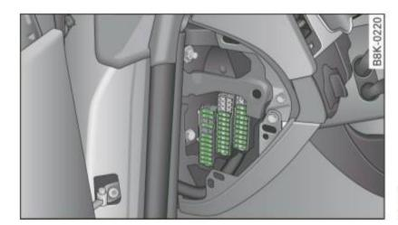
Fig. 236 Fuse panel layout
