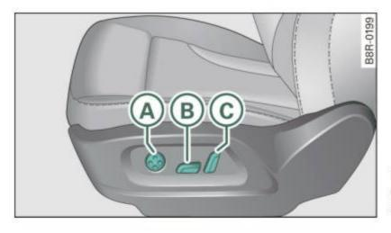
Fig. 74 Front seat: Controls for seat adjustment
