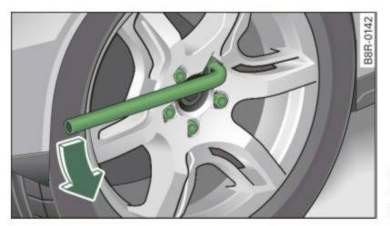
Fig. 230 Changing a wheel: loosening the wheel bolts
