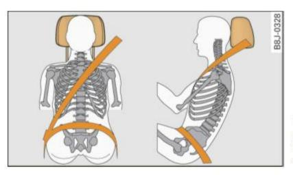
Fig. 177 Head restraint and safety belt position as seen from the side
