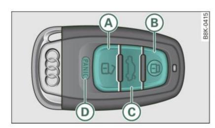
Fig. 38 Remote control: function buttons
