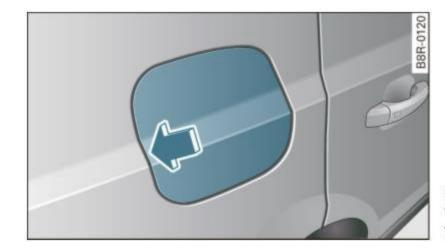
Fig. 206 Right rear vehicle side: Opening the fuel filler flap
