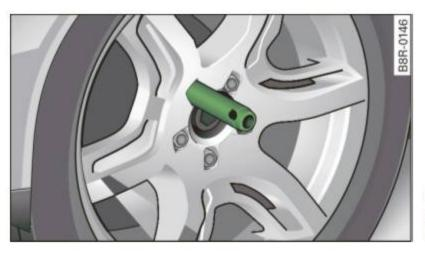
Fig. 234 Changing a wheel: alignment pin inside the top hole
