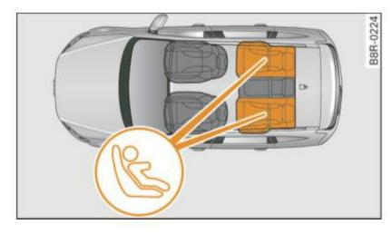
Fig. 193 Schematic overview: LATCH anchorage point locations
