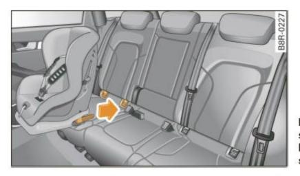
Fig. 196 LATCH-type seat with both latch bars extended (rigid system)
