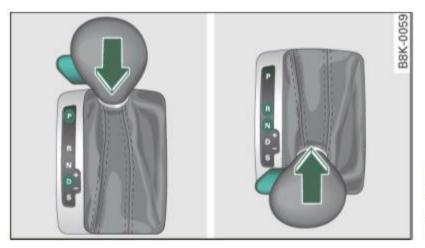
Fig. 146 Shift gate: selector lever lock positions and interlock button highlighted
