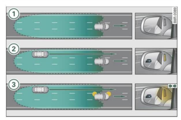
Fig. 134 Side assist: Fast approaching vehicles
