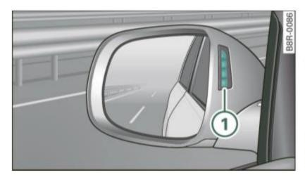
Fig. 131 Signal light on the outside mirror driver's side
