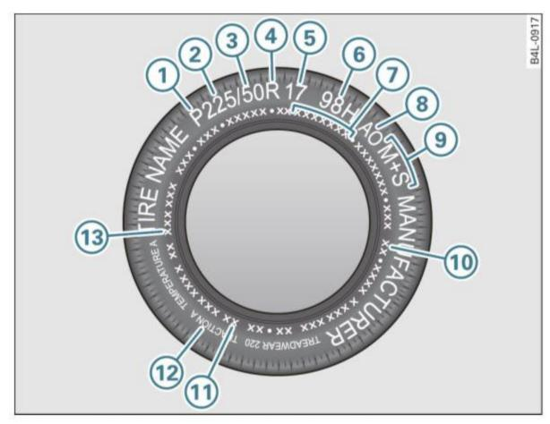
Fig. 222 Tire specification codes on the sidewall of a tire
