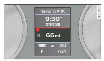
Fig. 16 Trip computer display: Fuel range
