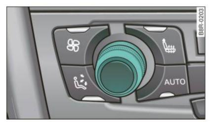
Fig. 115 Temperature setting regulator
