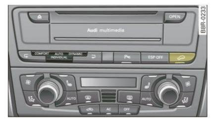
Fig. 203 Top of the center console: hill descent assist button
