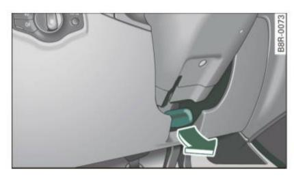
Fig. 124 Lever under the steering column
