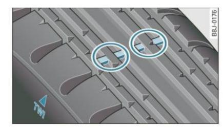
Fig. 220 Tire tread: tread wear indicators (TWI)
