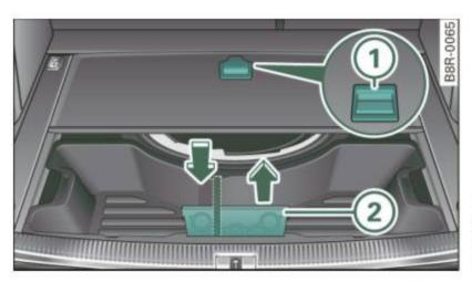
Fig. 90 Luggage compartment: cargo floor folded together with protective tray
