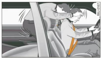
Fig. 174 A rear passenger not wearing a safety belt will fly forward and strike the driver
