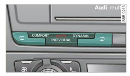
Fig. 142 Center console: Control for Audi drive select
