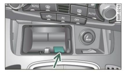
Fig. 151 Emergency release for selector lever
