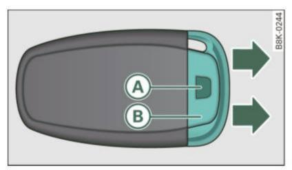
Fig. 31 Remote master key: Removing the mechanical key
