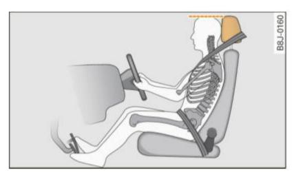
Fig. 167 Correct head restraint position for driver
