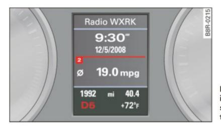
Fig. 145 Display in the instrument cluster: selector lever in position D
