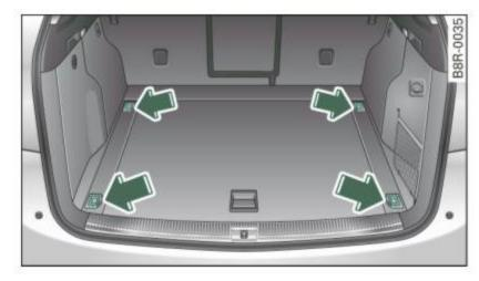
Fig. 85 Location of the tie-down rings in the luggage compartment
