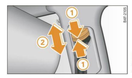
Fig. 180 Safety belt height adjustment for the front seats - looparound fittings
