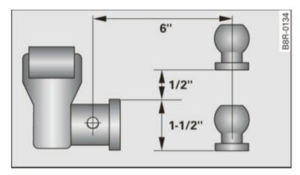
Fig. 205 Permitted ball position of the trailer hitch
