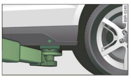
Fig. 247 Rear lifting point
