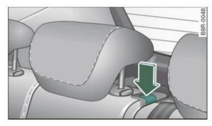
Fig. 83 Release button for the center backrest
