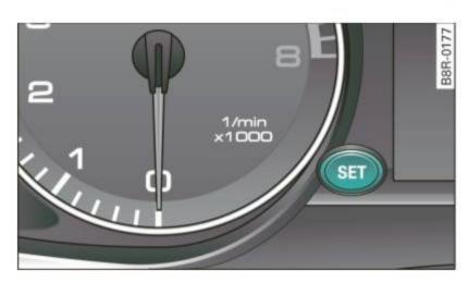
Fig. 21 SET button in the instrument cluster
