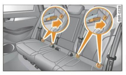
Fig. 197 Installation of child safety seat with rigid latches on bars
