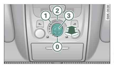
Fig. 51 Section from headliner: Knob for Panoramic sliding sunroof
