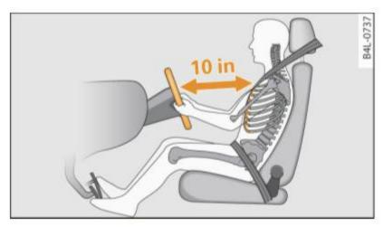
Fig. 166 The correct distance between driver and steering wheel
