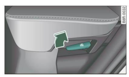
Fig. 82 Release lever for the outer backrest
