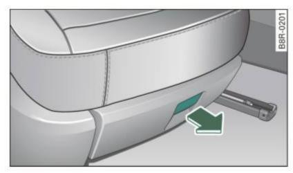
Fig. 111 Front side of passenger seat: storage compartment
