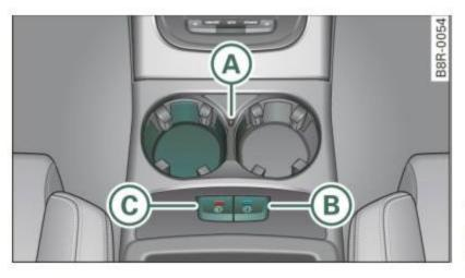
Fig. 101 Center console: climatized cupholder
