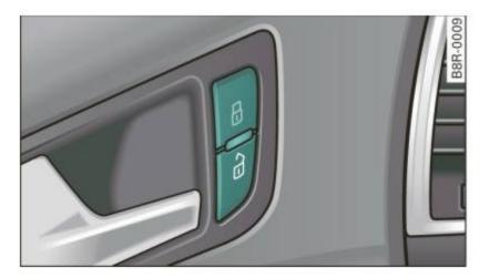
Fig. 41 Driver's door: power locking switch
