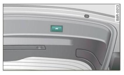
Fig. 46 Locking switch in the rear lid
