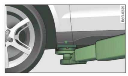
Fig. 246 Front lifting point
