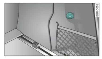
Fig. 106 Section of the trim panel of the luggage compartment: 12-volt socket
