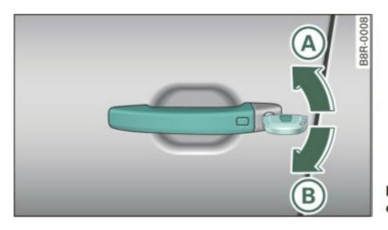
Fig. 50 Key turns for opening and closing
