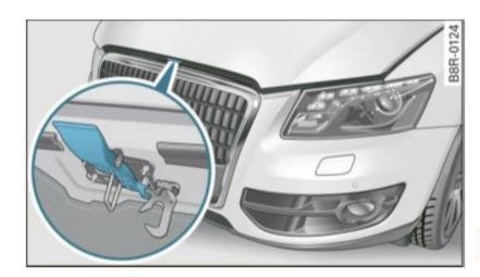
Fig. 210 Release lever under the engine hood
