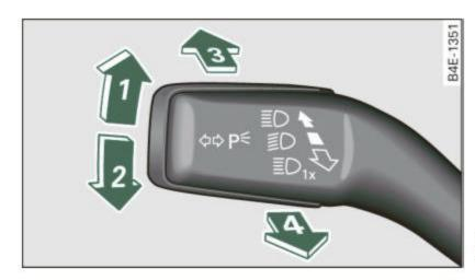
Fig. 60 Turn signal and high beam lever
