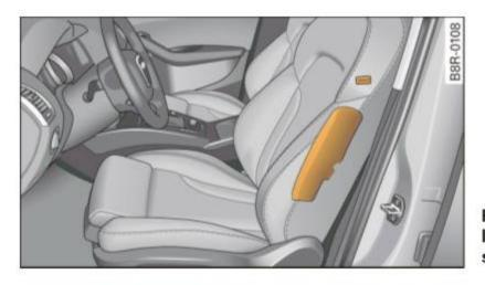
Fig. 185 Side airbag location in the driver's seat
