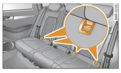
Fig. 195 Rear seats: lower anchorage bracket locations
