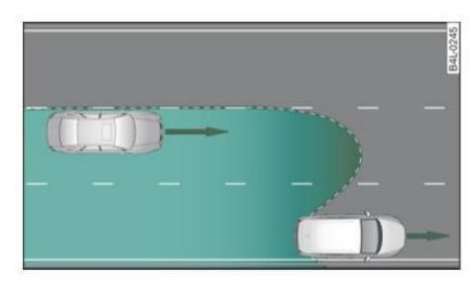
Fig. 139 Lanes of a normal width are in detection area
