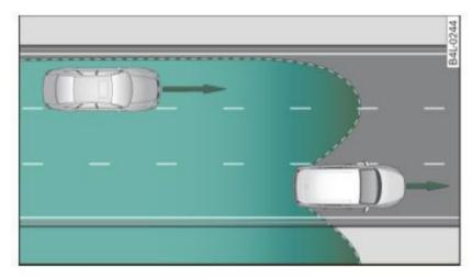
Fig. 140 Narrow lanes: Side assist may detect vehicles two lanes away
