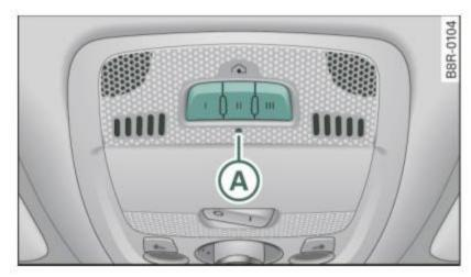
Fig. 163 Overhead console: HomeLink® keypad
