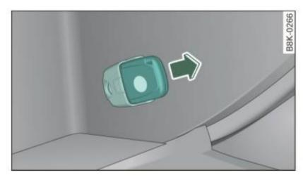
Fig. 35 Glove compartment: Adapter for emergency key
