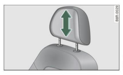
Fig. 79 Front seat: Adjusting the head restraint
