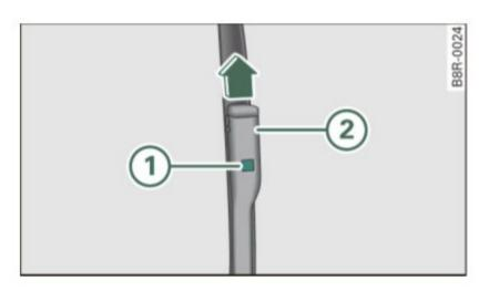
Fig. 68 Removing the wiper blade
