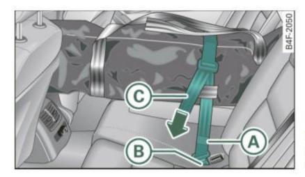
Fig. 95 Securing the ski sack at the center rear seat belt buckle
