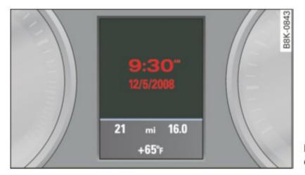
Fig. 4 Instrument cluster: time and date
