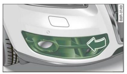
Fig. 241 Front bumper: removing the cover cap
