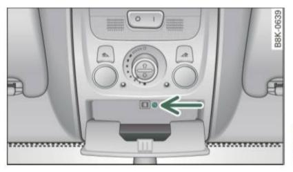
Fig. 52 Section from headliner: Unscrewing the lighting unit
