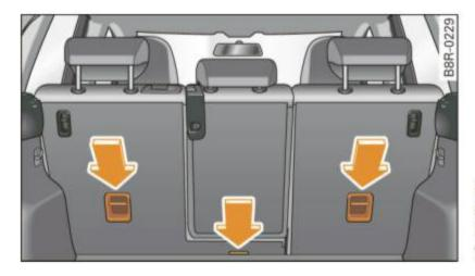
Fig. 198 Tether anchors: attachment hook locations behind the rear seatbacks
