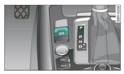
Fig. 127 Center console: Parking brake
