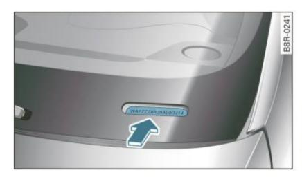
Fig. 248 Vehicle Identification Number (VIN) plate: location on driver's side dash panel
