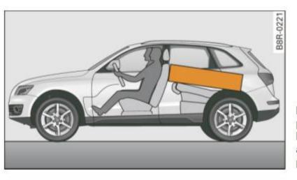
Fig. 169 Safe load positioning: place heavy objects as low and as far forward as possible.
