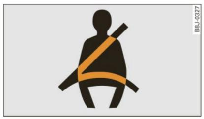
Fig. 170 Safety belt warning light in the instrument cluster enlarged
