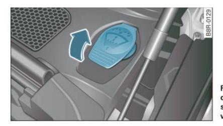
Fig. 217 Engine compartment: Windshield and headlight\* washer fluid container >
