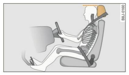
Fig. 168 Correctly adjusted head restraint viewed from the side
