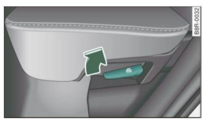
Fig. 77 Adjusting seat back angle
