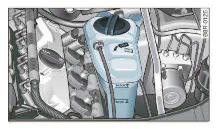
Fig. 214 Engine compartment: Coolant expansion tank
