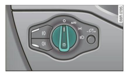
Fig. 54 Instrument panel: light switch
