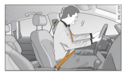
Fig. 175 Driver is correctly restrained in a sudden braking maneuver
