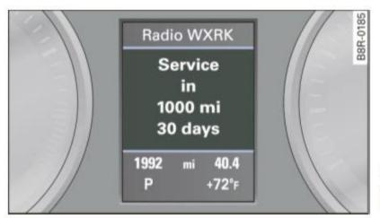
Fig. 14 Instrument cluster: Service interval display
