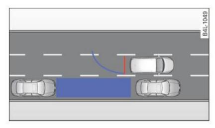
Fig. 153 Parking mode 2: parallel parking
