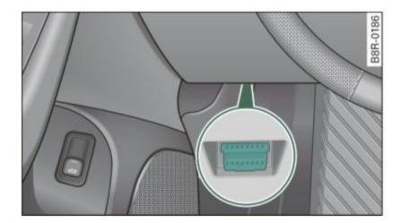
Fig. 15 Location of Data Link Connector (DLC)
