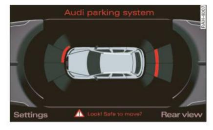
Fig. 157 MMI display: visual distance display
