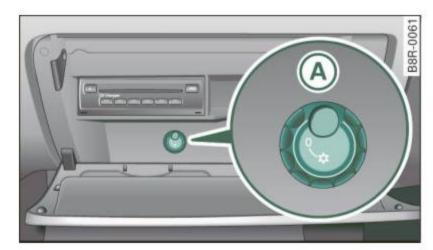
Fig. 109 Glove box with cooling box open and switched on
