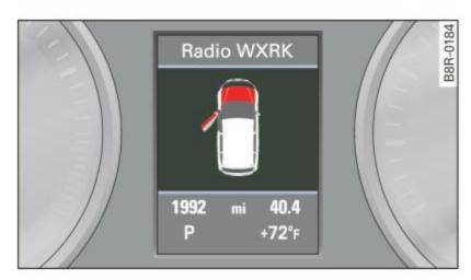
Fig. 12 Display: Open door- and trunk lid warning
