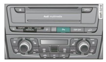
Fig. 156 Center console: Parking system switch
