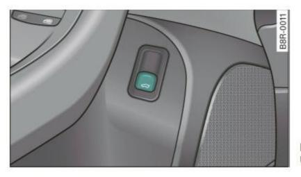
Fig. 45 Driver's door: Unlocking the rear lid
