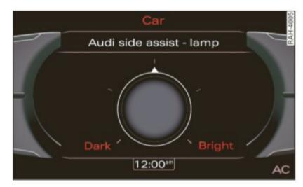
Fig. 138 Display: Adjusting signal brightness
