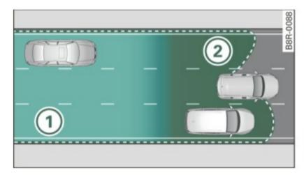
Fig. 133 Schematic illustration: Sensor detection area
