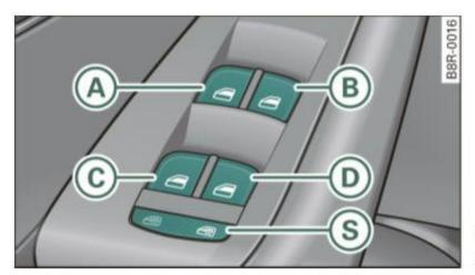
Fig. 49 Section of the driver's door: Controls
