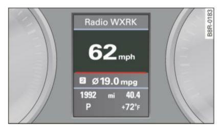
Fig. 11 Display: Digital speedometer
