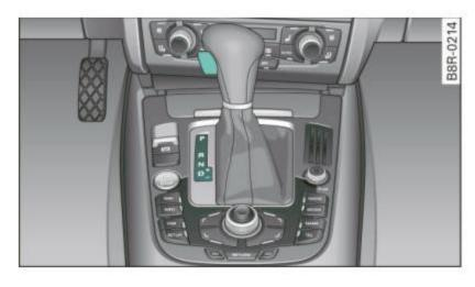
Fig. 144 Shift gate on the center console: selector lever with release button
