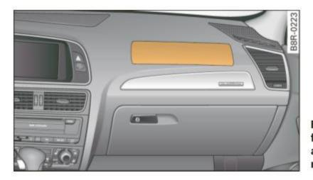
Fig. 182 Location of front passenger's airbag: in the instrument panel
