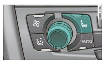
Fig. 123 Seat heating button and regulator
