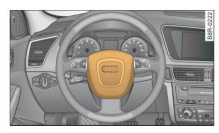
Fig. 181 Location of driver airbag: in steering wheel
