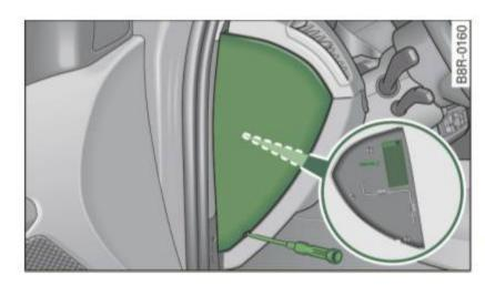
Fig. 235 Instrument panel left: Face cover
