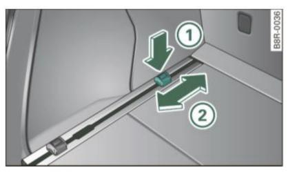
Fig. 86 Adjusting, removing the fastening eyelets in the luggage compartment
