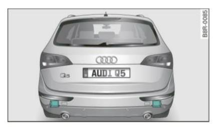
Fig. 130 Rear bumper: Position of radar sensors (not visible on outside)
