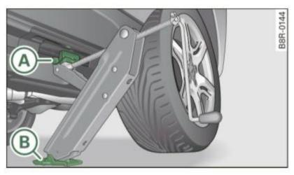
Fig. 232 Close-up: proper positioning of iack
