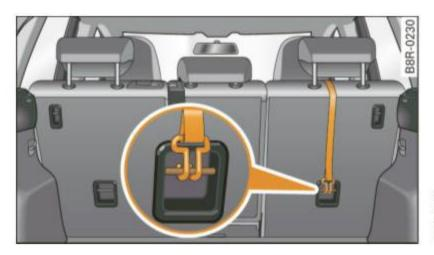
Fig. 200 Tether strap: proper routing and mounting
