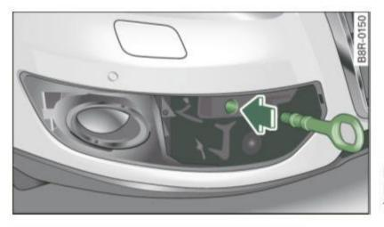
Fig. 242 Front bumper: screwing in the towing loop
