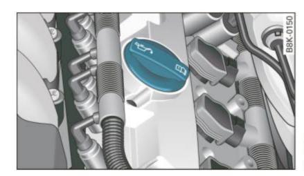
Fig. 213 Engine compartment: Oil filler cap location
