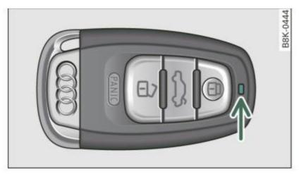
Fig. 30 Check light in the master key
