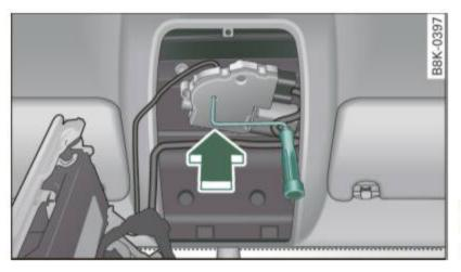
Fig. 53 Section from headliner: Crank for emergency operation
