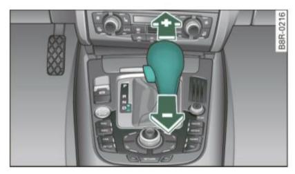
Fig. 147 Center console: shifting the tiptronic® manually
