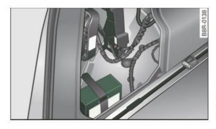
Fig. 227 Luggage compartment left side: compressor
