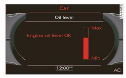
Fig. 212 Display: Oil level indicator
