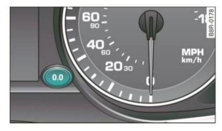
Fig. 6 Instrument cluster: reset button
