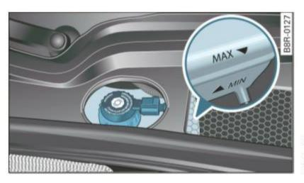
Fig. 215 Engine compartment: Brake fluid reservoir
