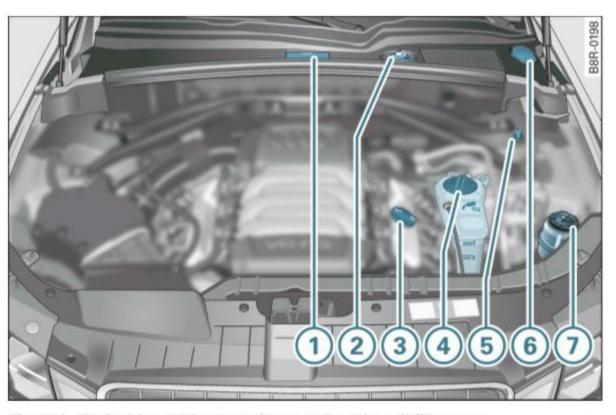
Fig. 211 Typical layout for containers and engine oil filler cap
