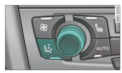
Fig. 119 Air distribution button and regulator
