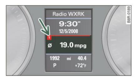
Fig. 18 Trip computer display: memory level 1
