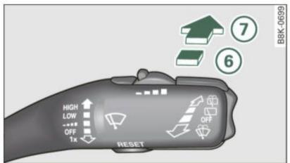
Fig. 66 Rear wiper actuation
