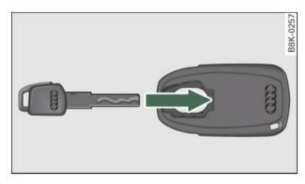
Fig. 36 Insert emergency key into the adapter
