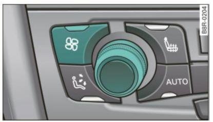
Fig. 117 Fan button and regulator
