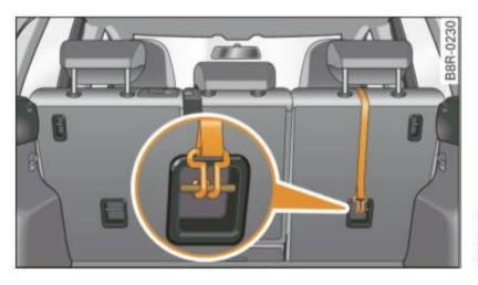
Fig. 199 Tether strap: proper routing and mounting
