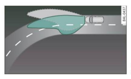
Fig. 58 Adaptive light when driving
