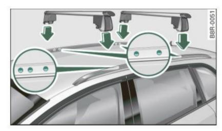
Fig. 96 Roof rack attachment points
