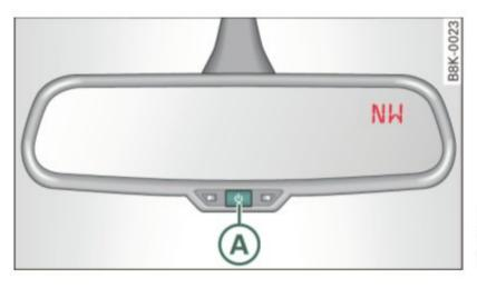
Fig. 72 Inside rear view mirror: digital compass activated
