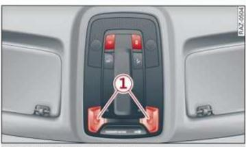
Fig. 41 Headliner: interior lighting
