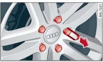
Fig. 161 Wheel: wheel bolts with caps
