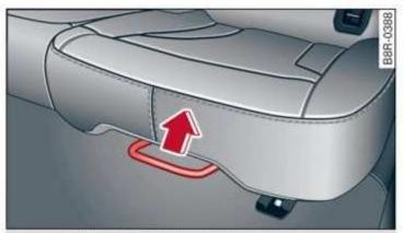
Fig. 53 Adjusting the seat position
