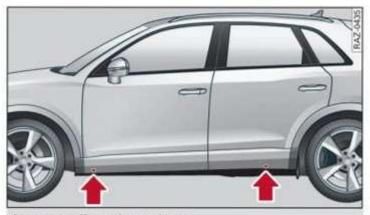
Fig. 164 Sill panels: markings
