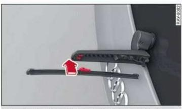
Fig. 48 Rear window wiper: installing the wiper blade
