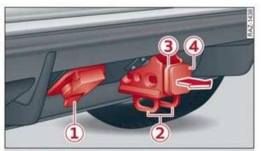
Fig. 88 Rear bumper: trailer hitch
