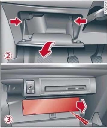
Fig. 174 Left side of the cockpit: storage compartment (left-hand drive) ② or storage compartment (right-hand drive) ③
