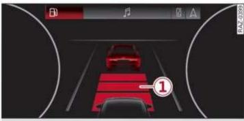
Fig. 104 Instrument cluster: brake intervention request
