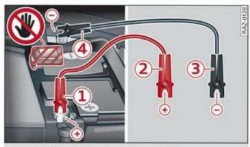
Fig. 170 Connecting the jump start cables
