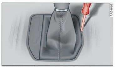
Fig. 85 Selector lever: removing the shifter boot
