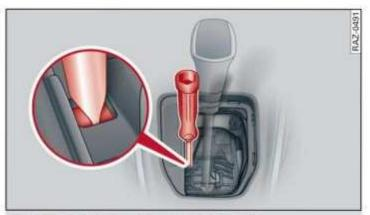
Fig. 86 Emergency release at the lower left
