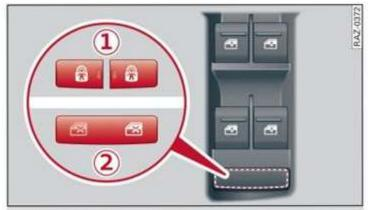
Fig. 34 Driver's door: controls
