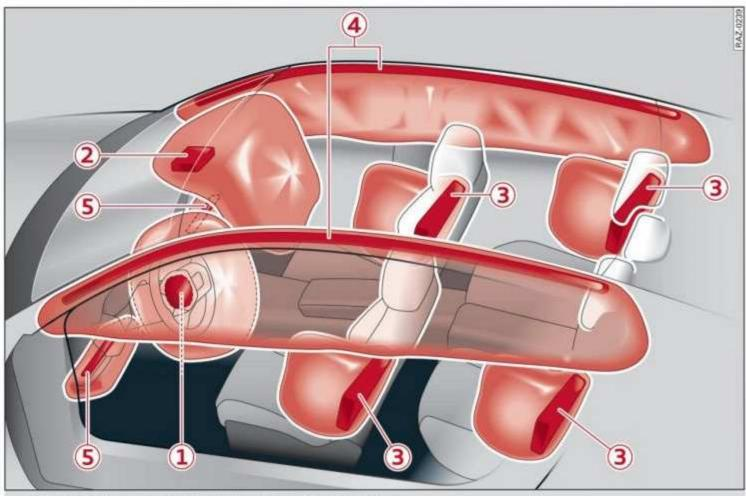
Fig. 64 Airbag overview image (enlarged section: deployed airbags)
