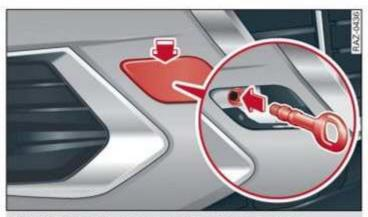
Fig. 171 Front bumper: installing the towing loop
