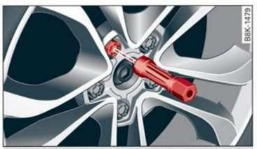
Fig. 166 Wheel: internal hex socket to turn the wheel holts
