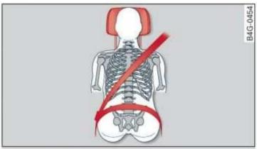
Fig. 56 Correctly-adjusted head restraint
