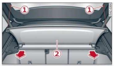
Fig. 72 Luggage compartment: cover when the luggage compartment lid is open
