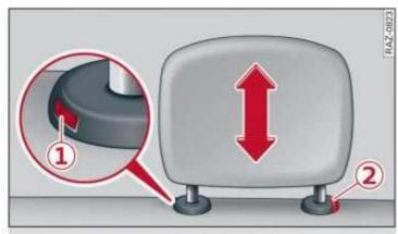
Fig. 58 Rear seat: operating the head restraints
