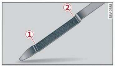
Fig. 150 Oil dipstick (example): checking the engine oil lev-
