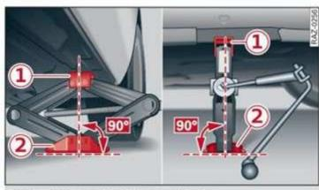
Fig. 165 Sill: positioning the vehicle jack
