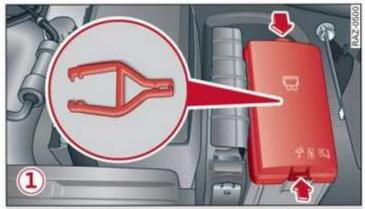
Fig. 173 Left side of the engine compartment: fuse cover
