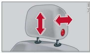
Fig. 57 Front seat: adjusting the head restraint
