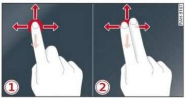
Fig. 13 Touch display: 1 dragging with one finger, 2 dragging with two fingers
