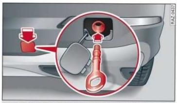
Fig. 172 Rear bumper: installing the towing loop
