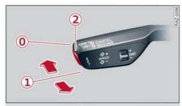
Fig. 106 Lever: using adaptive cruise assist
