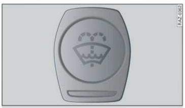
Fig. 155 Engine compartment: washer fluid reservoir cap
