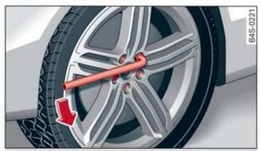
Fig. 163 Wheel: loosening the wheel bolts
