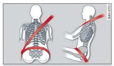
Fig. 59 Lap/shoulder belt positioning
