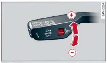
Fig. 105 Operating lever: setting the distance
