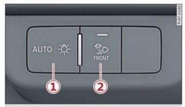
Fig. 38 Instrument panel: light button module
