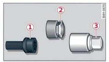
Fig. 162 Anti-theft wheel bolt with cap and adapter
