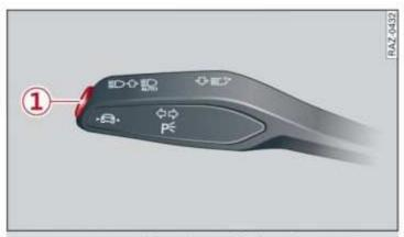
Fig. 110 Turn signal lever: button for lane departure warning and lane guidance for adaptive cruise assist\*
