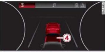
Applies to: vehicles with adaptive cruise assist: Fig. 109 Instrument cluster: distance warning
