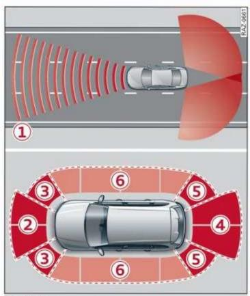
Fig. 89 Sensor coverage area
