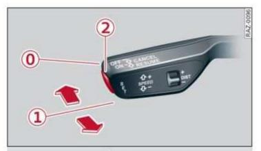
Fig. 101 Lever: using adaptive cruise assist
