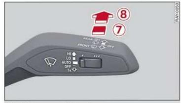
Fig. 46 Lever: rear window wiper
