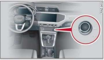
Fig. 21 Volume knob with joystick function
