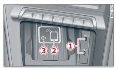
Fig. 125 Front center console: Audi phone box with connections
