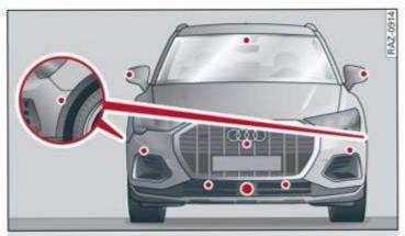
Fig. 91 Front area: sensors and cameras
