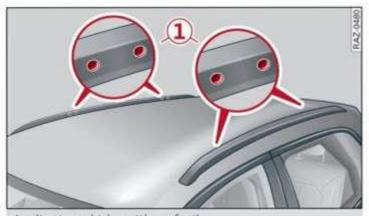
Applies to: vehicles with roof rail Fig. 78 Roof rail: mounting points
