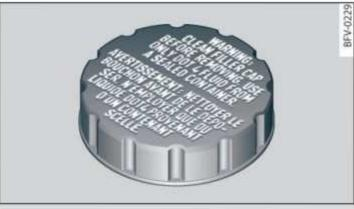
Fig. 153 Engine compartment: cap on brake fluid reservoir
