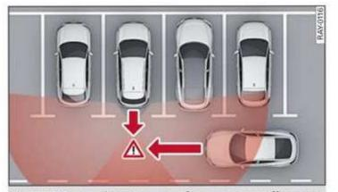
Fig. 120 Sensor detection range for rear cross-traffic assist
