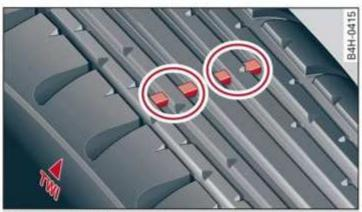
Fig. 157 Tire profile: treadwear indicator
