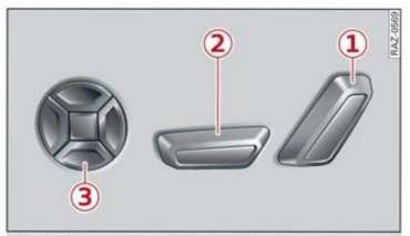
Fig. 52 Front seat: seat adjustment buttons
