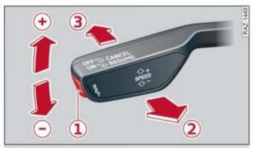
Fig. 96 Operating lever: switching the system on
