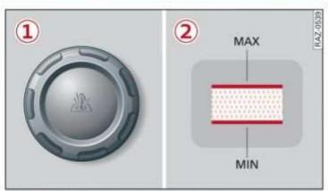
Fig. 152 Engine compartment - coolant expansion tank (diagram): 1 cover; 2 markings
