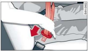
Fig. 61 Belt buckle and belt latch
