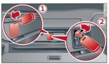
Fig. 33 Rear lid opening: access to the emergency release
