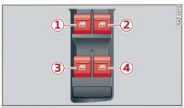
Fig. 36 Driver's door: power window switch
