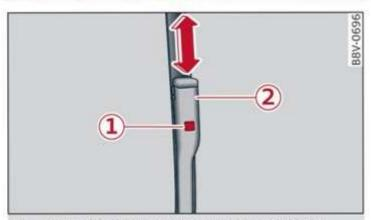
Fig. 47 Windshield wipers: changing the wiper blades
