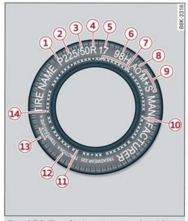
Fig. 156 Tire designations on the sidewall
