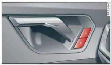
Fig. 22 Driver's door: central locking switch
