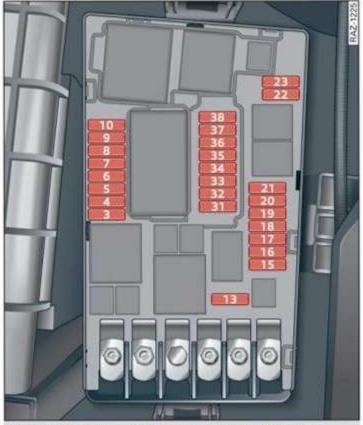
Fig. 175 Left side of engine compartment: fuse assignment
