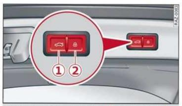
Fig. 31 Luggage compartment lid: 10 closing button\*, 20 lock button\* (vehicles with convenience key\*)
