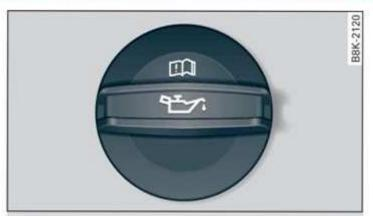
Fig. 151 Engine compartment: engine oil filling opening cover (example)
