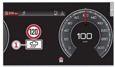
Fig. 94 Instrument cluster: traffic sign recognition
