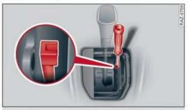
Fig. 87 Emergency release at the upper right
