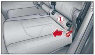
Fig. 54 Adjusting the backrests
