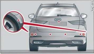
Fig. 92 Rear area: sensors and cameras
