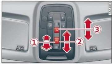
Fig. 37 Headliner: panoramic glass roof and sunshade\* buttons
