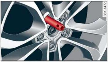
Fig. 167 Wheel: alignment pin in the top hole
