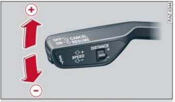
Fig. 102 Operating lever: changing the speed
