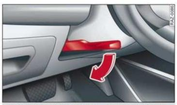
Fig. 55 Steering column: lever for adjusting the steering wheel position
