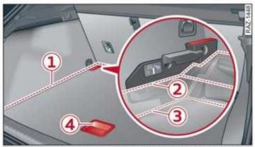
Fig. 77 Luggage compartment: lowering the cargo floor\*
