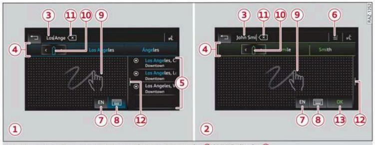
Fig. 17 Center display: text input diagram with MMI Navigation plus ① / MMI Radio plus ②
