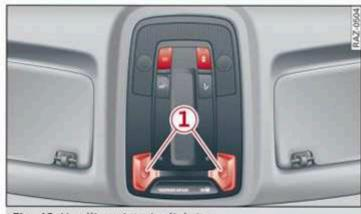
Fig. 40 Headliner: interior lighting
