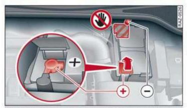
Fig. 152 Engine compartment with battery: connections for charger and jump start cable
