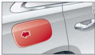
Fig. 142 Right rear side of the vehicle: opening the fuel filler door
