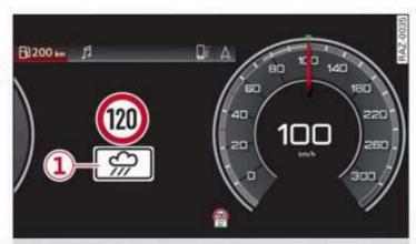
Fig. 92 Instrument cluster: traffic sign recognition
