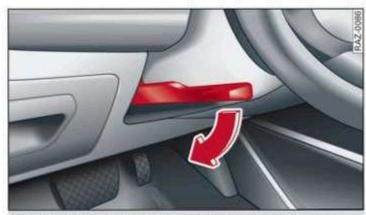
Fig. 54 Steering column: lever for adjusting the steering wheel position
