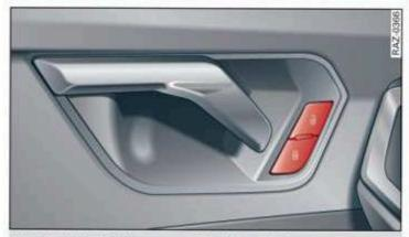
Fig. 21 Driver's door: central locking switch
