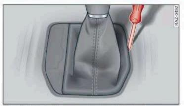
Fig. 84 Selector lever: removing the shifter boot
