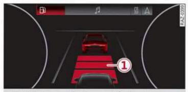
Fig. 105 Instrument cluster: request for driver intervention
