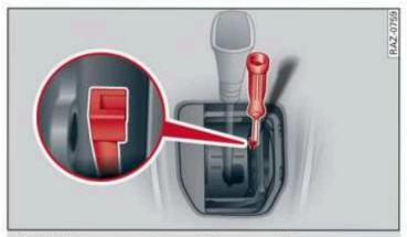
Fig. 86 Emergency release at the upper right
