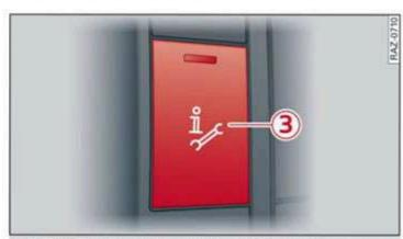
Fig. 127 Front headliner: online roadside assistance button
