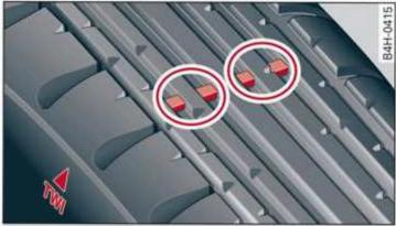
Fig. 155 Tire profile: treadwear indicator
