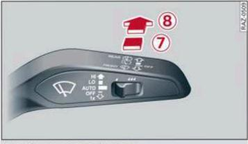
Fig. 45 Lever: rear window wiper
