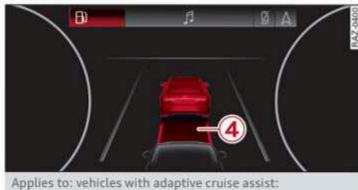
Applies to: vehicles with adaptive cruise assist: Fig. 107 Instrument cluster: distance warning
