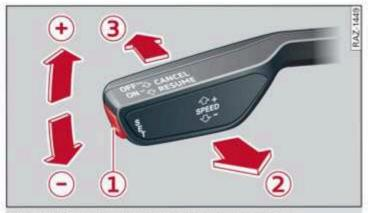
Fig. 94 Operating lever: switching the system on
