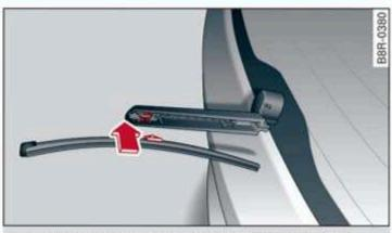
Fig. 47 Rear window wiper: installing the wiper blade
