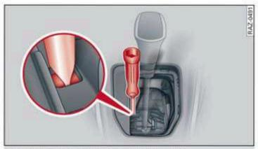
Fig. 85 Emergency release at the lower left
