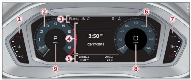
Fig. 3 Digital instrument cluster or Audi virtual cockpit overview
