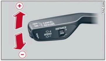
Fig. 100 Operating lever: changing the speed
