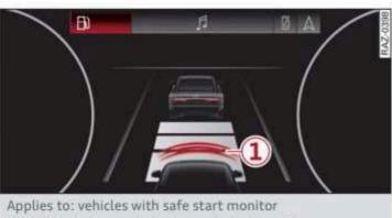
Fig. 104 Instrument cluster: safe start monitor
