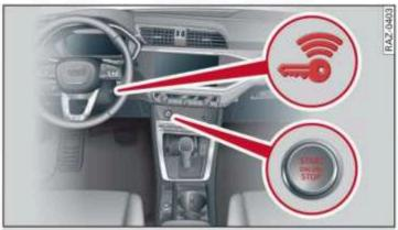
Fig. 79 Center console: starting the engine
