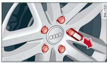
Fig. 159 Wheel: wheel bolts with caps
