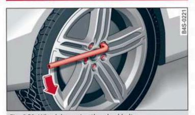
Fig. 161 Wheel: loosening the wheel bolts
