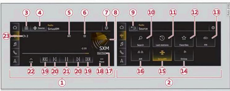
Fig. 138 Center display: left side: playback view of radio functions, right side: sources
