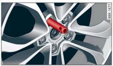
Fig. 165 Wheel: alignment pin in the top hole
