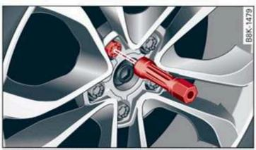
Fig. 164 Wheel: internal hex socket to turn the wheel holts
