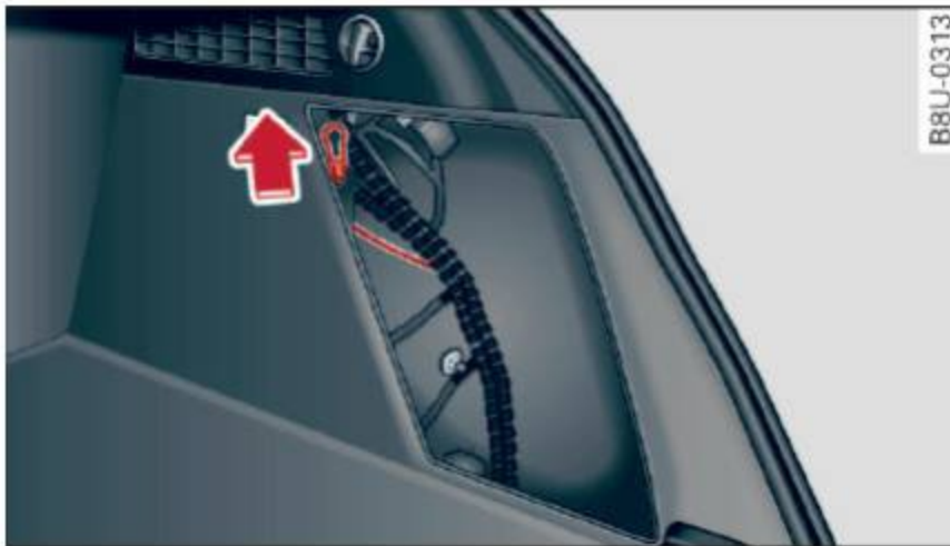
Fig. 134 Right side trim panel in the luggage compartment: emergency release mechanism
