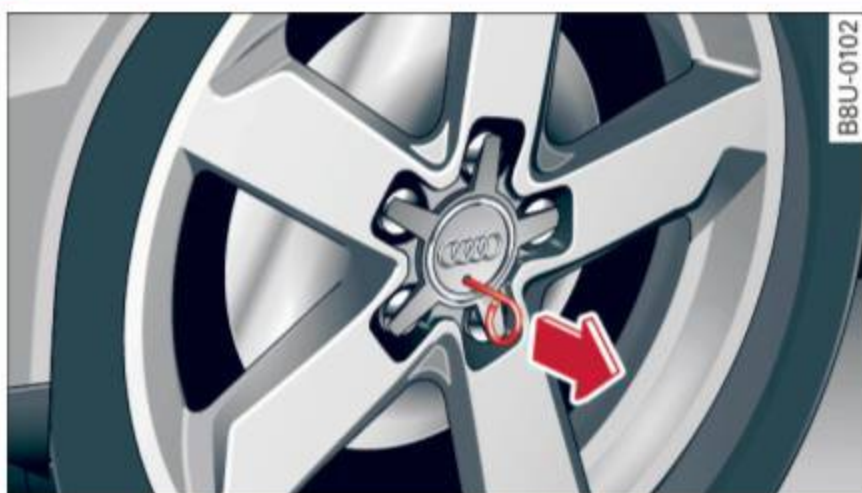
Fig. 149 Changing a wheel: removing the wheel cover
