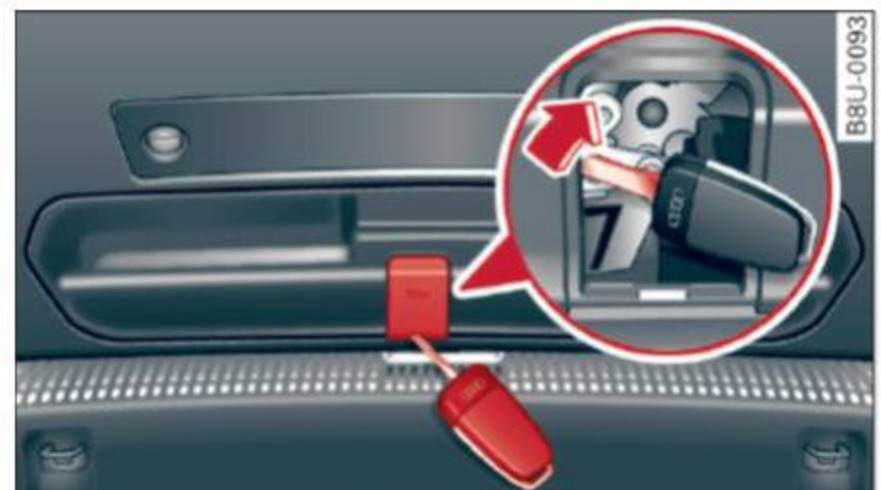
Fig. 25 Luggage compartment lid emergency release
