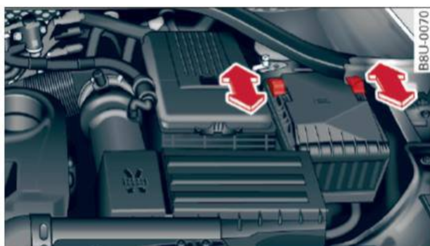
Fig. 159 Engine compartment: removing the fuse panel cover
