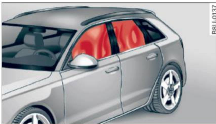
Fig. 119 Illustration of principle: Inflated side curtain airbags on the left side
