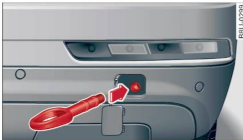
Fig. 165 Rear bumper: installing the towing loop
