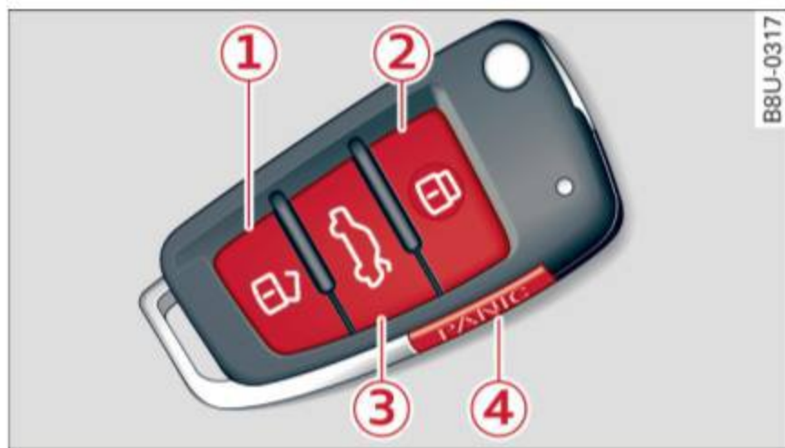
Fig. 15 Remote control key: button programming
