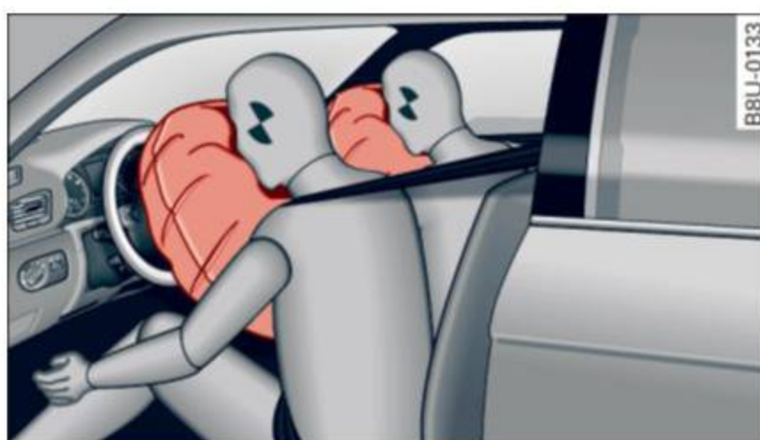
Fig. 114 Inflated front airbags
