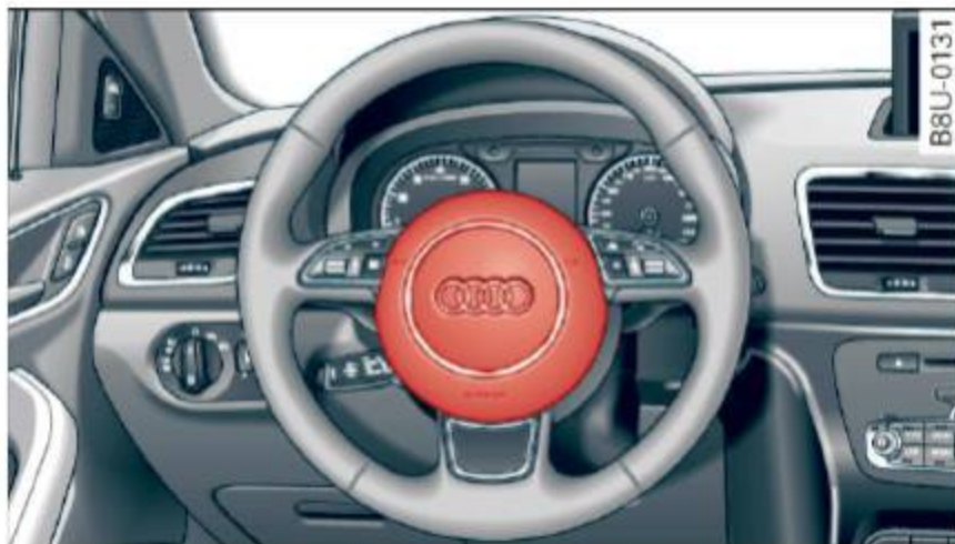
Fig. 112 Location of driver airbag: in steering wheel
