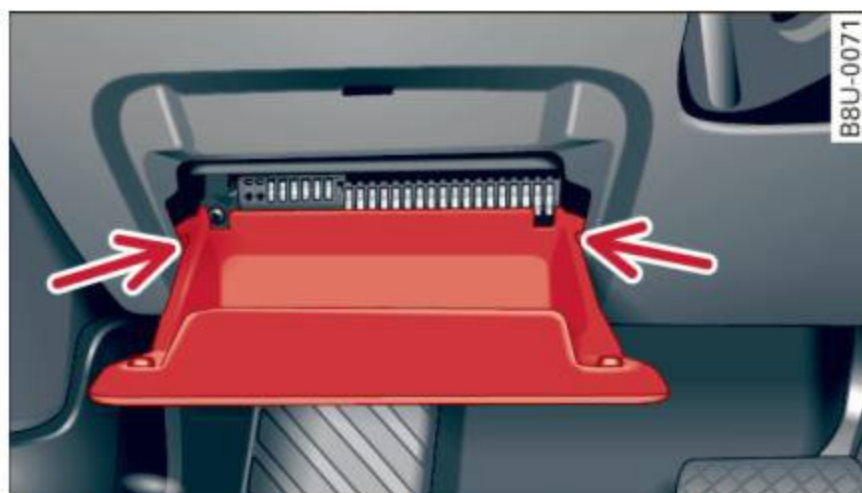
Fig. 158 Driver's side of the cockpit: folding the storage compartment down
