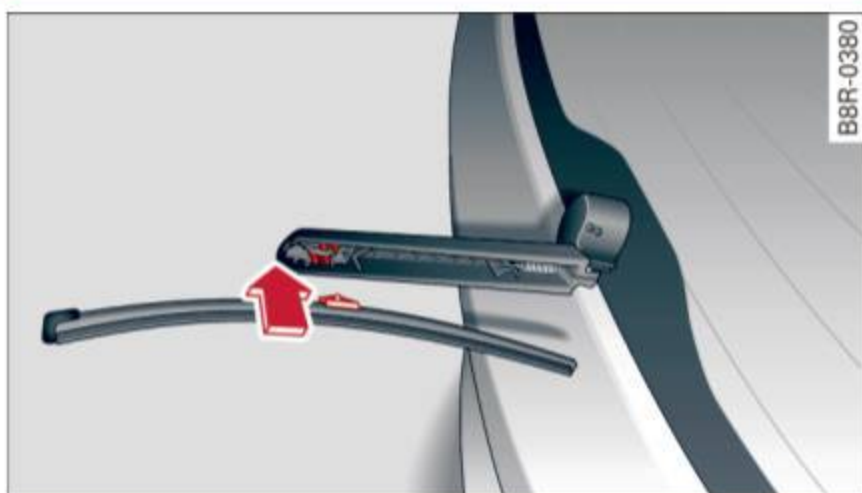
Fig. 42 Rear window wiper: removing the wiper blade
