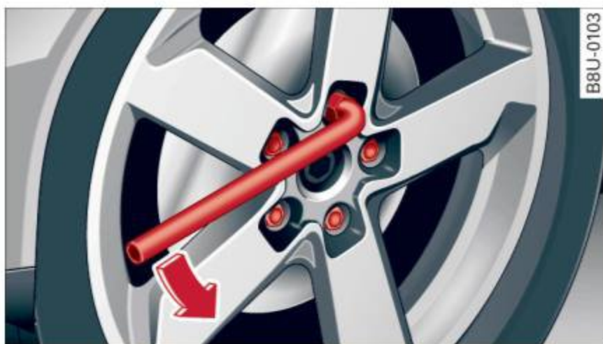
Fig. 151 Changing a wheel: loosening the wheel bolts
