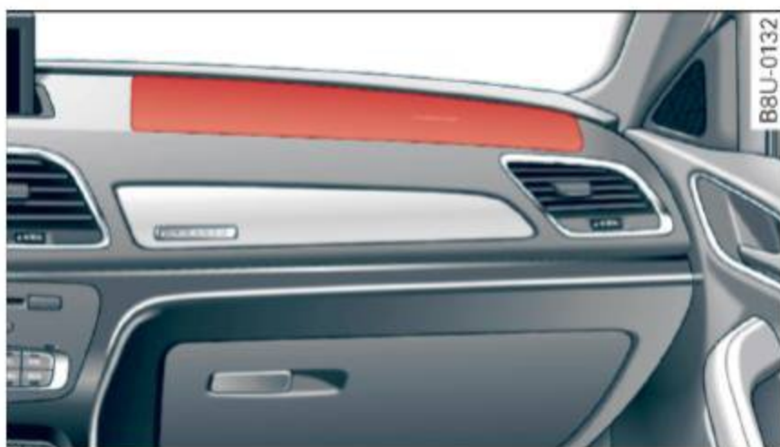
Fig. 113 Location of front passenger's airbag: in the instrument panel
