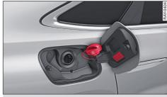
Fig. 121 Fuel tank flap with tank cap attached
