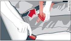
Fig. 42 The latch plate of the belt springs out of the buck-le
