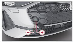
Fig. 8 Connecting a power source
