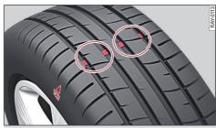
Fig. 136 Tyre tread: Tread wear indicators
