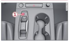
Fig. 82 Centre console: Button for driver assist systems
