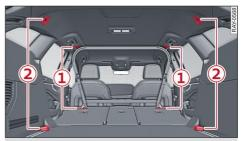
Fig. 59 Luggage compartment and folded-down backrest: Load guard
