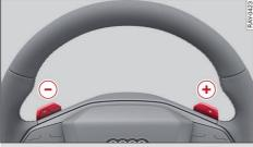
Fig. 72 Steering wheel: Paddle levers
