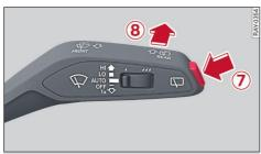
Fig. 28 Wiper lever: Rear window wiper
