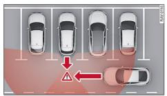
Fig. 112 Areas covered by sensors for rear cross-traffic assist
