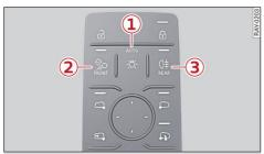
Fig. 18 Driver's door: Light switch module
