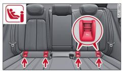
Fig. 50 Rear seat: Bottom ISOFIX anchorages
