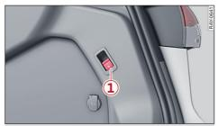
Fig. 73 Luggage compartment: Button for releasing towing bracket
