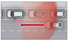
Fig. 87 Detected traffic approaching from behind
