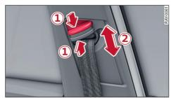
Fig. 43 Belt height adjustment for the front seats: guide fitting
