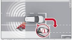
Fig. 102 Driving situation and warning signal on exterior mirror
