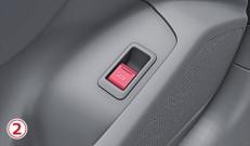
Fig. 14 Release catch in boot lid (1), button in driver's door (2)
