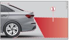
Fig. 79 Area covered by reversing camera
