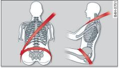
Fig. 39 Positioning seat belts over lap/shoulder
