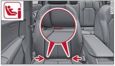
Fig. 51 Front passenger's seat: Bottom ISOFIX anchorages
