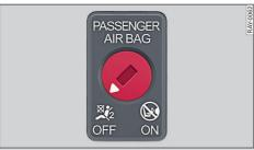
**Fig. 46** Glove box: Key-operated switch for deactivating front passenger's airbag
