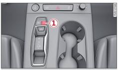
Fig. 107 Centre console: Button for park assist systems
