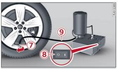
Fig. 141 Connecting the tyre repair kit
