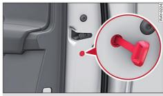
Fig. 10 Door: Locking the door manually
