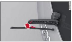
Fig. 30 Rear window wiper: Attaching the wiper blade
