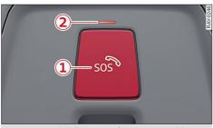
Fig. 118 Front headliner: Cover for emergency call button
