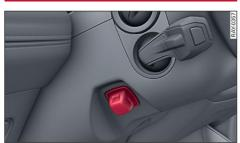
**Fig. 34** Steering column: Button for adjusting the steering wheel position
