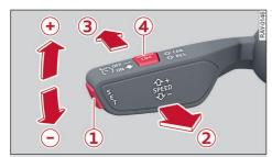
Fig. 93 Control lever: Switching the system on
