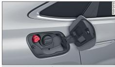
**Fig. 122** Vehicle as seen from the rear right: Unscrewing the AdBlue cap
