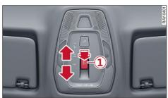
Fig. 24 Headliner: Switch for panoramic glass roof with switchable transparency
