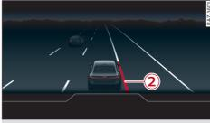
Fig. 90 Instrument cluster: Lane departure warning
