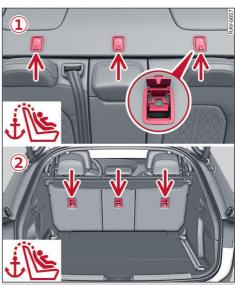
Fig. 52 ① Rear shelf / ② Rear backrest: Top tether anchorages for securing a child restraint system with a top tether strap
