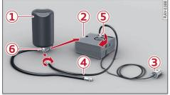
Fig. 140 Components of the tyre repair kit
