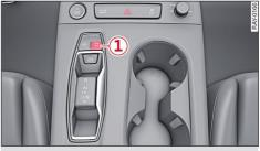
Fig. 83 Centre console: Button for park assist systems
