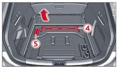
**Fig. 64** Luggage compartment: Load retention set under the floor
