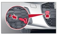
**Fig. 149** Front bumper: Fitting the towline anchorage (version 1)
