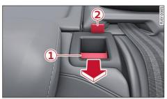
**Fig. 56** Outer backrest: Release lever and backrest lock indicator with red marking
