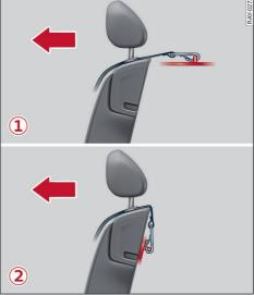
Fig. 53 ① Rear shelf / ② Rear backrest: Hooking strap into top tether anchorage
