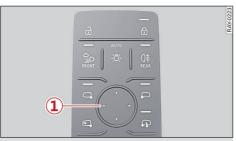
Fig. 23 Driver's door: Control panel for exterior mirrors
