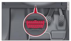
**Fig. 158** Driver footwell: connection socket for the onboard diagnostic system
