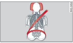
Fig. 35 Correctly adjusted head restraint
