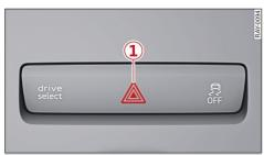
Fig. 20 Centre console: Hazard warning lights
