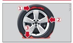
Fig. 139 Tyres: Irreparable tyre damage
