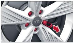
Fig. 142 Wheel: Wheel bolts with caps
