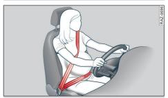
Fig. 40 Positioning seat belts during pregnancy
