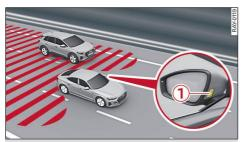
Fig. 85 Driving situation and warning signal on exterior mirror
