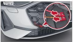
Fig. 7 Front bumper: Cap with 12-volt connections clipped
