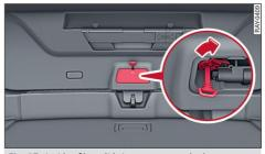
Fig. 17 Inside of boot lid: Access to manual release
