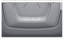
**Fig. 47** Headliner: Indicator lamp for status of front passenger's airbag
