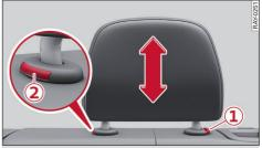
Fig. 38 Rear seat: Removing/installing head restraint
