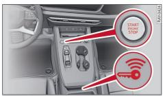
Fig. 70 Centre console: Switching on the drive system
