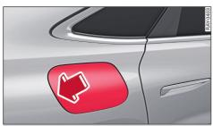
Fig. 120 Vehicle as seen from the rear right: Opening fuel tank flap
