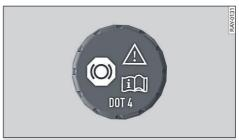
Fig. 132 Engine compartment: Cap of brake fluid reservoir
