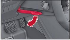
**Fig. 33** Steering column: Lever for adjusting the steering wheel position
