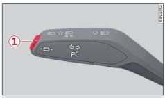
Fig. 91 Turn signal lever: Button for lane guidance and lane departure warning
