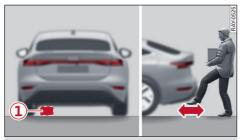
Fig. 16 Rear of vehicle: Kicking movement (example)
