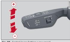
Fig. 98 Control lever: Setting a new speed
