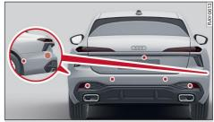
Fig. 81 Rear area: Sensors and cameras
