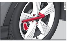
Fig. 145 Wheel: Loosening the wheel bolts
