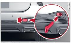
Fig. 151 Rear bumper: Fitting the towline anchorage
