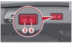
Fig. 15 Boot lid: (3) close button, (4) lock button
