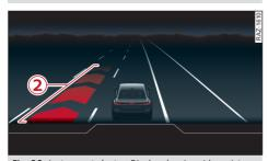
Fig. 86 Instrument cluster: Display showing side assist
