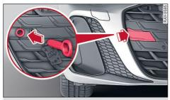
**Fig. 150** Front bumper: Fitting the towline anchorage (version 2)
