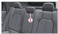
Fig. 58 Centre backrest: Release handle under head restraint
