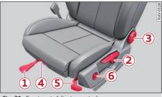
Fig. 31 Front seat: Adjuster controls
