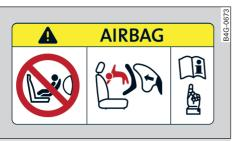
Fig. 48 Passenger's sun visor: Airbag sticker
