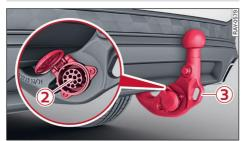
Fig. 74 Rear bumper: Connecting socket and eye for breakaway cable
