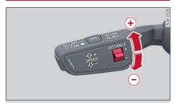
Fig. 99 Control lever: Setting the distance
