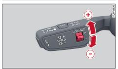
Applies to: vehicles with adaptive cruise control Fig. 94 Control lever: Deactivating distance regulating function
