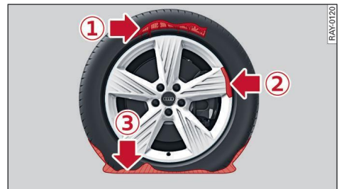
Fig. 183 Tire: tire damage that cannot be repaired
