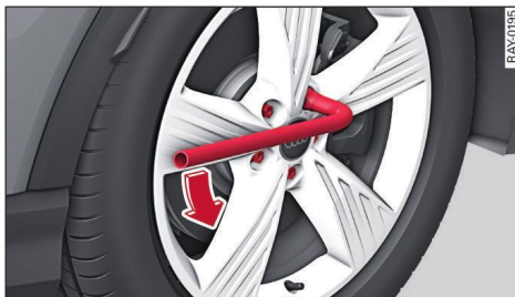
Fig. 188 Wheel: loosening the wheel bolts
