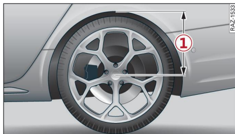
Fig. 97 Curb weight position
