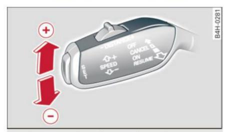
Fig. 95 Operating lever: changing the speed
