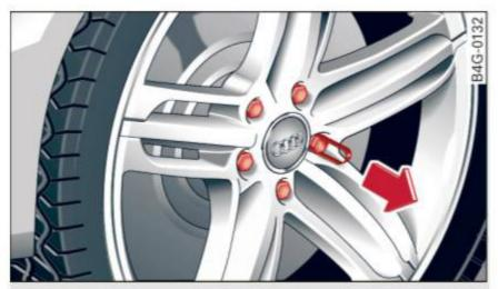
Fig. 196 Changing a wheel: removing the wheel bolt caps
