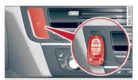
Fig. 79 Center console/remote control key: starting the engine if there is a malfunction
