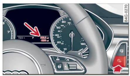
Fig. 11 Instrument cluster: odometer and reset button
