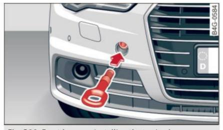
Fig. 211 Front bumper: installing the towing loop
