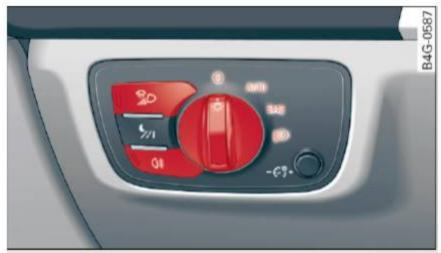
Fig. 37 Instrument panel: light switch with all weather lights
