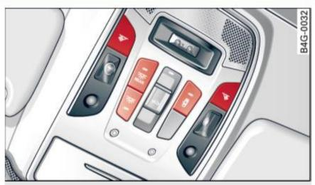
Fig. 40 Front headliner: interior lighting controls
