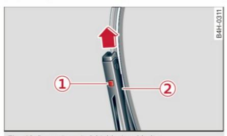
Fig. 49 Removing windshield wiper blades
