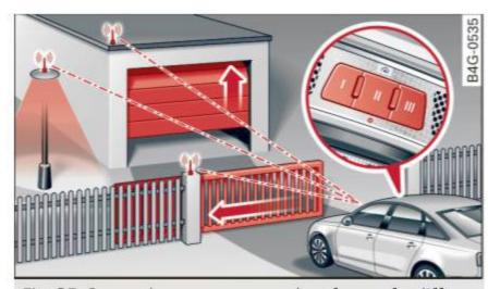
Fig. 35 Garage door opener: examples of usage for different systems
