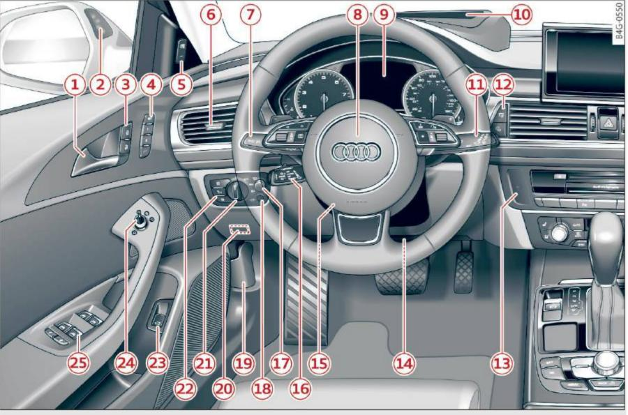
Fig. 1 Cockpit: left section
