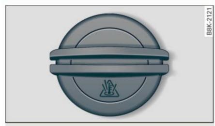
Fig. 184 Engine compartment: coolant expansion tank cover
