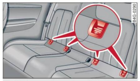
Fig. 170 Rear seats: lower anchorage bracket locations
