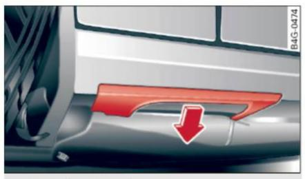
Fig. 200 Sill: removing the cover
