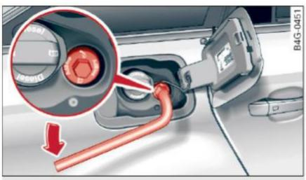
Fig. 178 Right rear side of the vehicle: removing the AdBlue cap
