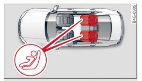
**Fig. 168** Schematic overview: LATCH anchorage point locations
