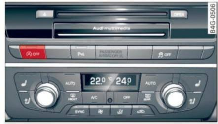
Fig. 81 Center console: Start/Stop system button
