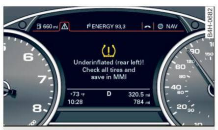
Fig. 192 Instrument cluster: indicator light with message
