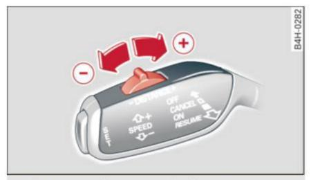
Fig. 97 Operating lever: setting the distance
