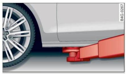
Fig. 215 Front lifting point
