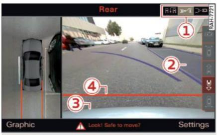
**Fig. 136** Infotainment: blue surfaces aligned in the parking space
