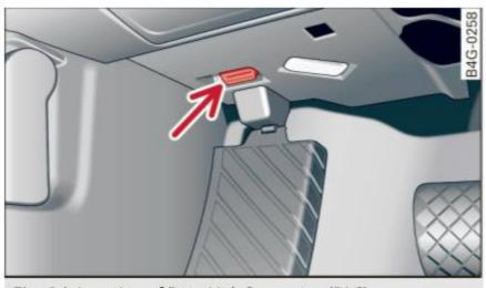
Fig. 14 Location of Data Link Connector (DLC)
