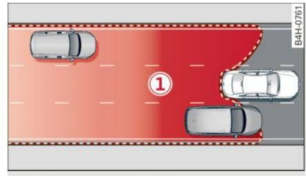
Fig. 104 Sensor detection range
