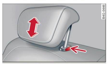
Fig. 54 Rear seat: adjusting the head restraint
