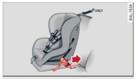
Fig. 171 Lower anchorages: proper mounting
