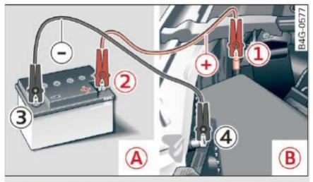
Fig. 209 Jump starting with the battery of another vehicle:
