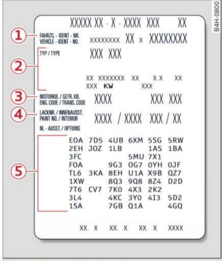
Fig. 218 Vehicle identification label
