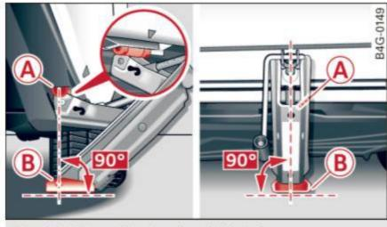
Fig. 199 Sill: positioning the vehicle jack
