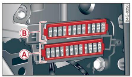
**Fig. 206** Front passenger side cockpit: fuse panel with plastic bracket
