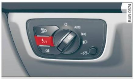
Fig. 114 Area around the light switch: night vision assistant button
