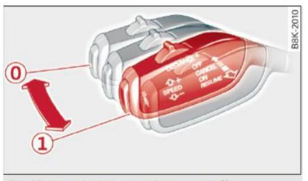
Fig. 93 Operating lever: switching on and off
