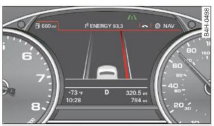
Fig. 102 Instrument cluster: active lane assist is switched on and providing warnings
