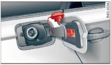
Fig. 175 Fuel filler door with attached fuel cap
