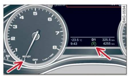
Fig. 80 Instrument cluster: engine switched off (stop phase)
