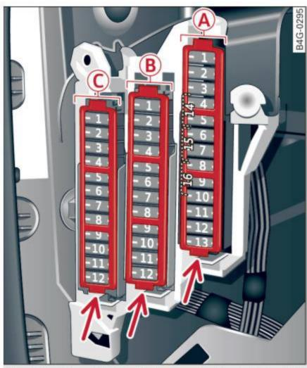
Fig. 205 Driver side cockpit: fuse panel with plastic bracket
