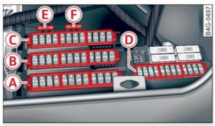
Fig. 207 Luggage compartment: fuse panel with plastic bracket
