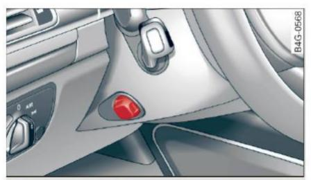
Fig. 77 Switch for adjusting the steering wheel position
