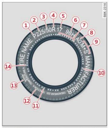
Fig. 188 Tire designations on the sidewall
