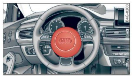
Fig. 153 Location of driver airbag: in steering wheel
