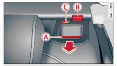
Fig. 66 Backrest: release lever, securing knob and lock\*
