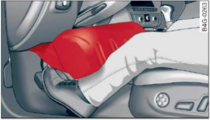
Fig. 158 Inflated airbags protecting in a frontal collision
