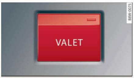
Fig. 34 Glove compartment: valet parking function button
