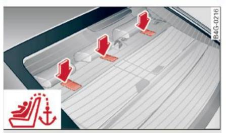
Fig. 172 Tether anchors: recess flaps behind the rear seatbacks
