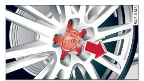
Fig. 195 Changing a wheel: Removing the wheel cover
