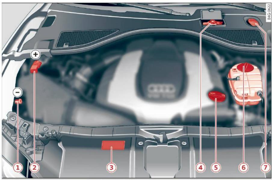
Fig. 182 Typical location of the reservoir and the engine oil filler opening
