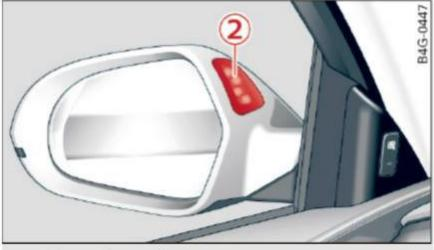
Fig. 105 Display on the exterior mirror
