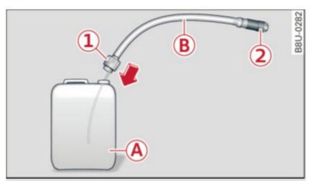
Fig. 179 Canister with attachable hose
