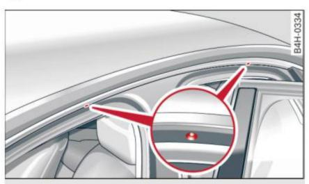
Fig. 65 Attachment points for the roof rack
