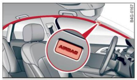
Fig. 161 Side curtain airbags, driver's side: side curtain airbag location
