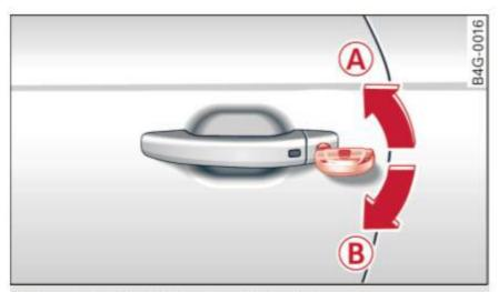
Fig. 22 Driver's door: door lock cylinder
