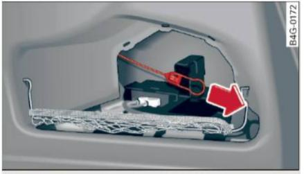
Fig. 177 Luggage compartment: fuel filler door emergency release
