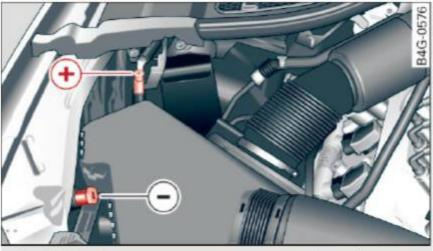
Fig. 186 Engine compartment: connectors for a charger and jump start cables
