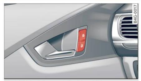
Fig. 20 Driver's door: central locking switch
