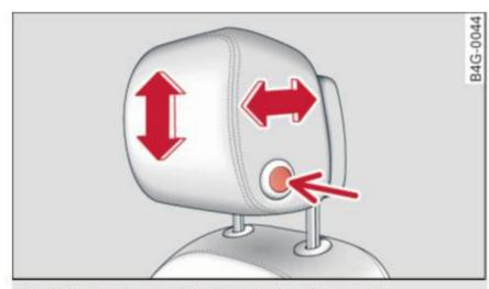
Fig. 53 Front seat: adjusting the head restraint
