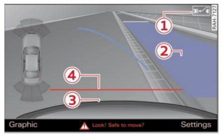
Fig. 124 Infotainment: blue surfaces aligned in the parking space
