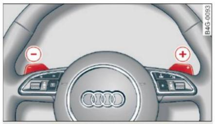
Fig. 86 Steering wheel: manual shifting with the shift paddles\*
