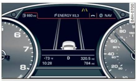
Fig. 103 Instrument cluster: active lane assist is switched on but not ready to provide warnings
