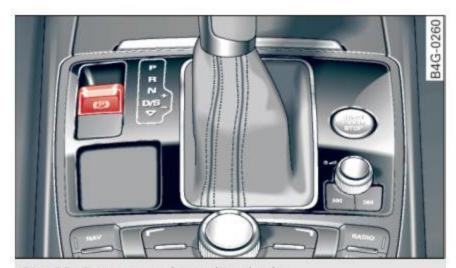
Fig. 82 Center console: parking brake
