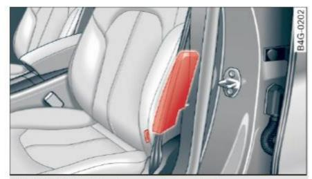
Fig. 159 Side airbag location in the driver's seat
