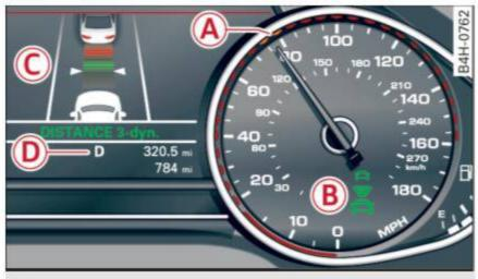
Fig. 94 Instrument cluster: adaptive cruise control
