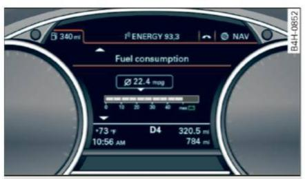
Fig. 8 Instrument cluster: fuel consumption display
