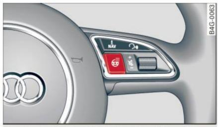
Fig. 75 Steering wheel: steering wheel heating button
