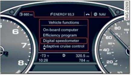
Fig. 7 Instrument cluster: opening the vehicle functions menu
