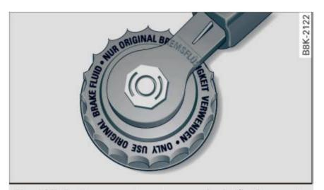
Fig. 185 Engine compartment: cap on brake fluid reservoir
