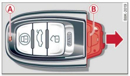
Fig. 17 Remote control key: removing the battery holder
