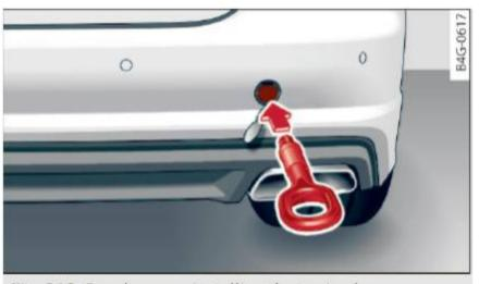
Fig. 213 Rear bumper: installing the towing loop
