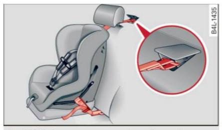
Fig. 173 Tether strap: proper routing and mounting
