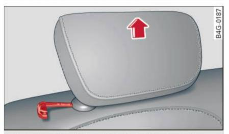
**Fig. 55** Rear seat: removing the head restraint, release point
