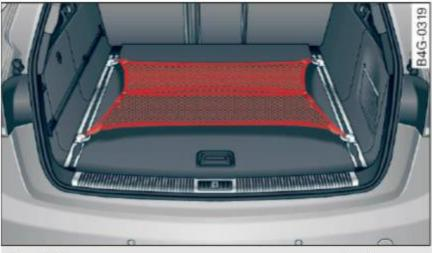
Fig. 68 Luggage compartment: cargo net stretched out
