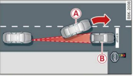
Fig. 92 Example: object changing lanes and stationary object
