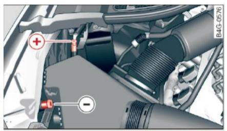
Fig. 208 Engine compartment: connectors for jump start cables and charger
