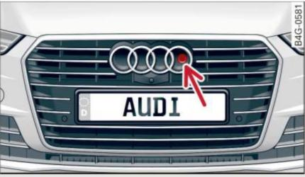
Fig. 113 Front of the vehicle: night vision assistant camera
