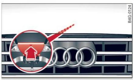
Fig. 181 Rocker switch under the hood
