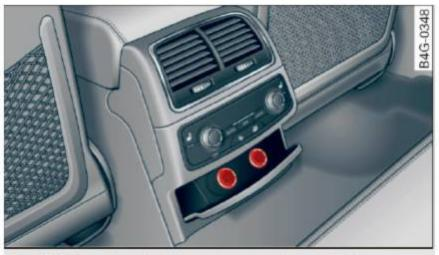
Fig. 61 Example of a rear center console: sockets\*
