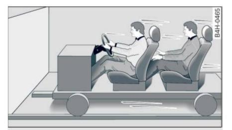
Fig. 143 Unbelted occupants in a vehicle heading for a wall
