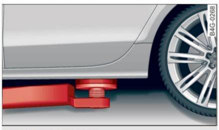
Fig. 216 Rear lifting point
