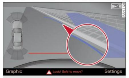
Fig. 125 Infotainment: contact of the blue curved line with the curb
