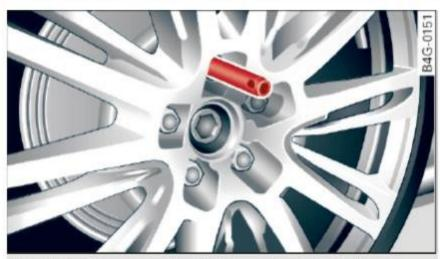
Fig. 202 Changing a wheel: alignment pin inside the top
