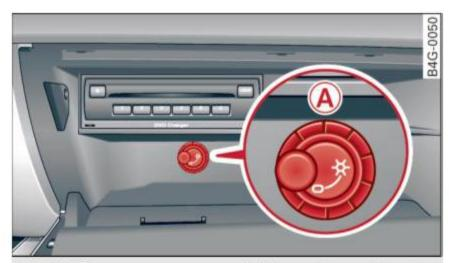
Fig. 64 Glove compartment: switching cooling mode on/
