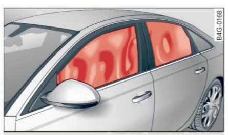
Fig. 162 Illustration of principle: Inflated side curtain airbags on the left side
