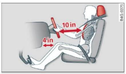
Fig. 140 Correct seating position
