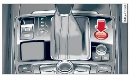
Fig. 78 Center console: START ENGINE STOP button
