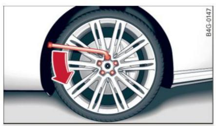
Fig. 197 Changing a wheel: loosening the wheel bolts
