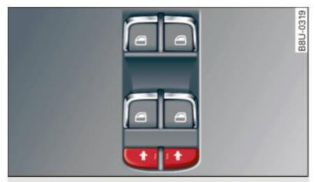
Fig. 31 Section of driver's door: child safety lock buttons
