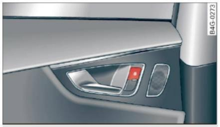
Fig. 21 Rear door: central locking switch
