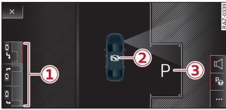
Fig. 136 Center display: activated parking space search
