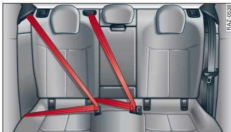
Fig. 75 Rear bench seat: securing unused safety belts
