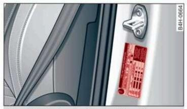
Fig. 174 Driver's side B-pillar: tire pressure label
