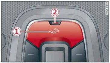
Fig. 145 Front headliner: cover for the emergency call but-
