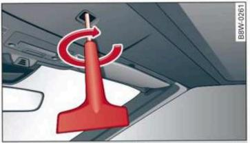
Fig. 50 Inside of the power top: locking the power top with the emergency release handle
