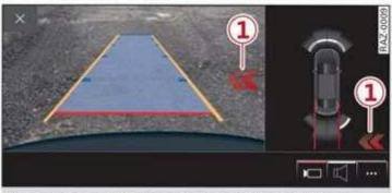
Fig. 137 Center display: rear cross-traffic assist display
