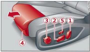
Fig. 67 Front seat: adjusting the seat (version B)
