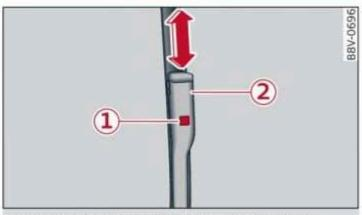
Fig. 63 Windshield wipers: changing the wiper blades
