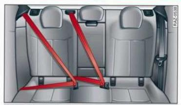
Fig. 87 Rear bench seat: securing unused safety belts
