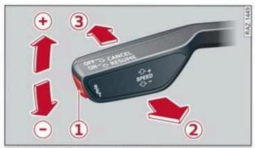
Fig. 112 Operating lever: switching the system on
