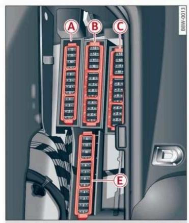
Fig. 195 Left side of the luggage compartment: fuse panel with plastic clip
