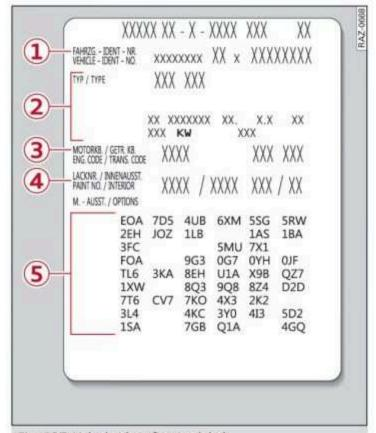
Fig. 197 Vehicle identification label
