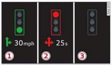
Fig. 111 Instrument cluster: traffic light information display
