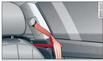
Fig. 77 Driver's seat: belt positioner
