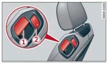
Fig. 69 Front seat: power entry assistance (version 1)
