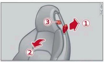
Fig. 70 Front seat: power entry assistance (version 2)
