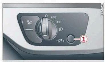
Fig. 59 Light switch: instrument illumination
