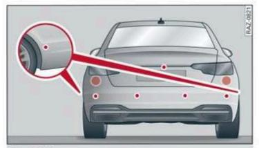
Fig. 109 Rear area: sensors and cameras
