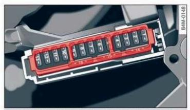
Fig. 194 Driver side cockpit: fuse panel with plastic bracket
