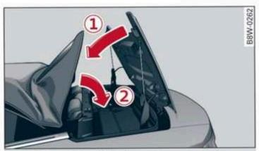
Fig. 51 Rear of the vehicle: closing the power top storage compartment lid and power top
