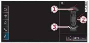
Fig. 131 Center display: distance display
