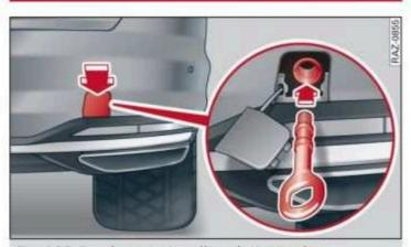
Fig. 188 Rear bumper: installing the towing loop
