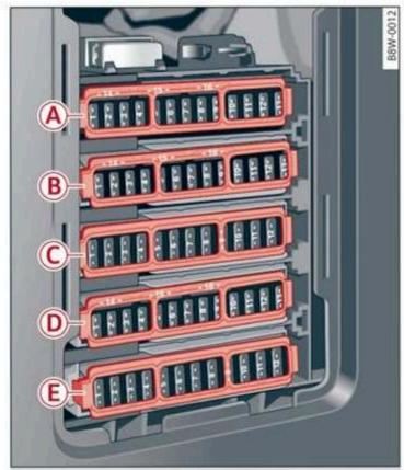
Fig. 193 Front passenger's footwell (right-hand drive vehicle): fuse panel with plastic clip
