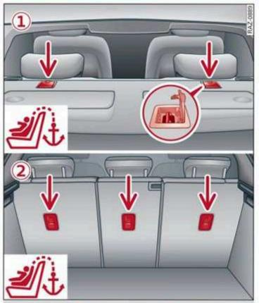
Fig. 85 Version 1 rear shelf / Version 2 rear backrest: top tether anchors for securing a child safety seat with an upper strap
