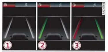
Fig. 125 Instrument cluster: driver assistance display
