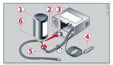
Fig. 178 Components of the tire mobility kit
