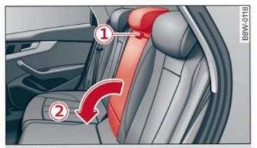
Fig. 93 Center backrest: folding the backrest forward
