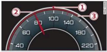
Fig. 114 Instrument cluster: display in speedometer
