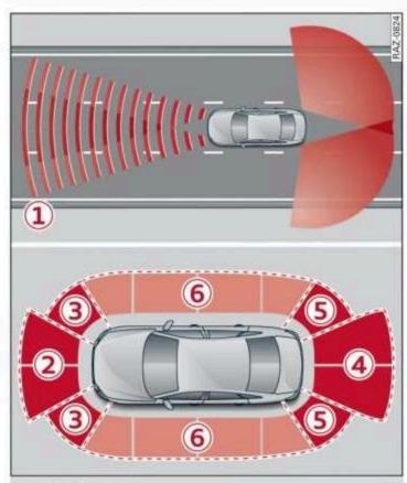
Fig. 106 Sensor detection ranges
