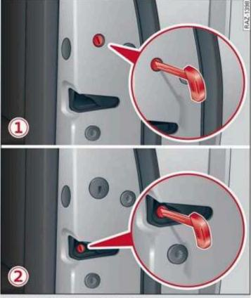
Fig. 25 Door: mechanically locking
