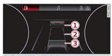
Applies to: vehicles with adaptive cruise control: Fig. 123 Instrument cluster: display of the current distance
