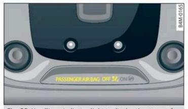
Fig. 83 Headliner: indicator light to display the status of the front passenger's airbag
