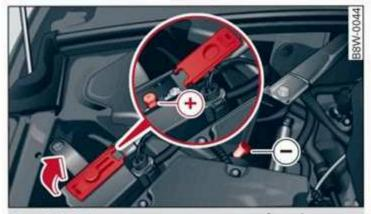
Fig. 170 Engine compartment: connectors for a charger or jump start cables
