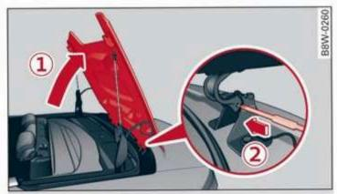
Fig. 48 Rear of the vehicle: lifting the power top storage compartment lid out and securing
