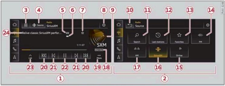
Fig. 157 Center display: left side: playback view of radio functions, right side: sources
