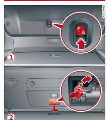
Fig. 34 Inner luggage compartment lid: access to the emergency release. ① Coupe, ② Sportback
