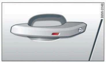
Fig. 27 Door handle: sensor for locking
