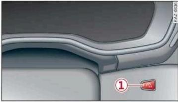
Fig. 7 Instrument cluster: reset button
