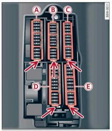
Fig. 192 Driver's footwell (left-hand drive vehicle): fuse panel with plastic clip
