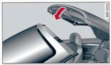
Fig. 49 Windshield: closing the power top
