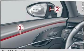
Fig. 129 Front door: exit warning
