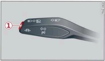
Fig. 126 Turn signal lever: button for Audi active lane assist
