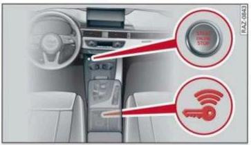
Fig. 100 Center console: starting the engine
