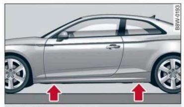
Fig. 182 Sill panels: markings
