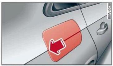
Fig. 161 Right rear side of the vehicle: opening the fuel filler door
