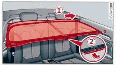
Fig. 44 Rear of the vehicle: inserting the wind deflector (1)
