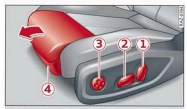
Fig. 66 Front seat: adjusting the seat (version A)
