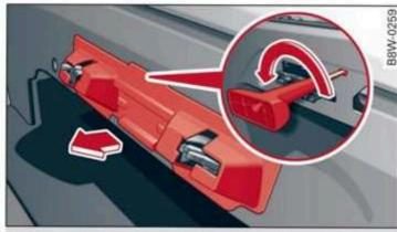
Fig. 47 Rear bench seat: releasing the power top storage compartment lid with the emergency release handle
