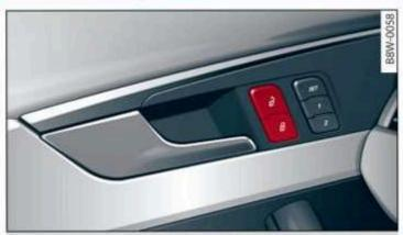
Fig. 23 Driver's door: central locking switch
