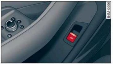
Fig. 31 Driver's door: opening the luggage compartment
