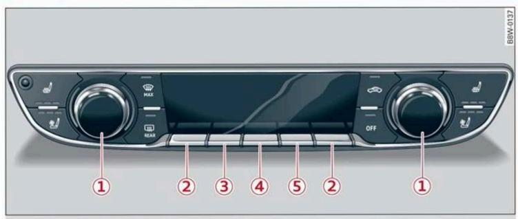
Fig. 98 3-zone deluxe automatic climate control system: controls
