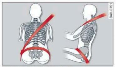
Fig. 75 Lap/shoulder belt positioning
