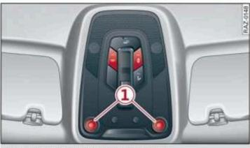
Fig. 57 Headliner: front interior lighting
