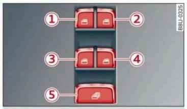
Fig. 39 Driver's door: power window switch\*
