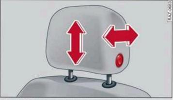
Fig. 73 Front seat: adjusting the head restraint
