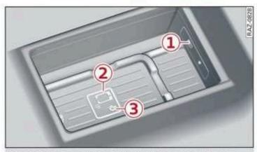
Fig. 141 Front center console: Audi phone box with connections
