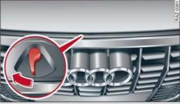
Fig. 164 Unlocked hood: lever
