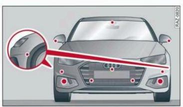
Fig. 108 Front area: sensors and cameras
