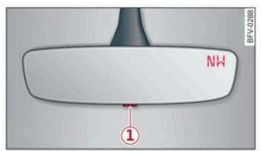
Fig. 64 Rearview mirror: digital compass is switched on
