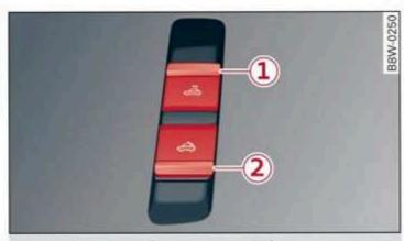
Fig. 41 Center console: power top switch
