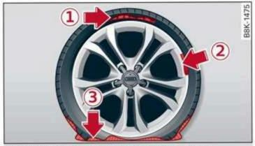
Fig. 177 Tire: tire damage that cannot be repaired
