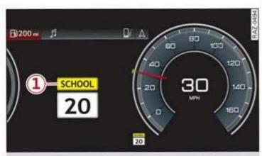
Fig. 110 Instrument cluster: traffic sign recognition
