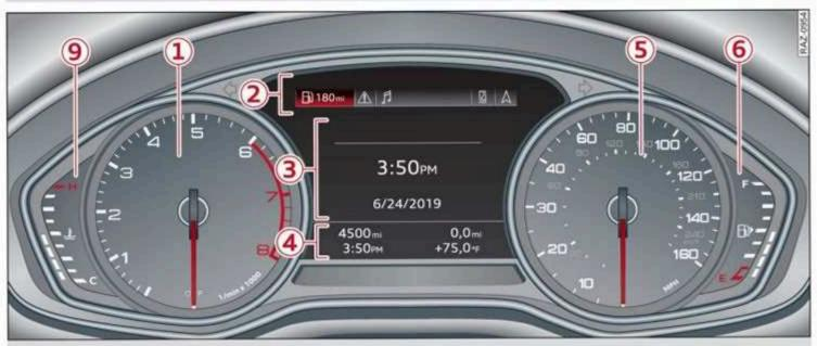
Fig. 3 Instrument cluster overview (analog)
