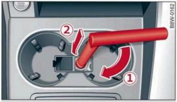
Fig. 105 Front cup holder: parking lock emergency release
