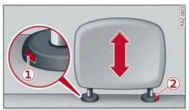
Fig. 74 Rear seat: adjusting or removing the head restraint
