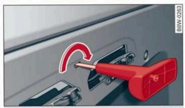
Fig. 52 Rear bench seat: locking the power top storage compartment lid with the emergency release handle
