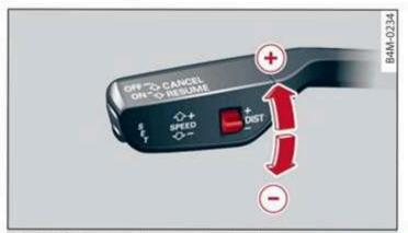
Fig. 118 Operating lever: setting the distance
