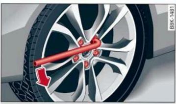
Fig. 181 Wheel: loosening the wheel bolts
