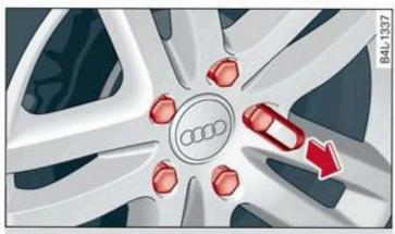
Fig. 180 Wheel: wheel bolts with caps
