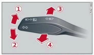
Fig. 54 Operating lever: switching the light functions on and off
