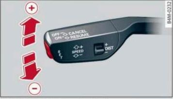
Fig. 117 Operating lever: changing the speed
