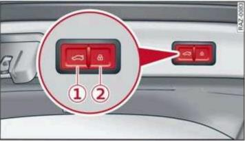
Fig. 32 Luggage compartment lid: (1) closing button\*, (2) lock button\* (vehicles with convenience key\*)
