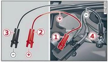
Fig. 187 Engine compartment: connectors for jump start cables or a charger
