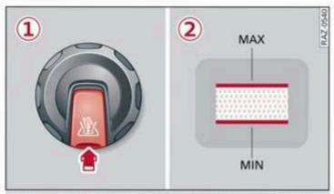
Fig. 168 Engine compartment - Coolant expansion tank (diagram): 1) cover with release button; 2) markings
