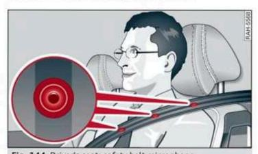
Fig. 144 Driver's seat: safety belt microphone
