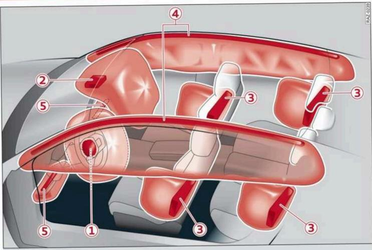
Applies to: vehicles without power top: Fig. 81 Airbag layout (enlarged section/deployed airbags)
