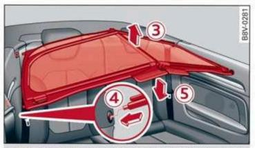
Fig. 45 Rear of the vehicle: inserting the wind deflector (2)
