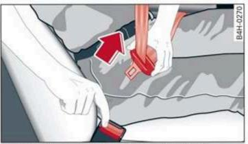
Fig. 79 Releasing the belt buckle from the belt latch
