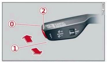
Fig. 116 Operating lever: operating adaptive cruise control
