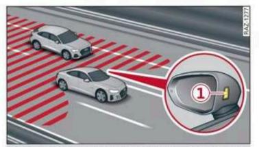
Fig. 127 Driving situations and displays in the exterior mirror
