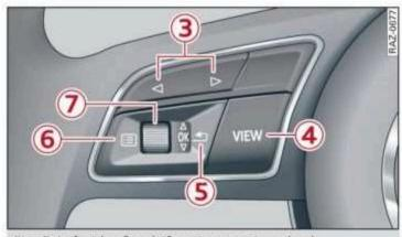
Fig. 5 Left side of multifunction steering wheel
