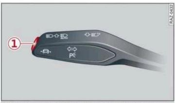
Fig. 122 Turn signal lever: button for traffic jam assist and Audi active lane assist
