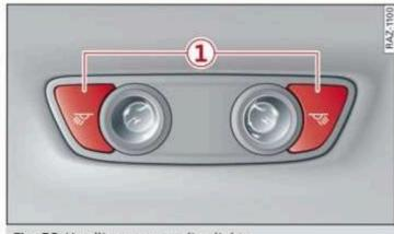
Fig. 58 Headliner: rear reading lights
