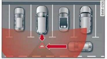
Fig. 136 Sensor detection range for rear cross-traffic assist
