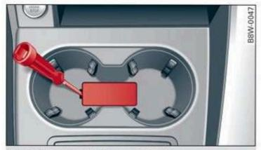
Fig. 104 Front cup holder: removing the cover
