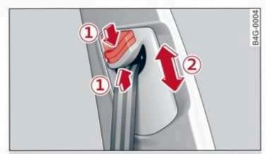
Fig. 80 Belt height adjustment for the front seats - safety belt relay
