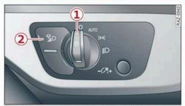
Fig. 53 Instrument panel: light switch with button
