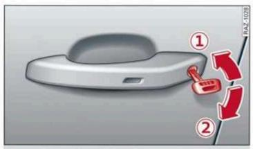
Fig. 42 Driver's door: turning the key to open and close
