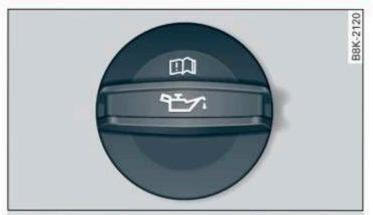
Fig. 167 Engine compartment: engine oil filling opening cover (example)
