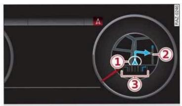
Fig. 152 Instrument cluster: default view: turning maneuver when route guidance has started
