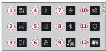
Fig. 16 Center display: frequently used symbols in the status bar
