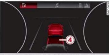
Applies to: vehicles with Audi adaptive cruise control Fig. 124 Instrument cluster: distance warning
