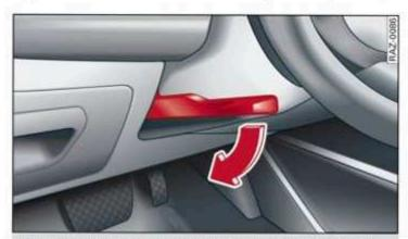
Fig. 71 Steering column: lever for adjusting the steering wheel position
