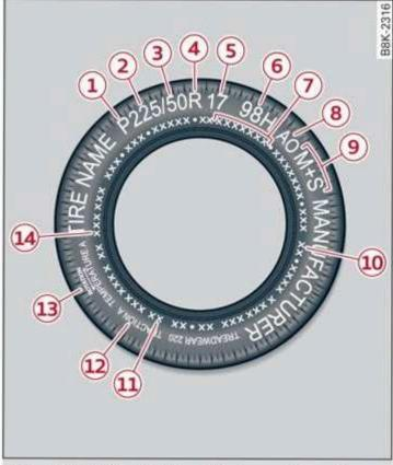
Fig. 172 Tire designations on the sidewall
