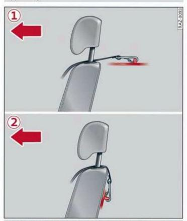
Fig. 86 Version 1 rear shelf / Version 2 rear backrest: securing the upper strap on the top tether anchor
