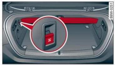
Fig. 43 Luggage compartment: power top storage compartment and button
