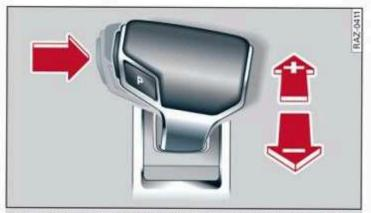
Fig. 102 Center console: shifting manually with the selector lever
