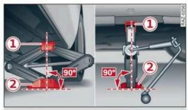
Fig. 183 Sill: positioning the vehicle jack
