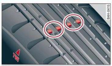
Fig. 173 Tire profile: treadwear indicator
