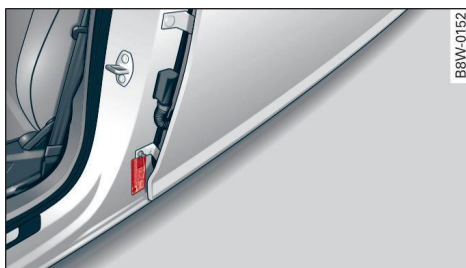
Fig. 170 Driver's side B-pillar: tire pressure label
