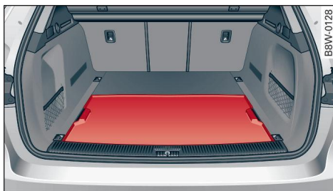
Fig. 90 Luggage compartment: cargo area floor reversed
