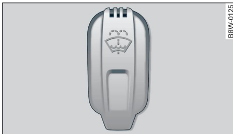
Fig. 167 Engine compartment: washer fluid reservoir cap
