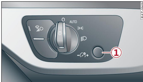
Fig. 49 Light switch: instrument illumination
