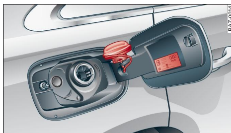
Fig. 157 Fuel filler door with attached fuel cap
