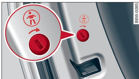
Applies to: vehicles with manual child safety locks Fig. 39 Rear door: manual child safety lock
