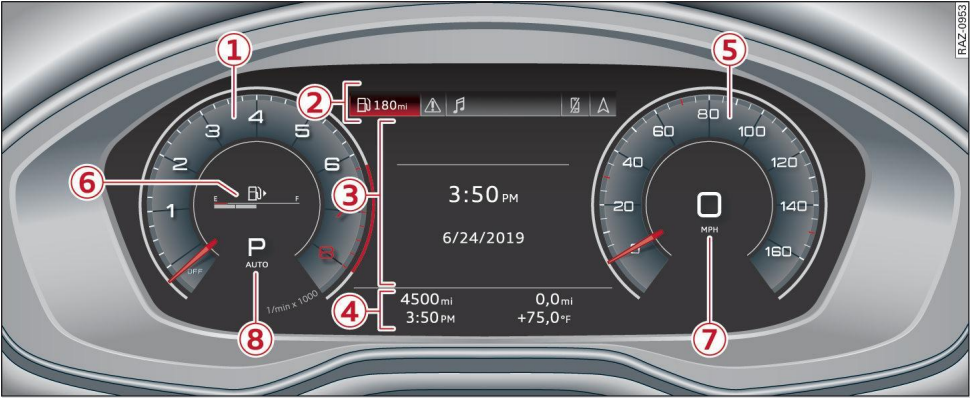
Fig. 3 Instrument cluster overview (Audi virtual cockpit)
