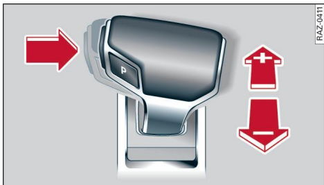
Fig. 97 Center console: shifting manually with the selector
