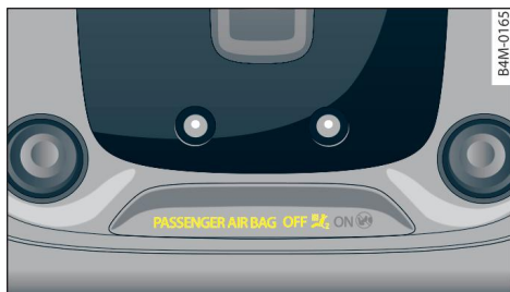
Fig. 72 Headliner: indicator light to display the status of the front passenger's airbag
