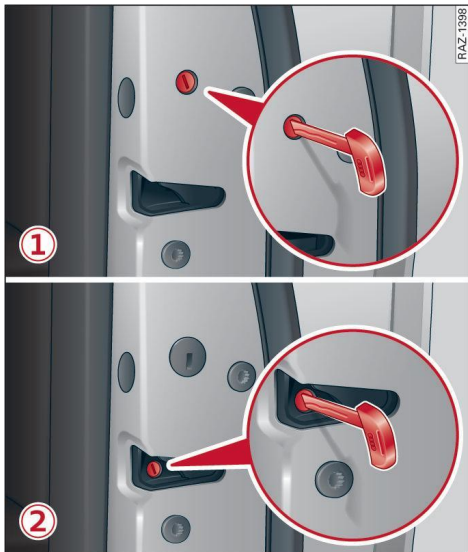
Fig. 26 Door: mechanically locking
