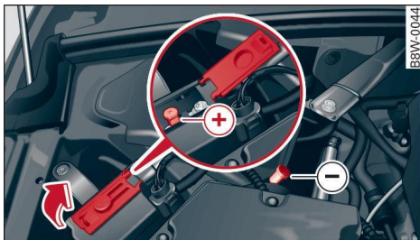
Fig. 182 Engine compartment: connectors for jump start cables or a charger
