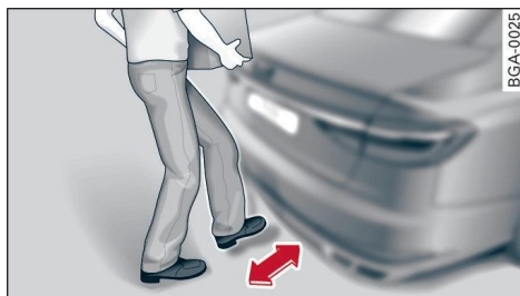
Fig. 34 Vehicle rear: foot motion (example)
