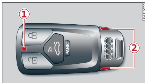
Fig. 29 Vehicle key: removing the battery holder
