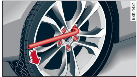
Fig. 177 Wheel: loosening the wheel bolts
