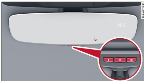
Fig. 43 Rearview mirror: buttons for the garage door opener
