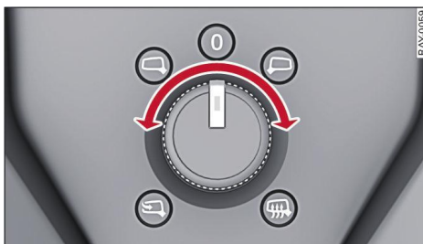
Fig. 50 Driver's door: knob for the exterior mirrors
