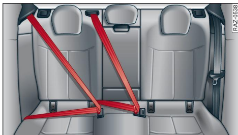
Fig. 76 Rear bench seat: securing unused safety belts
