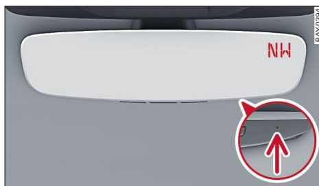
Fig. 57 Rearview mirror: digital compass is turned on
