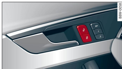
Fig. 24 Driver's door: central locking switch
