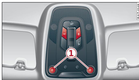
Fig. 47 Headliner: front interior lighting
