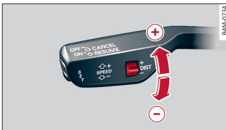
Fig. 115 Lever: setting the distance
