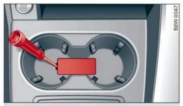
Fig. 98 Front cup holder: removing the cover
