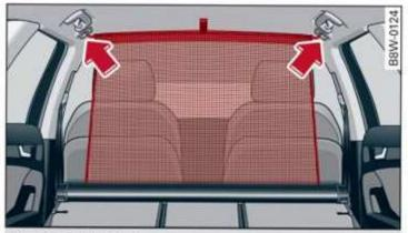
Fig. 86 Folded backrest: setting up the partition net
