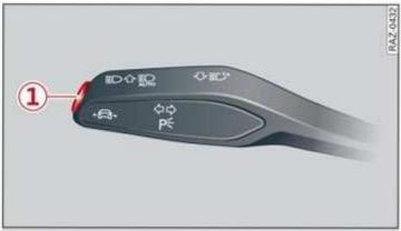
Fig. 121 Turn signal lever: button for Audi active lane assist
