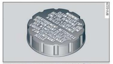
Fig. 164 Engine compartment: cap on brake fluid reservoir
