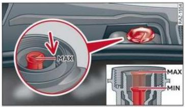
Fig. 163 Coolant expansion tank markings (6-cylinder engine)
