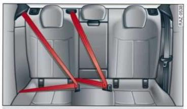
Fig. 75 Rear bench seat: securing unused safety belts
