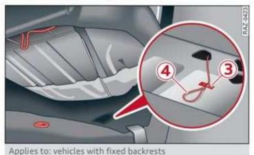
Fig. 36 Rear bench seat: release cable for emergency release in the sedan
