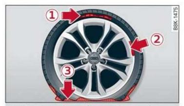
Fig. 172 Tire: tire damage that cannot be repaired
