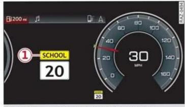
Fig. 105 Instrument cluster: traffic sign recognition
