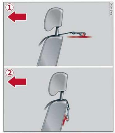
Fig. 74 Version 1 rear shelf / Version 2 rear backrest: securing the upper strap on the top tether anchor
