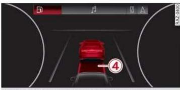
Applies to: vehicles with Audi adaptive cruise control Fig. 119 Instrument cluster: distance warning
