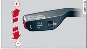
Fig. 112 Operating lever: changing the speed
