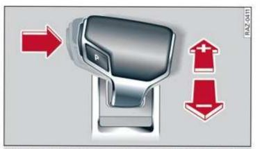
Fig. 96 Center console: shifting manually with the selector lever
