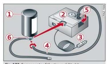
Fig. 173 Components of the tire mobility kit
