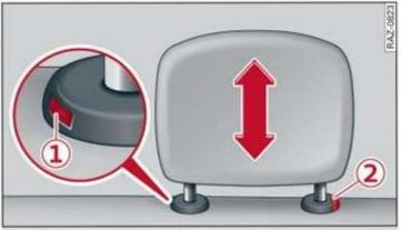
Fig. 64 Rear seat: adjusting or removing the head restraint
