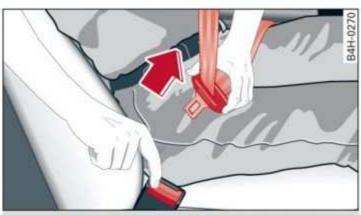
Fig. 68 Releasing the belt buckle from the belt latch
