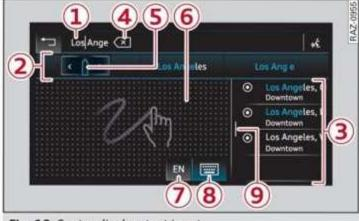
Fig. 19 Center display: text input
