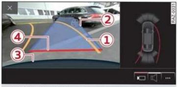
Fig. 129 Center display: aiming at a parking spot
