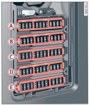
Fig. 187 Front passenger's footwell (right-hand drive vehicle): fuse panel with plastic clip
