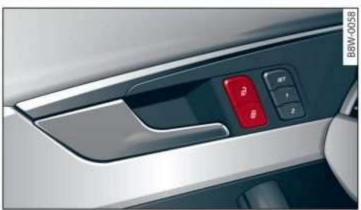
Fig. 24 Driver's door: central locking switch
