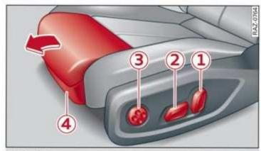
Fig. 58 Front seat: adjusting the seat (version A)
