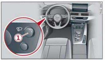
Fig. 20 Instrument panel: knob for the head-up display
