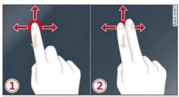
Fig. 14 Touch display: 1 dragging with one finger, 2 dragging with two fingers
