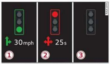
Fig. 106 Instrument cluster: traffic light information display
