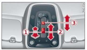
Fig. 42 Headliner: panoramic glass roof and sunshade\* buttons
