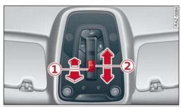
Fig. 41 Section of front headliner: sliding/tilting sunroof button
