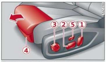
Fig. 59 Front seat: adjusting the seat (version B)
