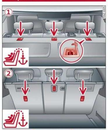
Fig. 73 Version 1 rear shelf / Version 2 rear backrest: top tether anchors for securing a child safety seat with an upper strap
