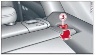
Fig. 78 Luggage compartment: removing the luggage compartment cover
