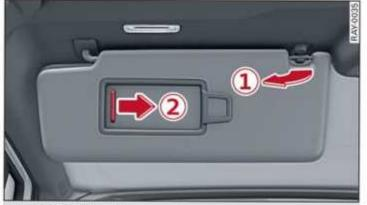
Fig. 50 Roof headliner: sun visor
