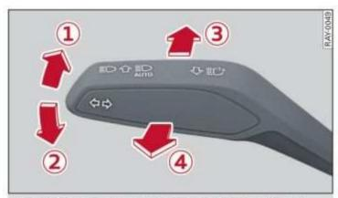
Fig. 44 Operating lever: switching the light functions on and off
