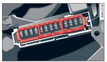
Fig. 188 Driver side cockpit: fuse panel with plastic bracket
