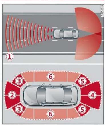
Fig. 100 Sensor detection ranges
