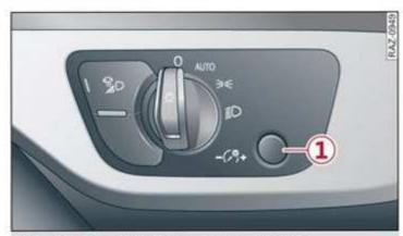
Fig. 48 Light switch: instrument illumination
