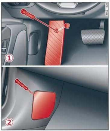
Fig. 184 Driver's side footwell (left-hand drive vehicles): footrest 1, front passenger's side footwell (right-hand drive vehicles): cover 2
