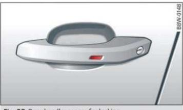
Fig. 28 Door handle: sensor for locking
