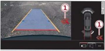
Fig. 132 Center display: rear cross-traffic assist display
