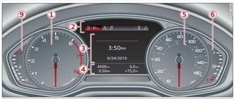
Fig. 4 Instrument cluster overview (analog)
