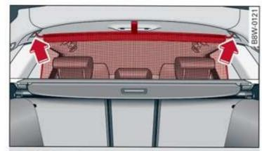
Fig. 83 Behind the backrest: hanging the partition net
