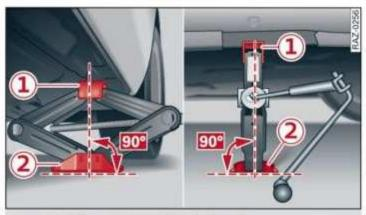
Fig. 178 Sill: positioning the vehicle jack
