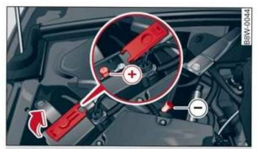
Fig. 181 Engine compartment: connectors for jump start cables or a charger
