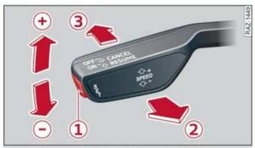
Fig. 107 Operating lever: switching the system on
