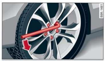
Fig. 176 Wheel: loosening the wheel bolts
