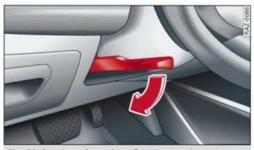
Fig. 61 Steering column: lever for adjusting the steering wheel position
