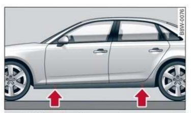
Fig. 177 Sill panels: markings
