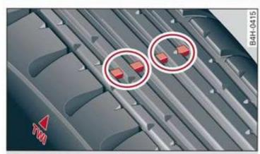
Fig. 168 Tire profile: treadwear indicator
