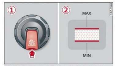
Fig. 162 Engine compartment - coolant expansion tank (diagram): 1 cover with release button; 2 coolant expansion tank markings (4-cylinder engine)
