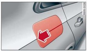
Fig. 155 Right rear side of the vehicle: opening the fuel filler door
