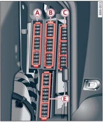
Fig. 189 Left side of the luggage compartment: fuse panel with plastic clip
