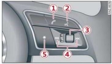
Fig. 22 Right side of the multifunction steering wheel
