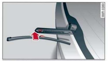
Fig. 55 Rear window wiper: installing the wiper blade
