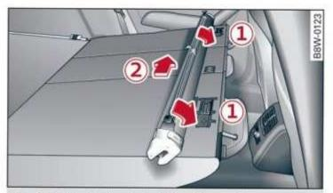
Fig. 85 Folded backrest: installing the partition net
