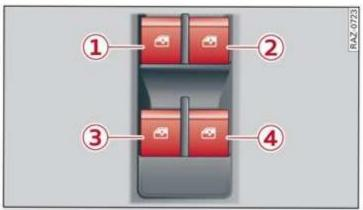
Fig. 40 Driver's door: power window switch
