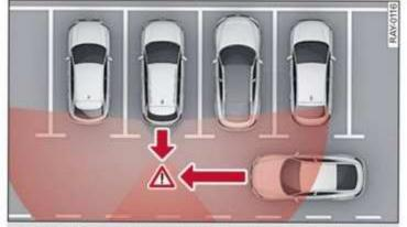
Fig. 131 Sensor detection range for rear cross-traffic assist
