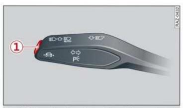
Fig. 117 Turn signal lever: button for traffic jam assist and Audi active lane assist
