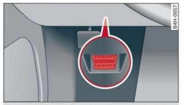
Fig. 190 Driver's side footwell: connection port for the On Board Diagnostic System (OBD)
