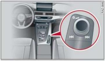
Fig. 23 MMI On/Off knob with joystick function
