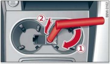
Fig. 99 Front cup holder: parking lock emergency release
