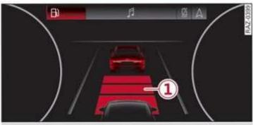
Fig. 113 Instrument cluster: brake intervention request
