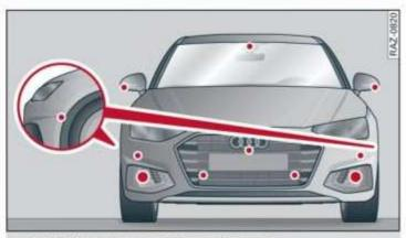
Fig. 102 Front area: sensors and cameras
