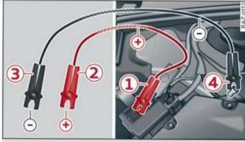
Fig. 182 Connecting the jump start cables
