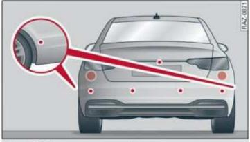
Fig. 103 Rear area: sensors and cameras
