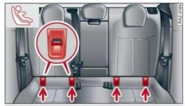
Fig. 72 Rear bench seat: lower LATCH anchors
