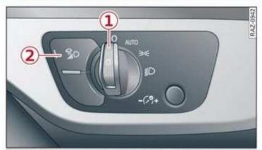
Fig. 43 Instrument panel: light switch with button
