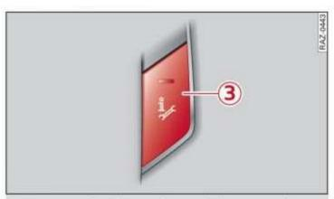
Fig. 140 Front headliner: online roadside assistance button
