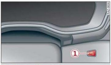
Fig. 8 Instrument cluster: reset button
