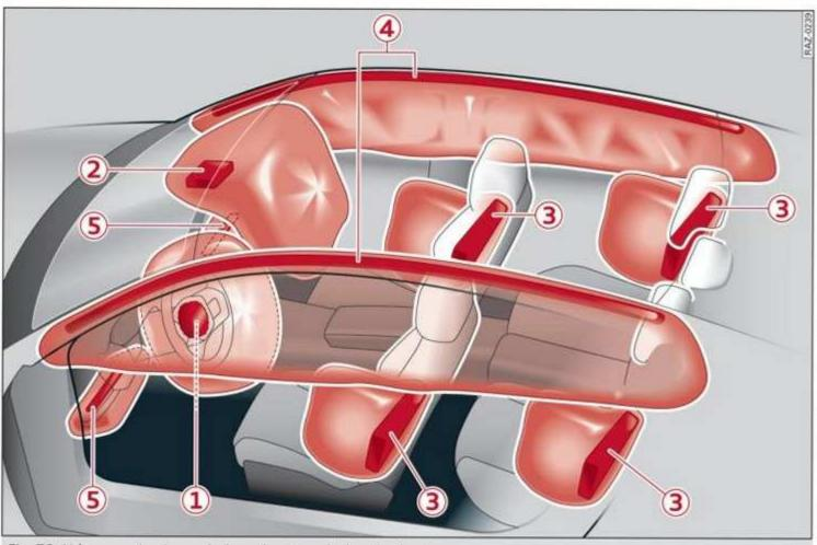
Fig. 70 Airbag overview image (enlarged section: deployed airbags)
