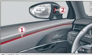
Fig. 124 Front door: exit warning
