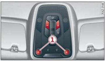
Fig. 46 Headliner: front interior lighting
