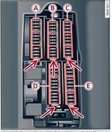
Fig. 186 Driver's footwell (left-hand drive vehicle): fuse panel with plastic clip
