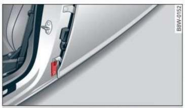
Fig. 169 Driver's side B-pillar: tire pressure label
