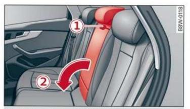
Fig. 81 Center backrest: folding the backrest forward
