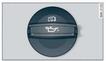
Fig. 161 Engine compartment: engine oil filling opening cover (example)
