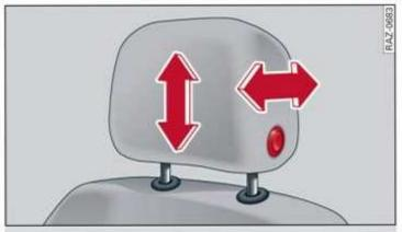
Fig. 63 Front seat: adjusting the head restraint
