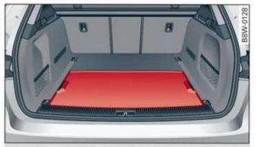
Fig. 89 Luggage compartment: cargo area floor reversed
