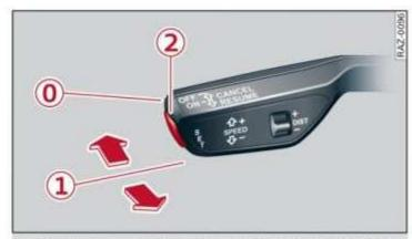
Fig. 115 Lever: operating the Audi adaptive cruise control
