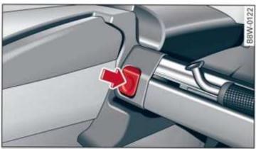
Fig. 84 Behind the backrest: removing the partition net
