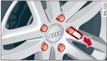
Fig. 175 Wheel: wheel bolts with caps
