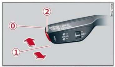
Fig. 111 Operating lever: operating adaptive cruise control
