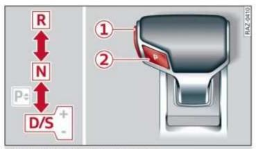
Fig. 95 Center console: selector lever
