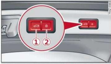
Fig. 33 Luggage compartment lid: (1) closing button\*, (2) lock button\* (vehicles with convenience key\*)
