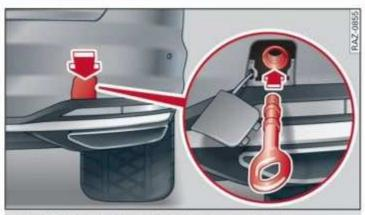
Fig. 183 Rear bumper: installing the towing loop
