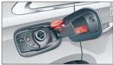
Fig. 156 Fuel filler door with attached fuel cap
