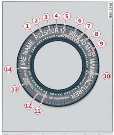
Fig. 167 Tire designations on the sidewall
