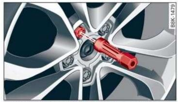
Fig. 179 Wheel: internal hex socket to turn the wheel bolts
