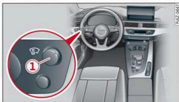
Fig. 19 Instrument panel: knob for the head-up display
