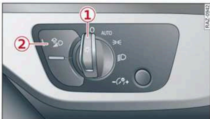
Fig. 42 Instrument panel: light switch with button
