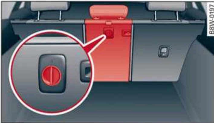
Fig. 81 Center backrest: folding the backrest forward
