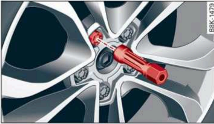
Fig. 176 Wheel: internal hex socket to turn the wheel bolts
