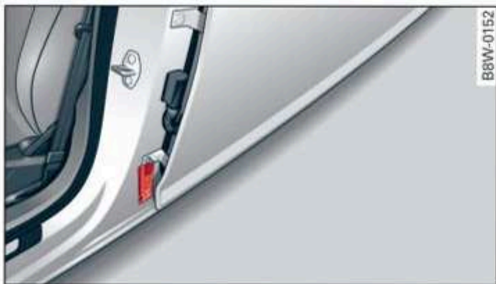
Fig. 166 Driver's side B-pillar: tire pressure label
