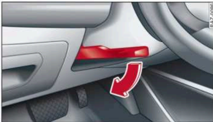
Fig. 60 Steering column: lever for adjusting the steering wheel position
