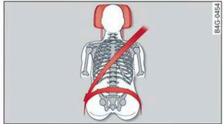
Fig. 61 Correctly-adjusted head restraint
