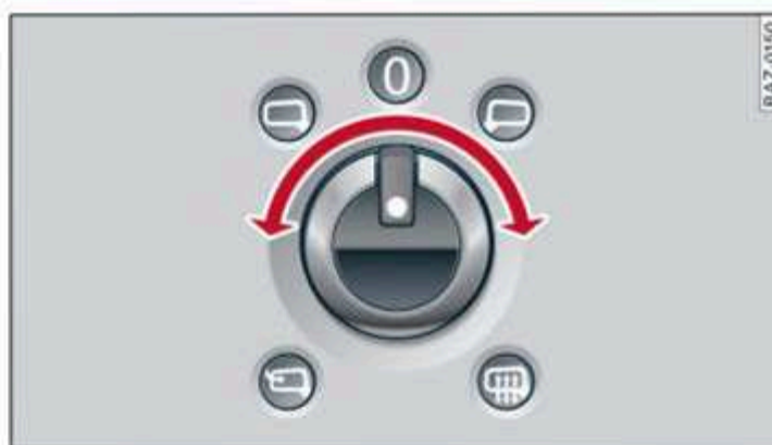
Fig. 48 Driver's door: knob for the exterior mirrors
