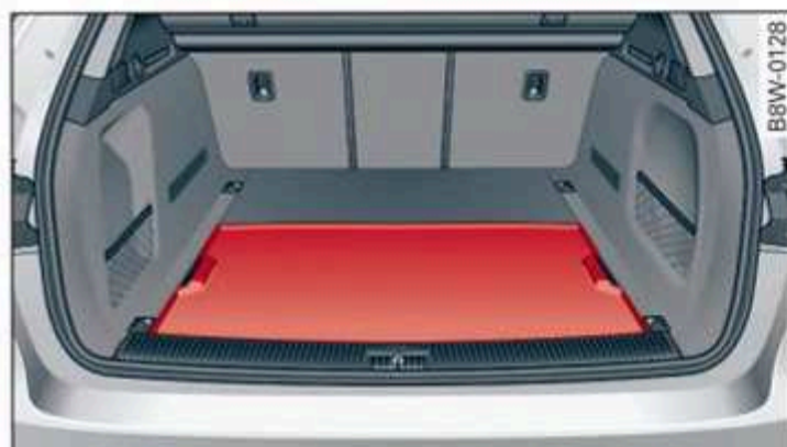
Fig. 88 Luggage compartment: cargo area floor reversed
