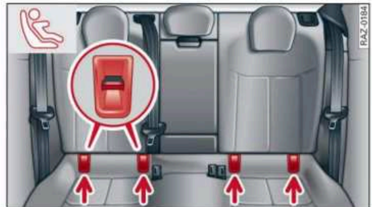
Fig. 71 Rear bench seat: lower LATCH anchors
