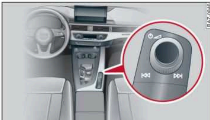
Fig. 22 MMI On/Off knob with joystick function
