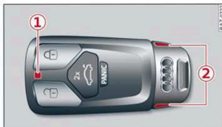
Fig. 28 Vehicle key: removing the battery holder
