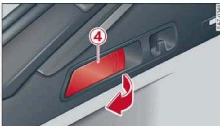
Fig. 79 Luggage compartment: release lever
