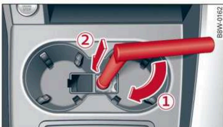
Fig. 98 Front cup holder: parking lock emergency release
