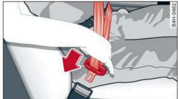
Fig. 66 Belt buckle and belt latch
