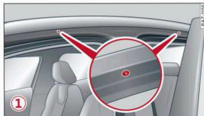
Fig. 89 Roof: mounting points
