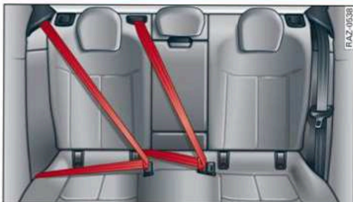
Fig. 74 Rear bench seat: securing unused safety belts
