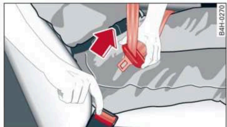
Fig. 67 Releasing the belt buckle from the belt latch
