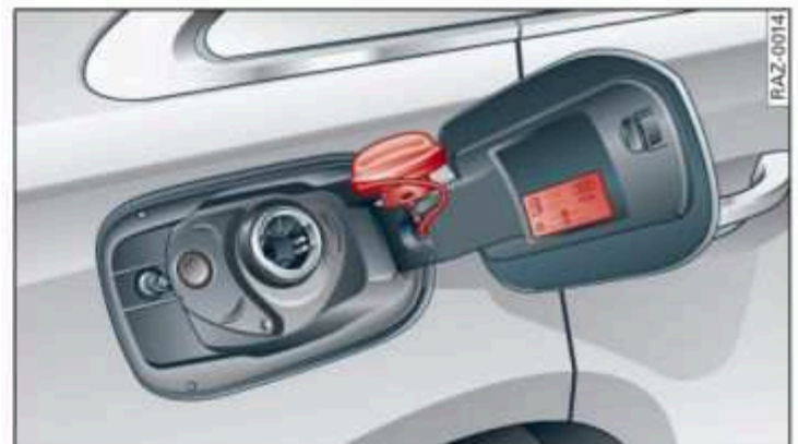
Fig. 154 Fuel filler door with attached fuel cap
