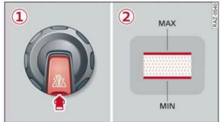
Fig. 160 Engine compartment - Coolant expansion tank (diagram): ① cover with release button; ② markings
