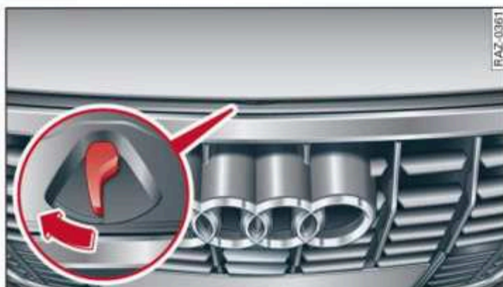
Fig. 156 Unlocked hood: lever
