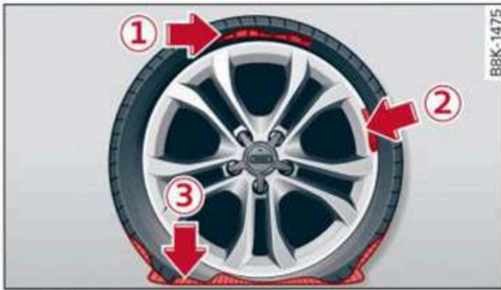
Fig. 169 Tire: tire damage that cannot be repaired
