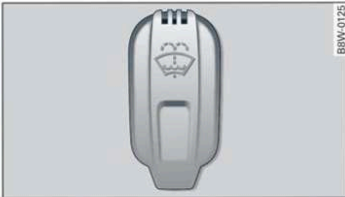
Fig. 163 Engine compartment: washer fluid reservoir cap
