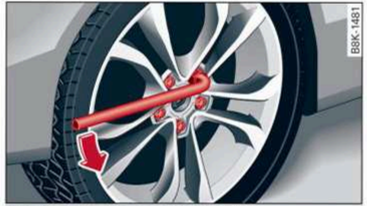
Fig. 173 Wheel: loosening the wheel bolts
