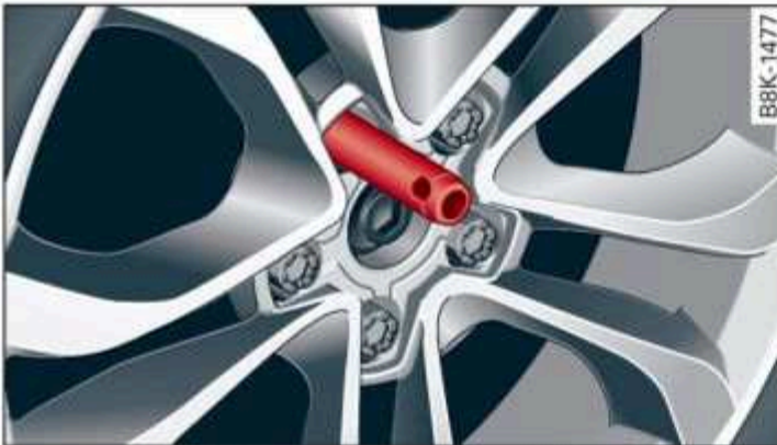
Fig. 177 Wheel: alignment pin in the top hole
