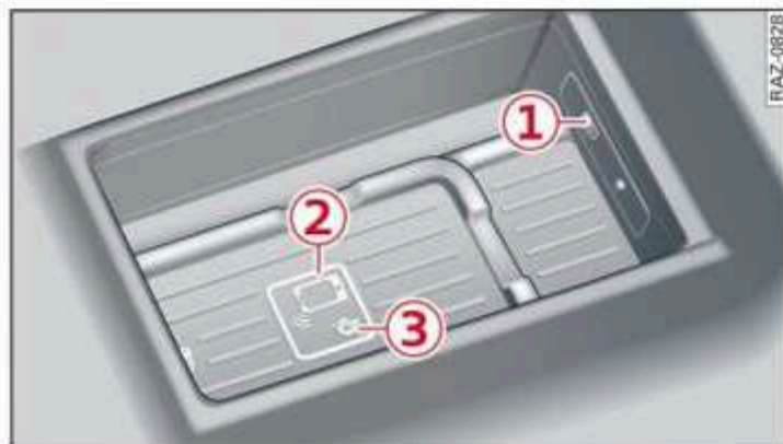
Fig. 134 Front center console: Audi phone box with connections
