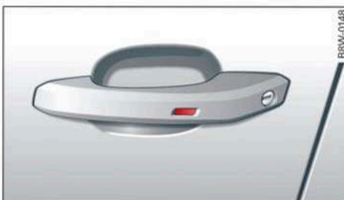
Fig. 27 Door handle: sensor for locking
