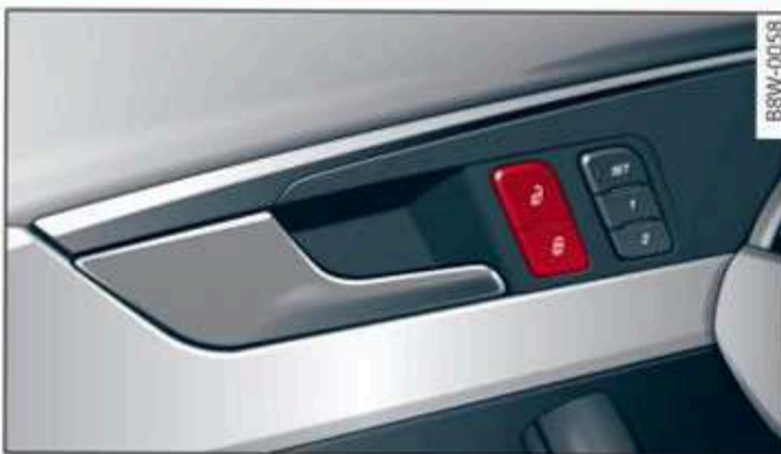
Fig. 23 Driver's door: central locking switch
