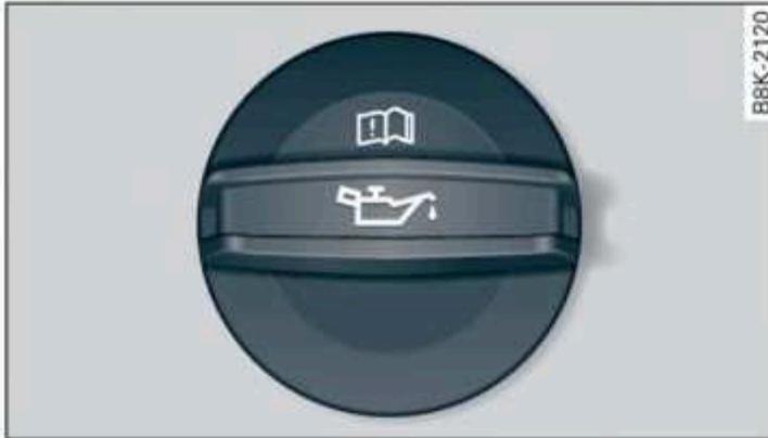
Fig. 159 Engine compartment: engine oil filling opening cover (example)
