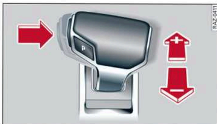
Fig. 95 Center console: shifting manually with the selector lever
