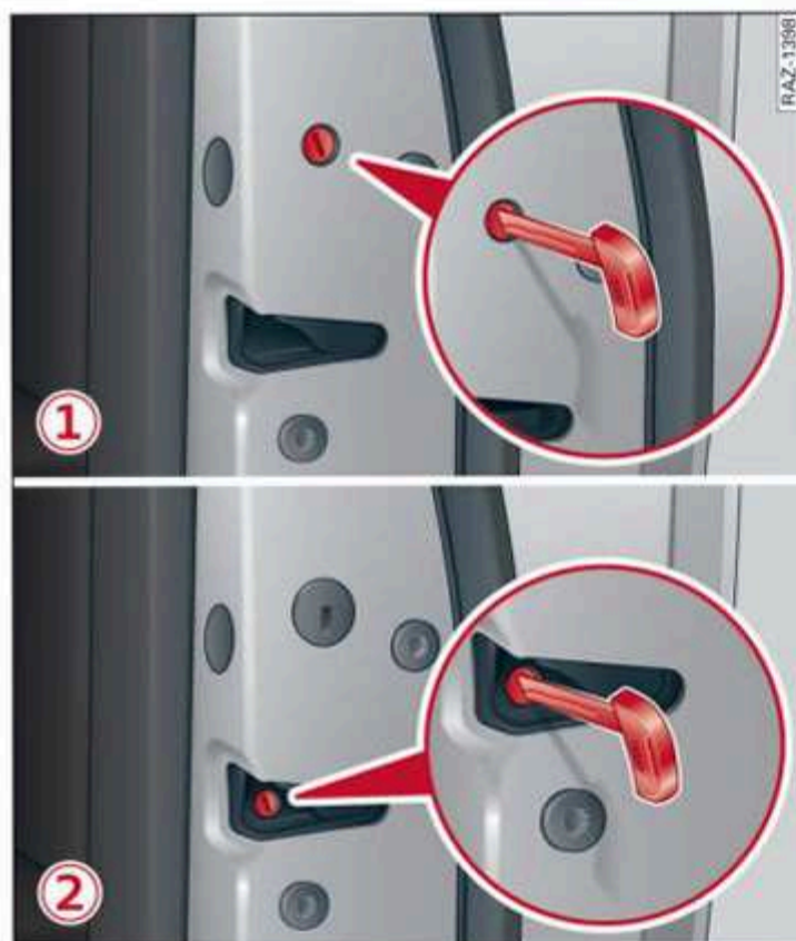
Fig. 25 Door: mechanically locking
