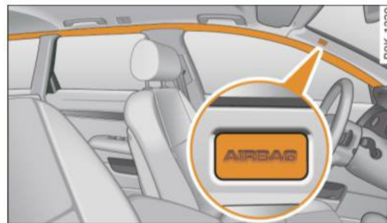
Fig. 192 Side curtain system, driver's side: side curtain airbag location
