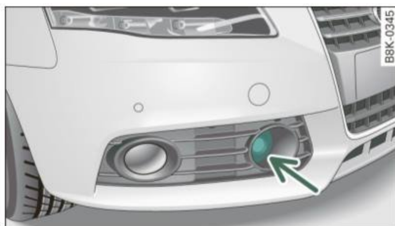
Fig. 121 Front bumper: Position of radar sensor
