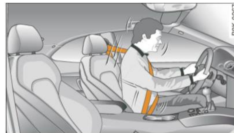
Fig. 180 Driver is correctly restrained in a sudden braking maneuver
