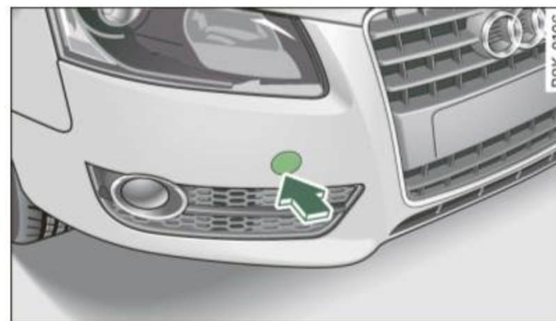
Fig. 241 Front bumper: removing the cover cap
