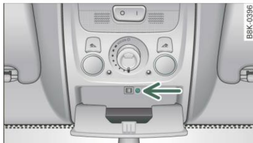
Fig. 48 Section from headliner: Unscrewing the lighting unit
