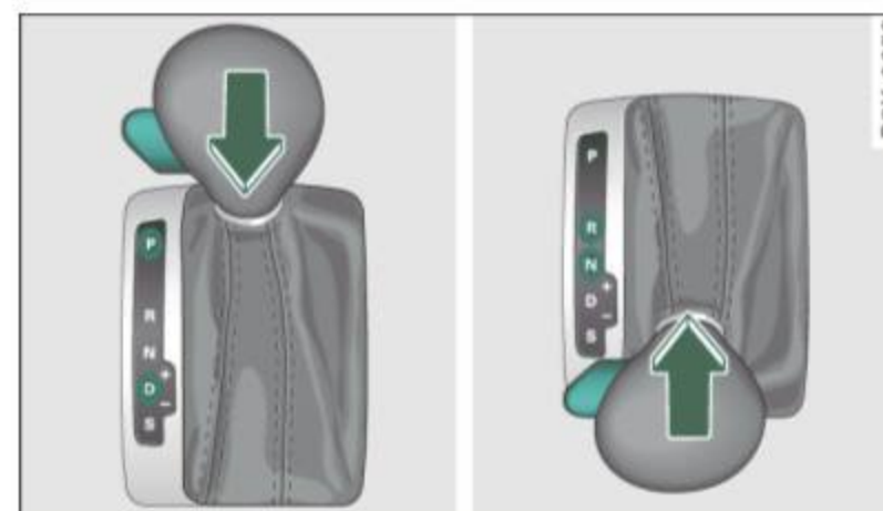
Fig. 155 Shift gate: selector lever lock positions and interlock button highlighted
