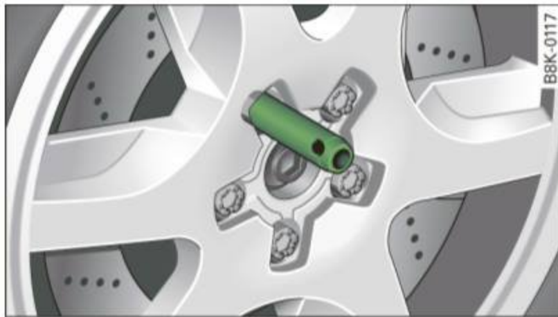
Fig. 234 Changing a wheel: alignment pin inside the top hole
