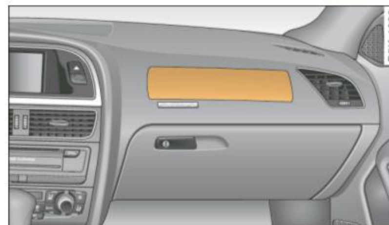
Fig. 187 Location of front passenger's airbag: in the instrument panel
