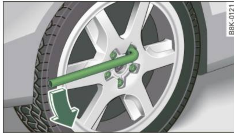
Fig. 230 Changing a wheel: loosening the wheel bolts
