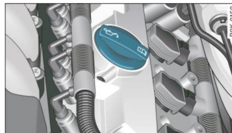
Fig. 214 Engine compartment: Oil filler cap location
