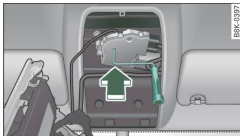
Fig. 49 Section from headliner: Crank for emergency operation
