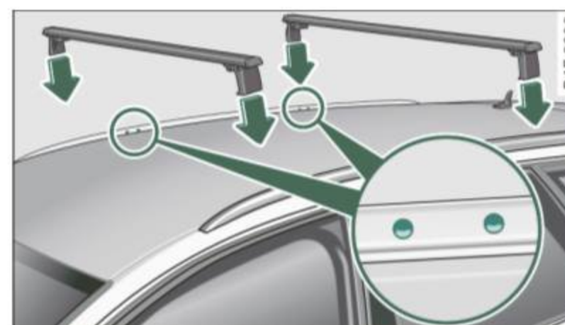
Fig. 96 Roof rails: front and rear mounting locations
