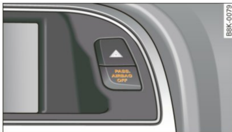
Fig. 189 Section from the instrument panel: PASSENGER AIRBAG OFF light
