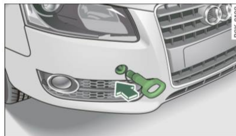
Fig. 242 Front bumper: screwing in the towing loop
