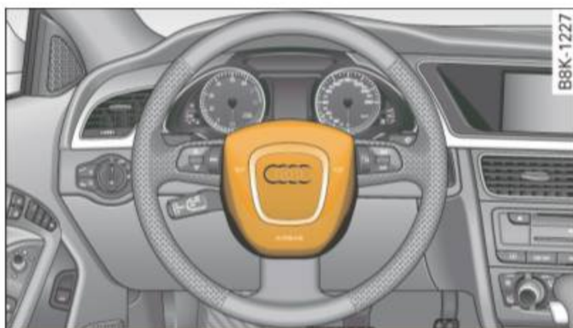
Fig. 186 Location of driver airbag: in steering wheel
