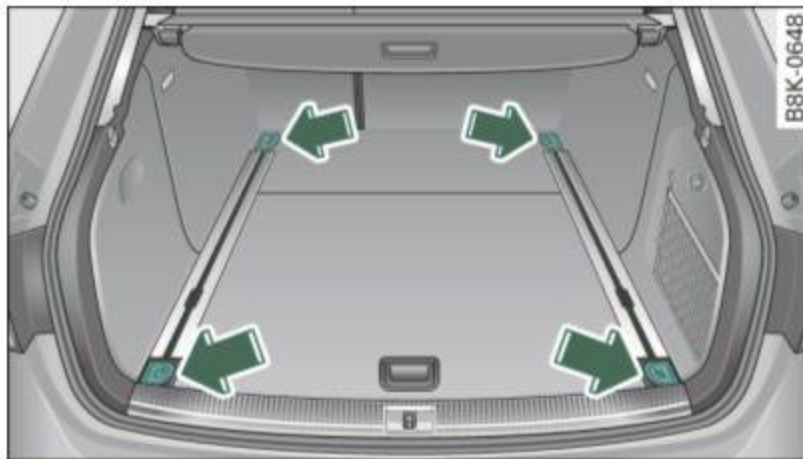
Fig. 78 Location of the fastening eyes in the luggage compartment
