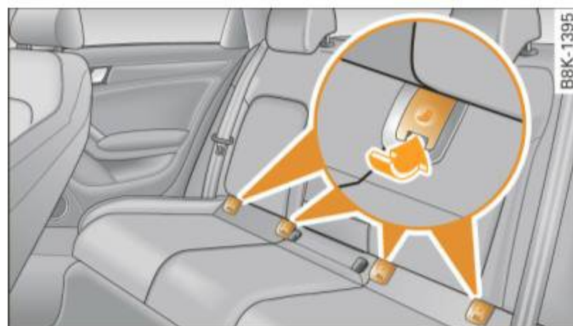
Fig. 199 Lower anchorages, covers marked
