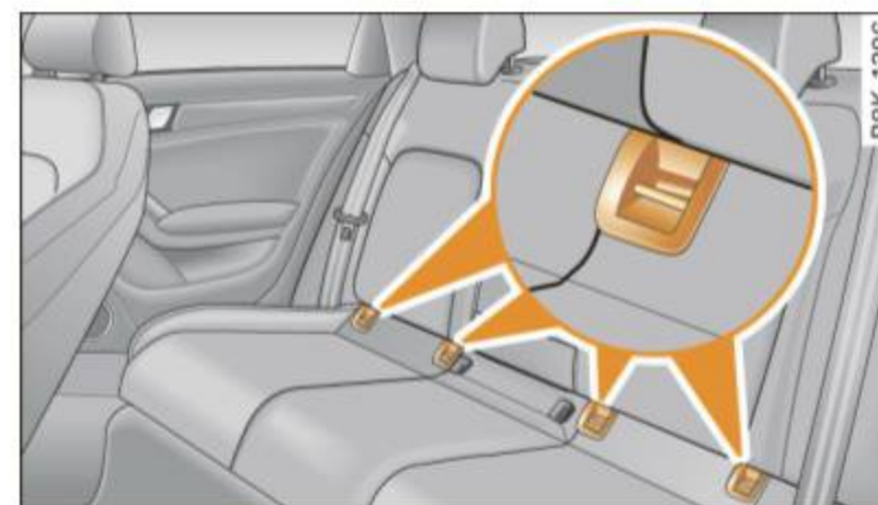
Fig. 200 Rear seats: lower anchorage bracket locations
