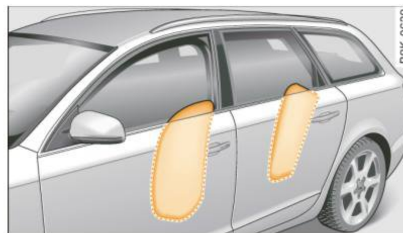
Fig. 191 Inflated side airbags on left side of vehicle
