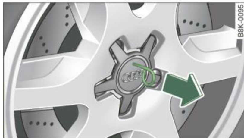
Fig. 228 Changing a wheel: removing the wheel cover
