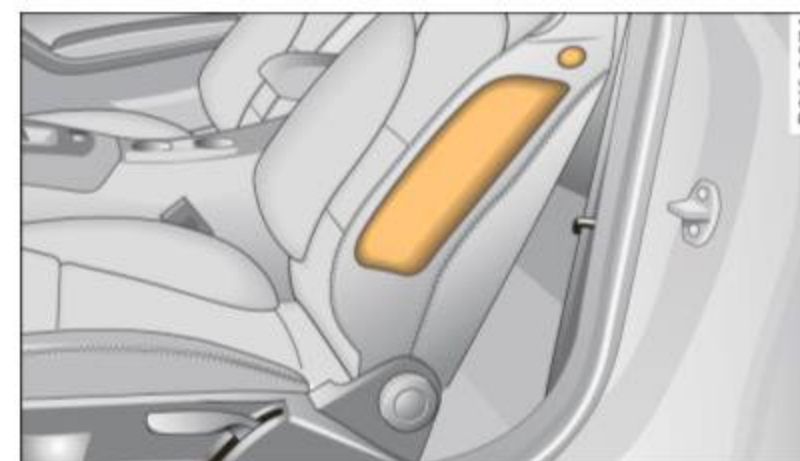
Fig. 190 Side airbag location in the driver's seat
