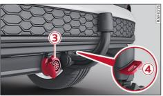
Fig. 103 Area below rear bumper: Connecting socket (3), eye for breakaway cable (4)
