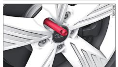
**Fig. 202** Wheel: Mounting pin in wheel bolt hole nearest to the top
