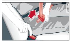
$\begin{tabular}{ll} \textbf{Fig. 56} & \textbf{The latch plate of the belt springs out of the buckle} \\ \textbf{le} & \end{tabular}$
