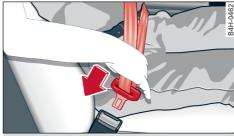
Fig. 55 Latch plate and buckle
