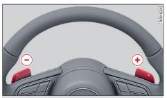
Fig. 81 Steering wheel: Paddle levers\*
