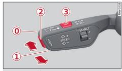
Fig. 121 Control lever: Operating adaptive cruise assist
