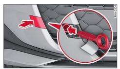
Fig. 205 Front bumper: Fitting the towline anchorage
