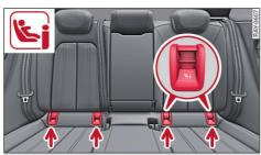
Fig. 62 Rear seat: Bottom ISOFIX anchorages
