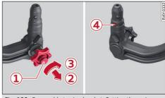
**Fig. 100** Removable towing bracket: Setting the spring mechanism to the "ready" position
