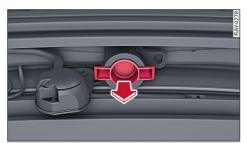
Fig. 98 Area below rear bumper: Pulling out plug
