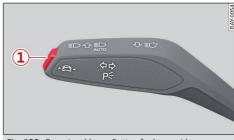
Fig. 123 Turn signal lever: Button for lane guidance
