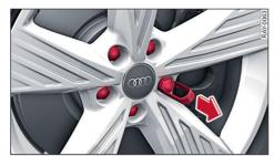
Fig. 196 Wheel: Wheel bolts with caps
