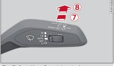
Fig. 43 Control lever: Rear window wiper\*
