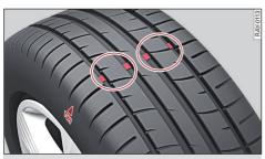
Fig. 185 Tyre tread: Tread wear indicators
