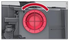
Fig. 213 Headlight: Cover for turn signal
