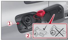
Fig. 169 Fuel tank flap with tank cap attached
