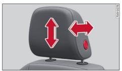
Fig. 51 Front seat: Adjusting head restraint
