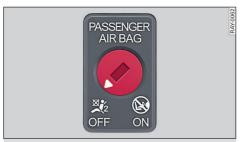
**Fig. 59** Glove box: Key-operated switch for deactivating front passenger's airbag
