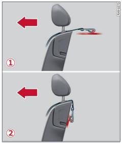
**Fig. 65** Version 1 rear shelf / version 2 rear backrest: Hooking strap into top tether anchorage
