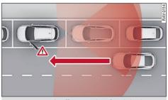
Fig. 137 Detected traffic approaching from behind
