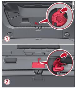
Fig. 30 Inside of boot lid: Access to manual release. ① Saloon, ② Sportback
