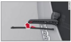
Fig. 45 Rear window wiper: Attaching the wiper blade
