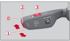
Fig. 128 Control lever: Operating adaptive cruise assist
