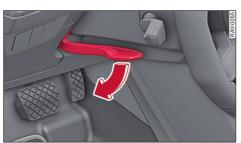
**Fig. 49** Steering column: Lever for adjusting the steering wheel position
