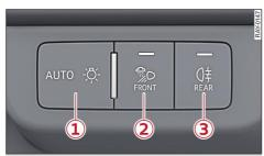
Fig. 35 Dashboard: Light switch module
