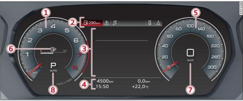
Fig. 2 Overview of Audi virtual cockpit plus
