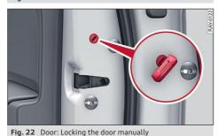
Applies to vehicles with anti-theft alarm system: Switch on the ignition or press the  $\widehat{\Box}$  button on the vehicle key after opening the driver's door manually. Otherwise the alarm will be triggered. The anti-theft alarm system is not activated when the doors are locked manually.
