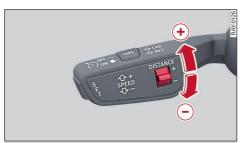
Fig. 127 Control lever: Setting the distance
