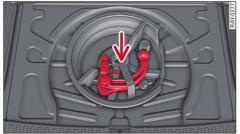
Fig. 97 Luggage compartment: Stowing the towing brack-
