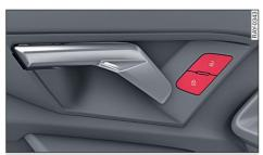
Fig. 20 Driver's door: Central locking switch
