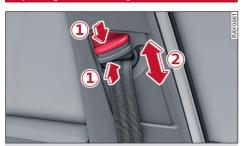
**Fig. 57** Belt height adjustment for the front seats: guide fitting
