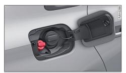
**Fig. 170** Vehicle as seen from the rear right: Unscrewing the AdBlue cap
