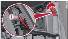
Fig. 88 Engine compartment: Manual release for charging connector
