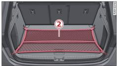
Fig. 72 Luggage compartment: Stretch net\* attached
