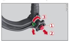
Fig. 104 Removable towing bracket: Removing the ball joint
