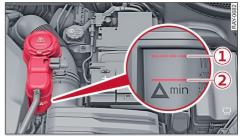
**Fig. 180** Engine compartment: Coolant expansion tank for high-voltage system
