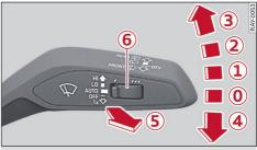
Fig. 42 Control lever: Windscreen wipers
