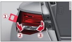
Fig. 217 Side panel: Removing rear light
