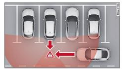
**Fig. 143** Areas covered by sensors for rear cross-traffic assist
