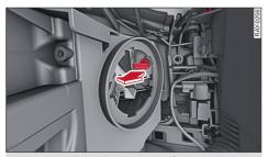
Fig. 214 Headlight: Plastic connector for turn signal
