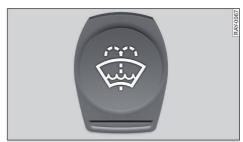
Fig. 184 Engine compartment: Cap of windscreen washer container
