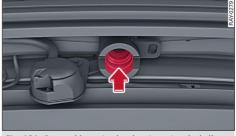
**Fig. 101** Removable towing bracket: Inserting the ball joint
