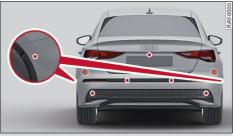
Fig. 111 Rear area: Sensors and cameras
