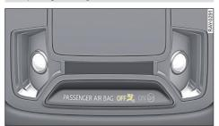
**Fig. 60** Headliner: Indicator lamp for status of front passenger's airbag
