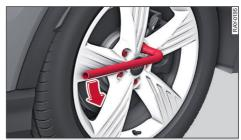
Fig. 198 Wheel: Loosening the wheel bolts
