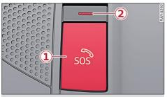
Fig. 152 Front headliner: Cover for emergency call button
