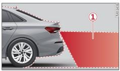
Fig. 109 Area covered by reversing camera
