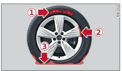
Fig. 192 Tyres: Irreparable tyre damage
