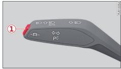
Fig. 133 Turn signal lever: Button for lane departure warning and lane guidance function of adaptive cruise assist\*
