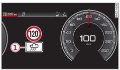
Fig. 114 Instrument cluster: Traffic sign recognition
