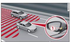
Fig. 136 Driving situation and warning signal on exterior mirror
