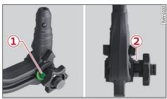
Fig. 102 Removable towing bracket: Safety check
