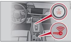
Fig. 79 Centre console: Starting the engine
