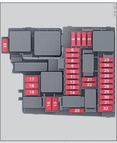
Fig. 210 Engine compartment (left-side): Fuse layout
