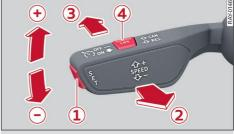
Fig. 116 Control lever: Switching the system on
