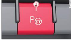
Fig. 146 Centre console: assisted parking button
