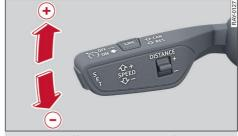
Fig. 122 Control lever: Setting a new speed
