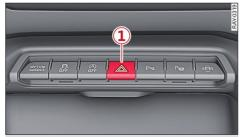
Fig. 37 Centre console: Hazard warning lights
