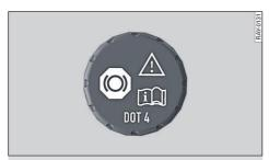
Fig. 181 Engine compartment: Cap of brake fluid reservoir
