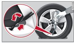
Fig. 193 Tyres: Filling the tyre
