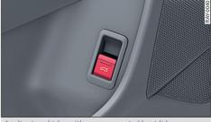
Applies to vehicles with power-operated boot lid: Fig. 27 Driver's door: Opening boot lid
