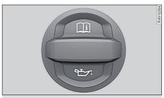
Fig. 178 Engine compartment: Engine oil filler cap (example)
