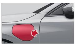
**Fig. 86** Front left side of vehicle: Opening high-voltage charging flap
