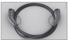
**Fig. 92** Charging cable for public charging stations with AC power (example)
