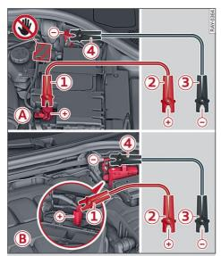
**Fig. 158** Engine compartment: connections for a charger or a jump start cable: (A) vehicles with battery in the engine compartment, (B) vehicles with jump start connection (+) in the engine compartment
