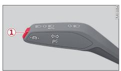
Fig. 89 Turn signal lever: lane guidance button
