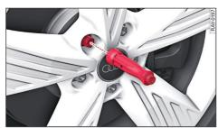
Fig. 155 Wheel: internal hex socket to turn the wheel holts
