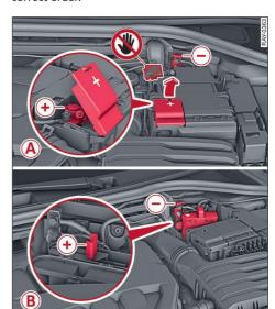
**Fig. 157** Engine compartment: connections for a charger or a jump start cable: (a) vehicles with battery in the engine compartment, (b) vehicles with jump start connection (+) in the engine compartment
