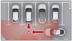
Fig. 105 Sensor detection range for rear cross-traffic assist
