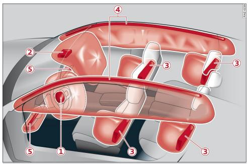
Fig. 58 Airbag overview image (deployment area/deployed airbags)
