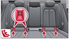
Fig. 60 Rear bench seat: lower LATCH anchors
