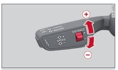
Fig. 92 Lever: setting the distance
