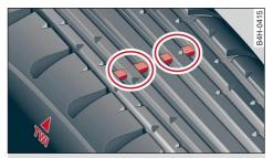
Fig. 143 Tire profile: treadwear indicator
