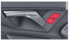
Fig. 20 Driver's door: central locking switch
