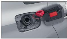
Fig. 129 Fuel filler door with attached fuel cap
