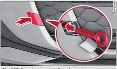
Fig. 159 Front bumper: installing the towing eye
