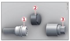
Fig. 151 Anti-theft wheel bolt with cap and adapter
