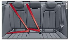
Fig. 63 Rear bench seat: securing unused safety belts
