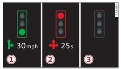
Fig. 81 Instrument cluster: traffic light information display
