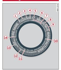
**Fig. 142** Tire designations on the sidewall
