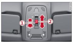
Fig. 34 Headliner: panoramic glass roof button
