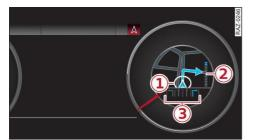
Fig. 119 Instrument cluster: default view: turning maneuver when route guidance has started
