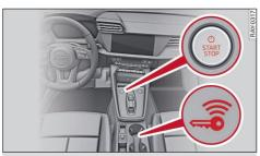
Fig. 71 Center console: starting the engine
