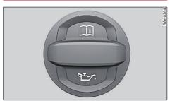
**Fig. 136** Engine compartment: engine oil filling opening cover (example)
