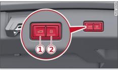
Fig. 28 Luggage compartment lid: (1) closing button\*, (2) lock button\* (vehicles with convenience key\*)
