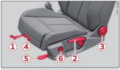
Fig. 46 Front seat: adjusting the seat
