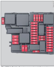
**Fig. 164** Left side of engine compartment: fuse assignment
