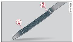
Fig. 134 Oil dipstick (example): checking the engine oil level
