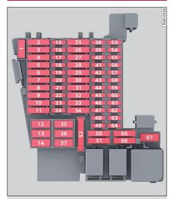
Fig. 163 Left side of cockpit: fuse assignment
