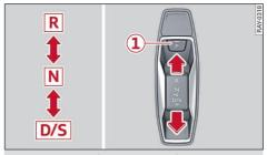
Fig. 72 Center console: transmission selector
