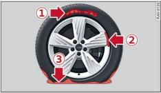
Fig. 147 Tire: tire damage that cannot be repaired
