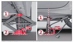
Fig. 154 Sill: positioning the vehicle jack
