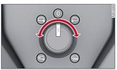
Fig. 40 Driver's door: knob for the exterior mirrors
