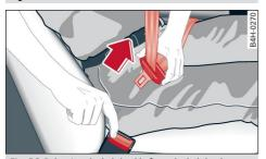
$\textbf{Fig. 56} \ \ \text{Releasing the belt buckle from the belt latch}$
