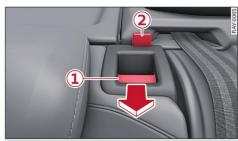
Fig. 65 Outer backrest: release lever and latching indicator with red marking
