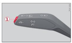
Fig. 97 Turn signal lever: button for lane departure warning and lane guidance for adaptive cruise assist\*
