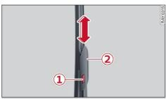
Fig. 43 Windshield wipers: replacing the wiper blades
