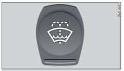
Fig. 141 Engine compartment: washer fluid reservoir cap
