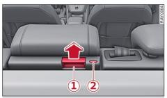
**Fig. 66** Center backrest: release lever and latching indicator with red marking
