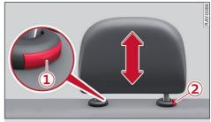
Fig. 52 Rear seat: adjusting or removing the head restraint
