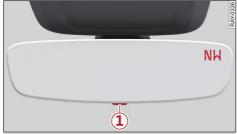
Fig. 44 Rearview mirror: digital compass is turned on
