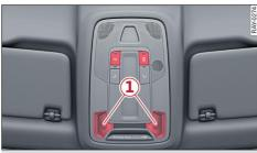
Fig. 38 Headliner: front interior lighting
