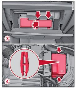
**Fig. 162** Glove compartment (right-hand drive): cover (3); left side of engine compartment: cover (4)
