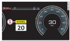
Fig. 80 Instrument cluster: traffic sign recognition
