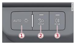
Fig. 35 Instrument panel: light button module
