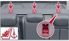
Fig. 61 Rear shelf: top tether anchors to secure a child safety seat with an upper belt
