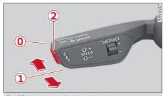
Fig. 87 Lever: using adaptive cruise assist
