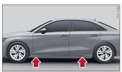
Fig. 153 Sill panels: markings
