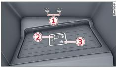
Fig. 110 Front center console: Audi phone box with connections
