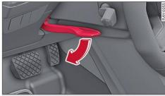
**Fig. 49** Steering column: lever for adjusting the steering wheel position
