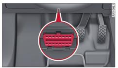
Fig. 165 Driver's side footwell: connection port for the On Board Diagnostic System (OBD)
