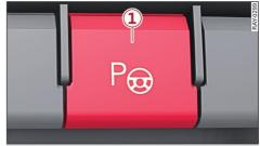
Fig. 108 Center console: button for assisted parking
