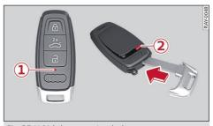
Fig. 25 Vehicle key: removing the battery cover
