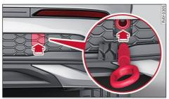
Fig. 160 Rear bumper: installing the towing eye
