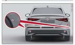
Fig. 77 Rear area: sensors and cameras
