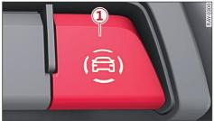
Fig. 78 Center console: driver assistance systems button
