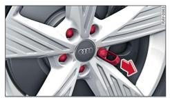
Fig. 150 Wheel: wheel bolts with caps
