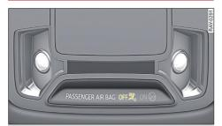
**Fig. 59** Headliner: indicator light to display the status of the front passenger's airbag
