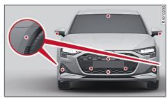
Fig. 76 Front area: sensors and cameras
