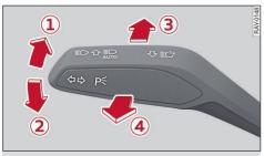
Fig. 36 Lever: turning the light functions on or off
