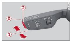
Fig. 93 Lever: using adaptive cruise assist
