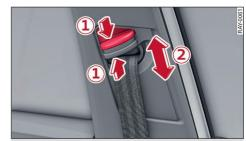
Fig. 57 Belt height adjustment for the front seats - safety belt relay
