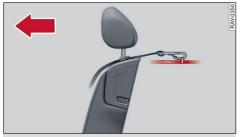
Fig. 62 Rear shelf: securing the upper belt to the top tether anchor
