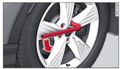
Fig. 152 Wheel: loosening the wheel bolts
