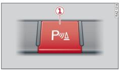
Fig. 132 Centre console: Button for parking aid
