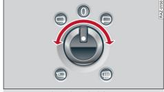
Fig. 41 Driver's door: Adjuster knob for exterior mirrors
