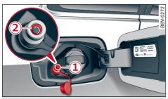
Fig. 163 Tank flap open: Gas filler neck 1 and filler neck seal 2
