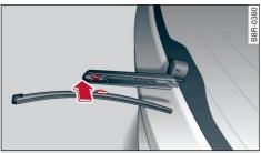
Fig. 46 Rear window wiper: Attaching the wiper blade
