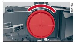
Fig. 202 Headlight: Cover for turn signal
