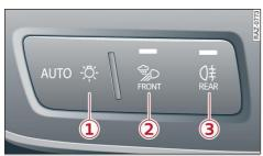
Fig. 36 Dashboard: Light switch module
