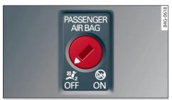
**Fig. 60** Glove box: Key-operated switch for deactivating front passenger's airbag
