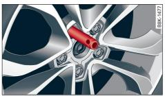
**Fig. 190** Wheel: Mounting pin in wheel bolt hole nearest to the top
