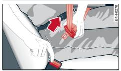
Fig. 57 The latch plate of the belt springs out of the buck-
