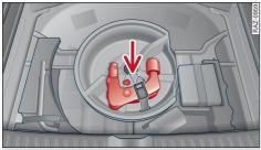
Fig. 94 Luggage compartment: Stowing the towing bracket
