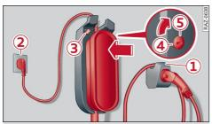
Fig. 93 Clip wall mount: Hooking in Audi charging system
