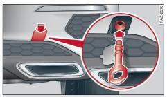
**Fig. 195** Rear bumper: Fitting the towline anchorage (version 2)
