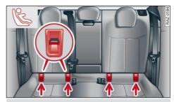
Fig. 63 Rear seat: Bottom ISOFIX anchorages
