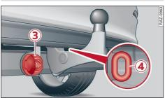
Fig. 100 Rear bumper: Socket and eye for safety cable
