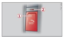
Fig. 144 Front headliner: Cover for emergency call button
