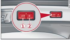
Fig. 29 Boot lid: (1) close button\*, (2) lock button\* (vehicles with convenience key\*)
