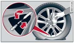
Fig. 183 Tyres: Filling the tyre
