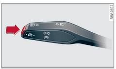
Fig. 117 Turn signal lever: Button for lane guidance and lane departure warning
