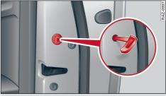
Fig. 24 Door: Locking the door manually
