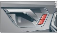
Fig. 22 Driver's door: Central locking switch
