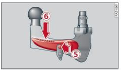
**Fig. 96** Removable towing bracket: Setting the spring mechanism to the "ready" position
