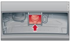
Fig. 98 Area below rear bumper: Inserting ball joint
