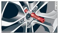
Fig. 189 Wheel: Hexagonal socket for turning wheel bolts
