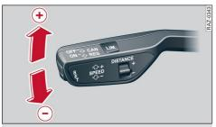
Fig. 116 Control lever: Setting a new speed
