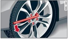
Fig. 186 Wheel: Loosening the wheel bolts
