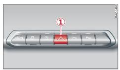
Fig. 38 Centre console: Hazard warning lights
