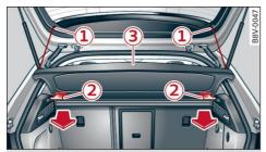
**Fig. 68** Luggage compartment: Removing and installing luggage compartment cover
