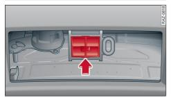
Fig. 102 Area below rear bumper: Fitting the plug
