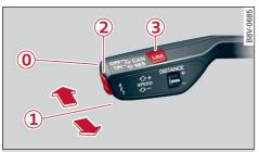
Fig. 115 Control lever: Operating adaptive cruise assist
