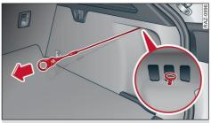
Fig. 164 Right-hand side trim in luggage compartment: Releasing tank flap manually
