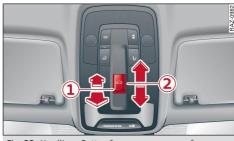
Fig. 35 Headliner: Button for panorama sun roof
