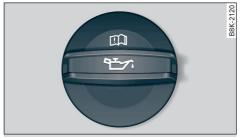
Fig. 171 Engine compartment: Engine oil filler cap (example)
