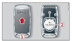
Fig. 79 Remote control: Changing battery
