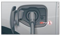
**Fig. 86** Charging unit: Charging connection and charging indicator
