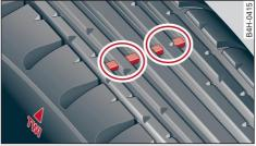
Fig. 176 Tyre tread: Tread wear indicators
