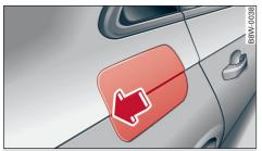
Fig. 162 Vehicle as seen from the rear right: Opening the fuel tank flap
