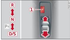
Fig. 81 Centre console: Selector lever
