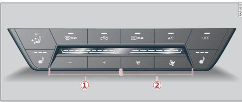
Fig. 76 Manual air conditioner: Controls
