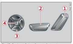
Fig. 48 Front seat: Buttons for seat adjustment
