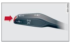
Fig. 126 Turn signal lever: Button for lane guidance and lane departure warning
