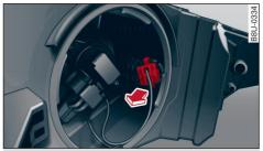
Fig. 203 Headlight: Plastic connector for turn signal
