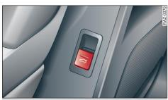
Applies to vehicles with power-operated boot lid: Fig. 28 Driver's door: Opening boot lid
