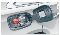
Fig. 165 Vehicle as seen from the rear right: Unscrewing the AdBlue cap
