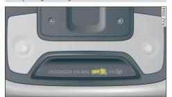
**Fig. 61** Headliner: Indicator lamp for status of front passenger's airbag
