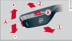
Fig. 110 Operating lever: Switching the system on
