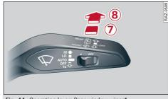
Fig. 44 Operating lever: Rear window wiper\*
