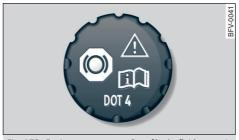
Fig. 173 Engine compartment: Cap of brake fluid reservoir
