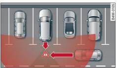
**Fig. 136** Areas covered by sensors for rear cross-traffic assist
