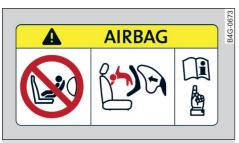
Fig. 62 Passenger's sun visor: Airbag sticker
