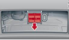
Fig. 97 Area below rear bumper: Pulling out plug
