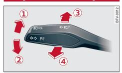
Fig. 37 Control lever: Switching light functions on/off
