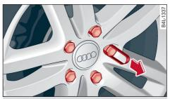
Fig. 184 Wheel: Wheel bolts with caps
