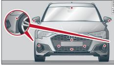
Fig. 106 Front area: Sensors and cameras
