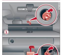
Fig. 31 Inside of boot lid: Access to manual release
