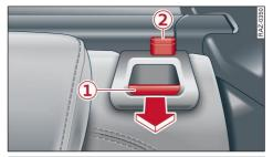
**Fig. 69** Outer backrest: Release lever and backrest lock indicator with red marking
