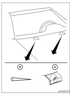
If you wax the surface of the hood, be careful not to let wax get into the washer nozzle (a). This may cause clogging or improper windshield-washer operation. If wax gets into the nozzle, remove it with a needle or small pin (b).
