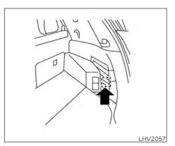
An air vent is located on the right hand side of the luggage room to cool the Li-ion battery and DC/DC converter. If the vent is covered, the battery will overheat resulting in reduced output performance of the hybrid system. For additional information, refer to "Lithium-ion (Li-ion) battery air vent" in the "Appearance and care" section of this manual.
