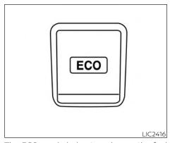
The ECO mode helps to enhance the fuel economy by controlling the throttle sensitivity and transmission points.
