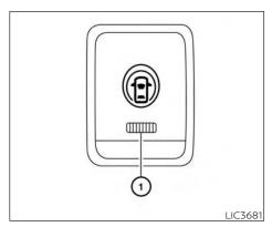
The dynamic driver assistance switch is used to temporarily turn on and off the Intelligent Lane Intervention (I-LI) system that is activated using the settings menu of the vehicle information display.
