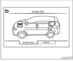
This is an example of the Energy Flow screen. The Energy Flow display changes, depending on the following operating conditions. The graphic indicates the amount of power in the Li-ion battery.
