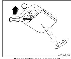
Room light (if so equipped) Use a cloth 1 to protect the housing.
