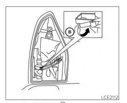
3. Unhook the clip (B) restraining the jack and tool kit.
