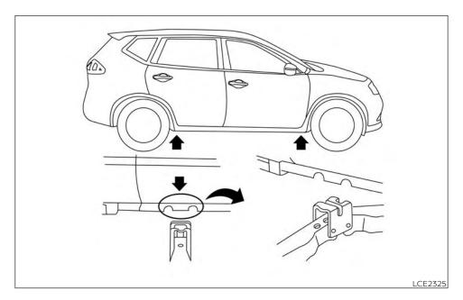
Jacking up vehicle and removing the damaged tire
