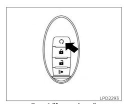
Type A (if so equipped) The  $\Omega$  button will be on the NISSAN Intelligent Key® if the vehicle has Remote Hybrid Start. This feature allows the hybrid system to start from outside the vehicle. The following features may be affected when the remote start feature is used.
