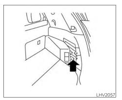
LITHIUM-ION (Li-ion) BATTERY AIR **VENT**
