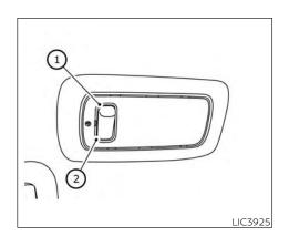
The luggage compartment light on the overhead trim has a two-position switch. To operate, push the switch to the desired position.
