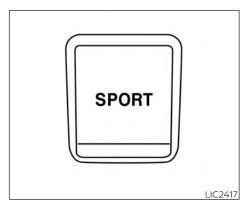
The SPORT mode switch adjusts the engine and transmission points to enhance performance. Push the SPORT mode switch on the instrument panel to activate. The SPORT mode indicator light appears in the meter.
