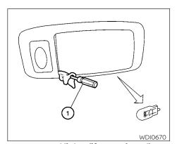
Personal lights (if so equipped) Use a cloth and a suitable tool 1 to protect the housing.
