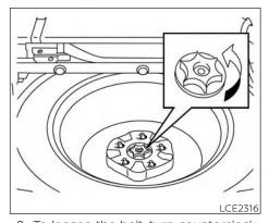
8. To loosen the bolt, turn counterclockwise.
