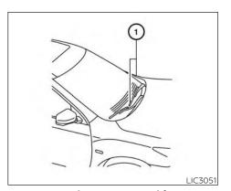
Be sure you do not put anything on top of the autolight sensor located in the top side (1) of the instrument panel. The autolight sensor controls the autolight; if it is covered, the autolight sensor reacts as if it is dark out and the headlights will illuminate. If this occurs while parked with the engine off and the ignition switch placed in the ON position, your vehicle's 12-volt battery could become discharged.
