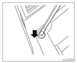
7. Use the slotted end of the jack tool to remove the clips that are holding the floor board in place by pressing the center pin downwards.
