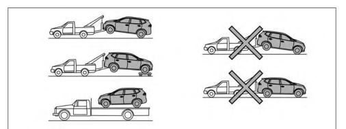
Front-Wheel Drive (FWD) models with Continuously Variable Transmission (CVT)
