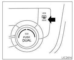
To defrost the rear window glass and outside mirrors start the hybrid system and push the rear window defroster switch on. The rear window defroster indicator light on the switch comes on Push the switch again to turn the defroster off.
