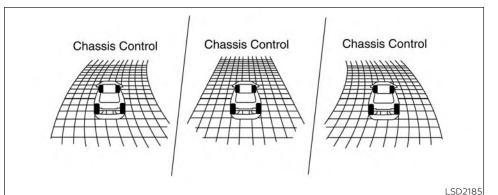
When the I-EB is operated at corners and the "Chassis Control" mode is selected in the vehicle information display, the I-EB graphics are shown in the vehicle information display. For additional information, refer to "Vehicle information display" in the "Instruments and controls" section of this manual
