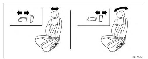
FRONT POWER SEAT ADJUSTMENT (for driver's seat)
