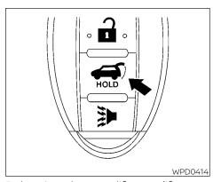
Releasing the rear liftgate (if so equipped)
