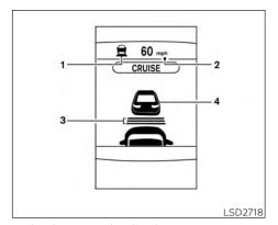
Vehicle-to-vehicle distance control mode display and indicators
