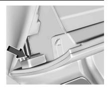
Push the dampener arm to the left until it releases the glove box.
