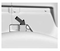
Pull the emergency manual charge cord release handle. The DC charge cord will release.
