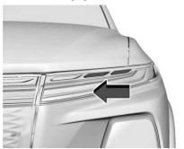
The headlight Charge Status Indicator bar is located on the headlights. As charging occurs, the blue light bars on the headlights fill towards the center of the vehicle.
