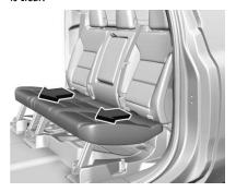
Pull the strap on the rear edge of the rear seat cushion to release the cushion. Tilt the seat cushion forward toward the front of the vehicle.
