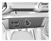
To open the glove box, pull the handle to the left. Use the mechanical key to lock or unlock. See Keys \$ 8.
