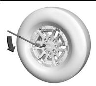
Turn the wheel wrench counterclockwise to loosen all the wheel nuts, but do not remove them yet.
