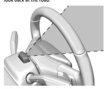
Sunglasses, hats, or other types of clothing that change the shape of the head may interfere with camera performance. To improve camera performance, raise or lower the steering wheel, or change the seat position.
