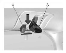
Squeeze and pull down the glass latch levers (A), located near the upper corners of the rear glass, to unlatch. Once unlatched, the glass-catch release button (C) will catch the rear glass and prevent it from falling forward.
