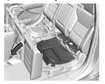
Pull the strap on the rear edge of the seat cushion to release. Tilt the seat cushion forward to access the storage. Rotate the seat bench rearward and push down to close.
