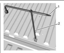
Assembly the wheel wrench (1) and wheel wrench adapter (2), and fit over the hexagon bolt as shown.
