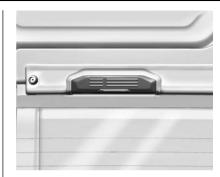
Hold the rear glass in place with one hand and push up on the glass stow retainer handle. You should hear a click sound when the handle is all the way up.
