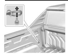
Place the loop end of the flat tire secure strap through the lower cargo tie-down on the driver side of the vehicle. Place the hook end of the strap through the loop and pull it until the strap is fastened securely to the tie-down.
