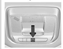
\(\to \): Press this button on the overhead console to make the front and rear turn signal lamps flash on and off. This warns others that you are having trouble. Press again to turn the flashers off.
