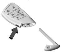
Press the button on the side of the remote key and pull the mechanical key out.
