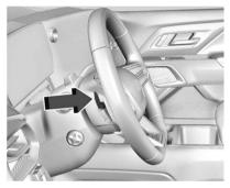
If equipped, Regen on Demand increases deceleration by pressing and holding the steering wheel paddle. Regen on Demand works in D (Drive). The accelerator pedal can be used to manage deceleration while using Regen on Demand. See *One-Pedal Driving*
