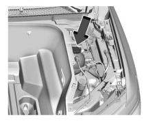
4. After the system has completely cooled, check that the coolant level in the reservoir.
