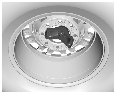
ZR2 Model Incorrectly Stored, Retainer Off-Center
