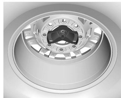
ZR2 Model Correctly Stored, Retainer Centered
