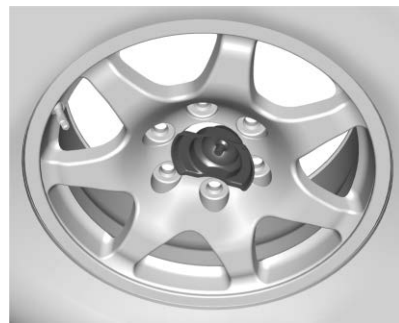
All Other Models Incorrectly Stored, Retainer Off-Center
