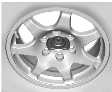
All Other Models Correctly Stored, Retainer Centered
